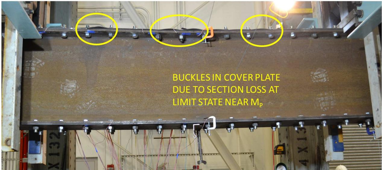
**Figure 1 – Photograph of Specimens 2. Coverplate included simulated section loss but no simulated pack-out. Buckles in the coverplate were due to applied flexural compressive stress in the top flange.**
