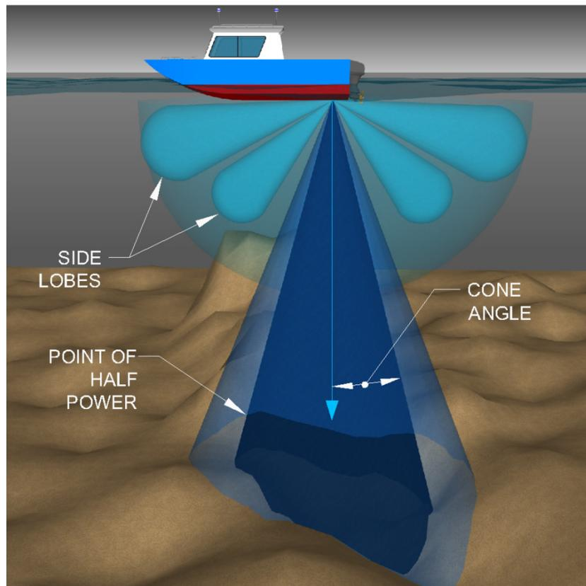
**Figure 2. Graphic. Sonar cone angle and side lobes.**
