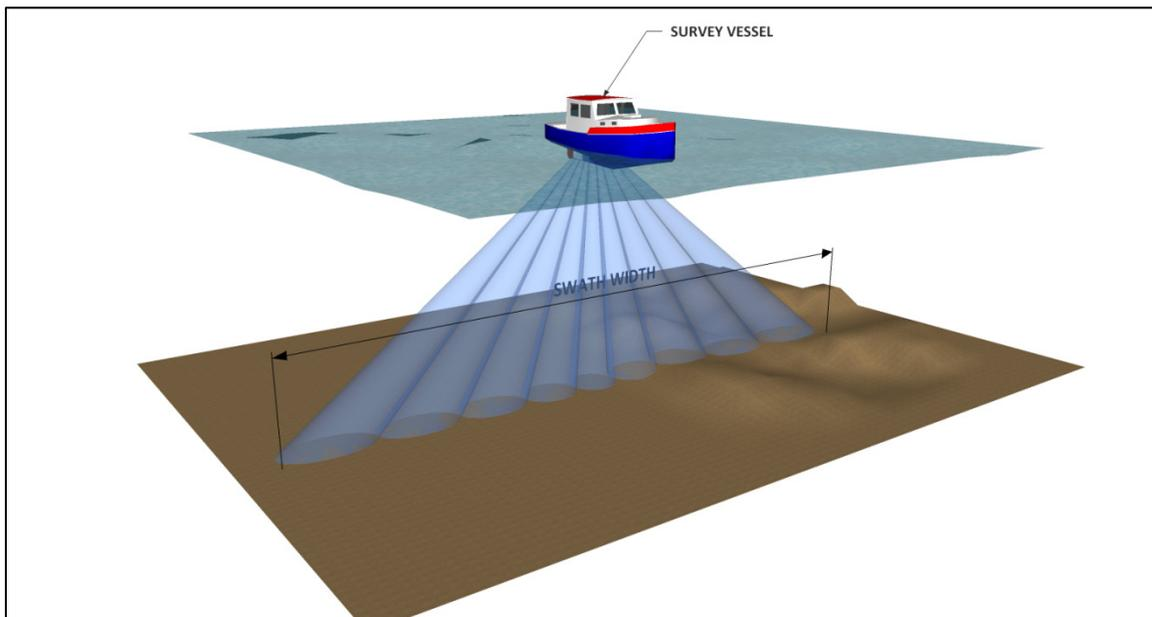
**Figure 8. Graphic. Multibeam swath sonar beam pattern.**
