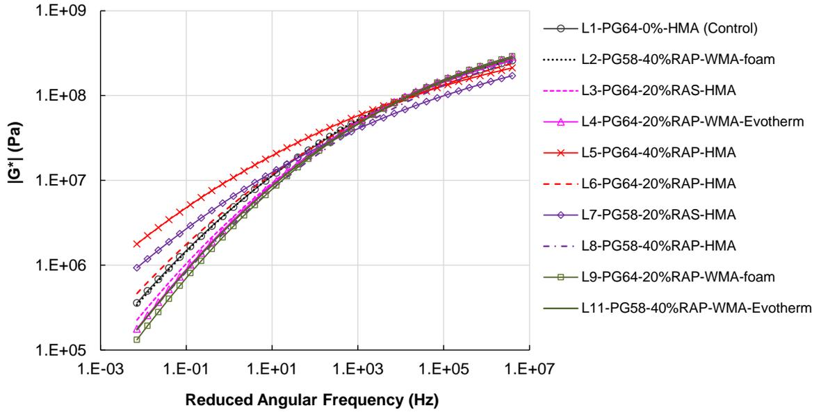
**Figure 28. Dynamic shear modulus master curves for the CO, FL, and LA extracted binders**
