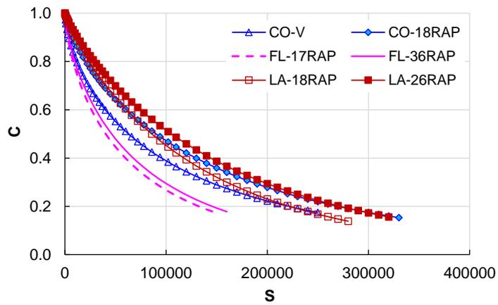
**Figure 10. The MFS parameter from the S-VECD test for all the asphalt mixtures**
