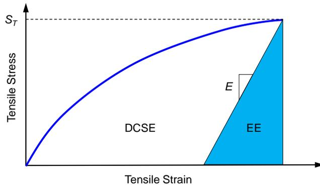
$ER$  is defined as the ratio of  $DCSE$  to the minimum dissipated creep strain energy  $DCSE_{\min}$  that is required to preclude top-down cracking in the pavement:
