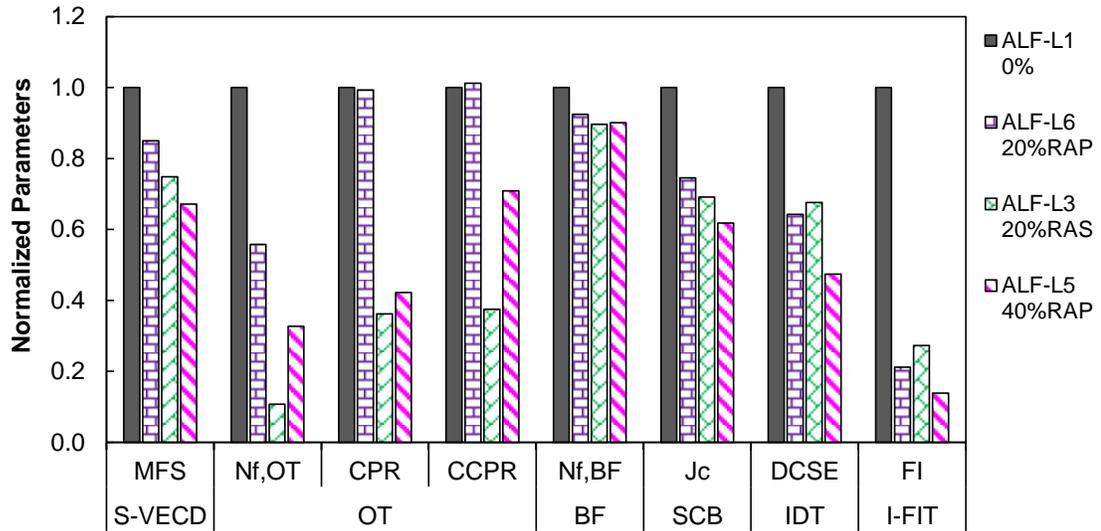
Figure 21. Normalized parameters for evaluating the effect of RAP on the CO, FL, and LA mixtures
