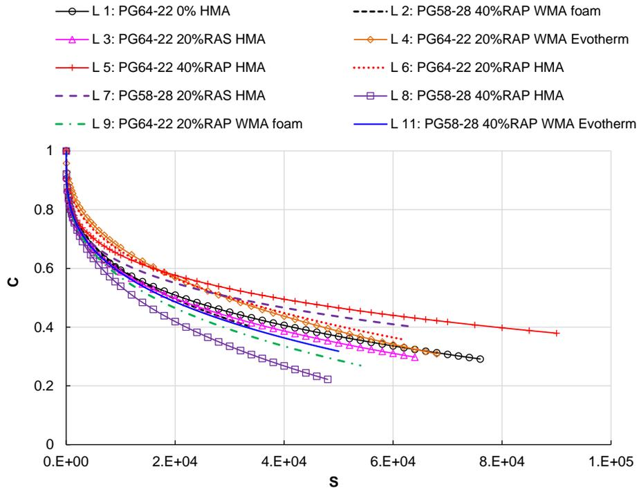
**Figure 31. Damage characteristic curves for the CO, FL, and LA extracted binders**
