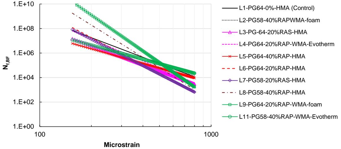
**Figure 15. Relationship of fatigue life  $N_{f,BF}$  versus strain level for the CO, FL, and LA mixtures**
