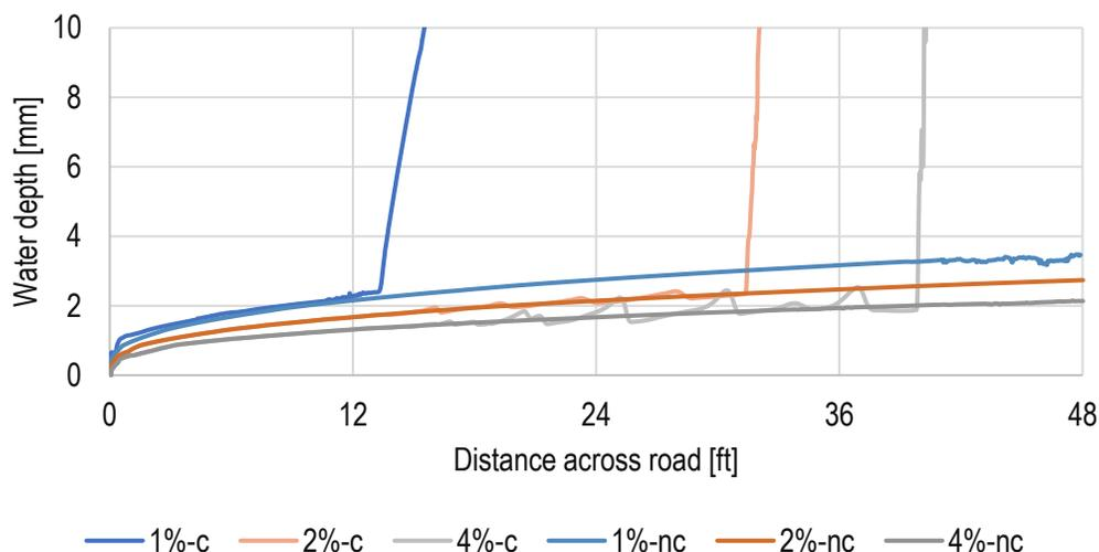
**Figure 7. Water film thickness across a 4-lane roadway with a 4-inch high curb at cross slopes 1%, 2%, and 4%. Rain intensity 10 in/hr. The 'c' is legend is with a curb and 'nc' denotes no curb.**
