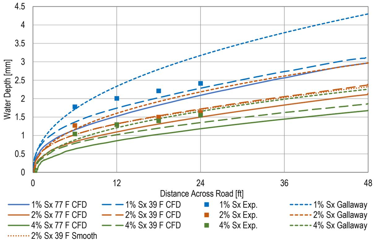
**Figure 2. Water film thickness across the roadway without a curb at cross slopes 1%, 2%, and 4% and rainfall intensity rate approximately 5 in/hr showing comparison with the Galloway equation and experimental results for a near smooth texture depth of 0.076 mm.**
