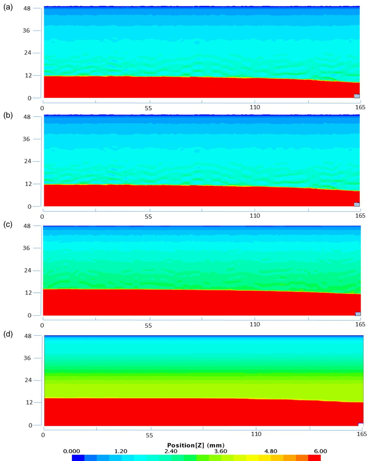
**Figure 4. Water surface on a 4 lane roadway with a curb and drainage, 2% cross slope, no longitudinal slope, and at rain intensity (a) 2 in/hr, (b) 5 in/hr, (c) 10 in/hr, and (d) 20 in/hr (curb overflow). The length scale of the computational domain is in feet.**
