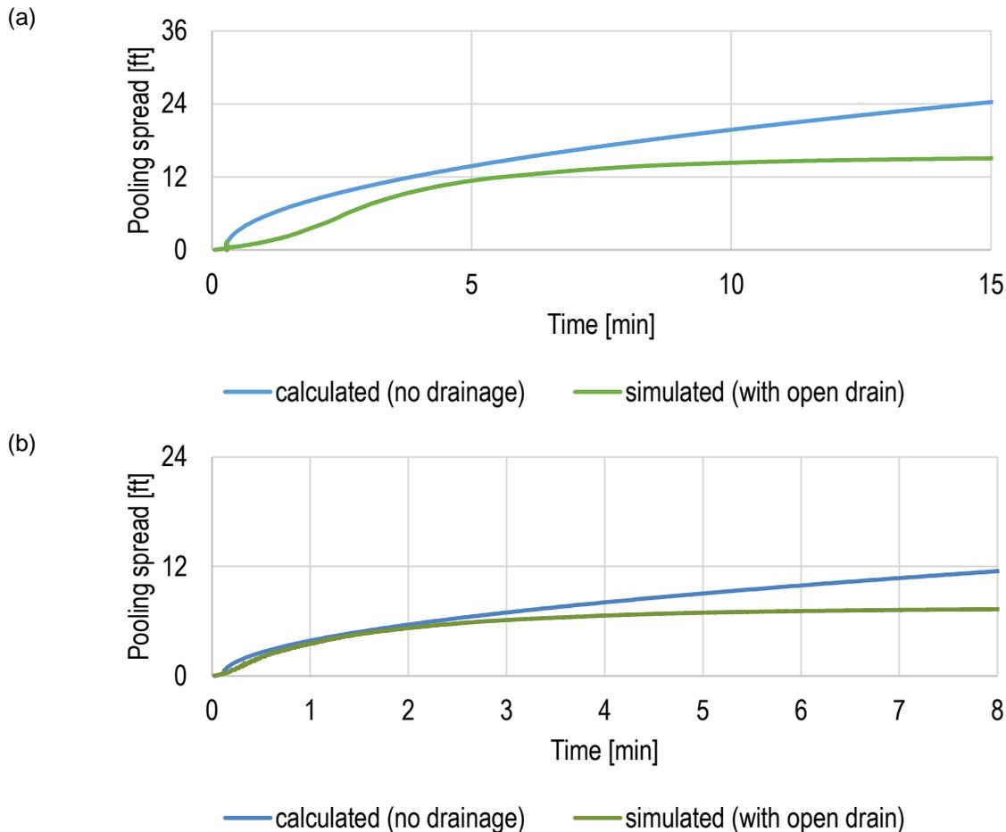
**Figure 5. The development of the pooling spread in time for a case without drainage (debris clogged) and an open drain at 10 in/hr, (a) 1% cross-slope, (b) 4% cross-slope**
