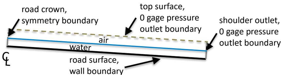
**Figure 1. Diagram of computational domain with boundary conditions for thin strip of road from crown to shoulder.**
