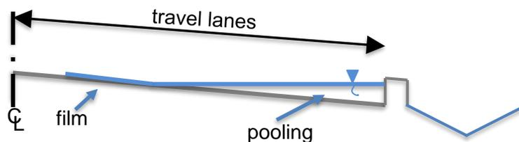
**Figure 6. Diagram showing pool that forms at the curb when drainage is not fast enough.**
