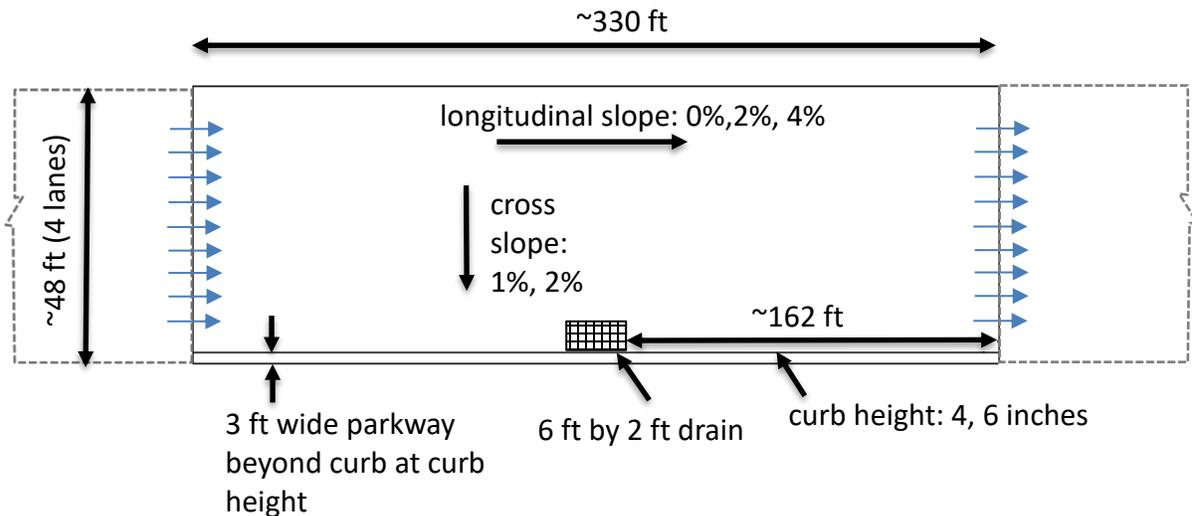
**Figure 3. Top view of the CFD domain with dimensions for road with curb and drainage. Values of the main analysis parameters are shown. The blue arrows mark the inflow and outflow surfaces where the periodic boundary condition was used.**
