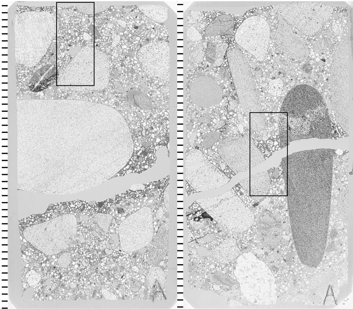
Figure S-12: Transmitted light scanned images of thin sections to show locations of elemental maps. The top of each thin section represents the wear surface of the pavement, the large cracks, sub-parallel to the surface, are at a depth of about 25 mm, (tic marks every mm).
