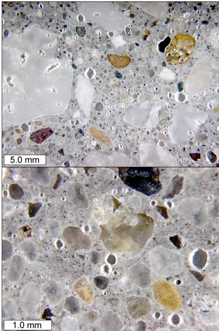
Figure IA-7: Stereo microscope images to show air void structure of concrete overlay on polished slab from core IA-4.
