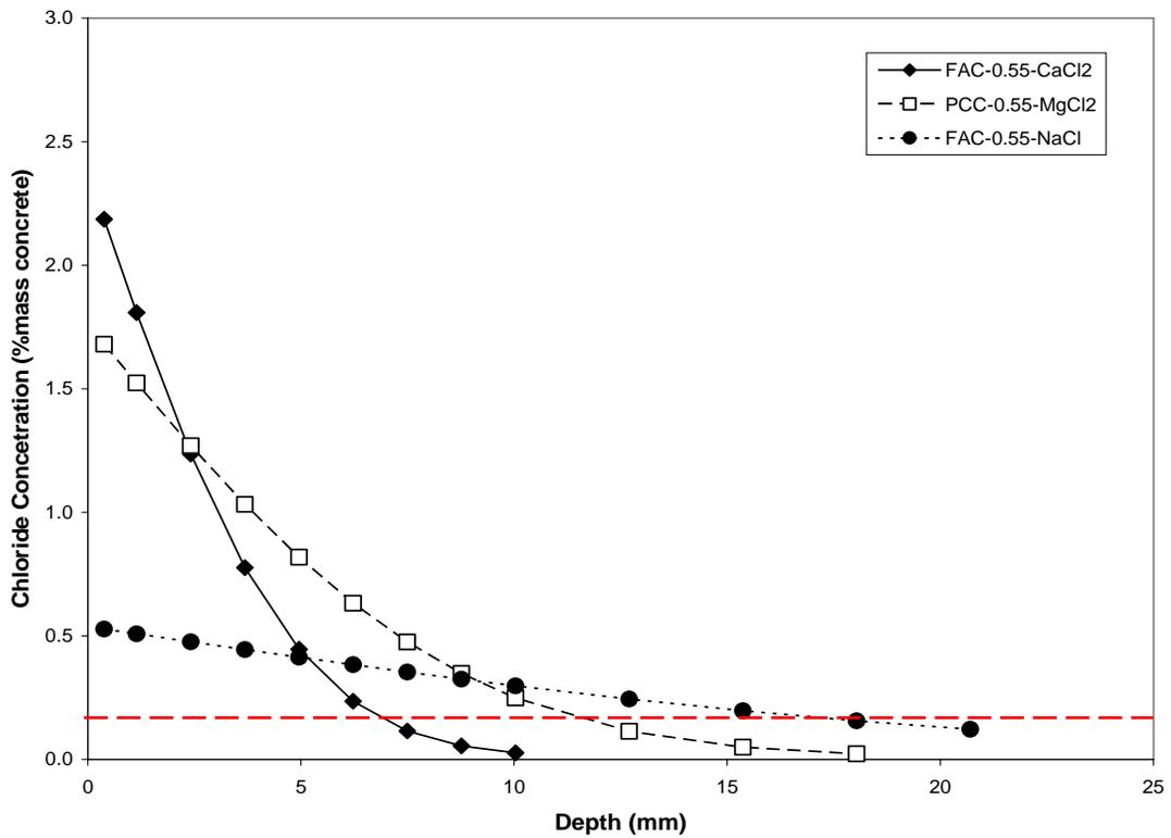
Figure 4. Portland cement + 15% fly ash concrete samples (w/cm=0.55) - chloride profiles for different salts
