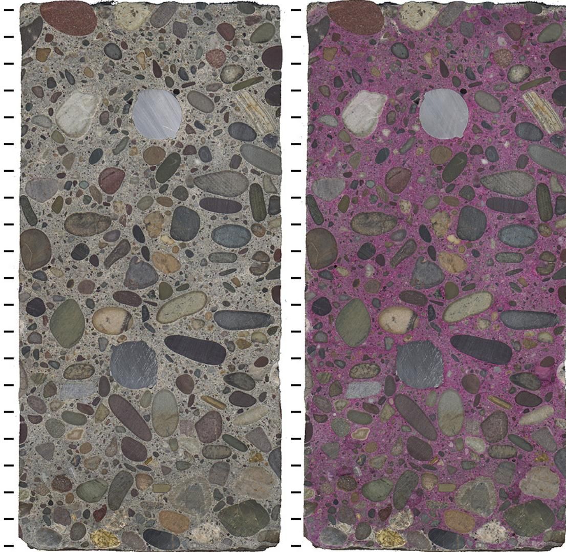
Figure S-5: Polished slabs to show complete cross-section through core S-2 both before (left) and after application of phenolphthalein stain (right) tic marks every cm.
