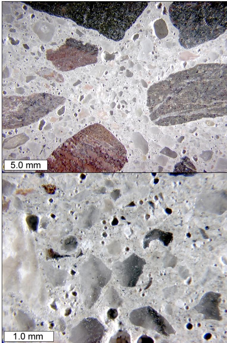
Figure ID-14: Stereo microscope images to show air void structure on polished slab from core IDR-7.
