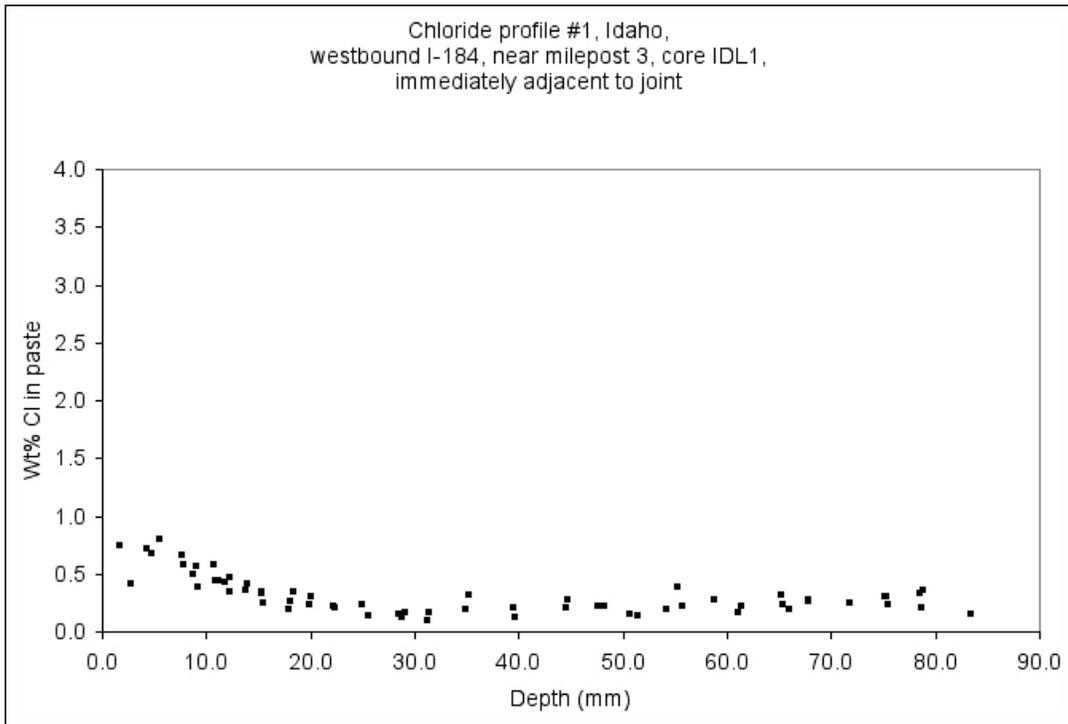
Figure ID-17: Chloride profile through cement paste immediately adjacent to joint, from billet prepared from core IDL-1.
