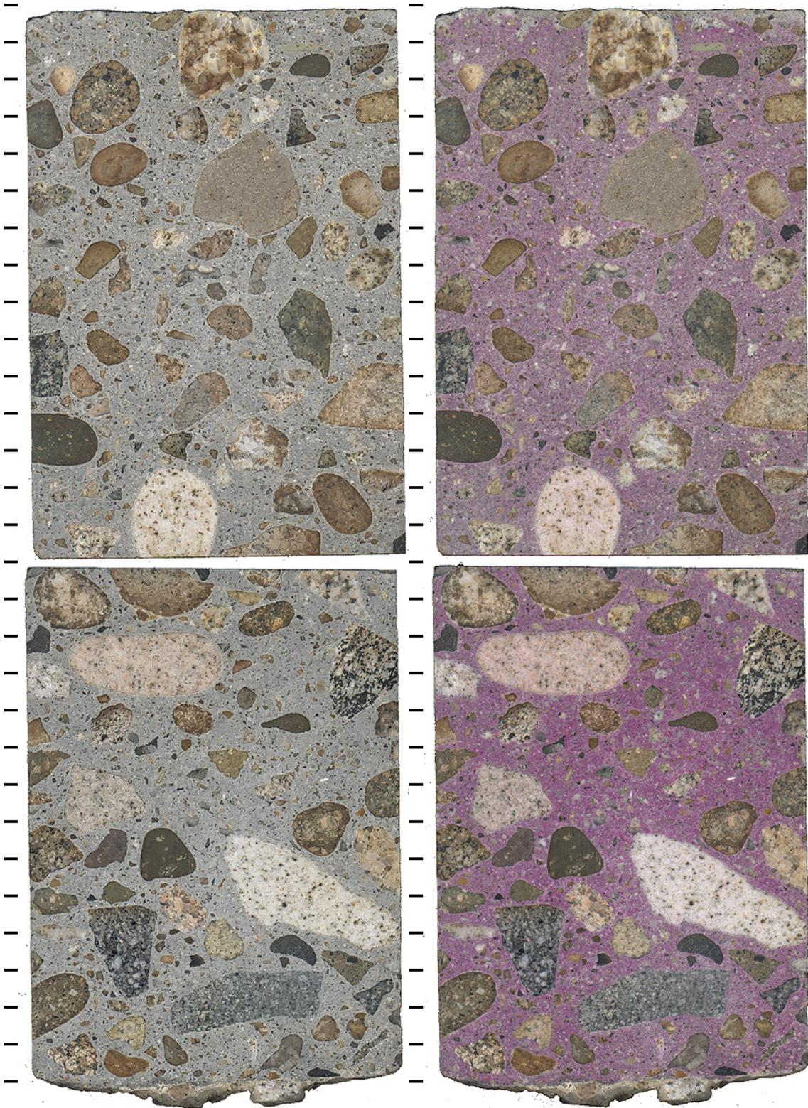
Figure ID-12: Polished slabs to show complete cross-section through core IDR-3 both before (left) and after application of phenolphthalein stain (right) tic marks every cm.
