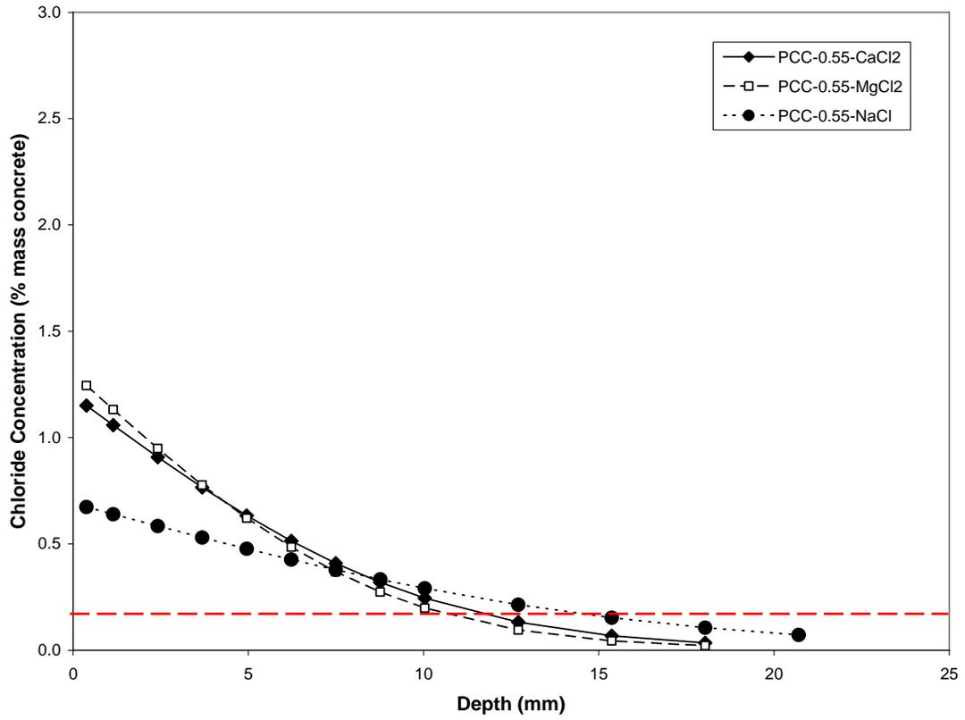
Figure 2. Portland cement concrete samples (w/c=0.55) - chloride profiles for different salts
