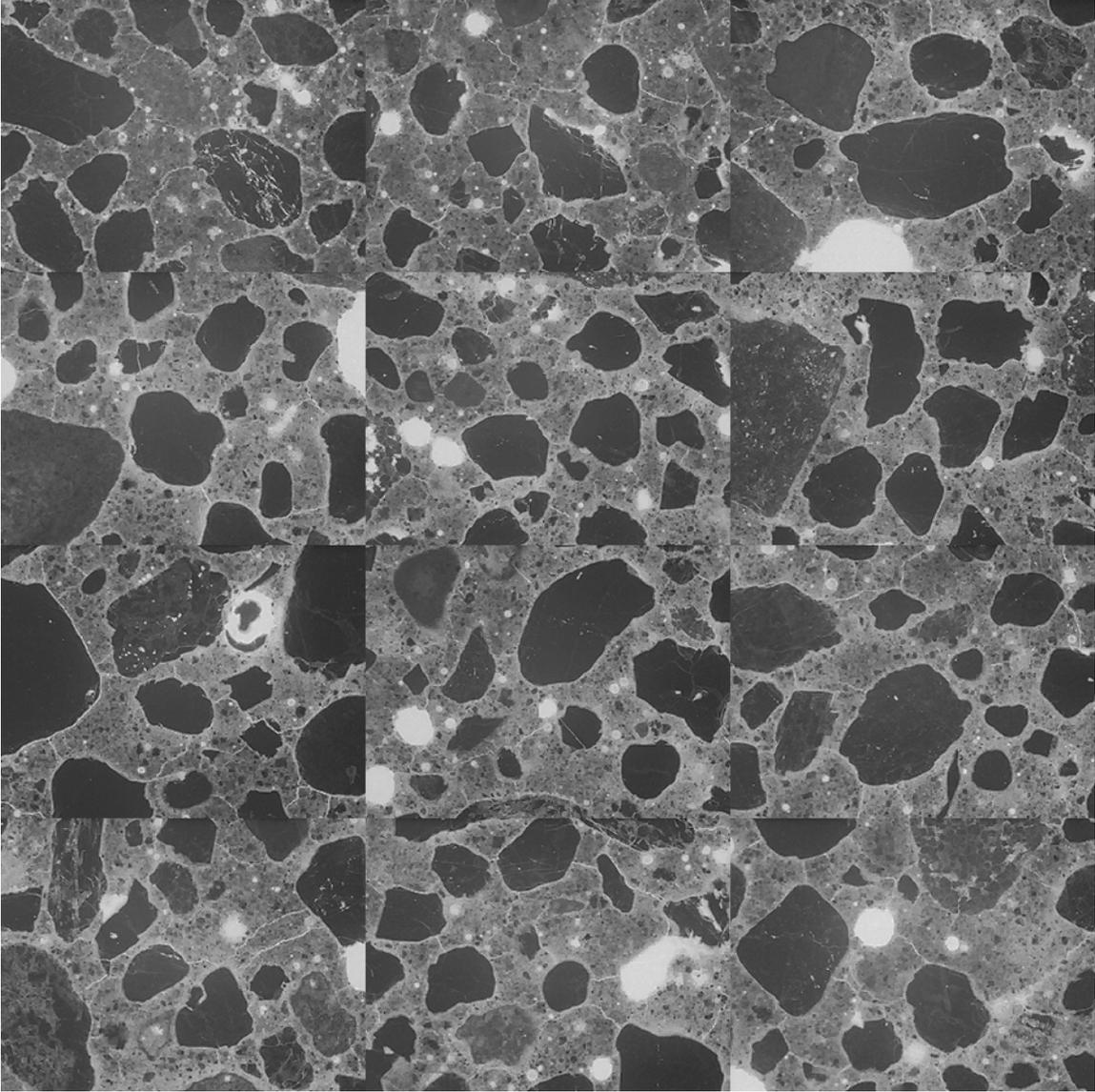
Figure IA-9: Mosaic of 12 frames collected from thin section prepared from billet cut from top portion of concrete overlay, core IA-3 (each individual frame measures 2.612 x 1.959 mm).
