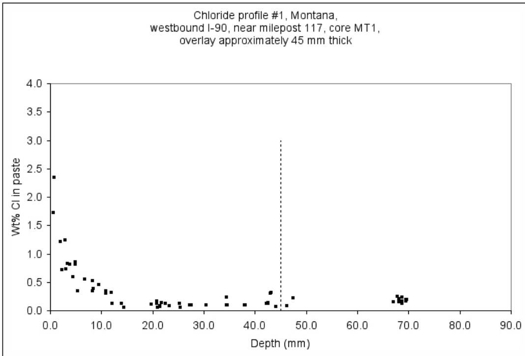
Figure MT-12: Chloride profile through cement paste from billet prepared from core MT-1, dashed line marks the transition between the overlay and the original concrete below.
