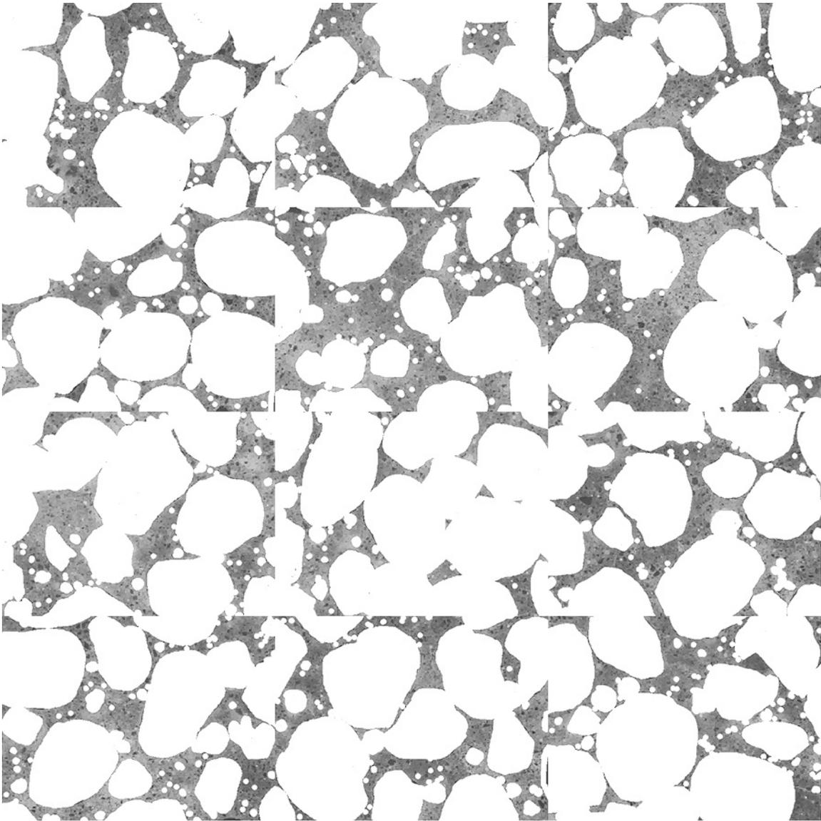
Figure A-2: Mosaic of 12 frames collected from 0.40 w/c 28 day moist cured mortar standards after masking out air voids and fine aggregate to isolate cement paste (each individual frame measures 2.612 x 1.959 mm).
