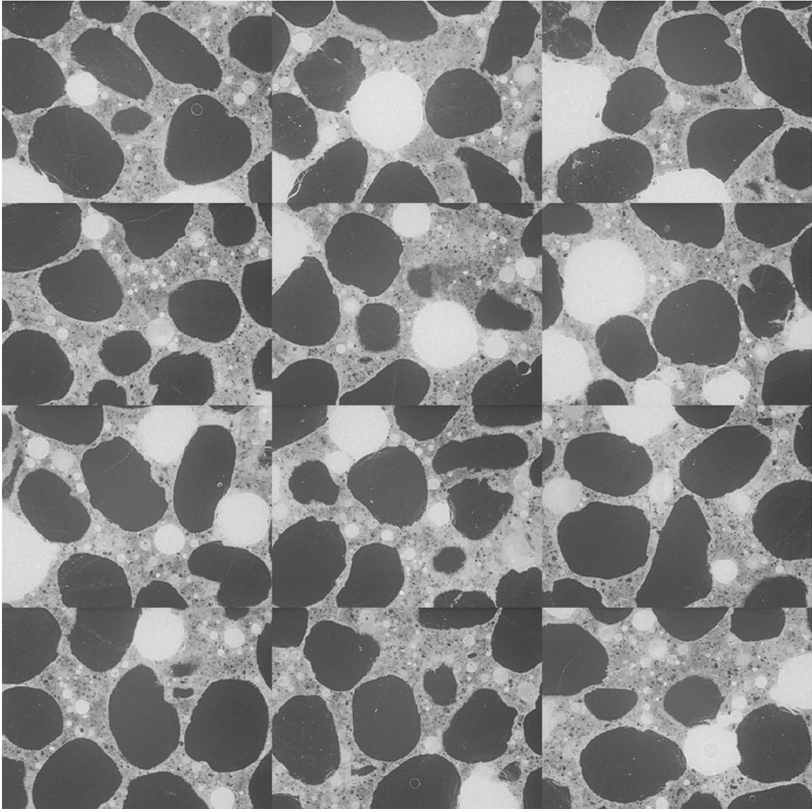
Figure A-3: Mosaic of 12 frames collected from 0.50 w/c 28 day moist cured mortar standards (each individual frame measures 2.612 x 1.959 mm).
