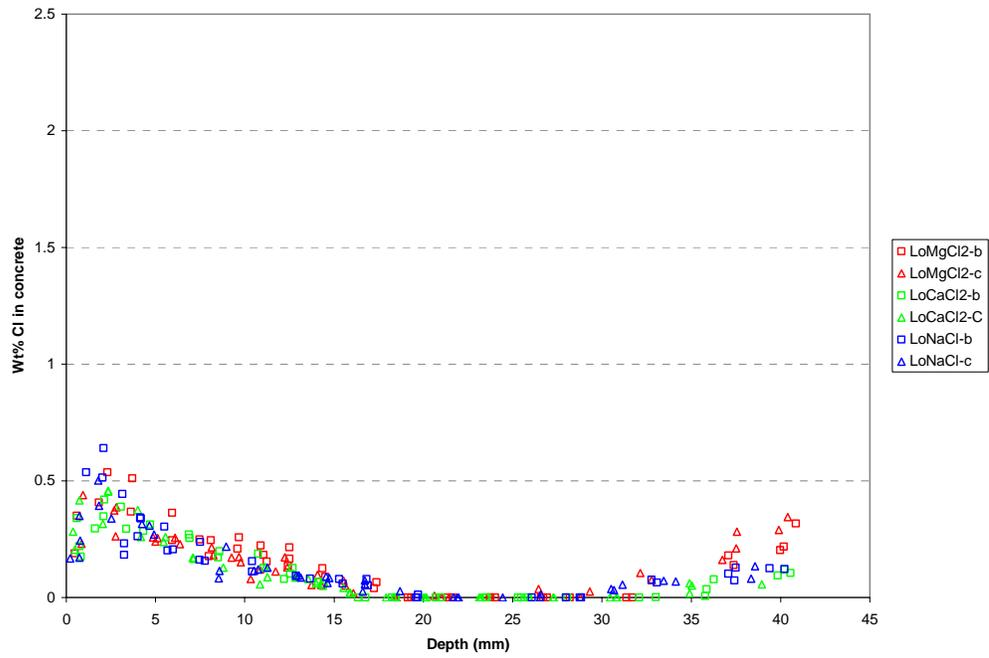
Figure 4. Chloride profiles of 0.55w/c PCC billets in three low concentration deicer solutions.
