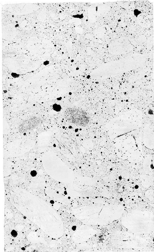
Figure T-6: Polished slabs to show complete cross-section through core T-2 after treatment to enhance appearance of air voids and cracks, tic marks every cm.
