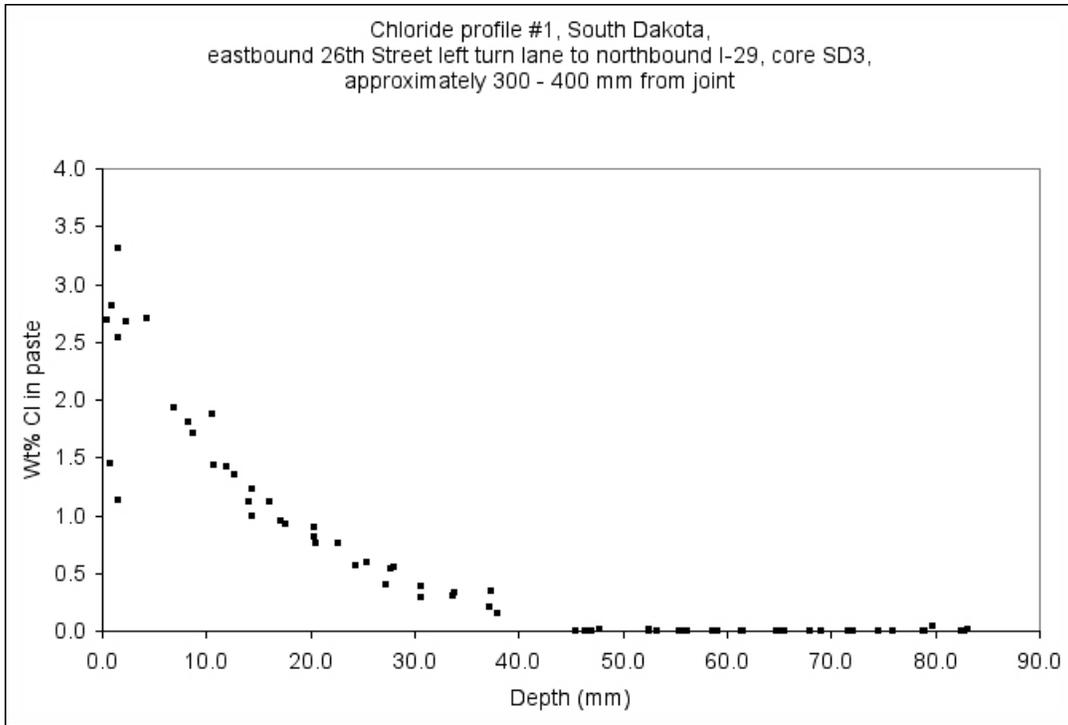
Figure SD-22: Chloride profile through cement paste, from billet prepared from core SD-3.
