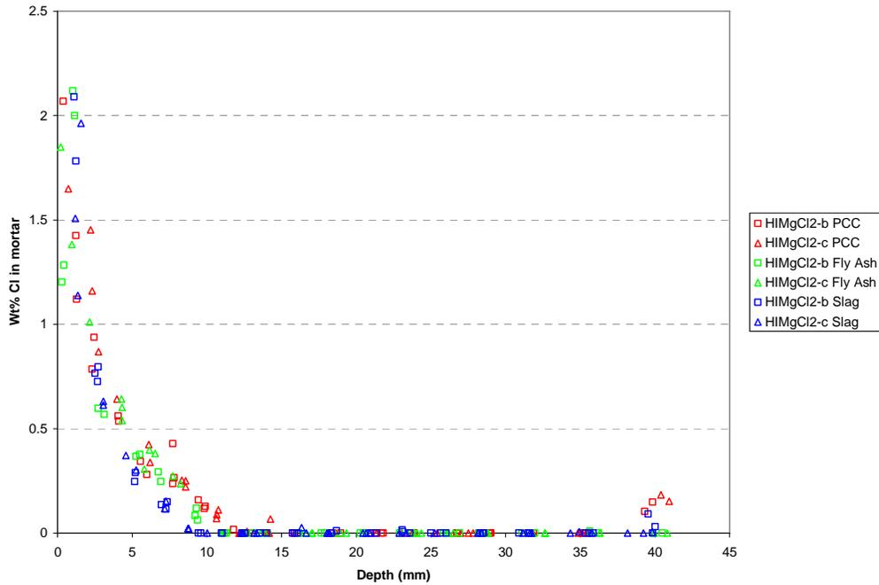
Figure 7. Chloride profiles of 0.45w/c PC mortar, mortar with fly ash and mortar with slag billets in high concentration  $MgCl_2$  deicer solution.
