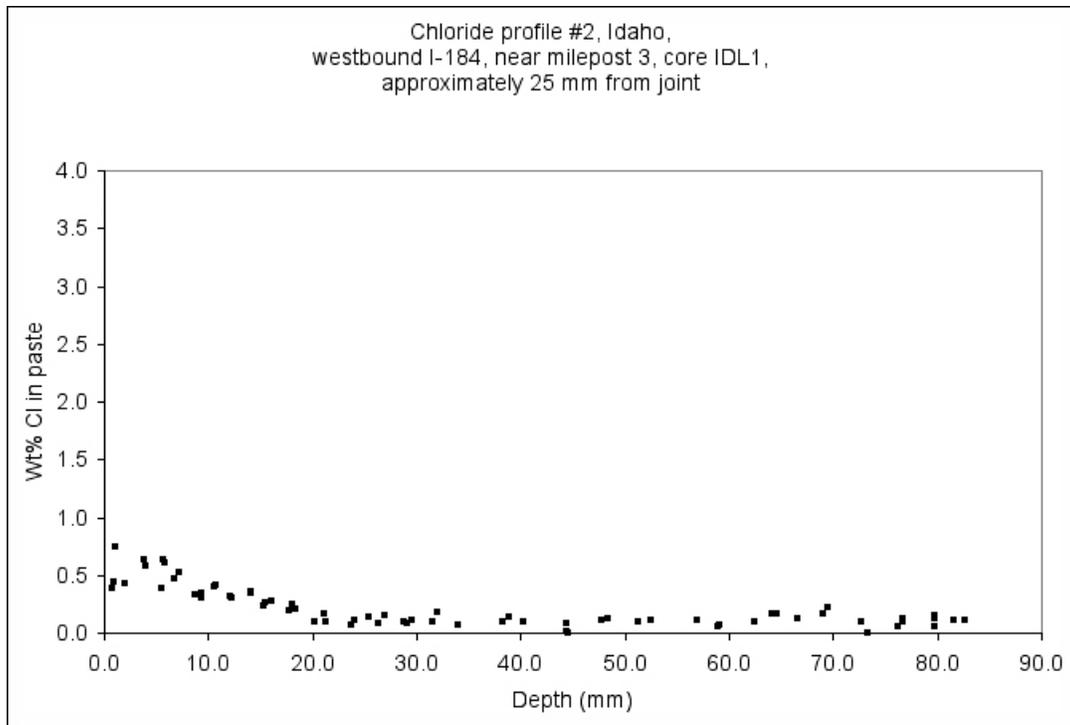
Figure ID-18: Chloride profile through cement paste 25 mm away from joint, from billet prepared from core IDL-1.
