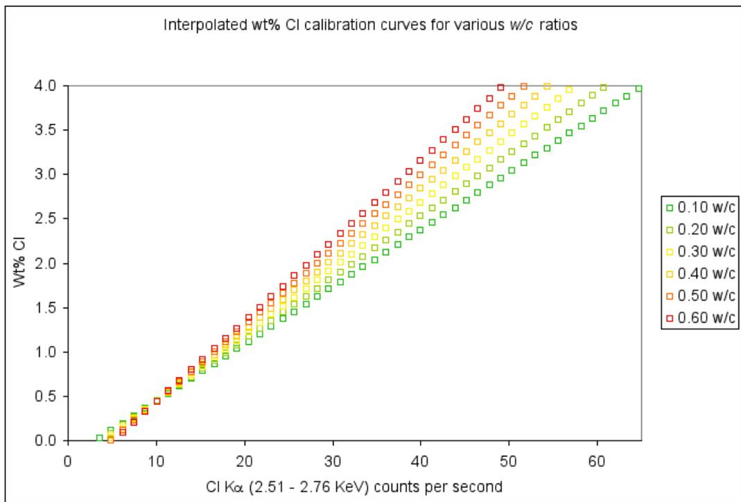
Figure B-4: Interpolated calibration curves plotting CI Ka counts per second versus wt% Cl for cement pastes at various w/c levels.
