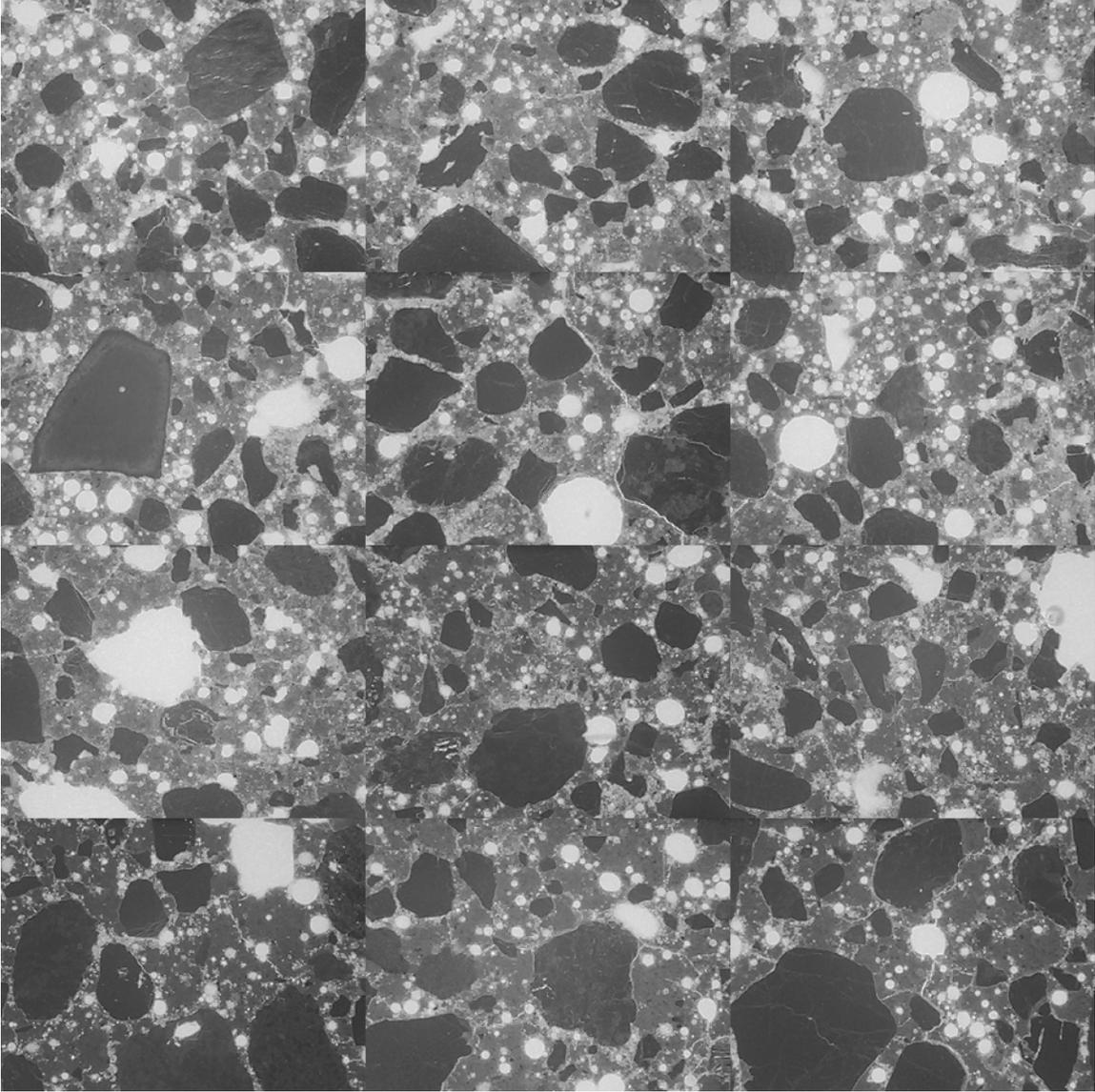
Figure SD-19: Mosaic of 12 frames collected from thin section prepared from billet cut from top portion of core SD-5 (each individual frame measures 2.612 x 1.959 mm).
