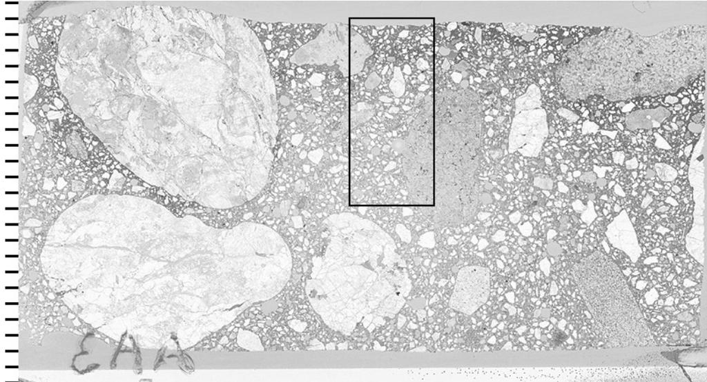
Figure T-13: Transmitted light scanned image of thin section to show location of elemental map. The top of the thin section represents the wear surface of the pavement, (tic marks every mm).
