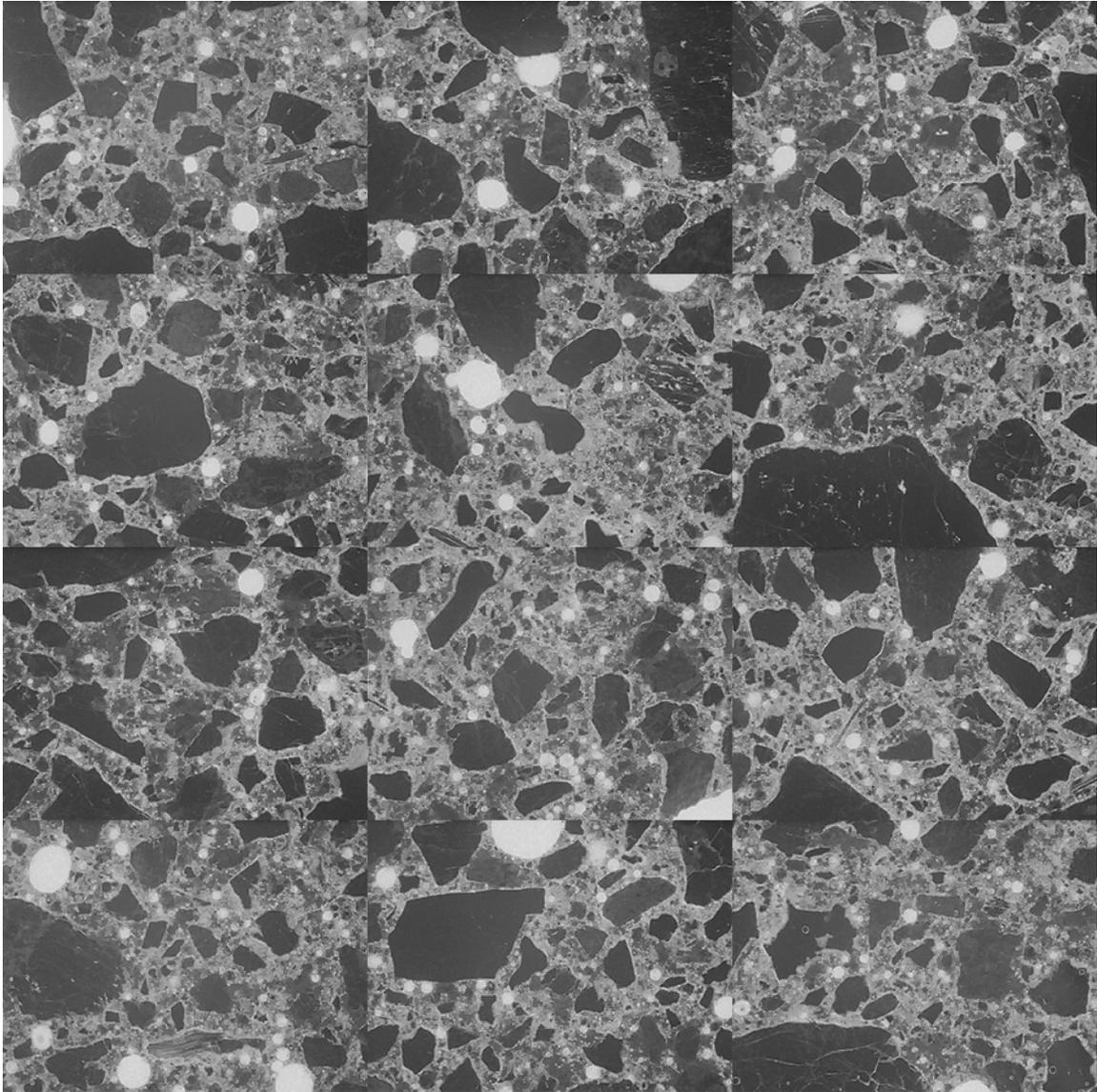
Figure T-8: Mosaic of 12 frames collected from thin section prepared from billet cut from top portion of core T-2 (each individual frame measures 2.612 x 1.959 mm).
