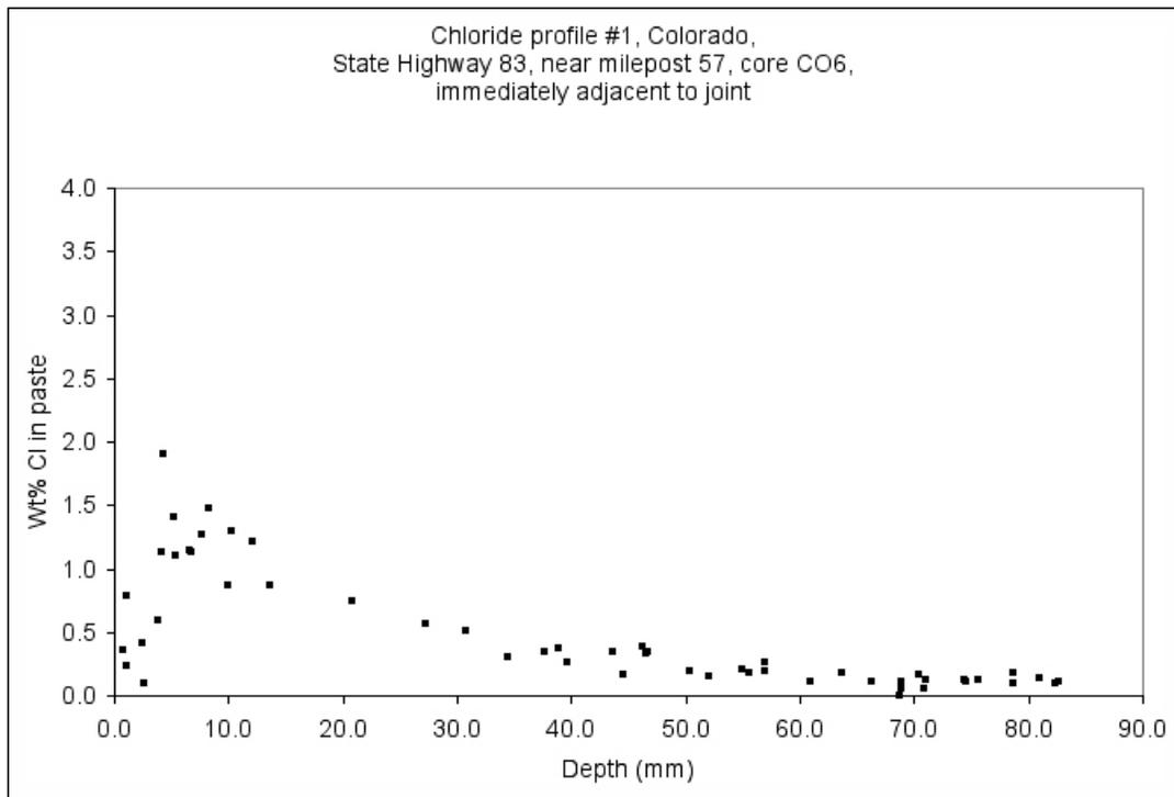
Figure CO-13: Chloride profile through cement paste, from billet prepared from core CO-6.
