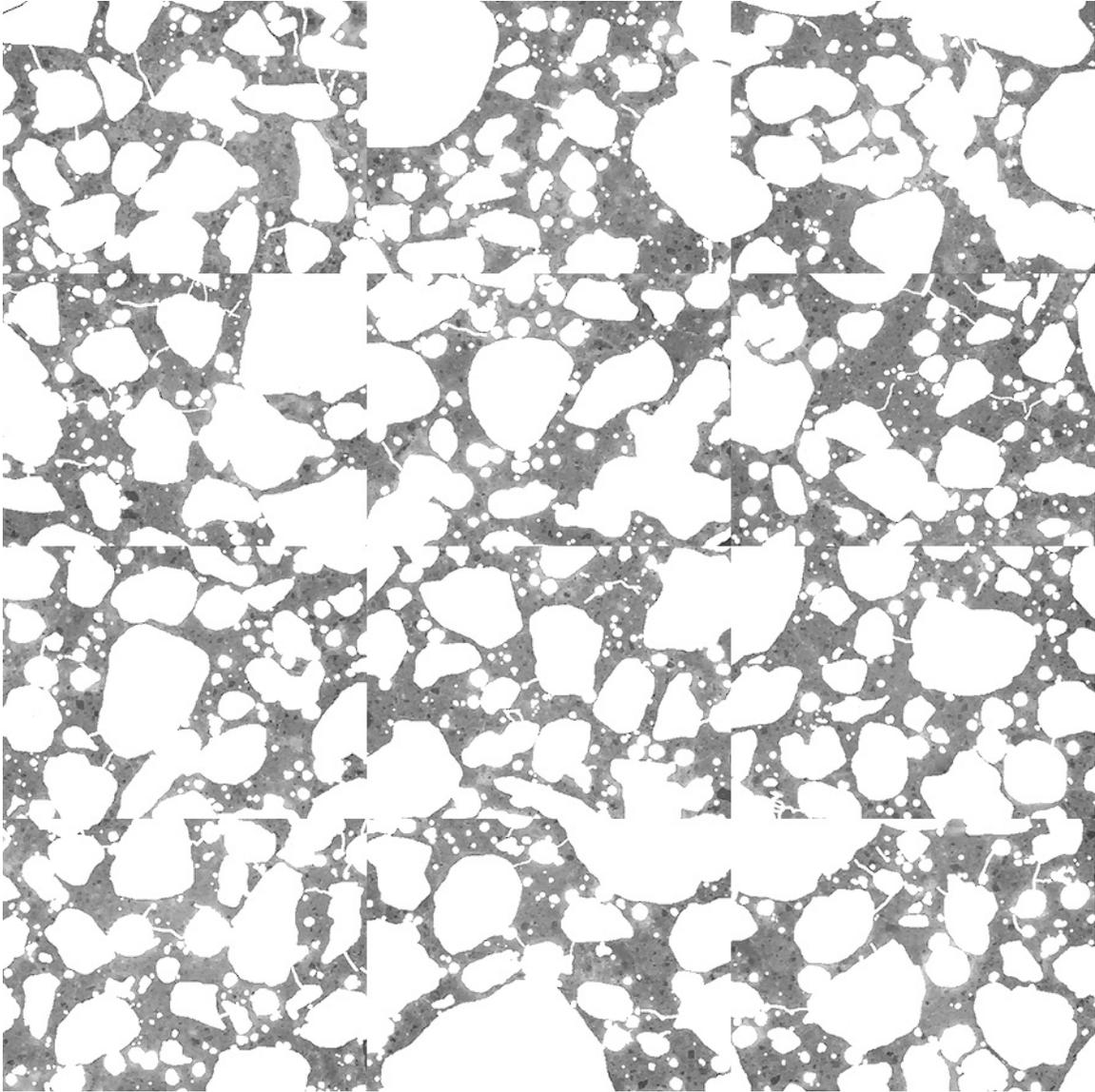
Figure IA-12: Mosaic of 12 frames collected area of thin section representing the original concrete below the concrete overlay, core IA-11, after masking out air voids, fine aggregate, and micro-cracks to isolate cement paste (each individual frame measures 2.612 x 1.959 mm).
