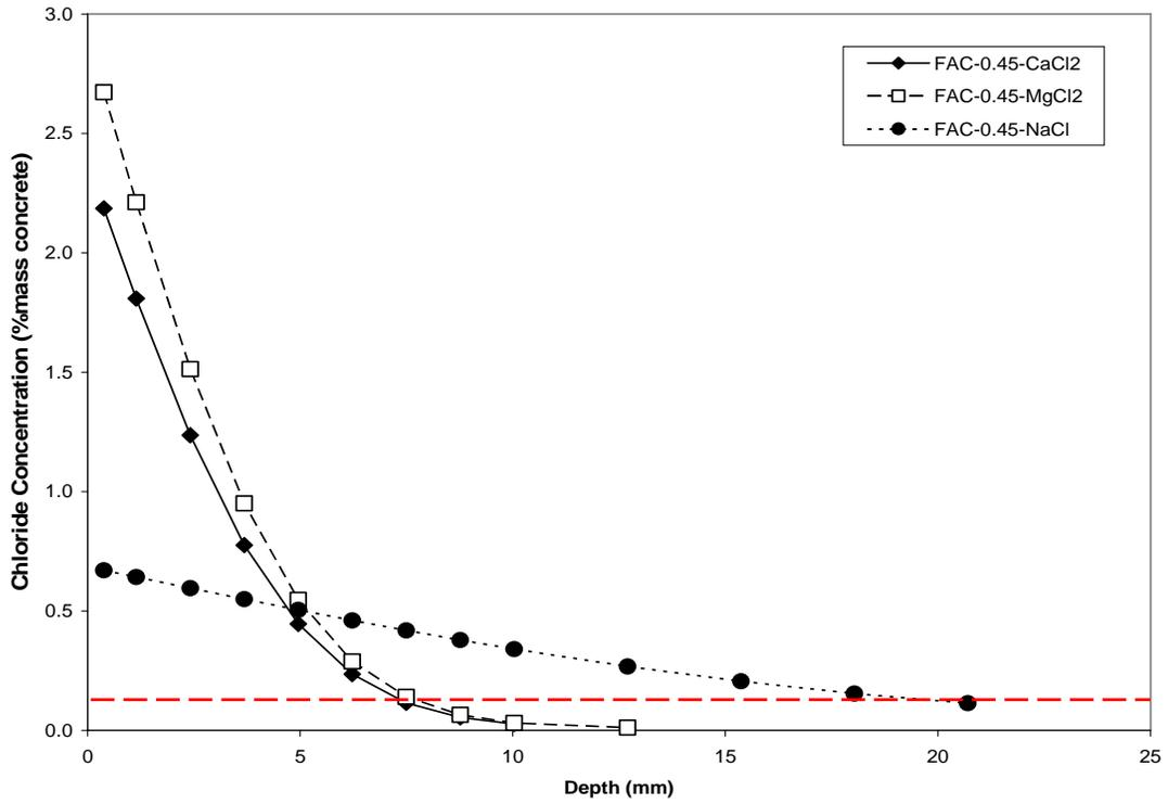
Figure 3. Portland cement + 15% fly ash concrete samples (w/cm=0.45) - chloride profiles for different salts
