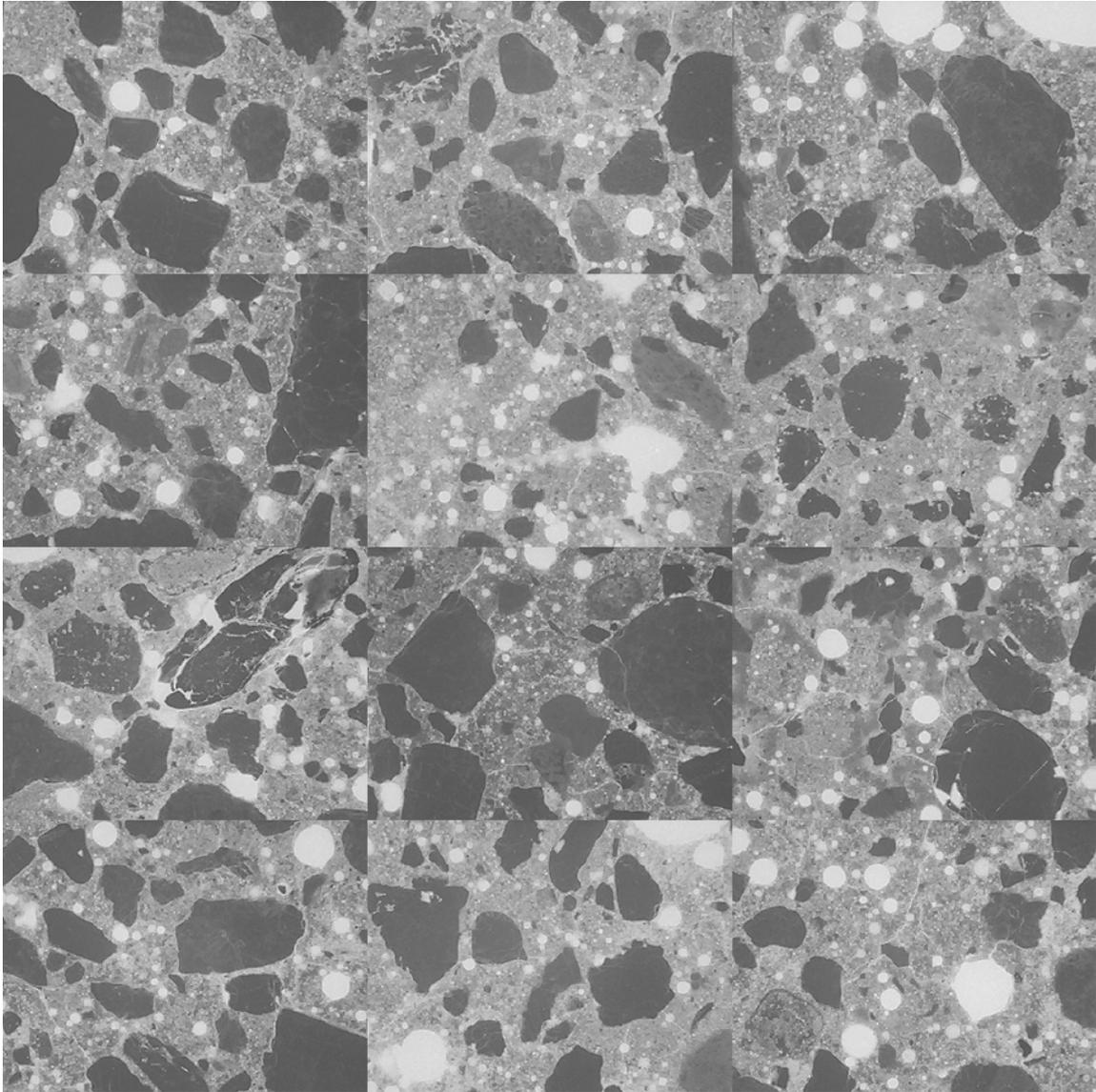
Figure SD-18: Mosaic of 12 frames collected from thin section prepared from a second billet cut from top portion of core SD-4 (each individual frame measures 2.612 x 1.959 mm). These frames were not masked and used for w/c determination, but recorded as visual check against the first section prepared from core SD-4.
