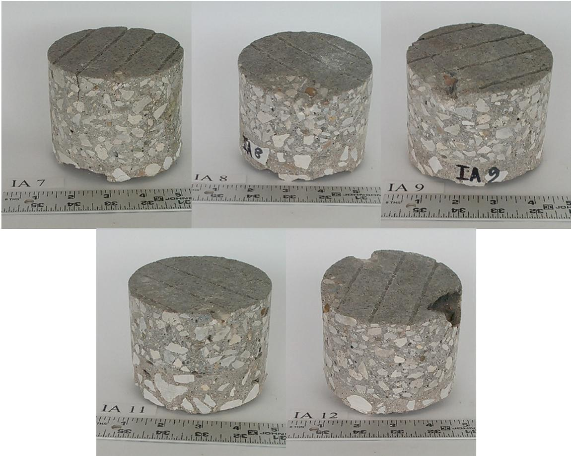
Figure IA-4: Partial depth cores through bridge deck from left hand side of lane.
