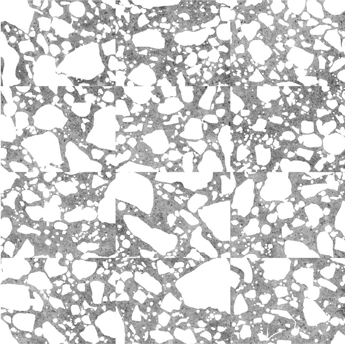
Figure ID-16: Mosaic of 12 frames collected from thin section prepared from billet cut from top portion of core IDL-1 after masking out air voids and fine aggregate to isolate cement paste (each individual frame measures 2.612 x 1.959 mm).
