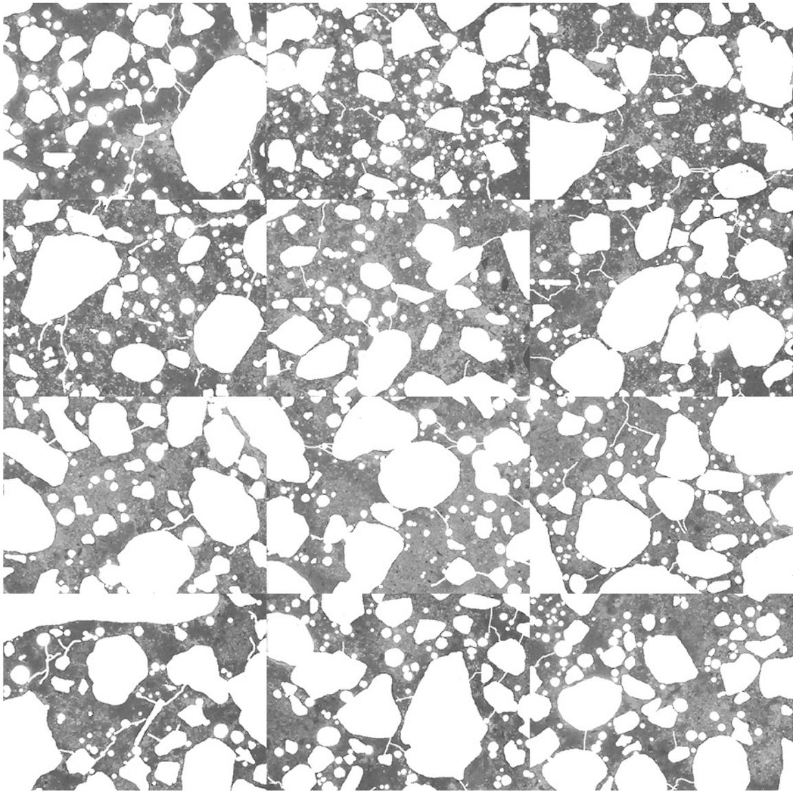
Figure SD-17: Mosaic of 12 frames collected from thin section prepared from billet cut from top portion of core SD-4 after masking out air voids, fine aggregate, and micro-cracks to isolate cement paste (each individual frame measures 2.612 x 1.959 mm).
