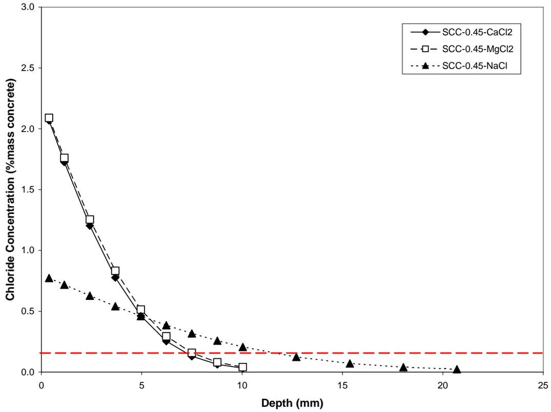
Figure 5. GGBFS blended cement concrete samples (w/cm=0.45) - chloride profiles for different salts
