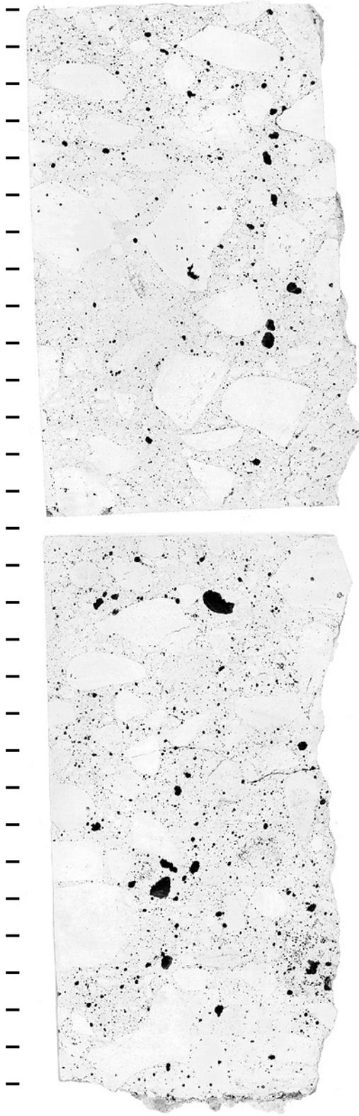
Figure ID-11: Polished slabs to show complete cross-section through core IDR-7 after treatment to enhance appearance of air voids and cracks, tic marks every cm.
