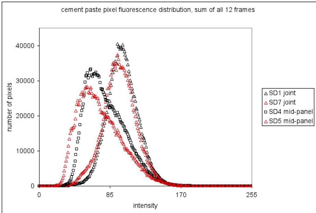
Figure SD-21: Histogram comparing cement paste pixel intensities using all 12 frames as collected from thin sections prepared from cores taken at the joint versus cores taken mid-panel
