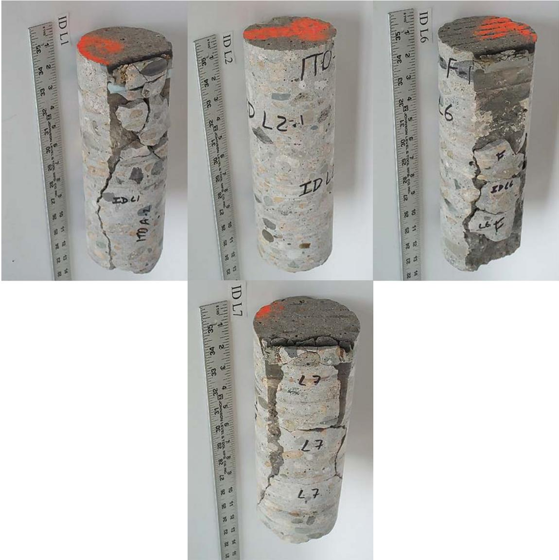
Figure ID-2: Cores from left lane taken near pavement joints.
