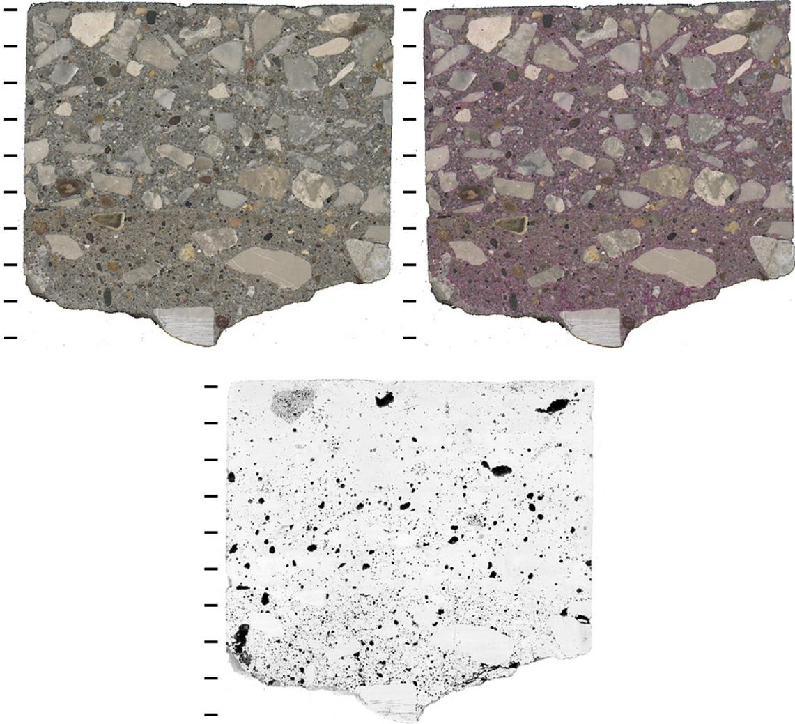
Figure IA-5: Polished slabs to show complete cross-section through core IA-4, before (upper left) and after application of phenolphthalein stain (upper right) and after treatment to enhance appearance of air voids and cracks (bottom) tic marks every cm.
