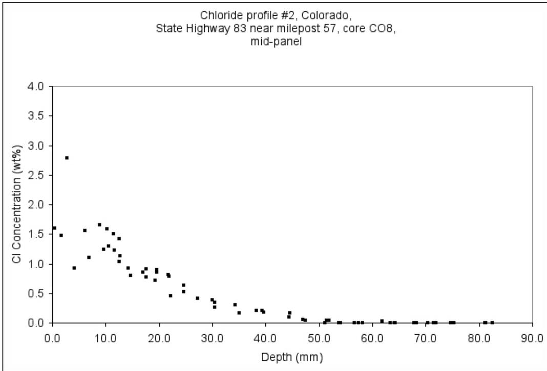
Figure CO-16: Chloride profile through cement paste, from billet prepared from core CO-8.
