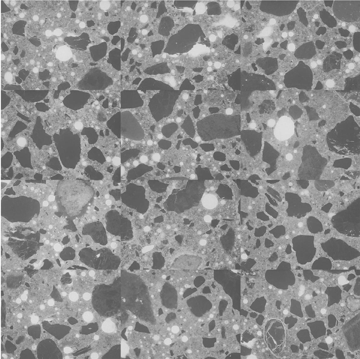
Figure SD-11: Mosaic of 12 frames collected from thin section prepared from billet cut from top portion of core SD-1 (each individual frame measures 2.612 x 1.959 mm).
