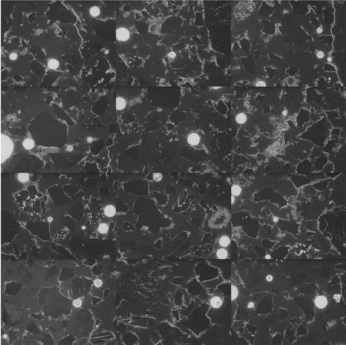
Figure MT-8: Mosaic of 12 frames collected from thin section prepared from billet cut from top portion of concrete overlay, core MT-3 (each individual frame measures 2.612 x 1.959 mm).
