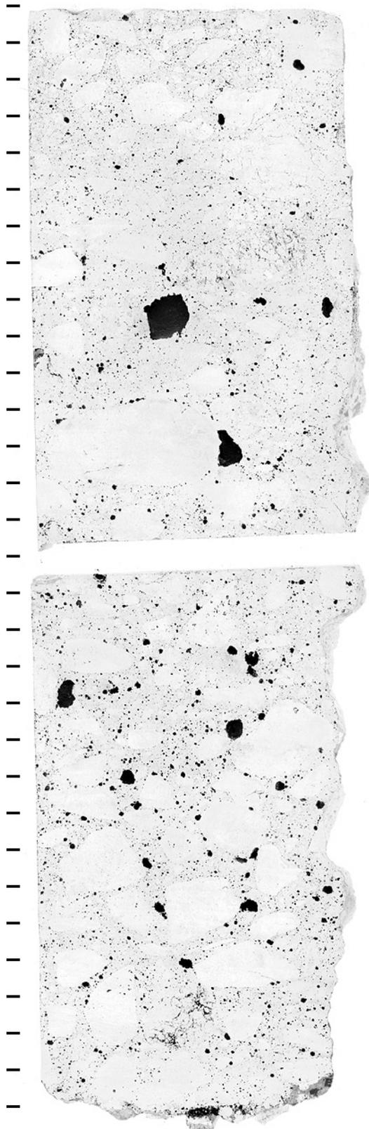
Figure ID-7: Polished slabs to show complete cross-section through core IDL-6 after treatment to enhance appearance of air voids and cracks, tic marks every cm.
