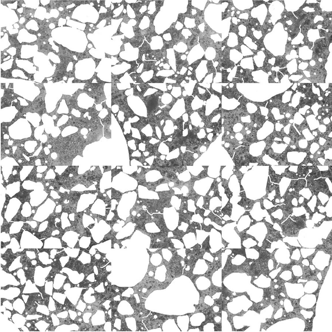
Figure S-9: Mosaic of 12 frames collected from thin section prepared from billet cut from top portion of core S-2 after masking out air voids, fine aggregate, and micro-cracks to isolate cement paste (each individual frame measures 2.612 x 1.959 mm).
