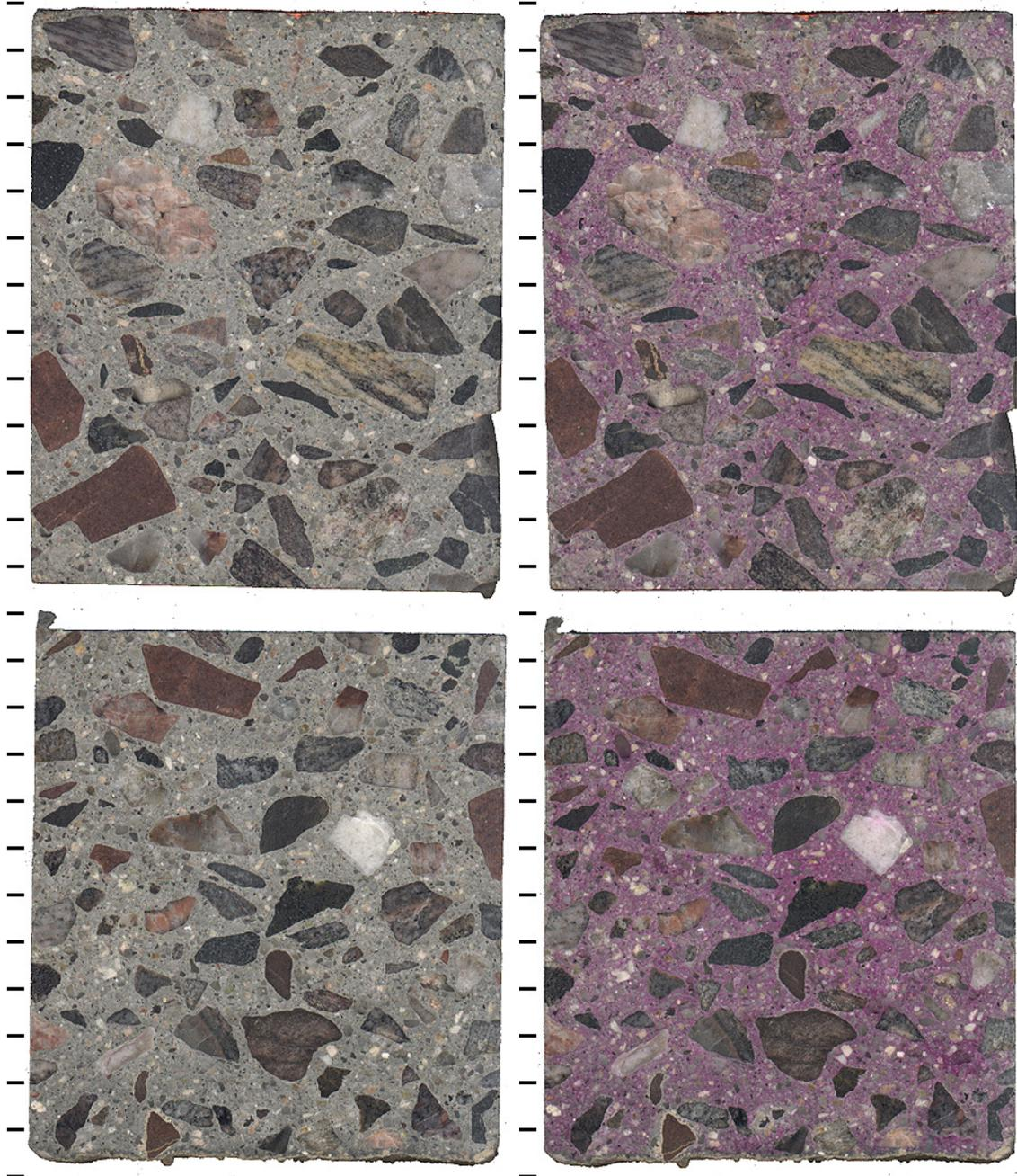
Figure CO-7: Polished slabs to show complete cross-section through core CO-5 both before (left) and after application of phenolphthalein stain (right) tic marks every cm.
