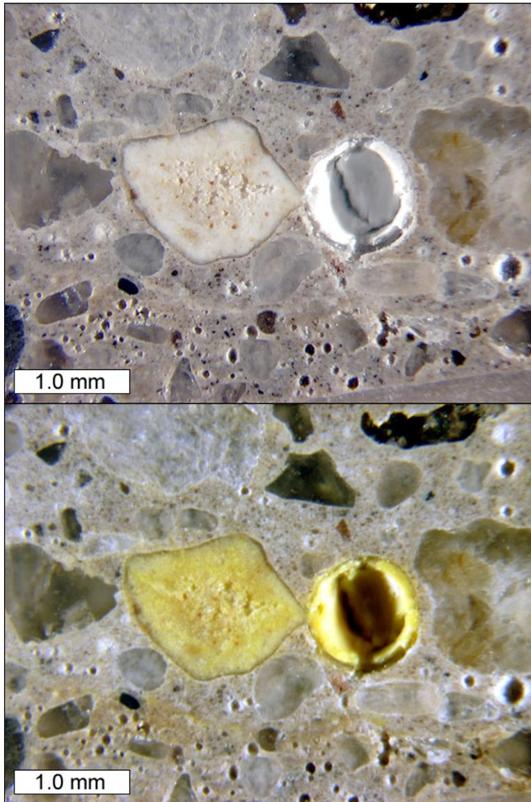
Figure IA-8: Stereo microscope images to show reactive aggregate particle both before (top) and after (bottom) treatment with sodium cobaltinitrite stain (sample IA-7). Image also illustrates the contrast in texture between the concrete overlay (top  $\frac{3}{4}$  of image) and the original concrete below (bottom  $\frac{1}{4}$  of image).
