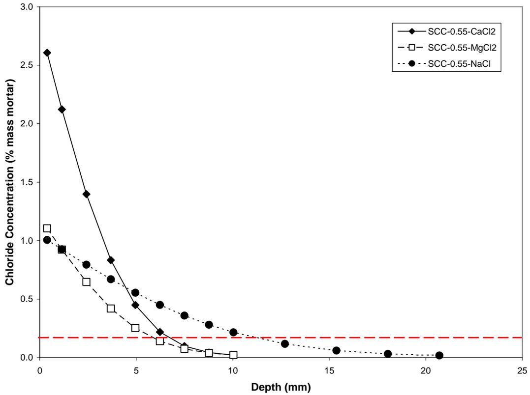
Figure 6. GGBFS blended cement concrete samples (w/cm=0.55) - chloride profiles for different salts
