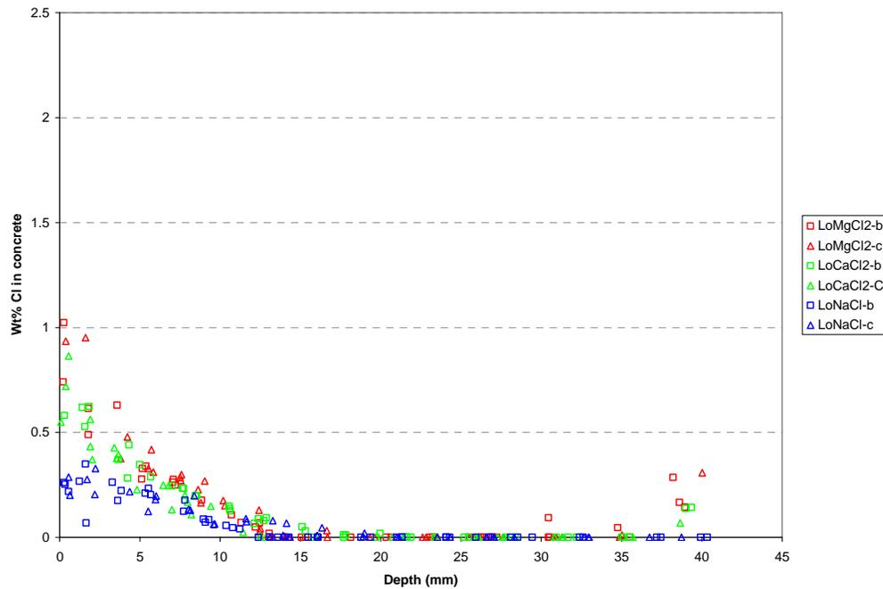
Figure 3. Chloride profiles of 0.45w/c PCC billets in three low concentration deicer solutions.
