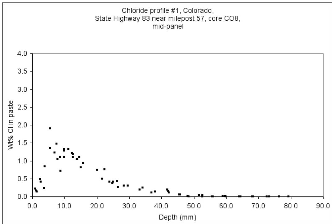
Figure CO-15: Chloride profile through cement paste, from billet prepared from core CO-8.
