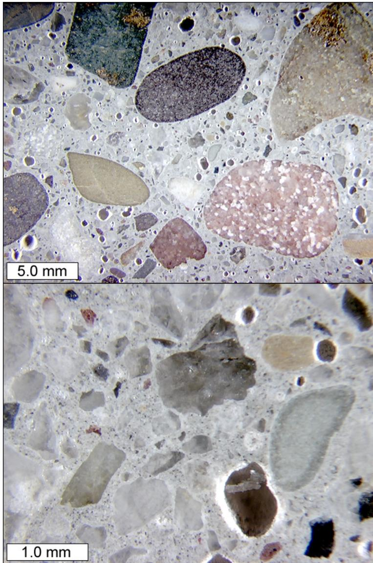
Figure MT-7: Stereo microscope images to show air void structure of concrete overlay on polished slab from core MT-2.
