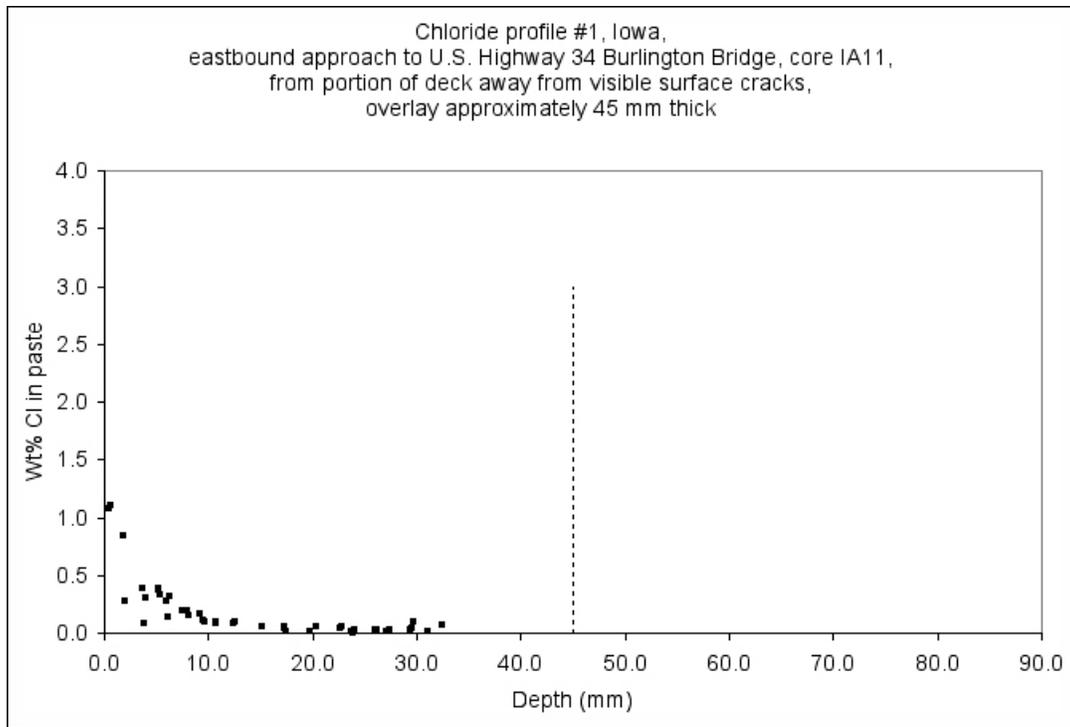
Figure IA-15: Chloride profile through cement paste, from billet prepared from core IA-11, dashed line marks the transition point between concrete overlay and the original concrete below the overlay.
