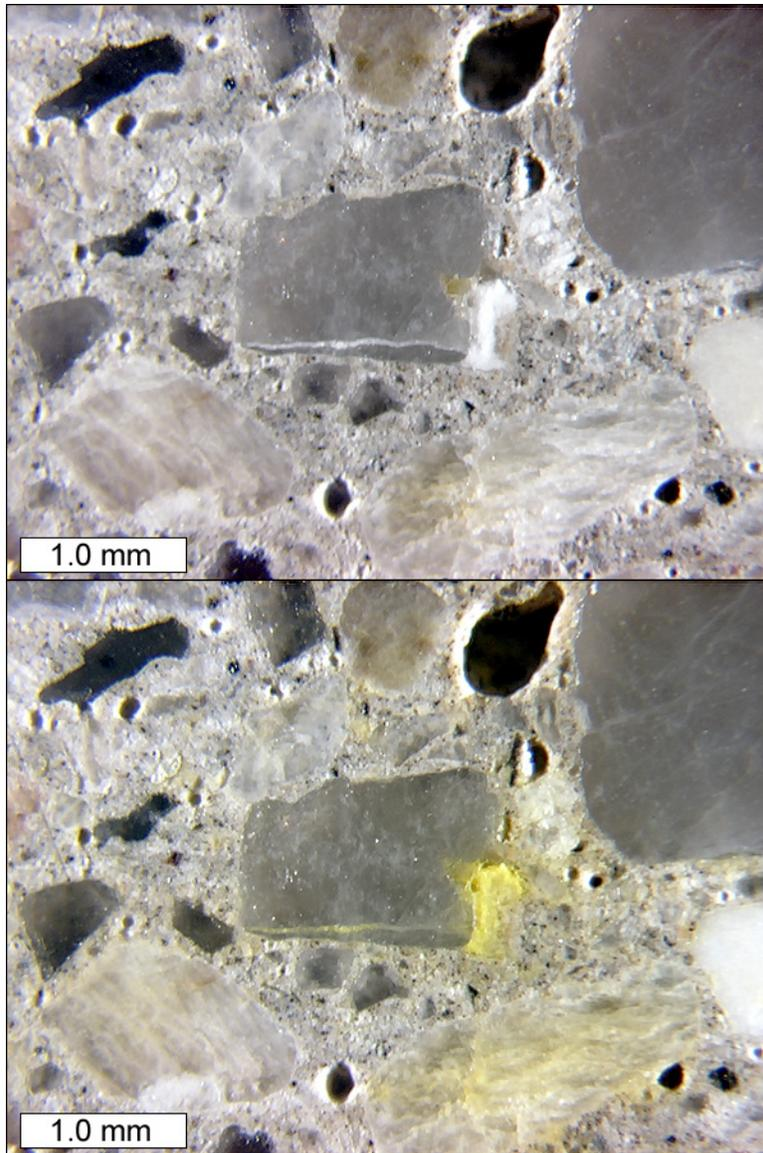
Figure CO-10: Stereo microscope images to show reactive aggregate particle both before (top) and after (bottom) treatment with sodium cobaltinitrite stain (sample CO-5).
