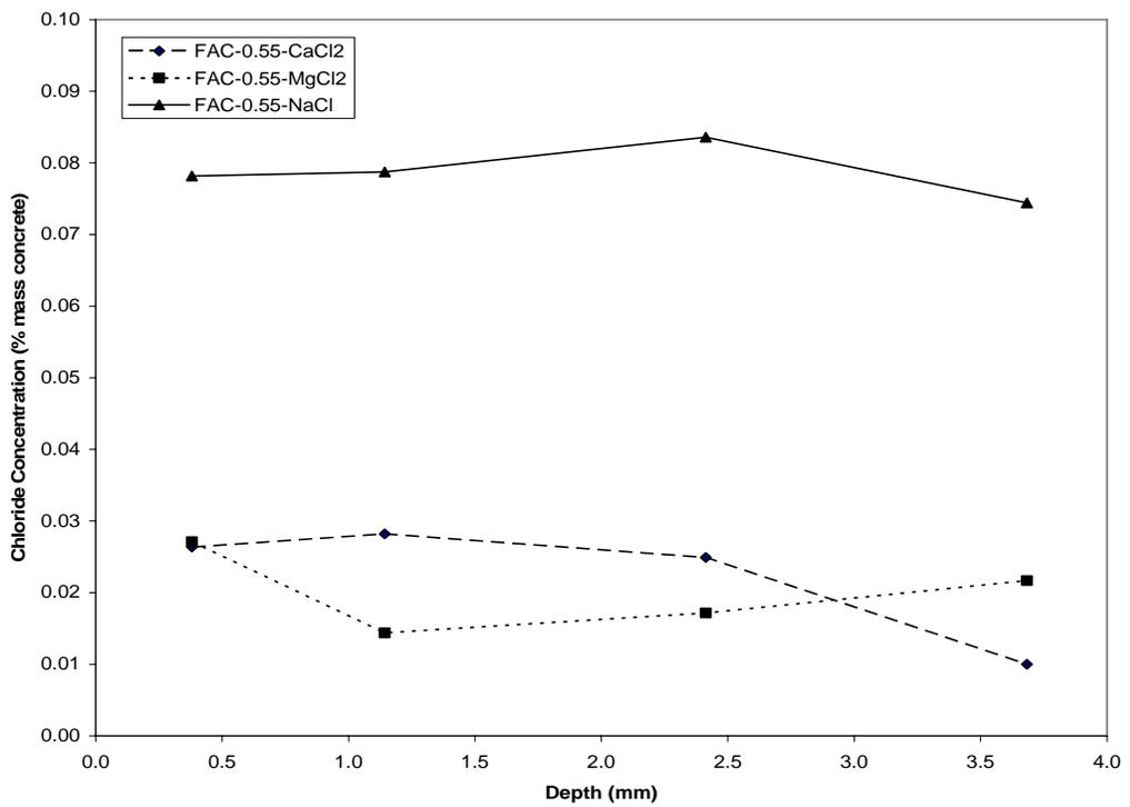
Figure 8. Portland cement + 15% fly ash concrete samples (sealer 1) - chloride profiles
