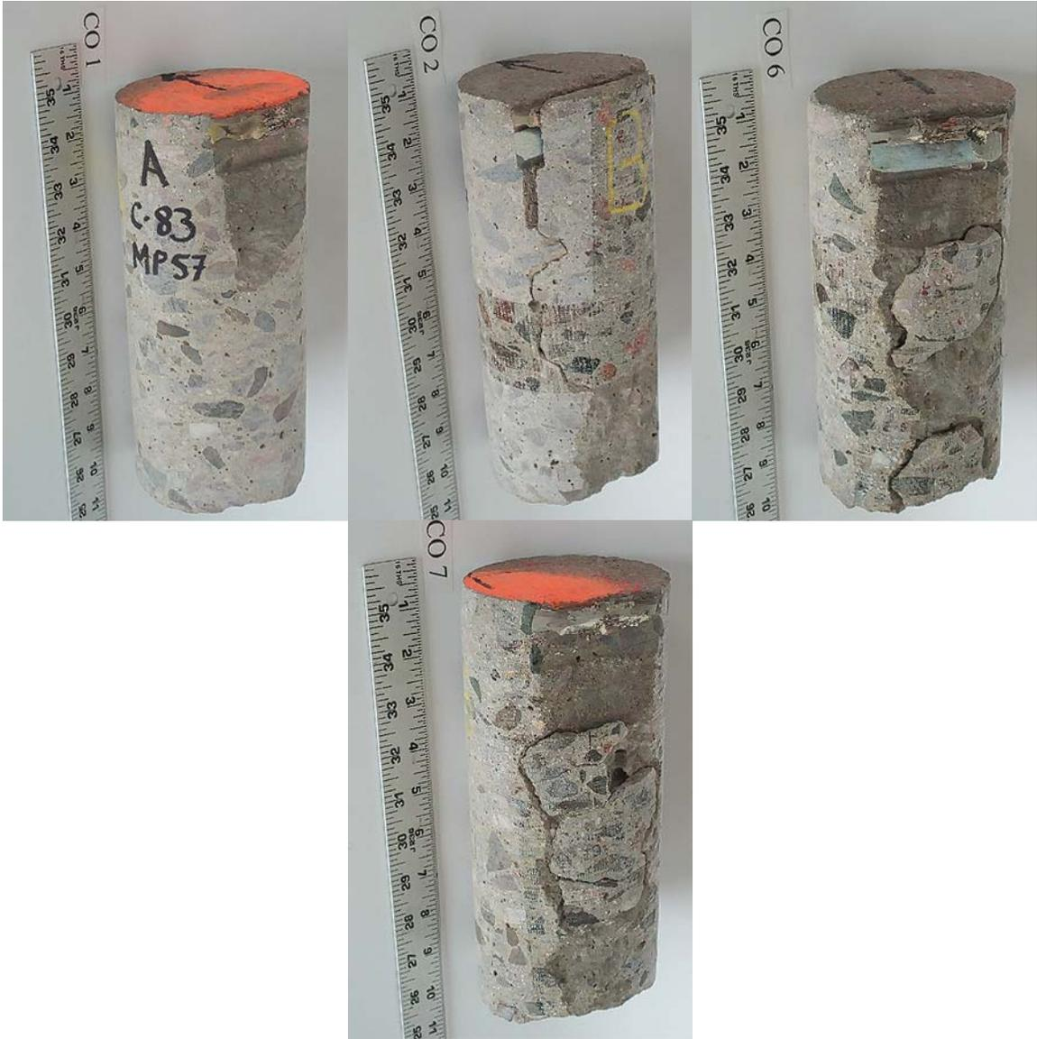
Figure CO-3: Cores taken at joint.
