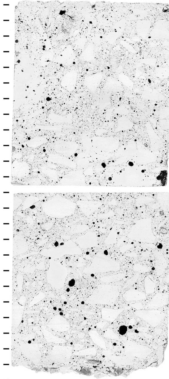
Figure SD-7: Polished slabs to show complete cross-section through core SD-1 after treatment to enhance appearance of air voids and cracks, tic marks every cm.
