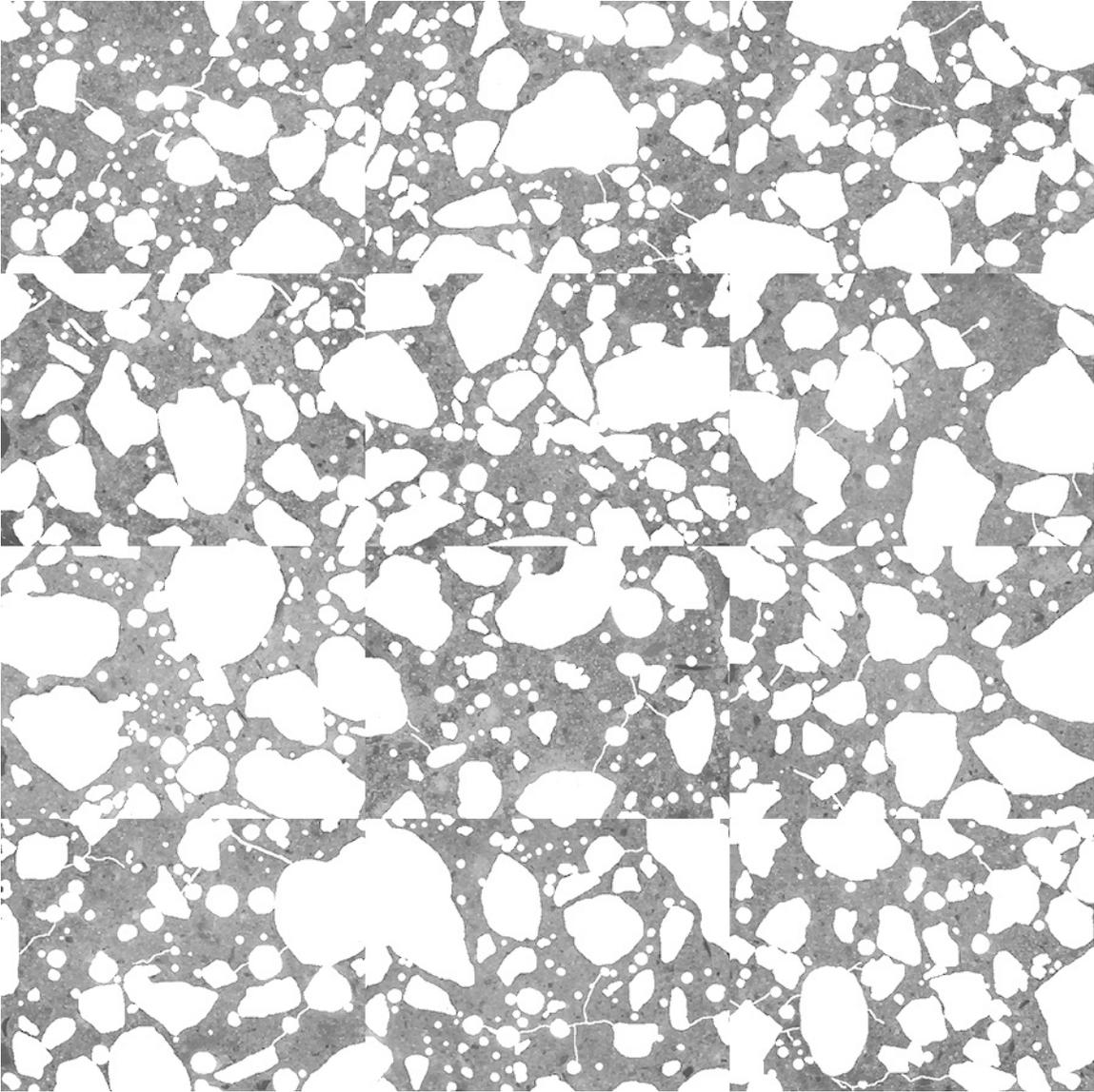
Figure SD-12: Mosaic of 12 frames collected from thin section prepared from billet cut from top portion of core SD-1 after masking out air voids, fine aggregate, and micro-cracks to isolate cement paste (each individual frame measures 2.612 x 1.959 mm).
