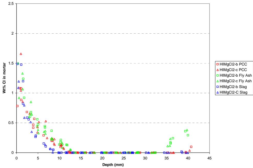
Figure 8. Chloride profiles of 0.55w/c PC mortar, mortar with fly ash and mortar with slag billets in high concentration  $MgCl_2$  deicer solution.
