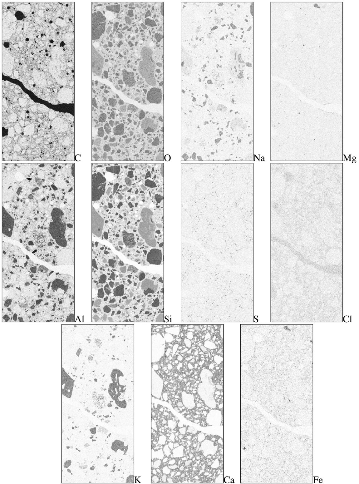
Figure T-16: Elemental maps from crack at depth, darker regions indicate higher concentrations.
