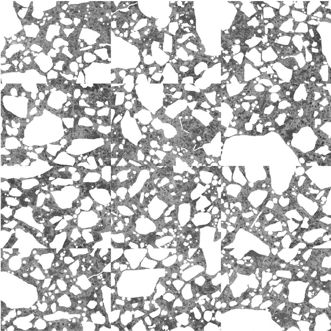
Figure T-9: Mosaic of 12 frames collected from thin section prepared from billet cut from top portion of core T-2 after masking out air voids, fine aggregate, and micro-cracks to isolate cement paste (each individual frame measures 2.612 x 1.959 mm).
