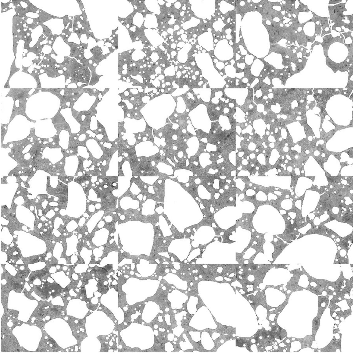
Figure SD-15: Mosaic of 12 frames collected from thin section prepared from billet cut from top portion of core SD-7 after masking out air voids, fine aggregate, and micro-cracks to isolate cement paste (each individual frame measures 2.612 x 1.959 mm).
