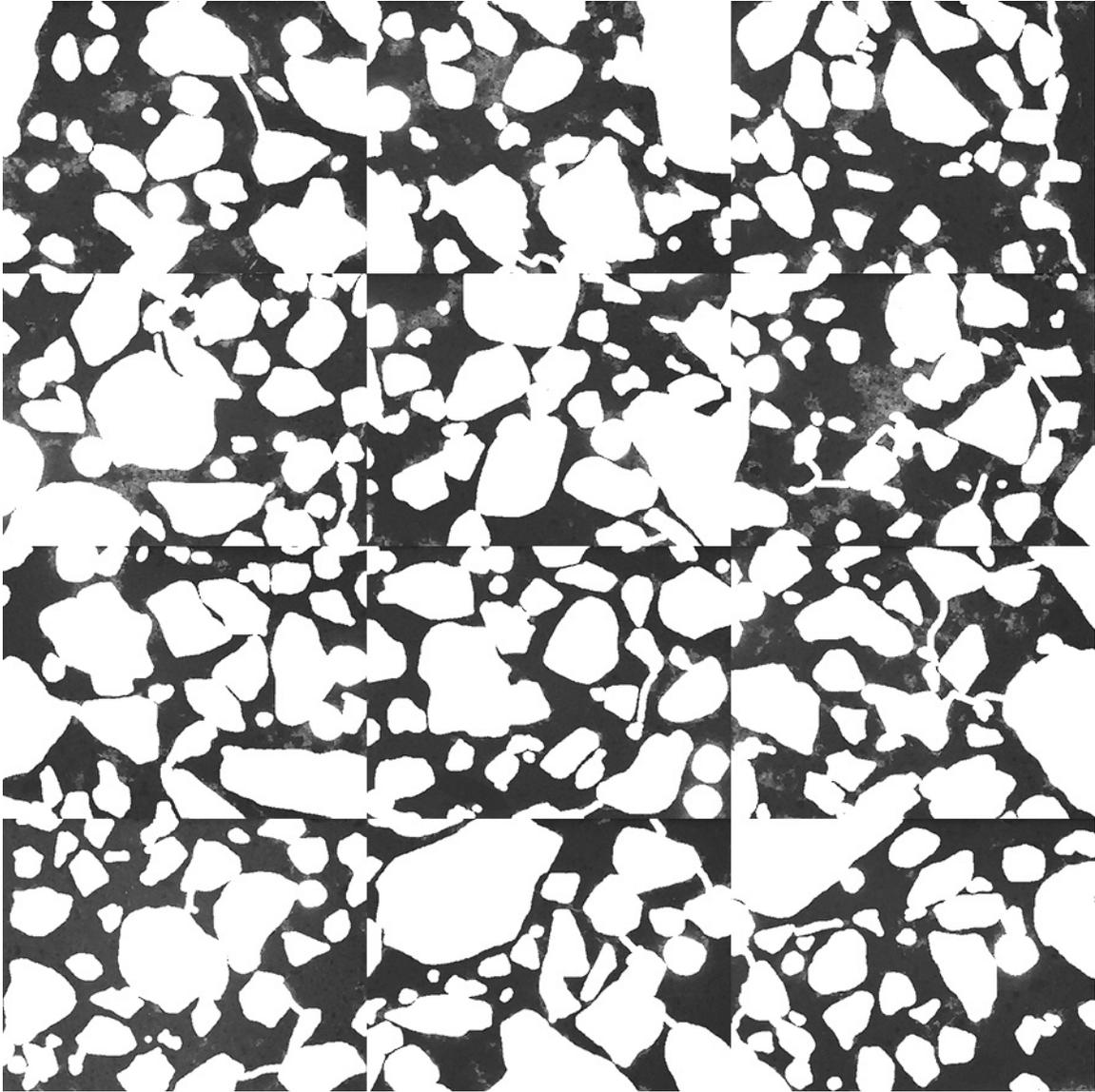
Figure MT-9: Mosaic of 12 frames collected from thin section prepared from billet cut from top portion of concrete overlay, core MT-3, after masking out air voids, fine aggregate, and micro-cracks to isolate cement paste (each individual frame measures 2.612 x 1.959 mm).
