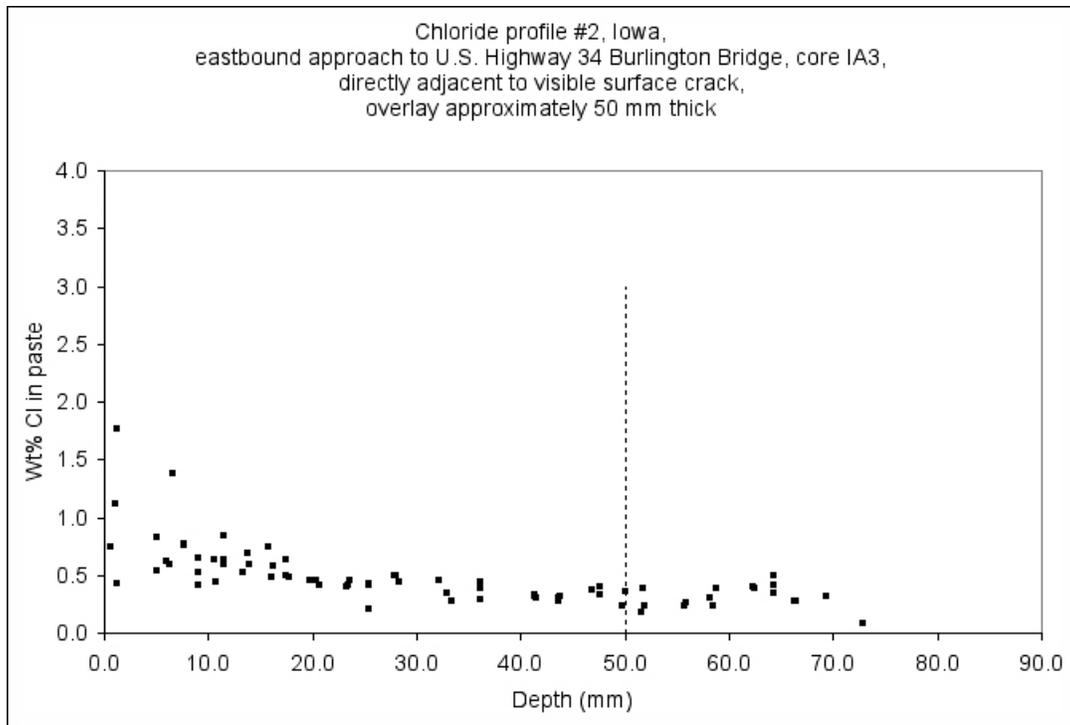
Figure IA-14: Chloride profile through cement paste, directly adjacent to visible surface crack, from billet prepared from core IA-3, dashed line marks the transition point between concrete overlay and the original concrete below the overlay.
