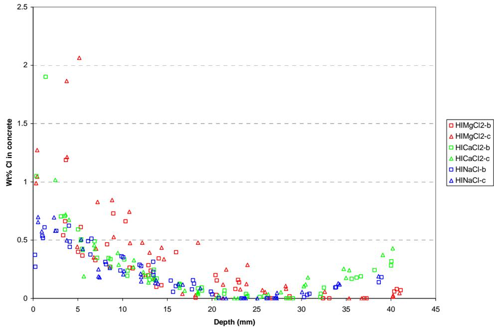
Figure 2. Chloride profiles of 0.55w/c PCC billets in three high concentration deicer solutions.
