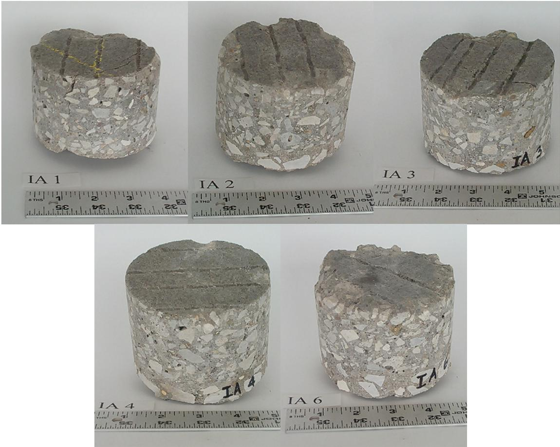
Figure IA-3: Partial depth cores through bridge deck from right hand side of lane.
