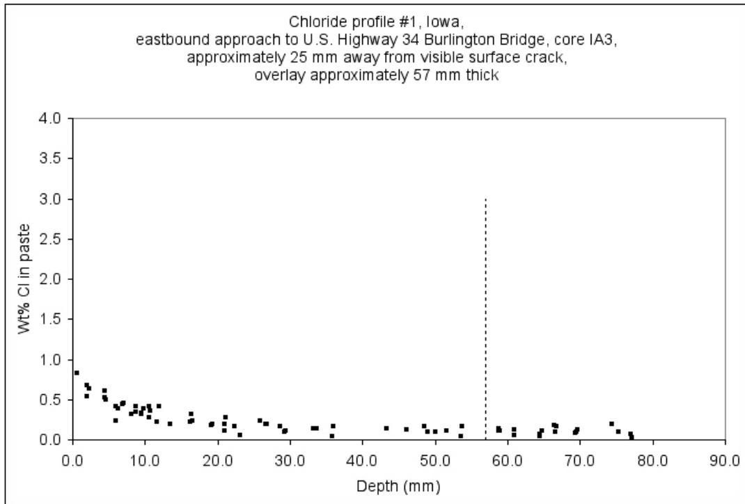
Figure IA-13: Chloride profile through cement paste about 25 mm away from visible surface crack, from billet prepared from core IA-3, dashed line marks the transition point between concrete overlay and the original concrete below the overlay.
