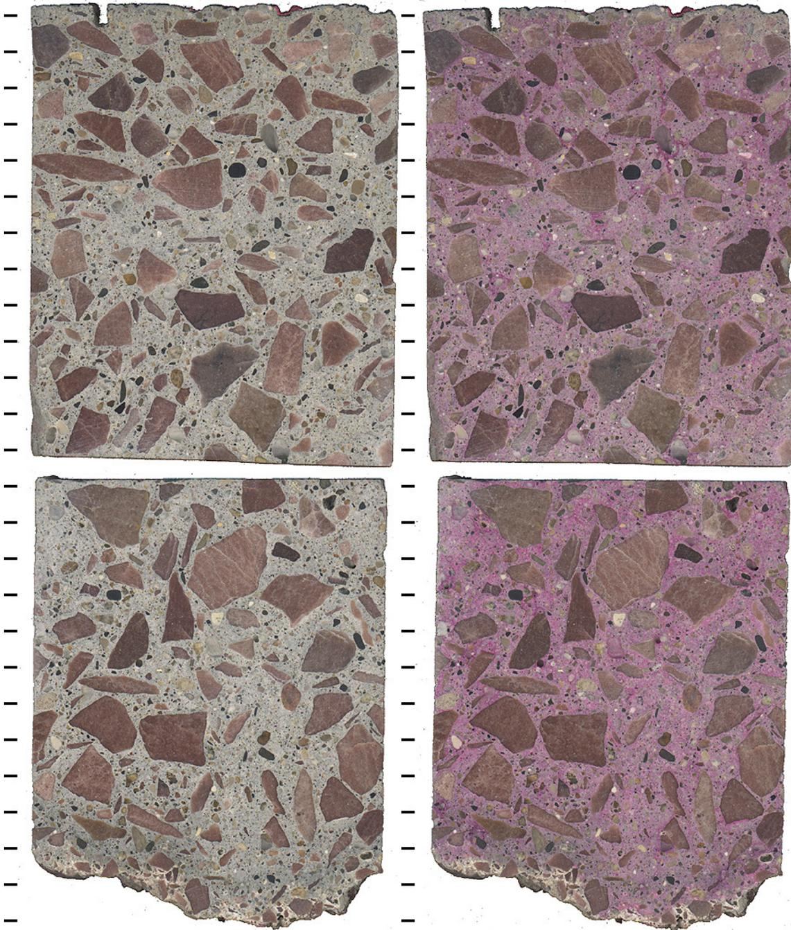
Figure SD-8: Polished slabs to show complete cross-section through core SD-4 both before (left) and after application of phenolphthalein stain (right) tic marks every cm.
