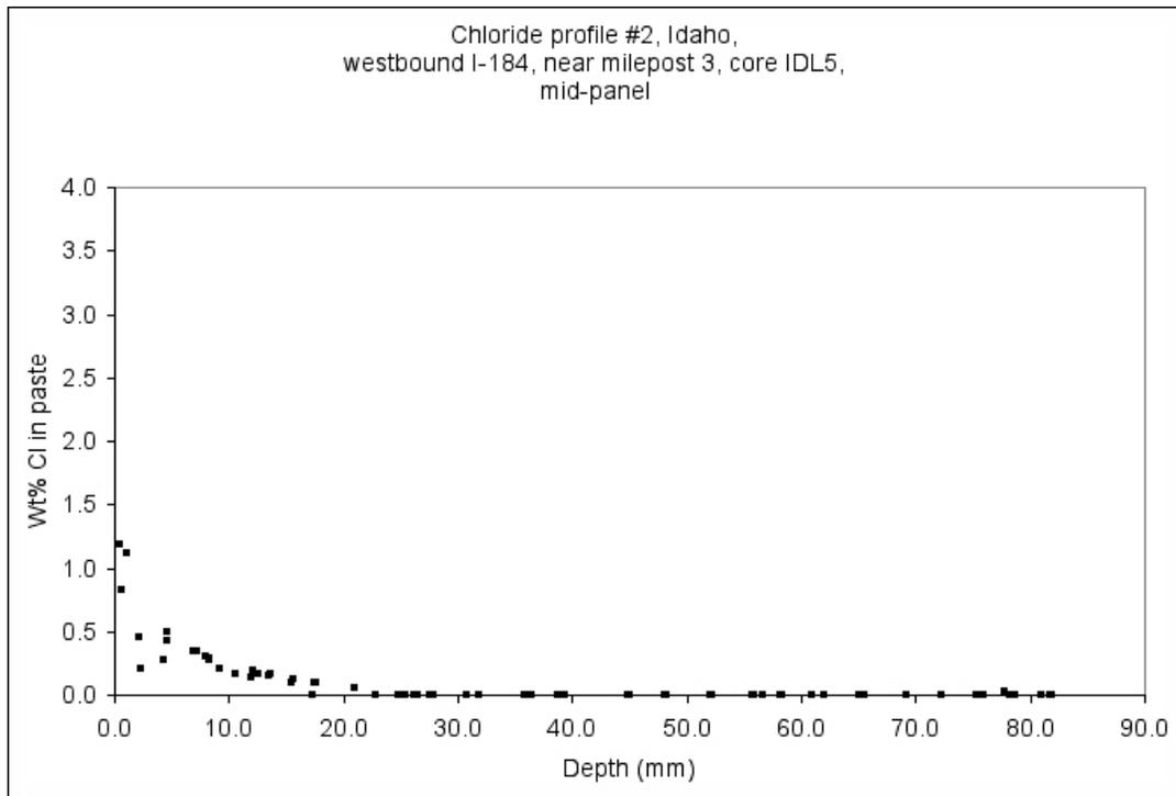
Figure ID-20: Chloride profile through cement paste at mid-panel, from billet prepared from core IDL-5.
