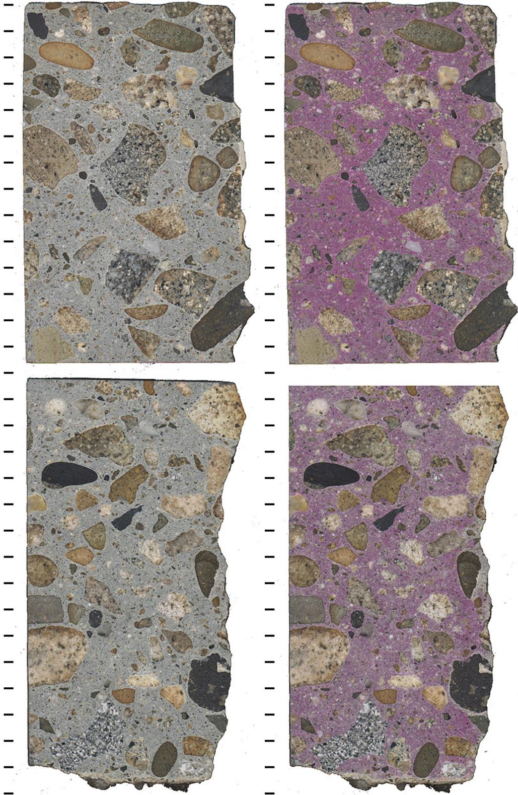
Figure ID-10: Polished slabs to show complete cross-section through core IDR-7 both before (left) and after application of phenolphthalein stain (right) tic marks every cm.
