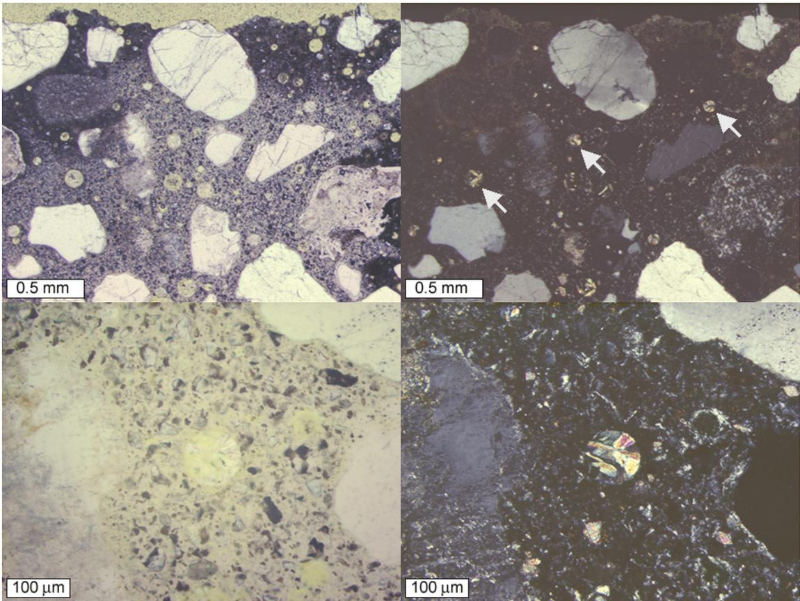
Figure IA-17: Transmitted light (left) and crossed polars (right) images showing  $\text{Ca}(\text{OH})_2$  deposits in air voids just below the pavement wear surface. White arrows in crossed polars image indicate some of the filled voids.
