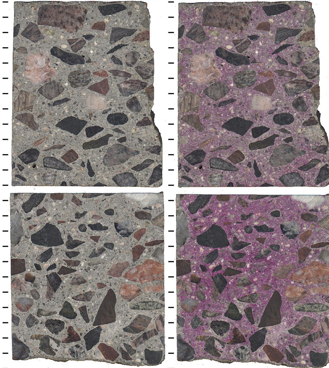
Figure CO-5: Polished slabs to show complete cross-section through core CO-1 both before (left) and after application of phenolphthalein stain (right) tic marks every cm.
