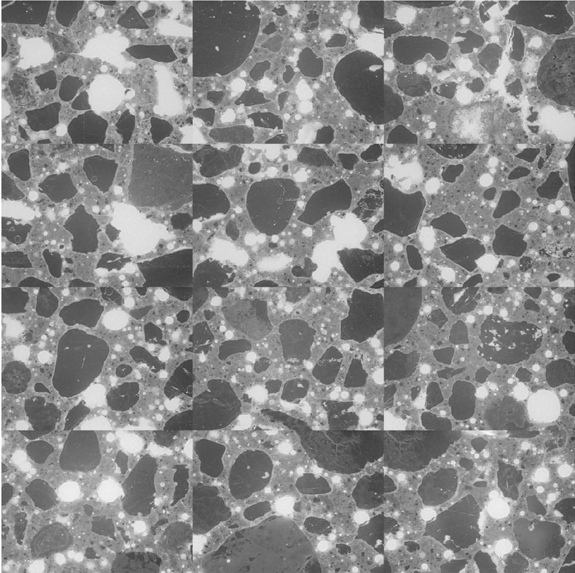
Figure IA-11: Mosaic of 12 frames collected from area of thin section representing the original concrete below the concrete overlay, core IA-11 (each individual frame measures 2.612 x 1.959 mm).
