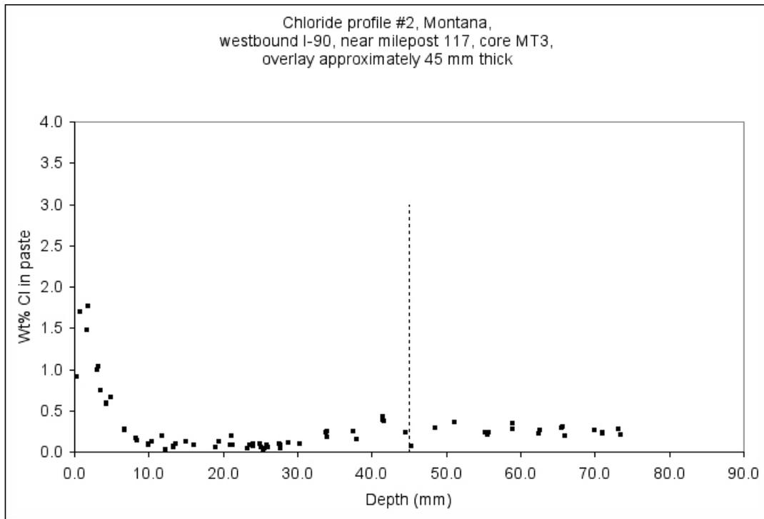
Figure MT-15: Chloride profile through cement paste from billet prepared from core MT-3, dashed line marks the transition between the overlay and the original concrete below.
