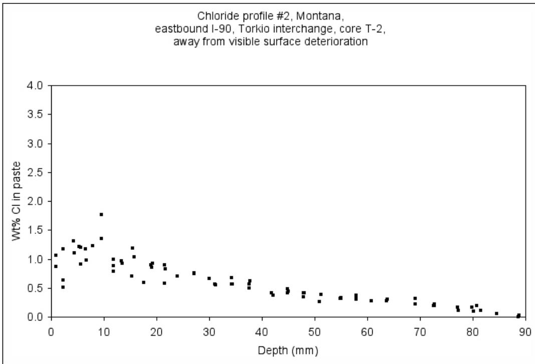
Figure T-11: Chloride profile through cement paste, from billet prepared from core T-2.
