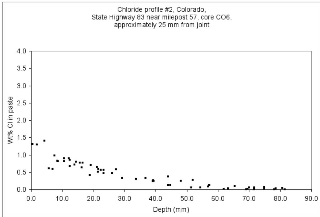
Figure CO-14: Chloride profile through cement paste, from billet prepared from core CO-6.
