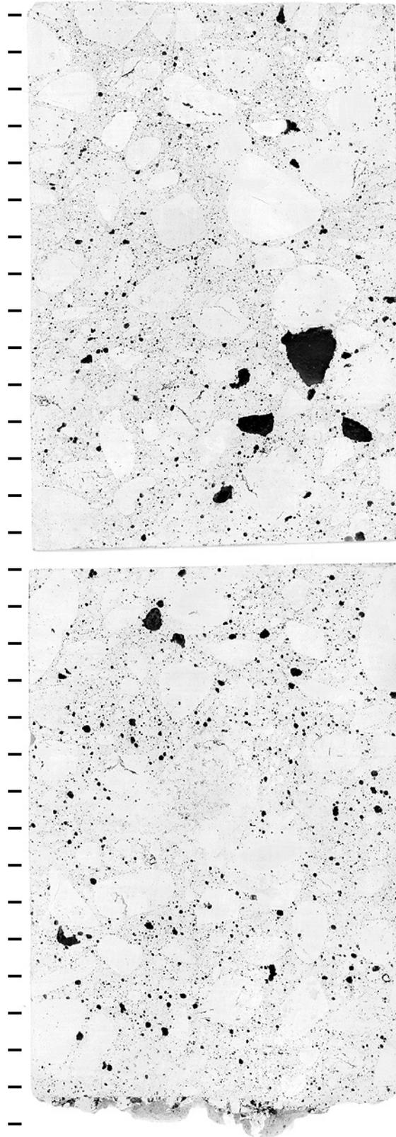
Figure ID-9: Polished slabs to show complete cross-section through core IDL-4 after treatment to enhance appearance of air voids and cracks, tic marks every cm.
