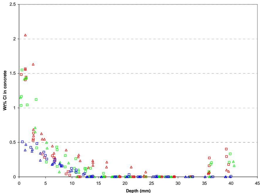
Figure 1. Chloride profiles of 0.45w/c PCC billets in three high concentration deicer solutions.
