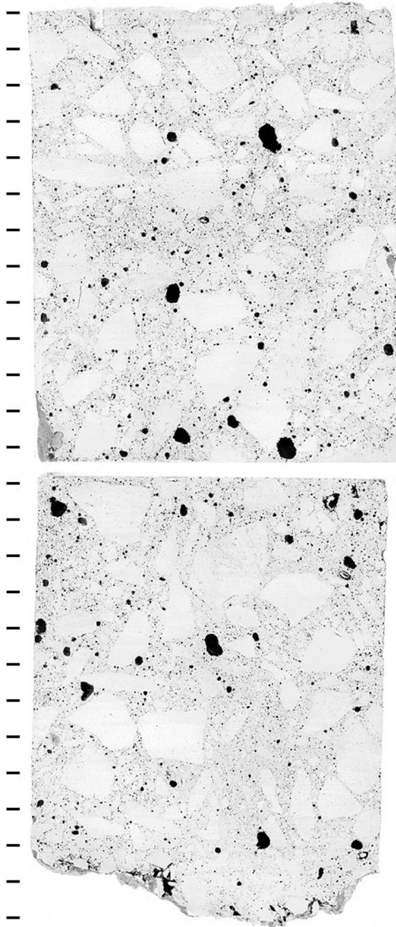
Figure SD-9: Polished slabs to show complete cross-section through core SD-4 after treatment to enhance appearance of air voids and cracks, tic marks every cm.
