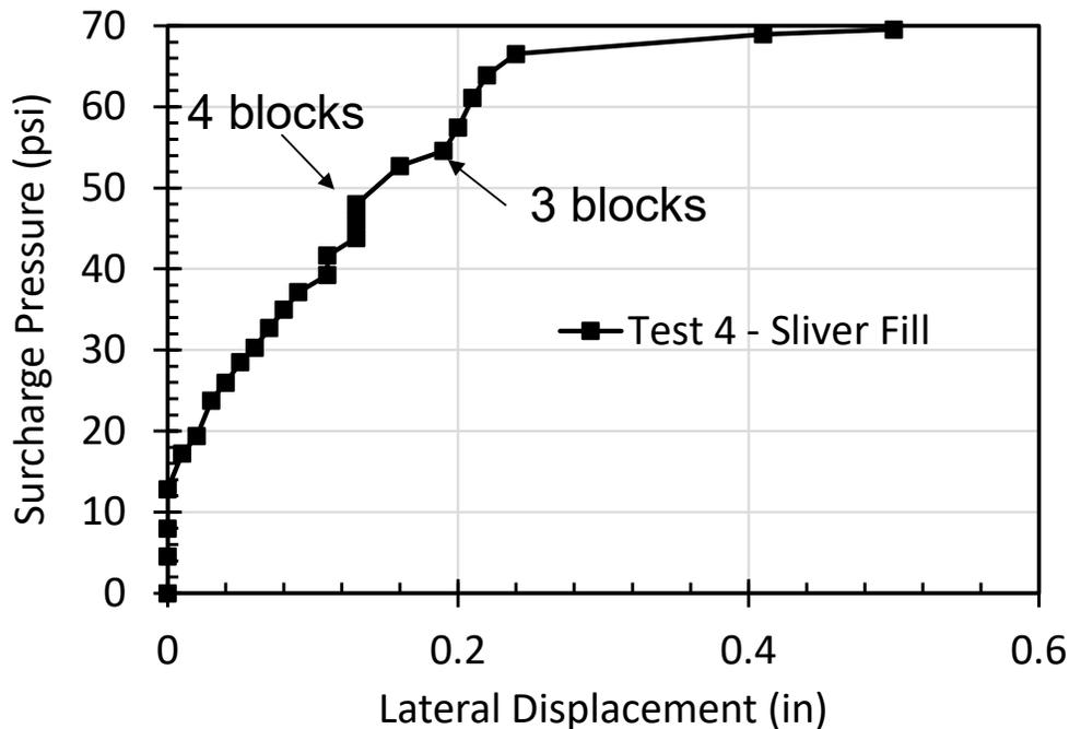
Fig. 5. Applied surcharge pressure vs. lateral displacement at the MSE wall for the sliver fill test.
