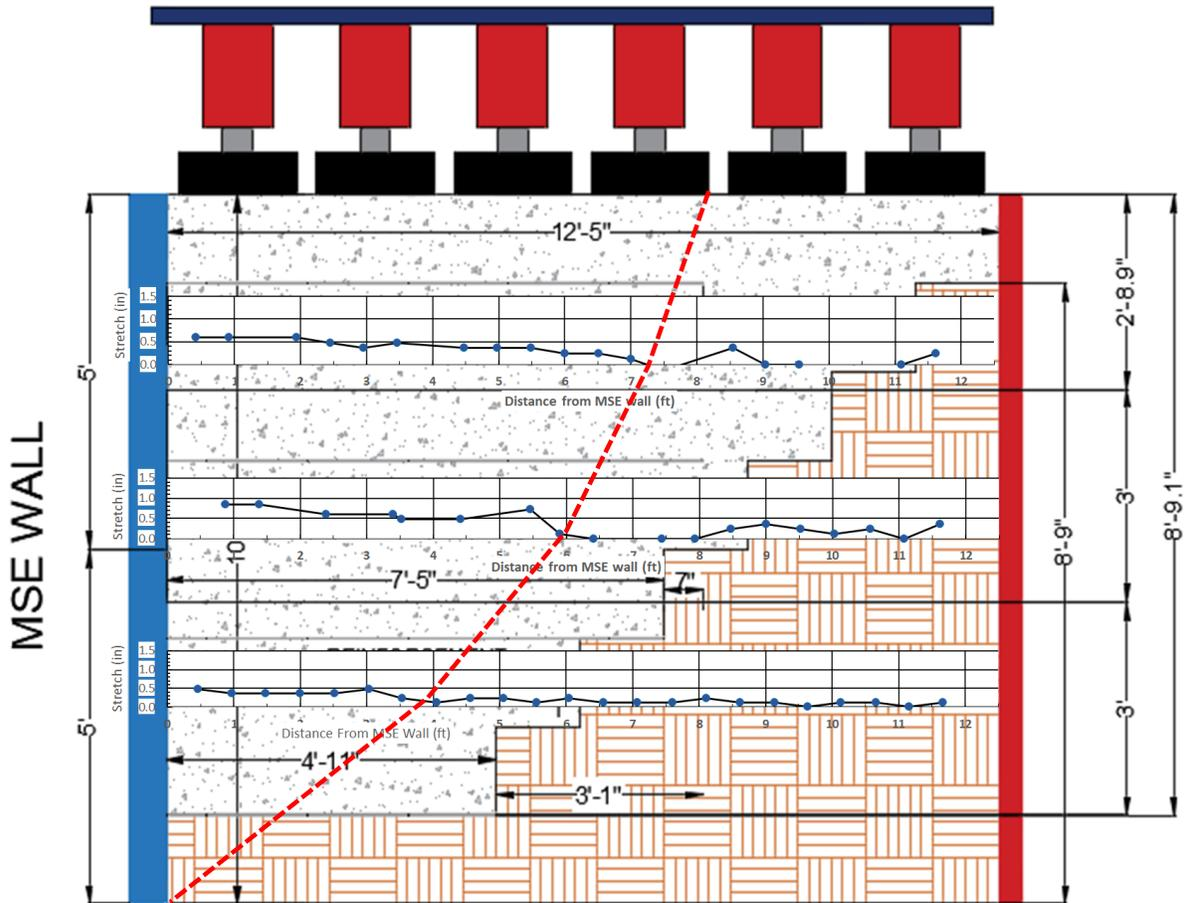
Fig. 10 Cross-section showing elongation vs. distance plots from horizontal Sondex pipes.
