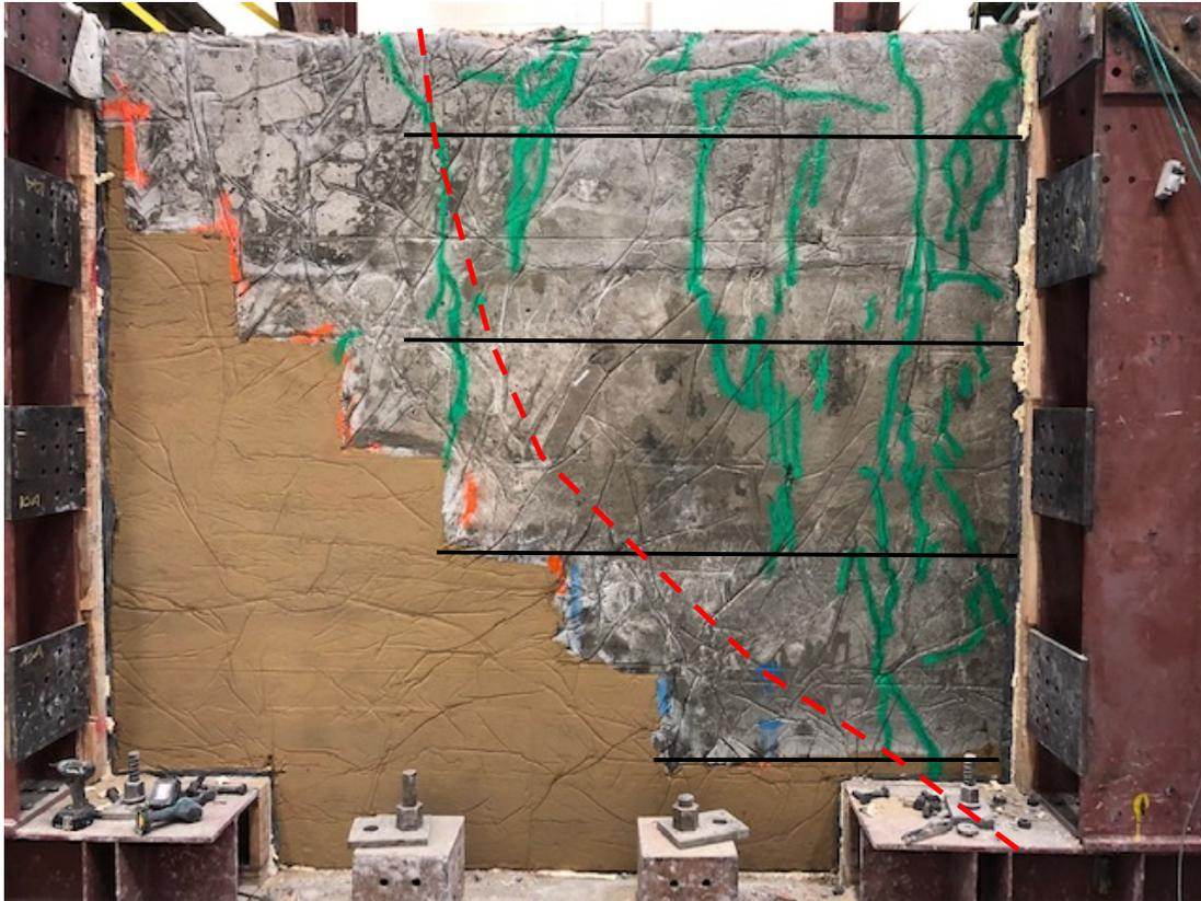
Fig. 11 Photograph showing the green crack patterns adjacent to the MSE wall with the eight-foot wide surcharge load at the surface. Reinforcement locations are shown by horizontal black lines. Red dashed line is boundary of extension from Sondex measurements.
