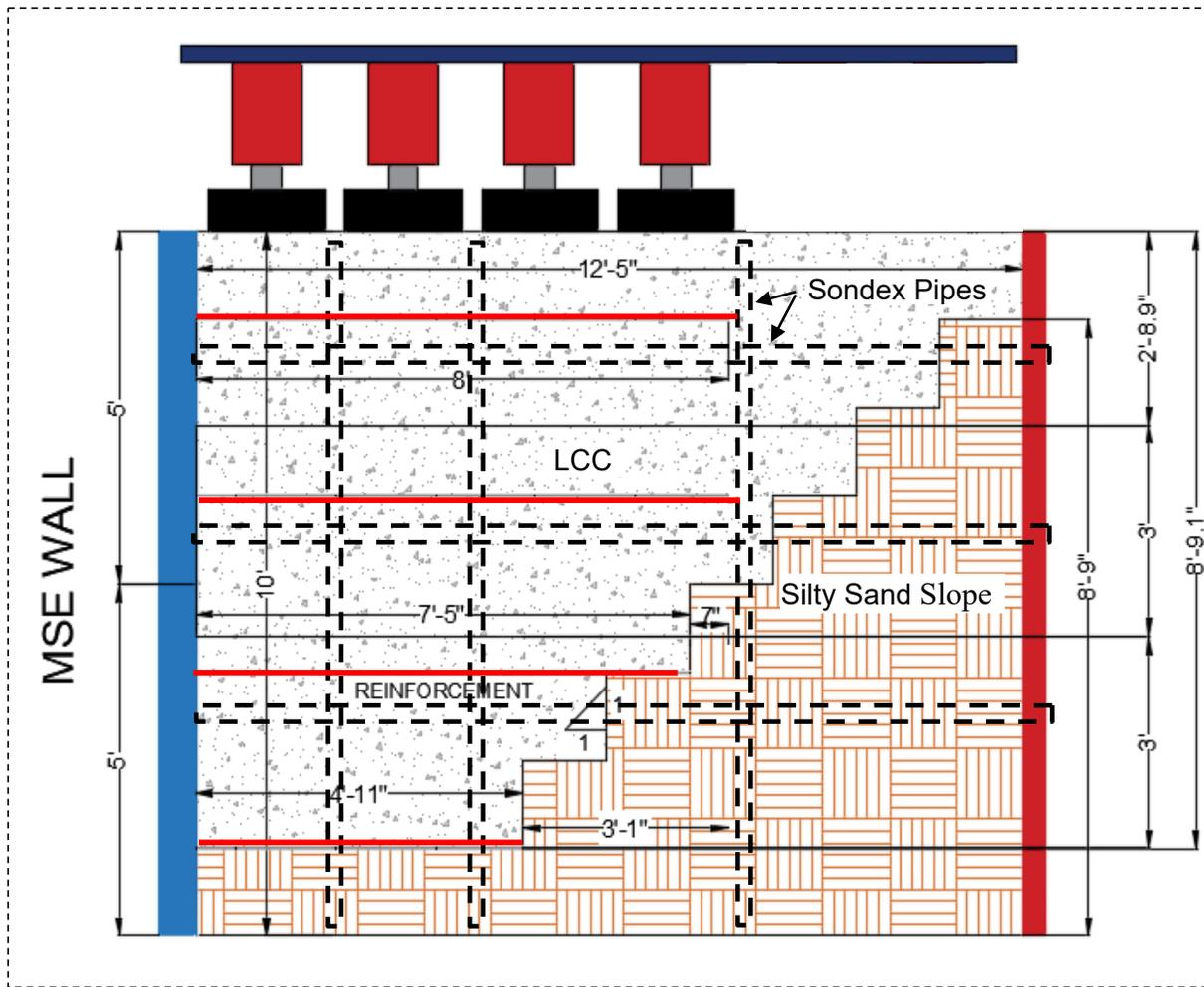
Fig. 1. Schematic profile drawing of the test involving MSE wall with sliver fill of reinforced LCC adjacent to 1:1 stair-stepped silty sand slope. Note: MSE reinforcements in red along with vertical and horizontal corrugated Sondex pipes shown by dashed black rectangles.
