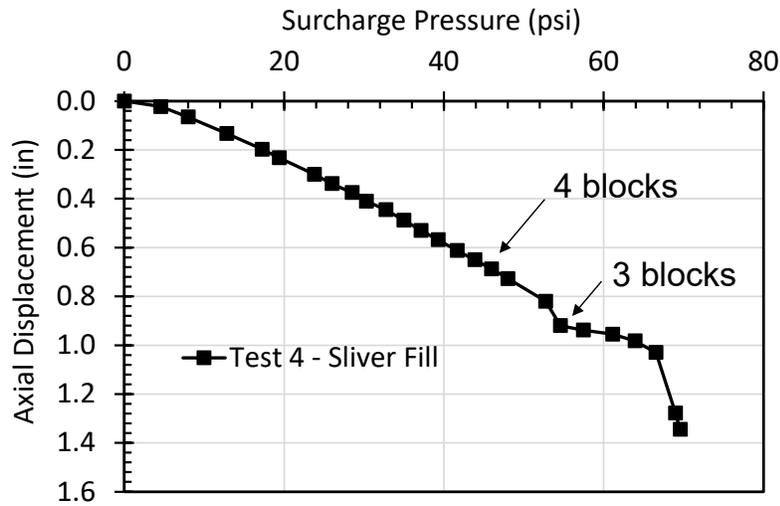
Fig. 3. Applied surcharge pressure versus axial displacement for the sliver fill test.
