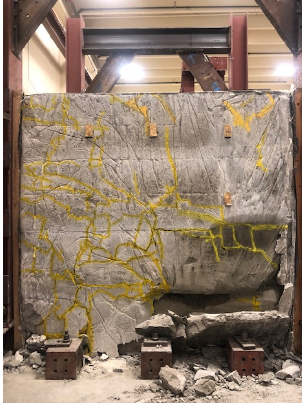
Fig. 13. Photograph of the crack pattern in the LCC on the free face opposite to the cantilever retaining wall side.
