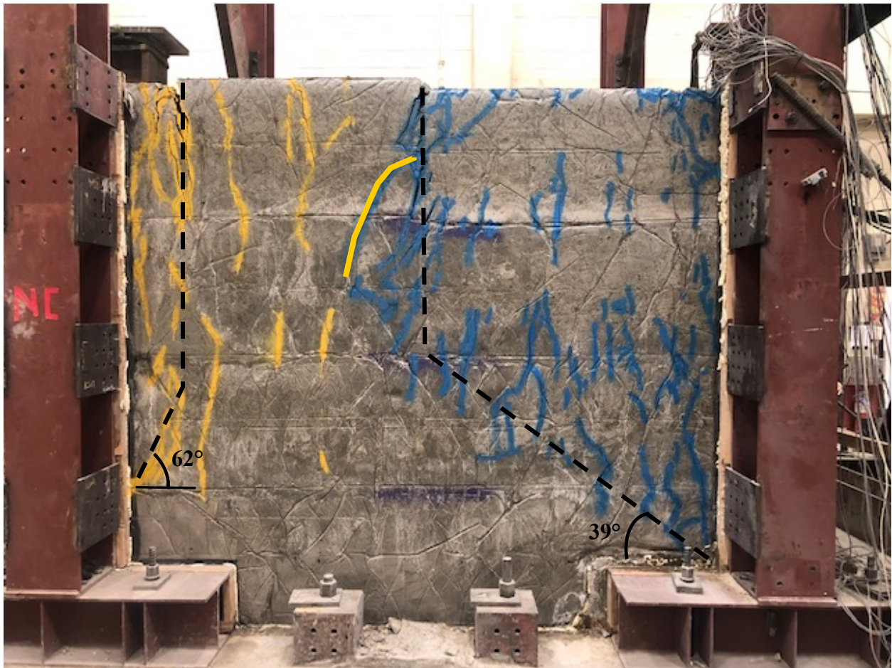
Fig. 11. Photo showing the blue crack patterns adjacent to the cantilever wall with the six-foot wide surcharge load at the surface. Yellow crack patterns are for a second test with six-foot wide surcharge adjacent to free-face without retaining wall.
