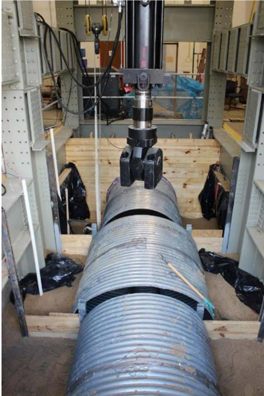
Figure A 16: 3 CMPs inside the Soil Box
