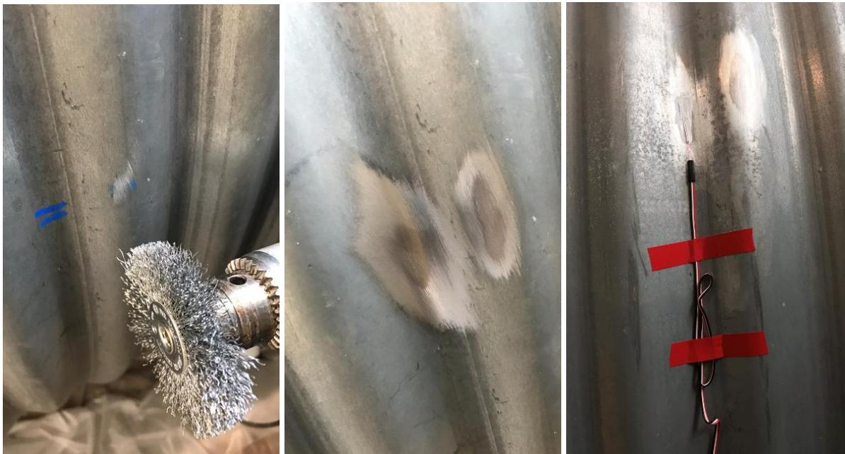
Figure A 9: Surface Preparation for Attaching Strain Gauges
