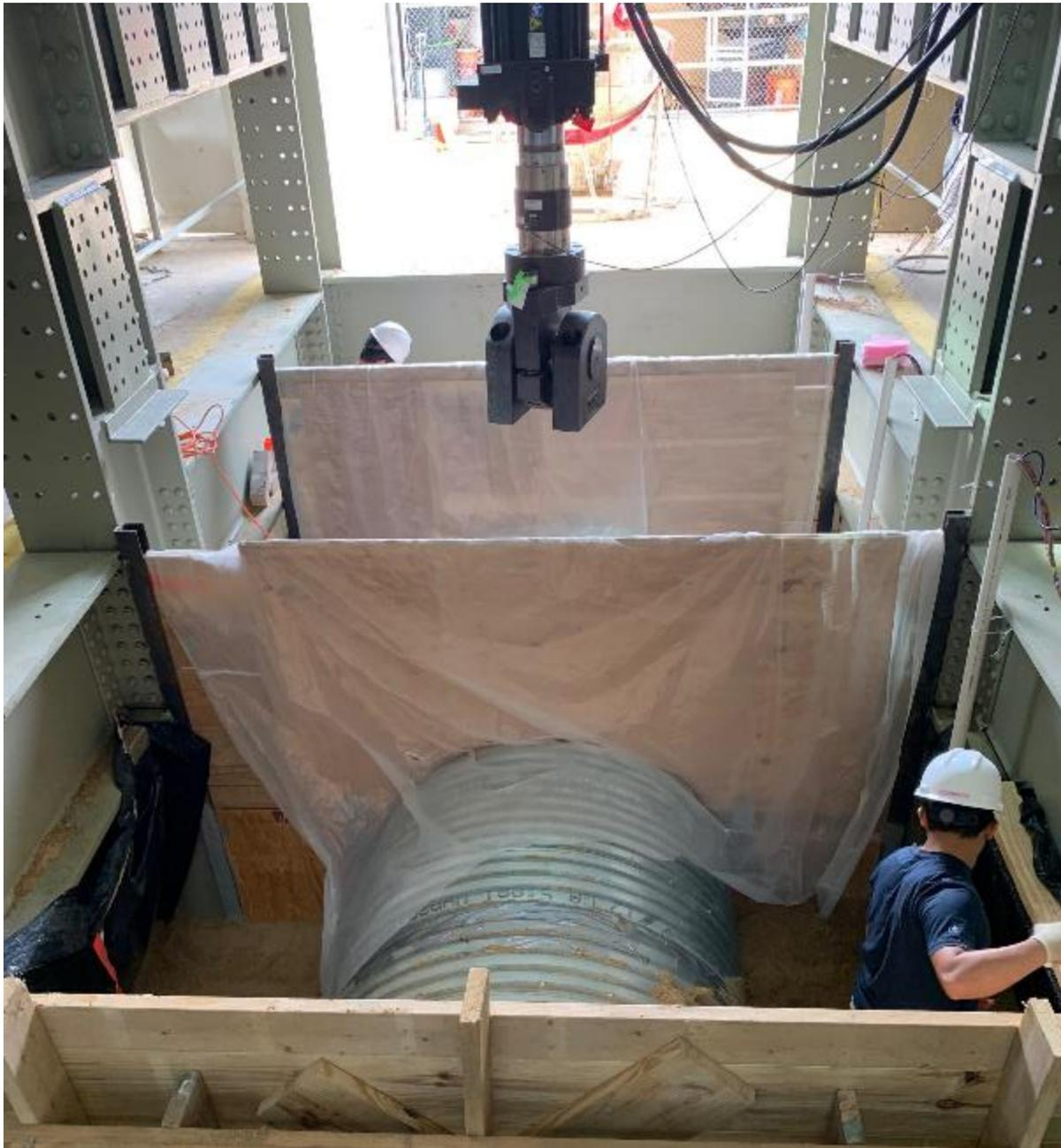
Figure A 17: Completion the Installation of Partition Walls and Placing Plastic Sheets
