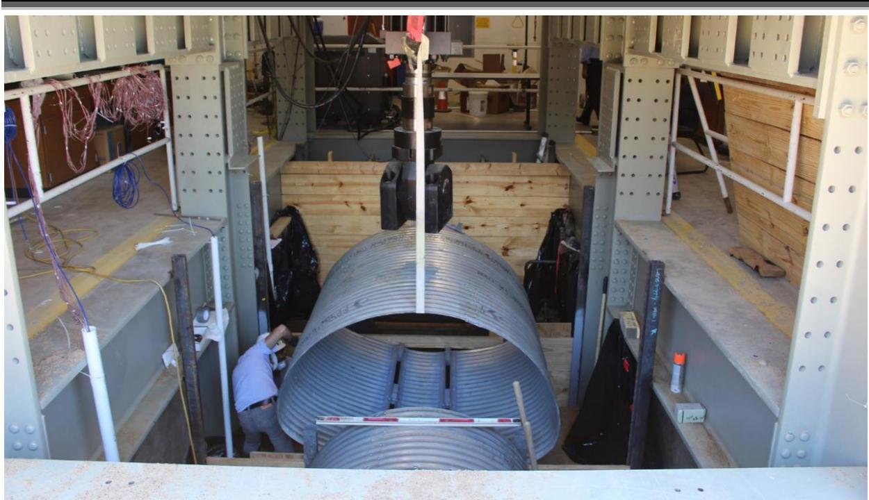
Figure A 13: Placing Arch CMP
