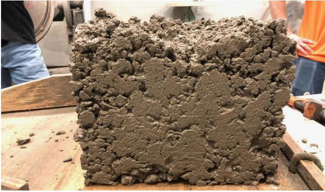
**Figure 2.7.4 shows the sample from the Box Test.**
