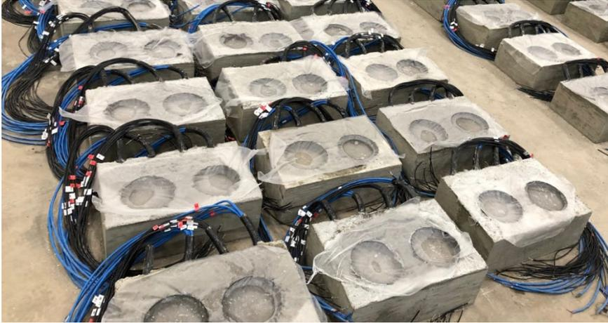
**Figure 3.4.4 – An overview of the mortar samples being prepared and also surrounded by the concrete cover and ready for the instrumentation box.**
