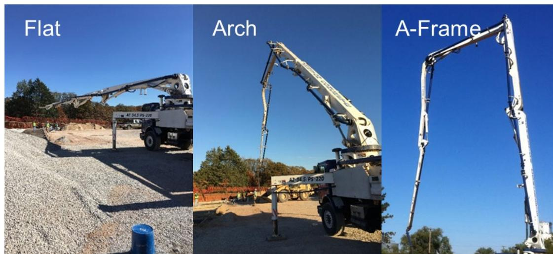
**Figure 2.6.1. The flat, arch, and A-Frame orientations of the concrete pump.**
