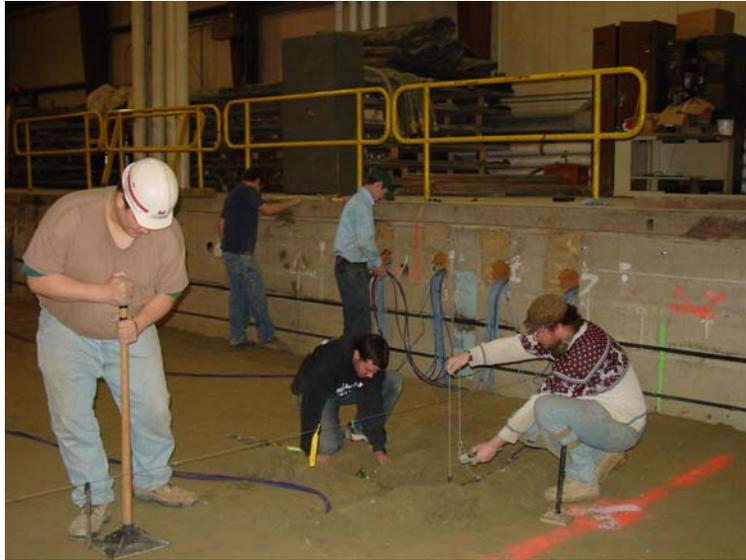
**Figure 19. Image of instrumentation installation, showing wire extended across the test basin for the purpose of precisely locating sensors.**
