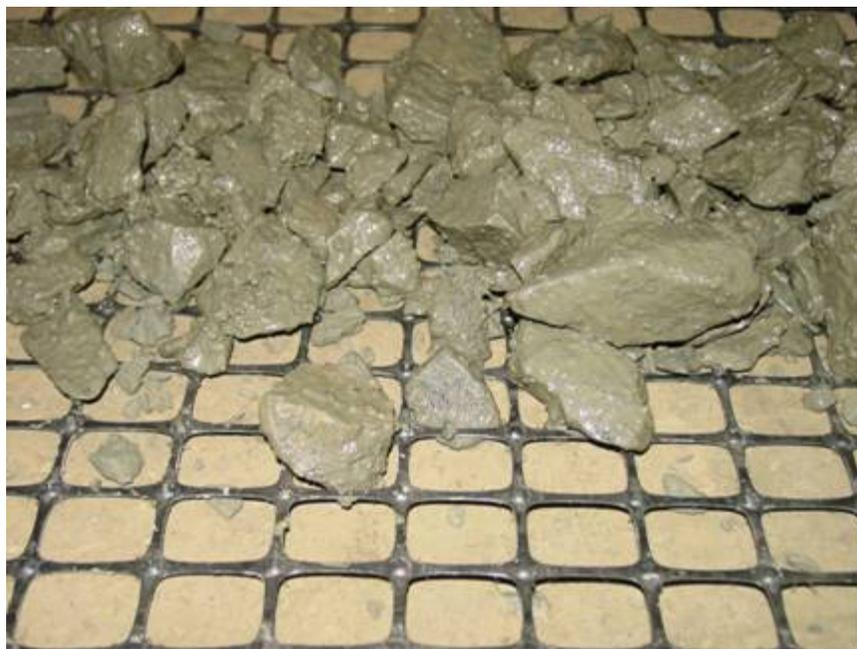
**Figure 25. Close-up of geogrid and base aggregate particles.**
