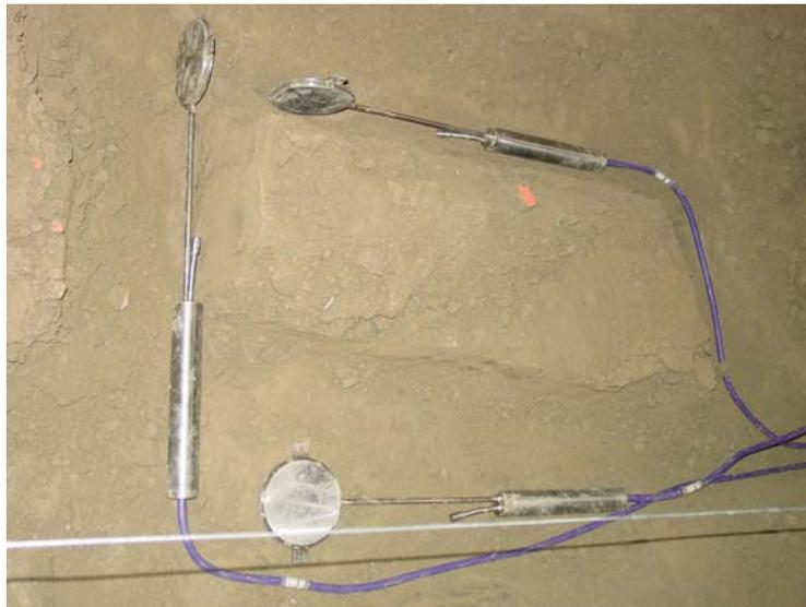
**Figure 20. Image (top view) of pressure cells during installation showing trenches and cable.**
