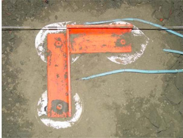
**Figure 21. Image of installation mold for placement of three  $\epsilon$ mu coils.**
