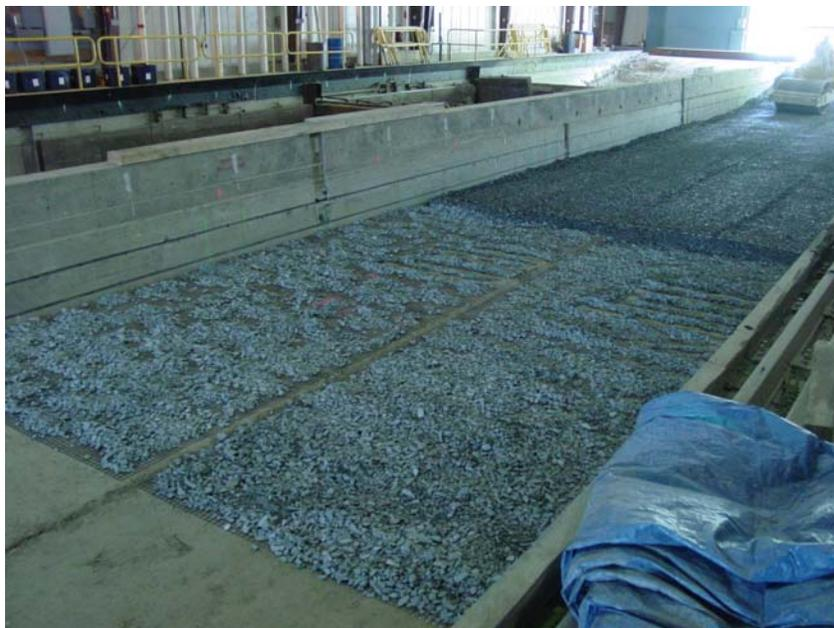
**Figure 24. Geogrid partially covered with base course aggregate.**
