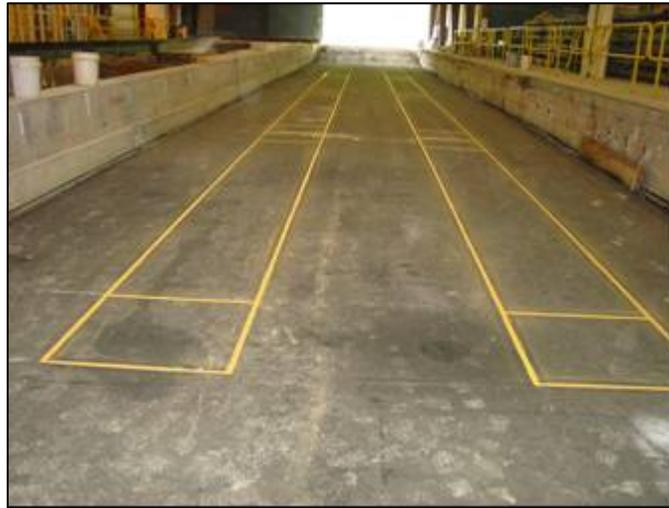
**Figure 3. Paved test sections showing test windows (outlined in yellow) to which traffic was applied, including the short transition sections. Traffic was applied in a direction away from the viewer of this image.**
