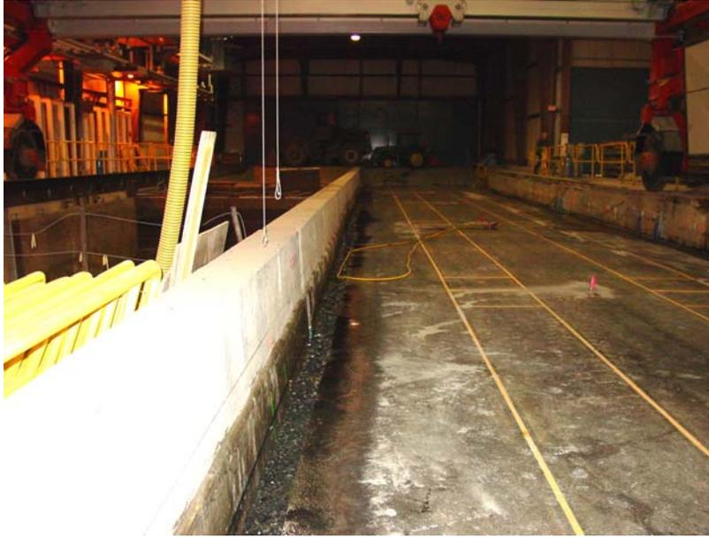
**Figure 30. Image showing trench formed by asphalt removal from the edge of the test basin. Water was added to the base layer exposed in the trench to decrease the stiffness of the subgrade layer.**
