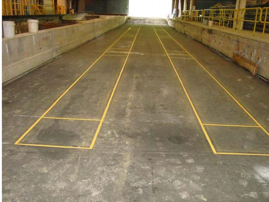
**Figure 29. Paved test sections and marked test windows. The traffic was applied in the direction away from the viewer, hence the loading transition zone is in the foreground of the image.**
