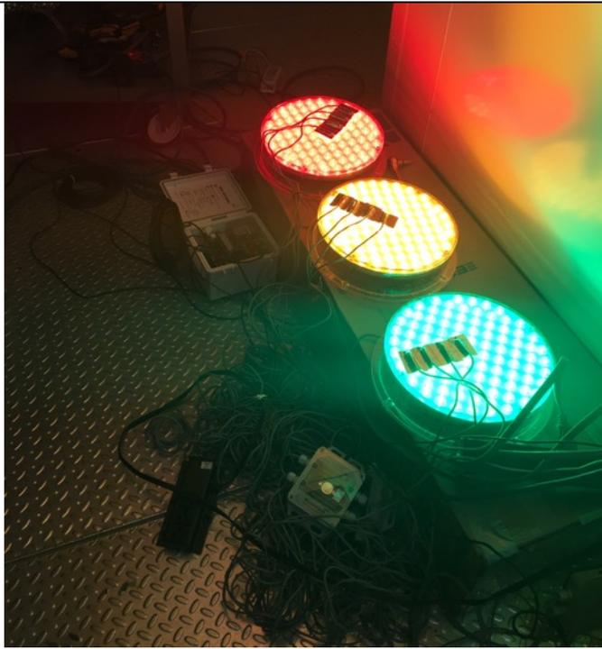
**Figure 4** The tests of the fourth generation of prototype signals in the cold room, to double check the switching performance of the ambient air temperature sensor attached to each signal.
