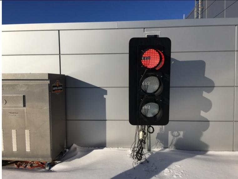
**Figure 2** In real-time snowy winter, the closed-course performance and reliability tests of the fully working prototypes mounted on the roof of M2SEC building. The roof tests will be continuously conducted in 2019 with necessary real-time adjustments.
