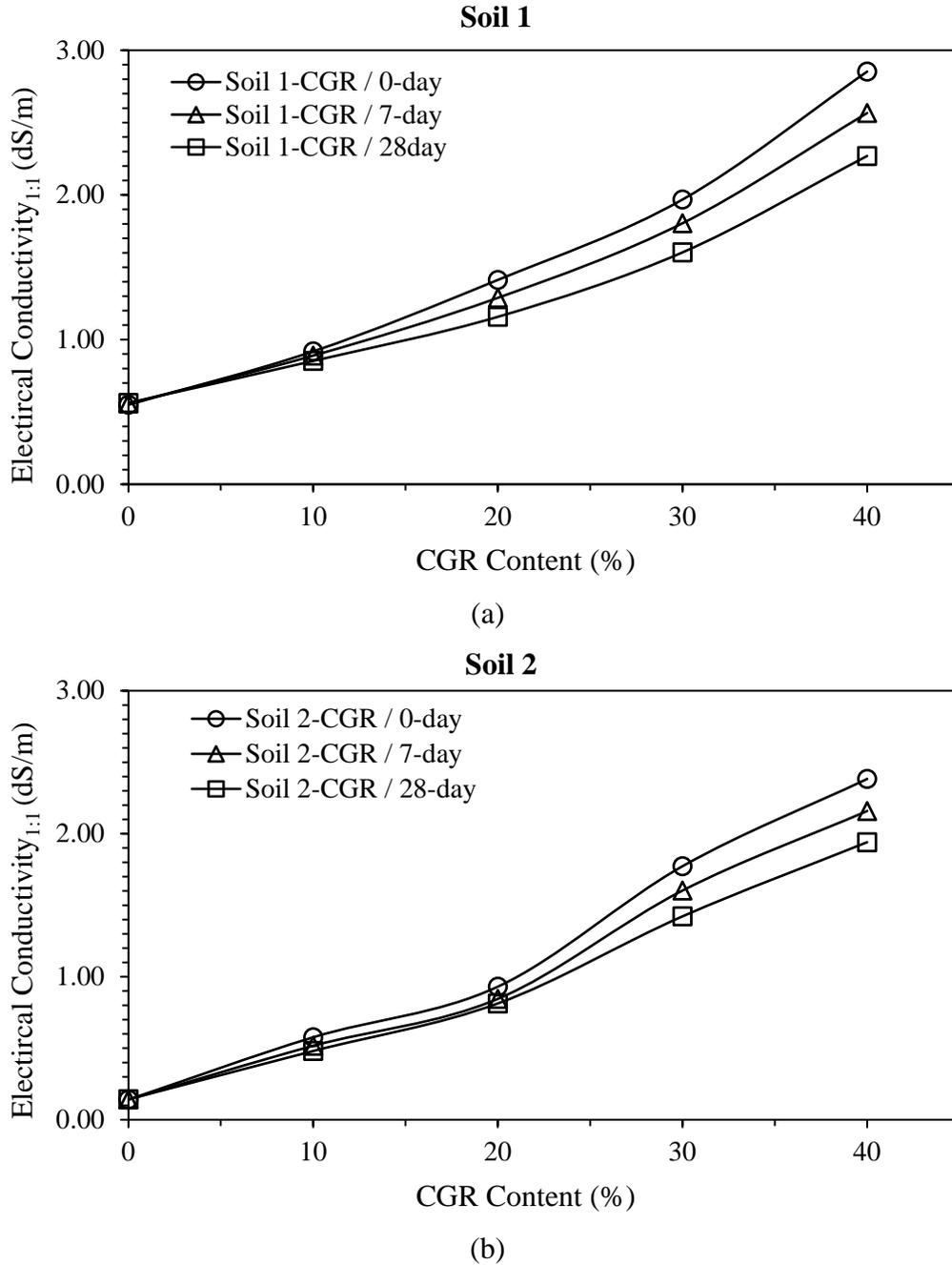
**Figure 30. Effects of CGR on soil electrical conductivity.**
