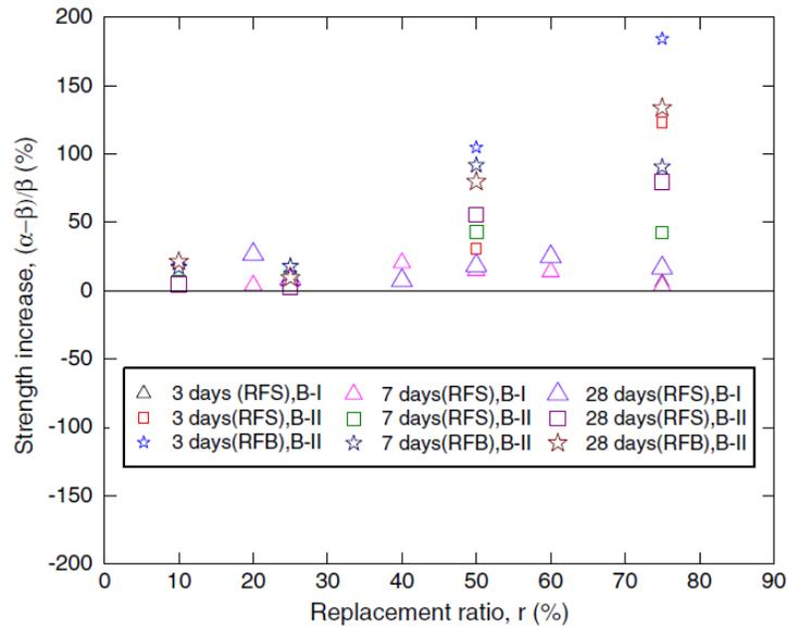
**Figure 4. Percentage strength increases caused by replacement of recycled fines from brick aggregate concrete (RFB) and stone aggregate concrete (RSB) at different ages (Amin et al., 2016 (14)).**
