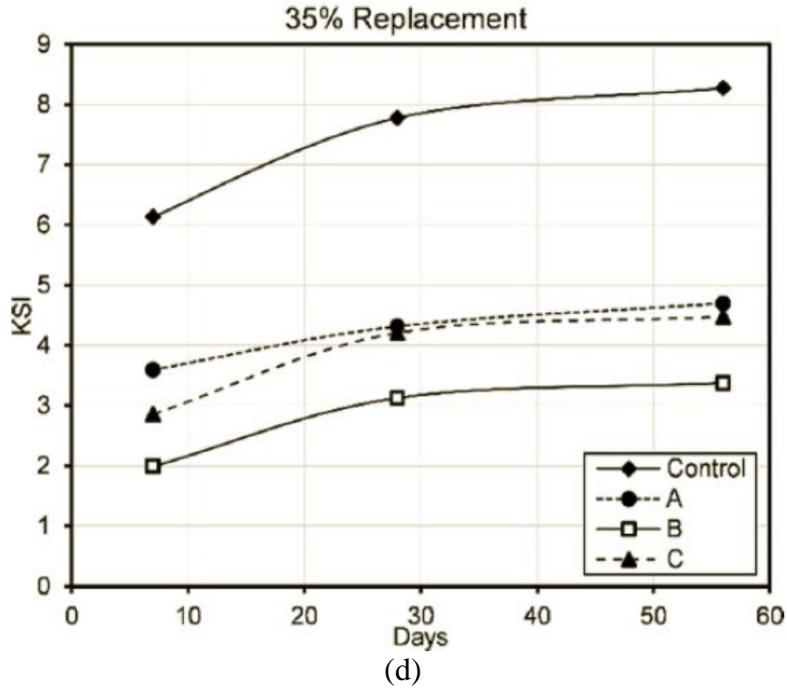
**Figure 3. Three CGR samples (A, B and C) were used as cement replacements in 2-inch cubes and subjected to compressive strength tests (Kluge et al., 2018 (10)).**
