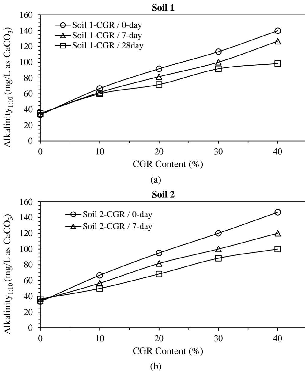
**Figure 31. Effects of CGR on soil alkalinity.**
