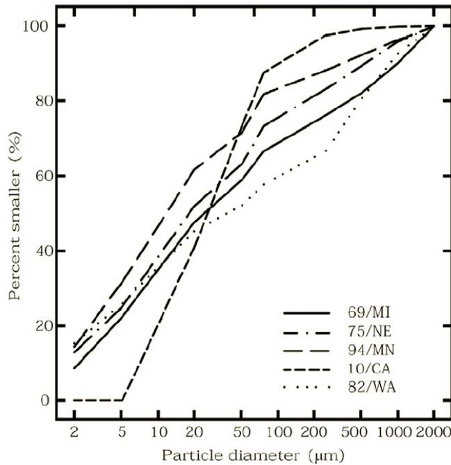
**Figure 1. Particle size distributions for five CGR samples from five roadway sites (DeSutter et al., 2010 (2)).**
