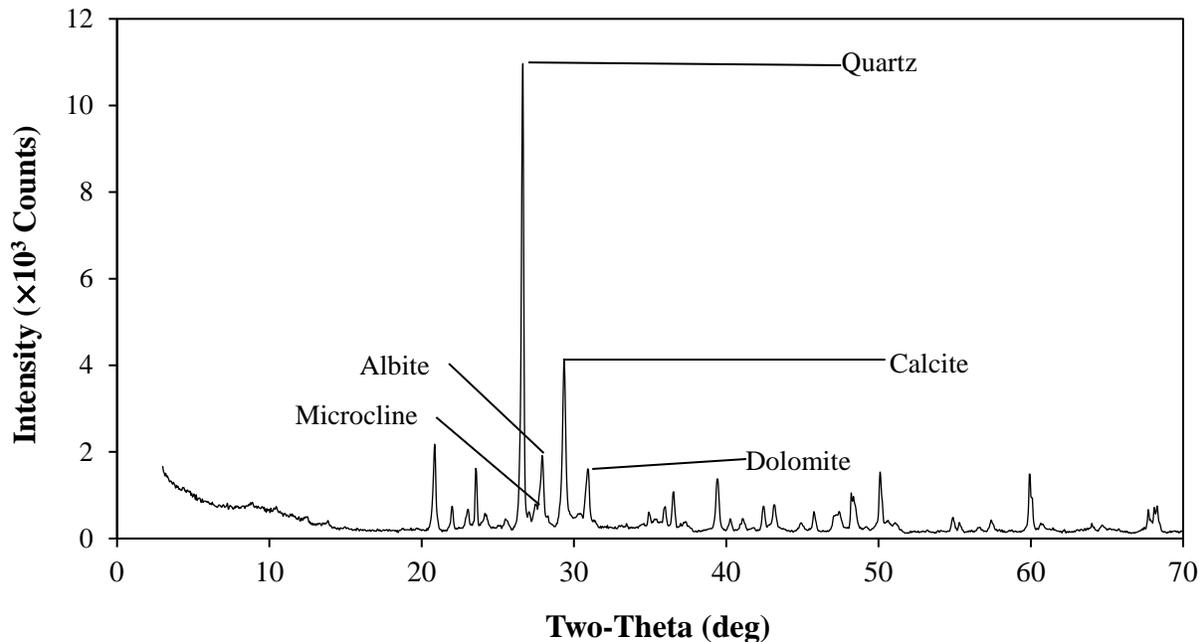
**Figure 25. X-ray diffraction pattern for CGR.**
