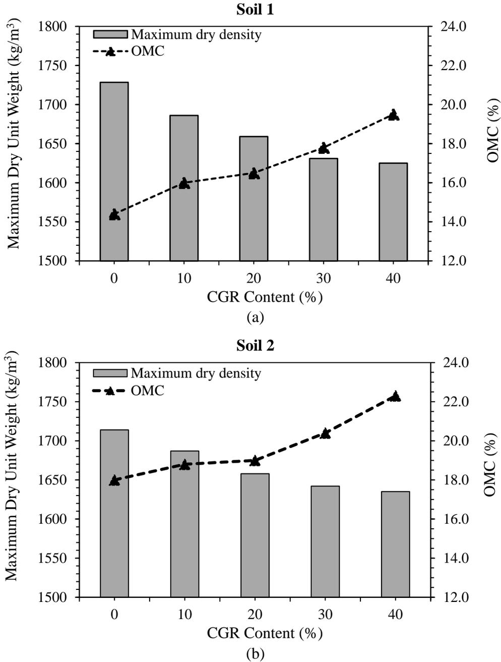
**Figure 27. Effects of CGR on moisture-density relationship of (a) Soil 1 and (b) Soil 2.**
