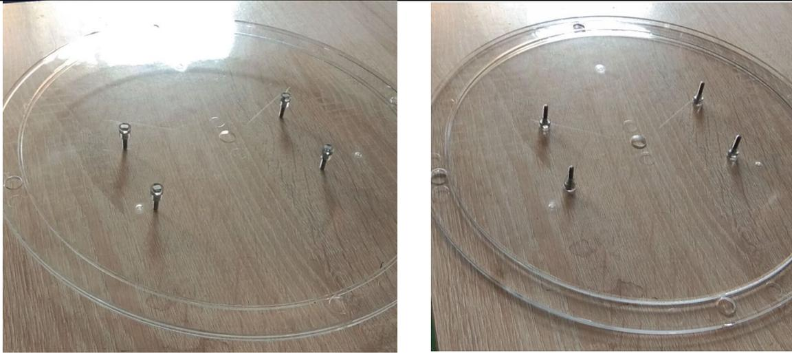
**Figure 5** Samples the finalized design of the new housing of the fully working prototype signals of Type 1, prepared for field tests, with changes made to accommodate new screws, new LED drivers, adding a temperature sensor mounting hole in the side surface of part 1 for mounting temperature sensors, and improvement of the surface smoothness during molding process of part 1 with 96 niches for mounting Fresnel lenses.
