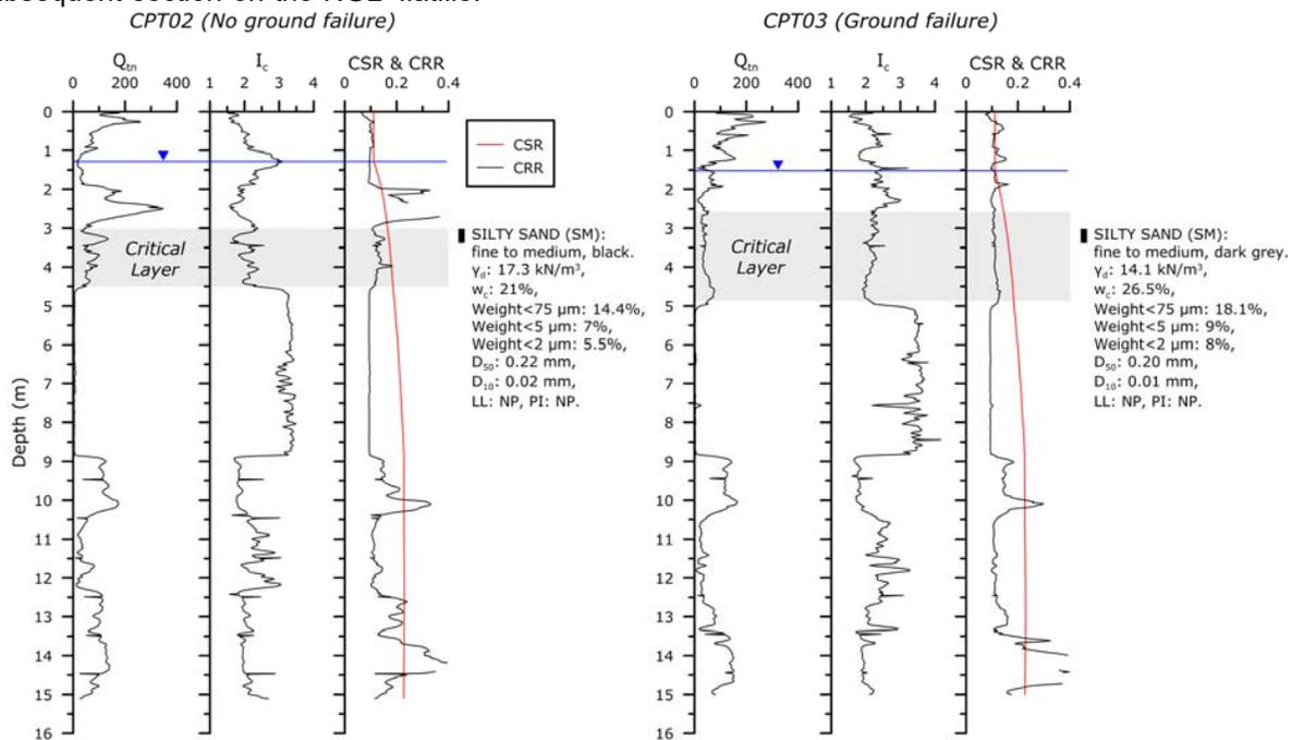
**Figure 2.** Normalized CPT resistance ( $Q_{tn}$ ), soil behavior type index ( $I_c$ ), cyclic stress ratio (CSR) and cyclic resistance ratio (CRR) profiles on the location of no ground failure and ground failure. Laboratory index test results from the samples retrieved by a CPT sampler are indicated.
