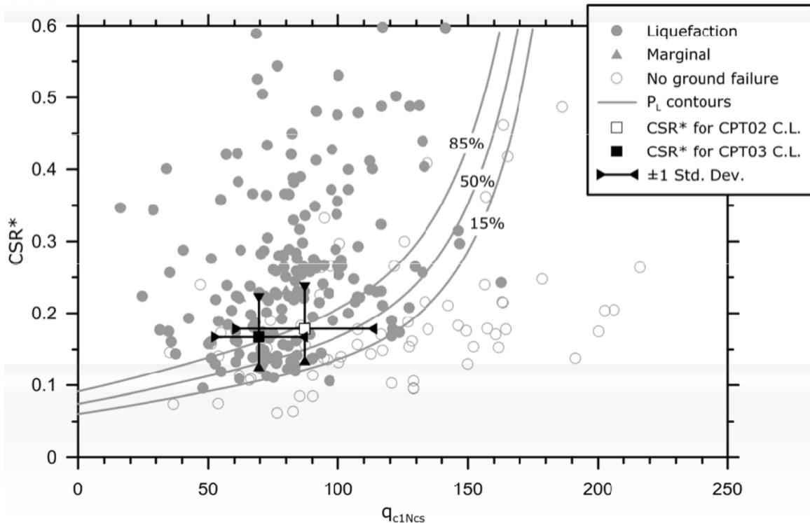
**Figure 3.** Liquefaction triggering database showing  $CSR^*$  vs.  $q_{c1Ncs}$  and  $CRR_{M7.5, \sigma' = 1atm}$  for 15, 50, and 85% probabilities of liquefaction (after Boulanger and Idriss, 2014). Data points for critical layers and  $\pm 1$  standard deviations of  $CSR^*$  and  $q_{c1Ncs}$  are shown for no ground failure (CPT02) and ground failure (CPT03) locations at example site in Urayasu, Japan.
