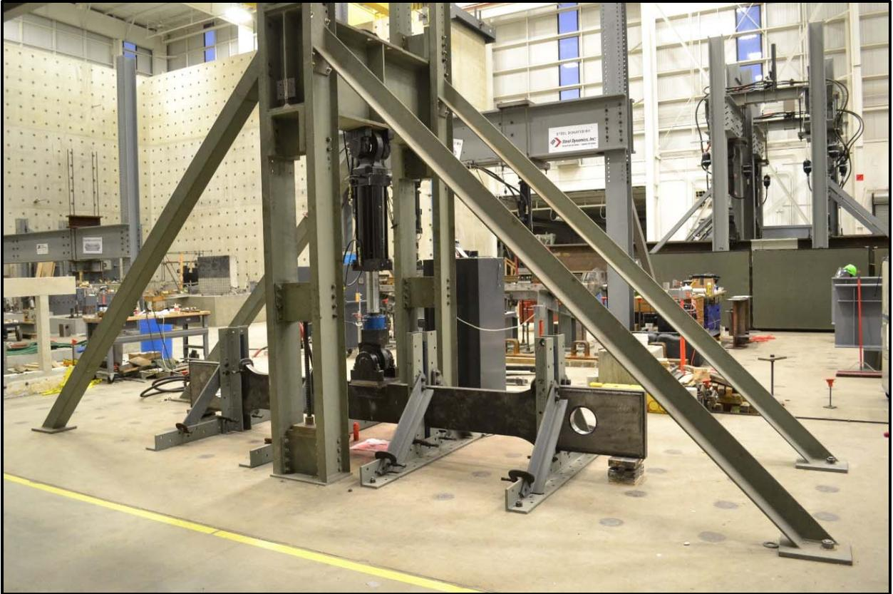
**Figure 3.21: Axial test fatigue setup**
