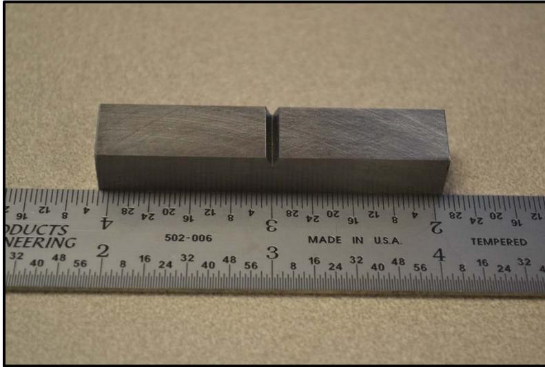
**Figure 3.3: Type A, 10 mm Charpy v-notch impact specimen**
