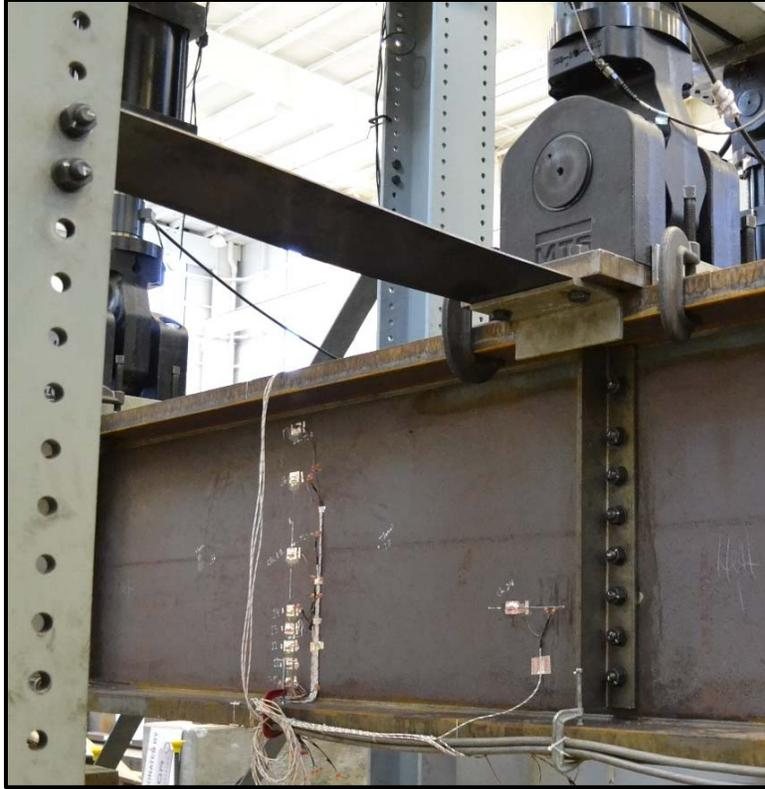
**Figure 3.19: Lateral torsional buckling bracing**
