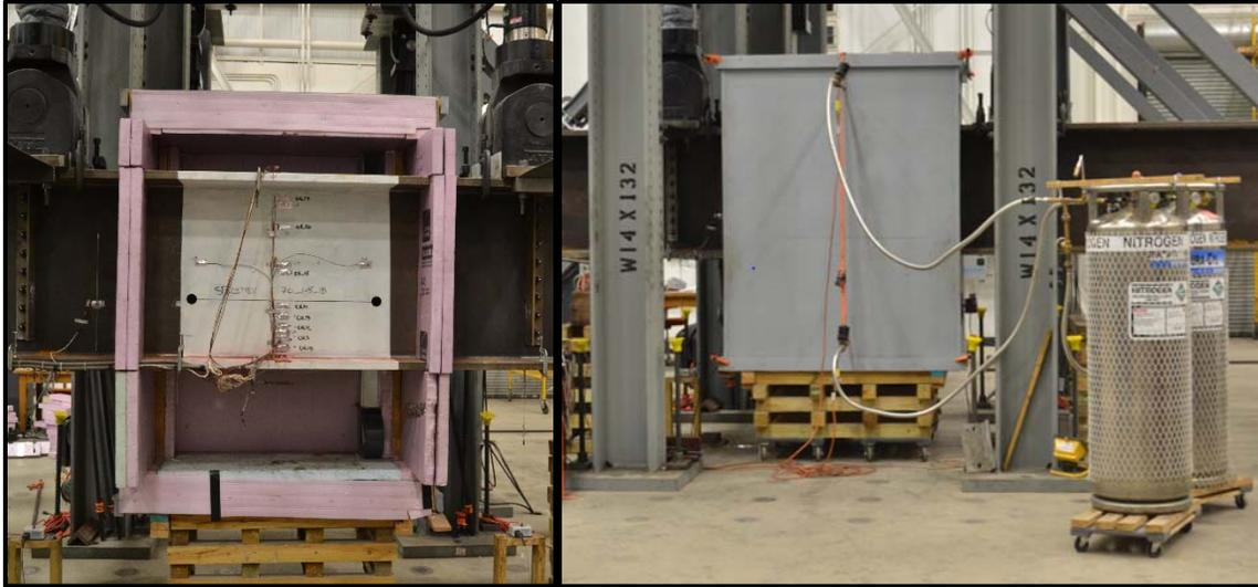
**Figure 3.33: Bending temperature chamber**
