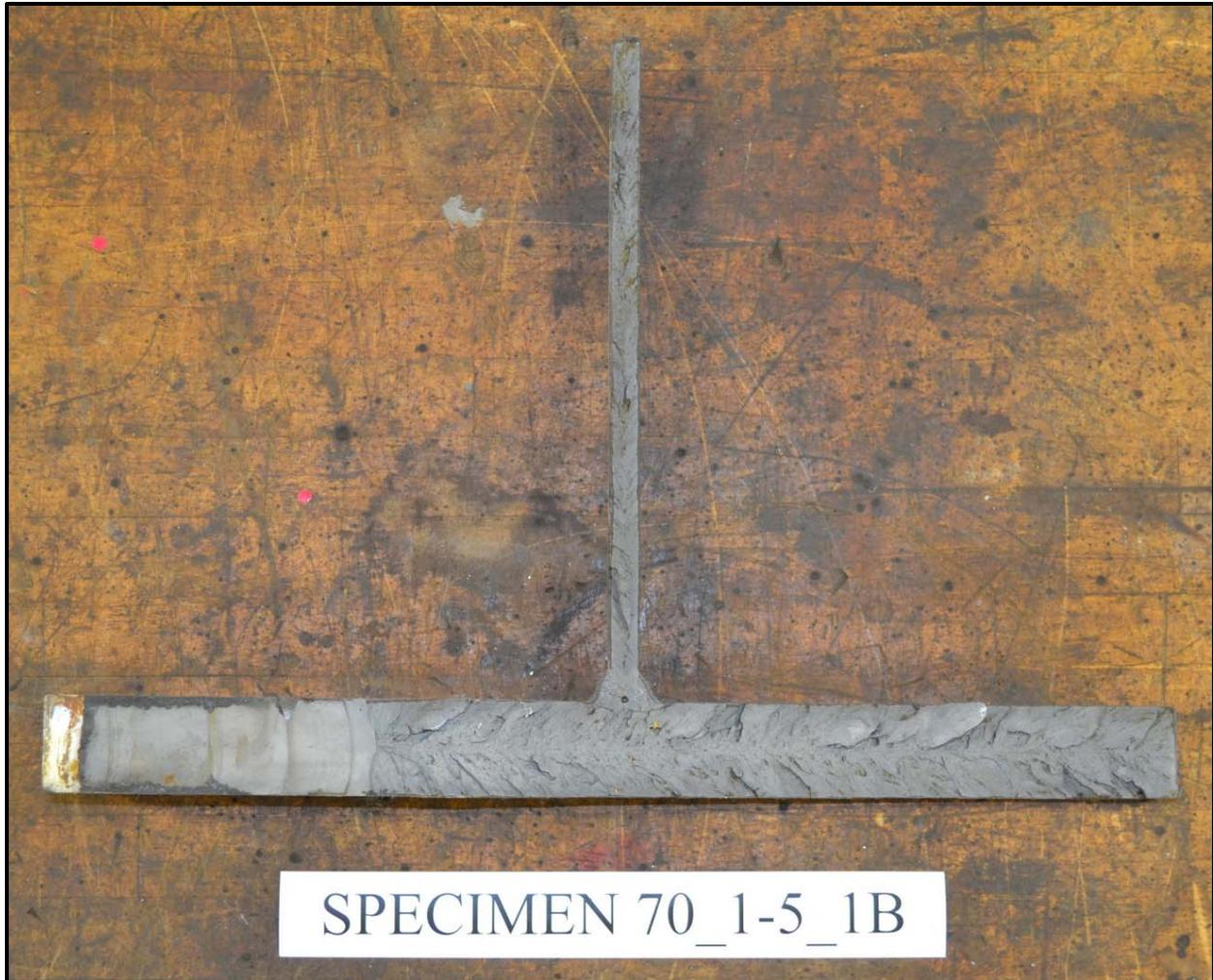
**Figure 3.48: Specimen 70\_1-5\_1B fracture surface**
