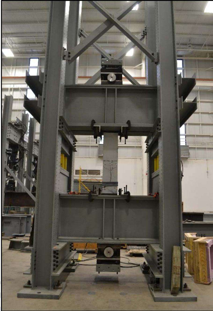
**Figure 3.24: Axial test fracture setup**
