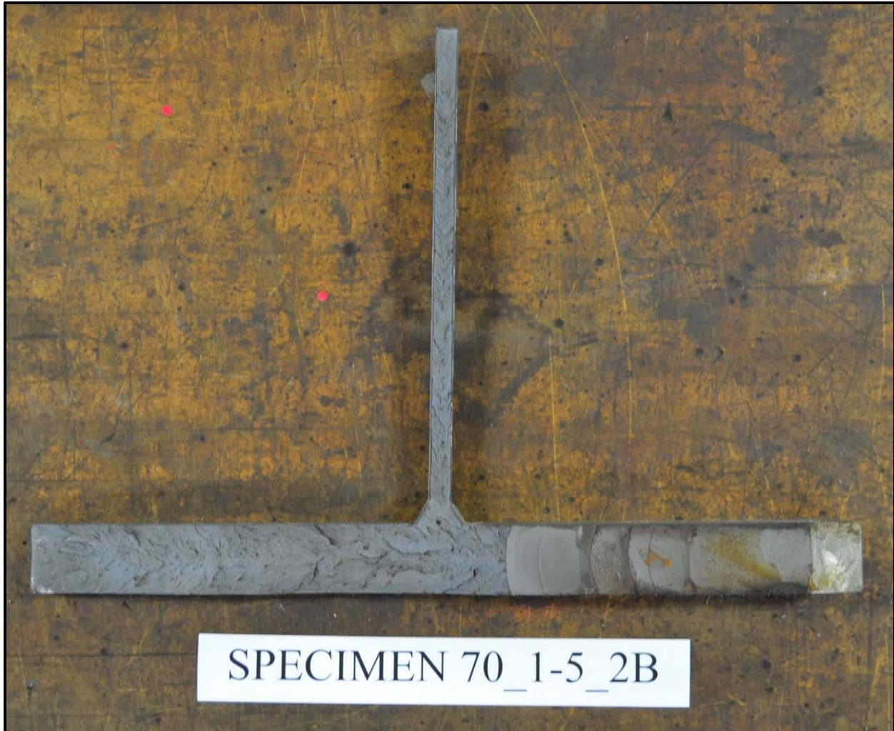
**Figure 3.50: Specimen 70\_1-5\_2B fracture surface**
