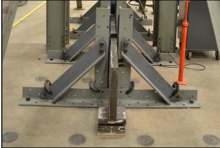
**Figure 3.22: Axial fatigue test setup lateral bracing**
