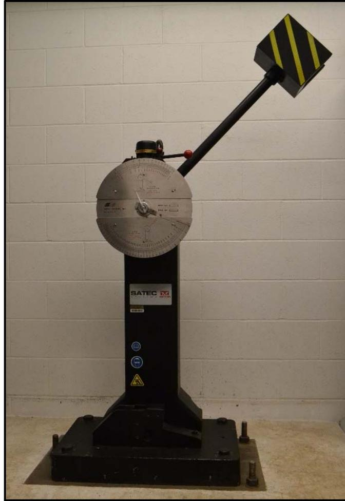
**Figure 3.4: SATEC Series Impact Testing Machine**
