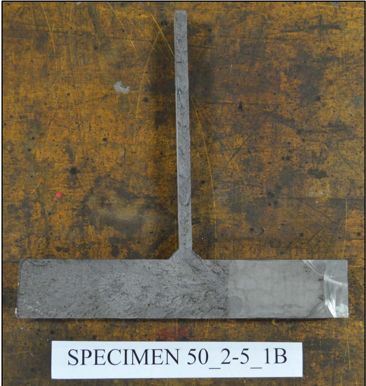
**Figure 3.44: Specimen 50\_2-5\_1B fracture surface**
