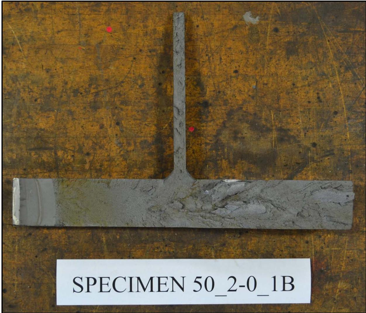
**Figure 3.39: Specimen 50\_2-0\_1B fracture surface**
