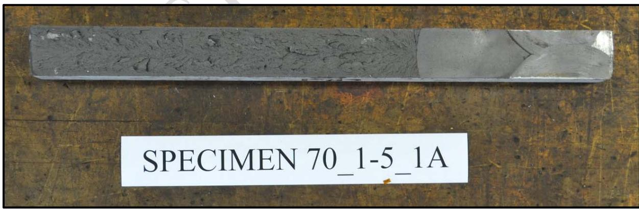
**Figure 3.58: Specimen 70\_1-5\_1A fracture surface**
