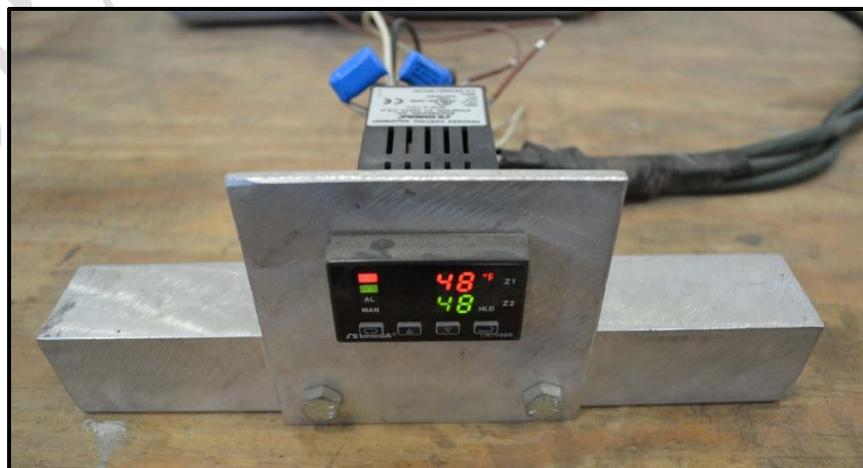
**Figure 3.32: Dual zone temperature controller**
