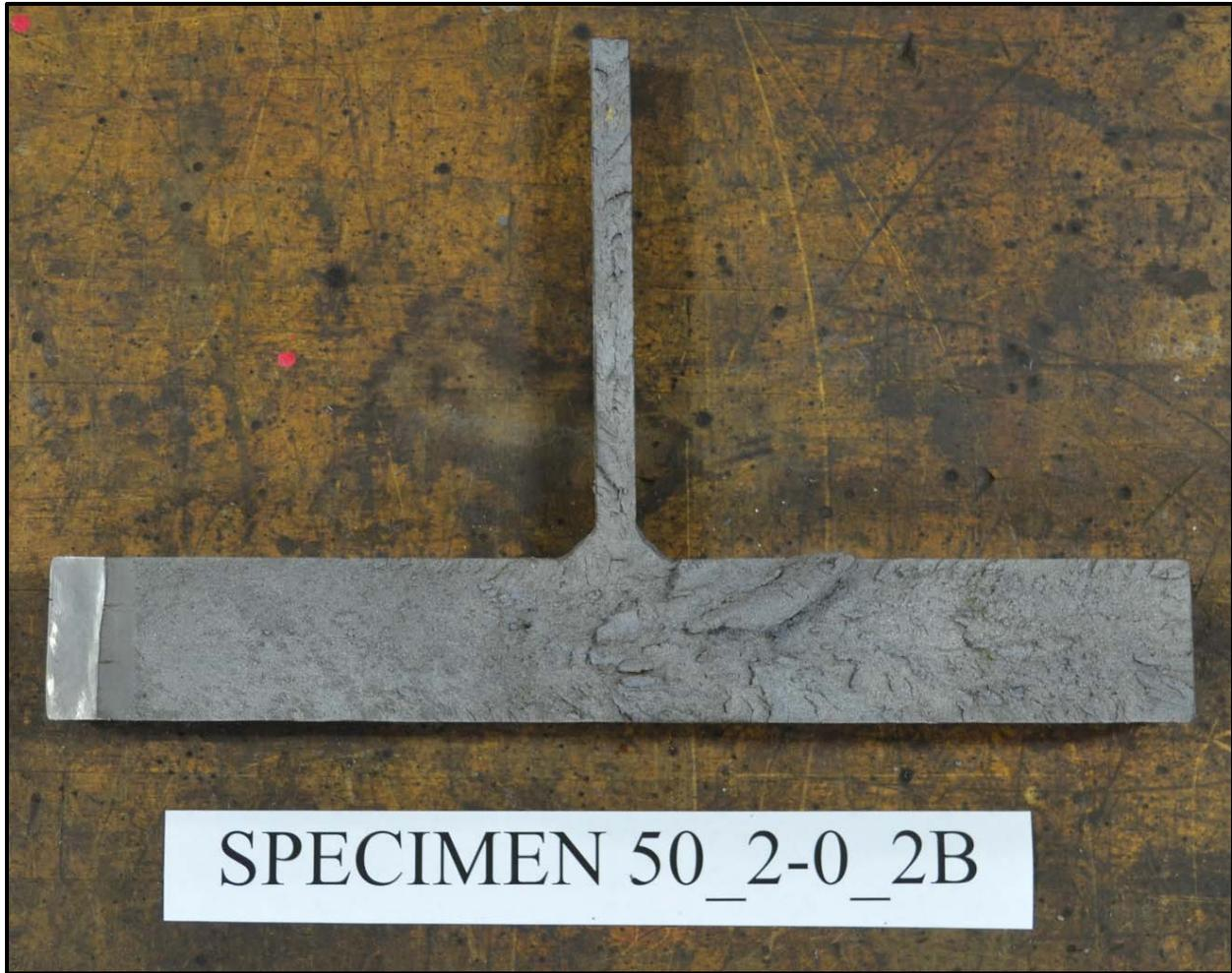
**Figure 3.41: Specimen 50\_2-0\_2B fracture surface**
