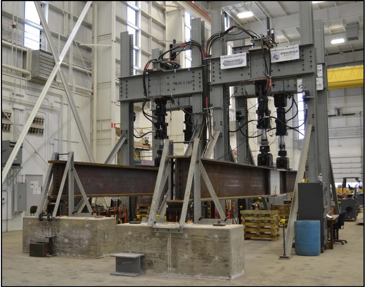
**Figure 3.16: Twin bending test setups**
