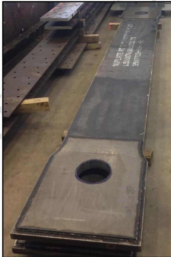
**Figure 3.14: Representative axial test specimen**
