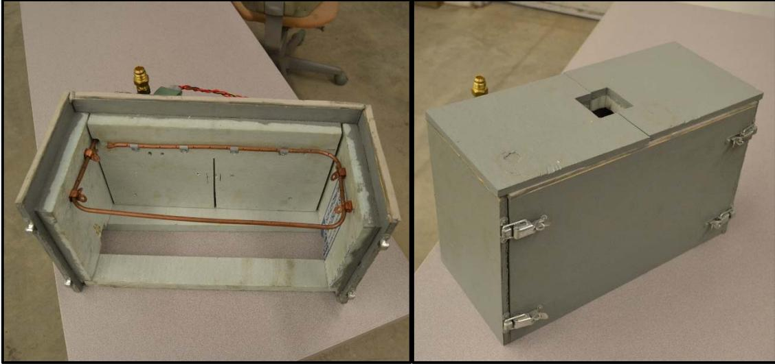
**Figure 3.9: Fracture mechanics testing temperature chamber**
