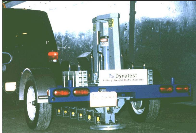
**Figure 25. FWD measurements on the subgrade lift.**
