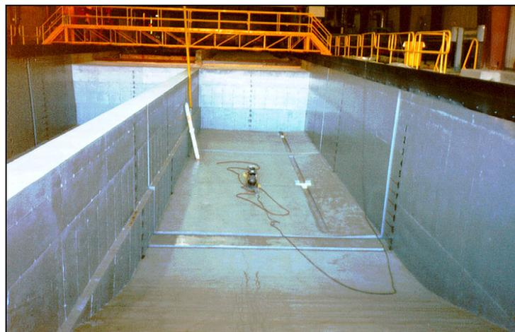
**Figure 11. Longitudinal wall separating the test basins.**
