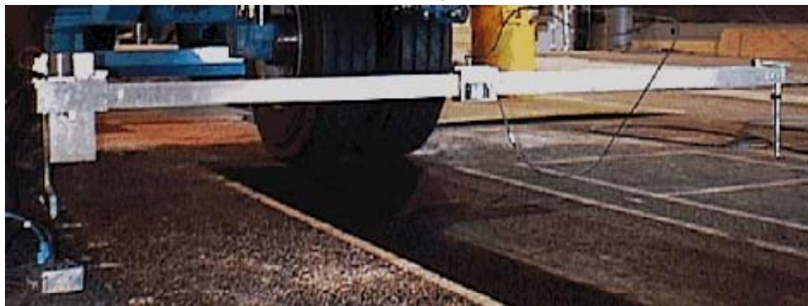
Figure 10. The laser Profilometer
