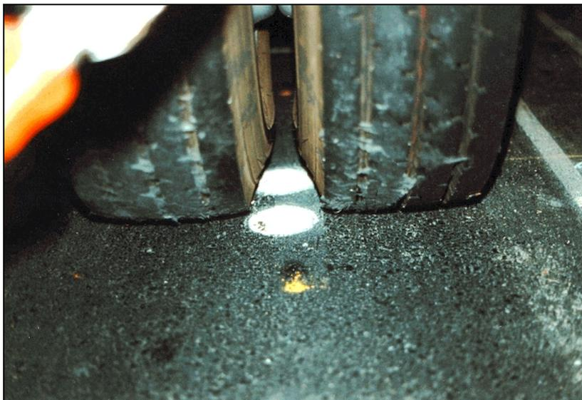
**Figure 6. Location of test wheels over coil and stress cells.**
