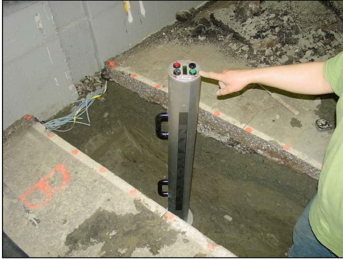
Figure 24. Portable falling weight deflectometer being used in the trenches.
