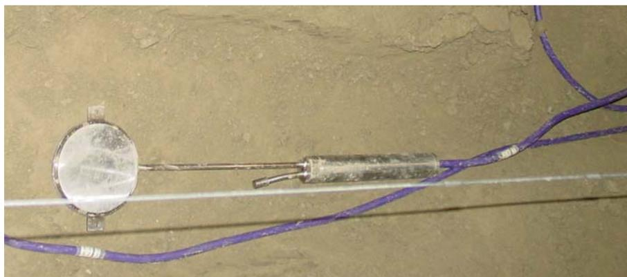
**Figure 10. Small Geokon® stress cell used in the subgrade.**
