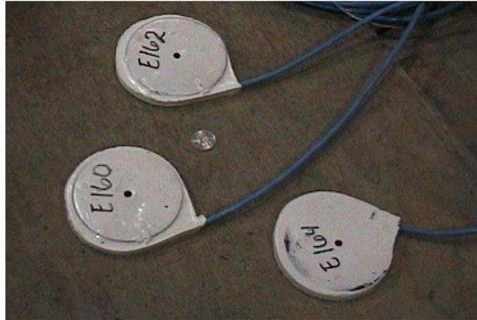
**Figure 9. Emu coils in a co-planar arrangement to measure longitudinal and transverse displacements. A US 25-cent coin is included for scale reference.**
