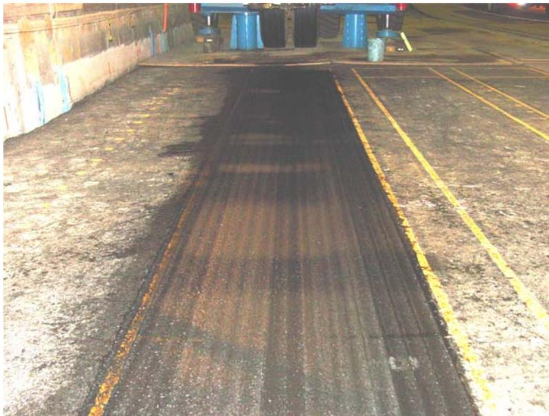
*Figure 20b. Test Window 712c1 at the end of HVS traffic.*
