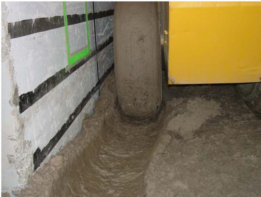
*Figure 19. Unstable soil behavior with gravimetric moisture contents between 27 and 35 percent..*
