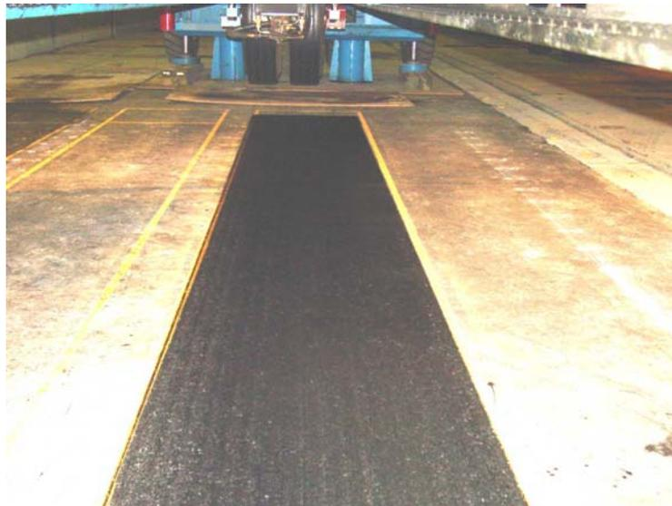
Figure 24b. Test Window 712c5 at the end of HVS traffic
