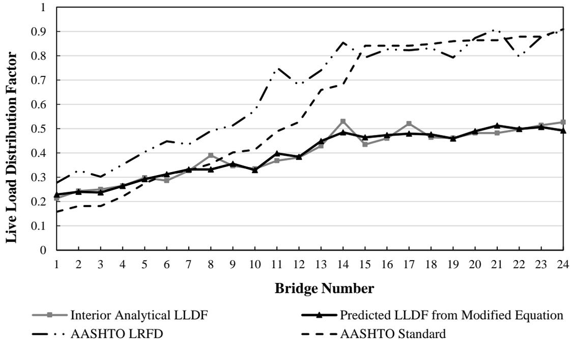
**Figure 25. Interior analytical LLDFs with 121 farm vehicles – multiple traffic lane steel-concrete bridges**
