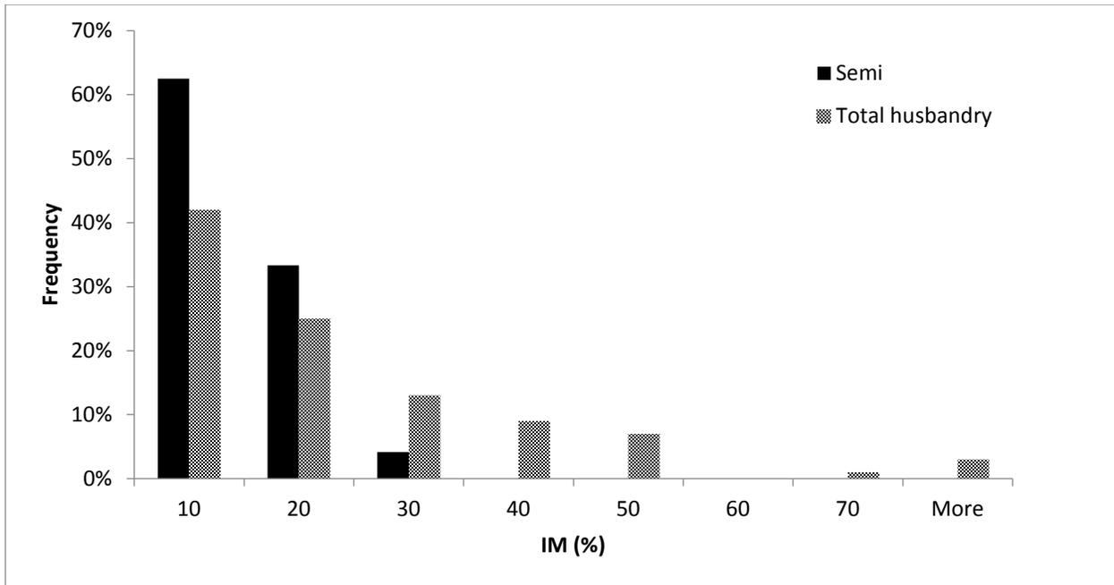
**Figure 20. IM frequency for all girders and all vehicles for timber-timber bridges**
