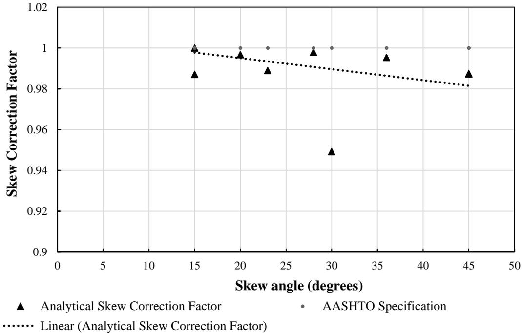
**Figure 38. Skew correction factors – steel-timber bridges**
