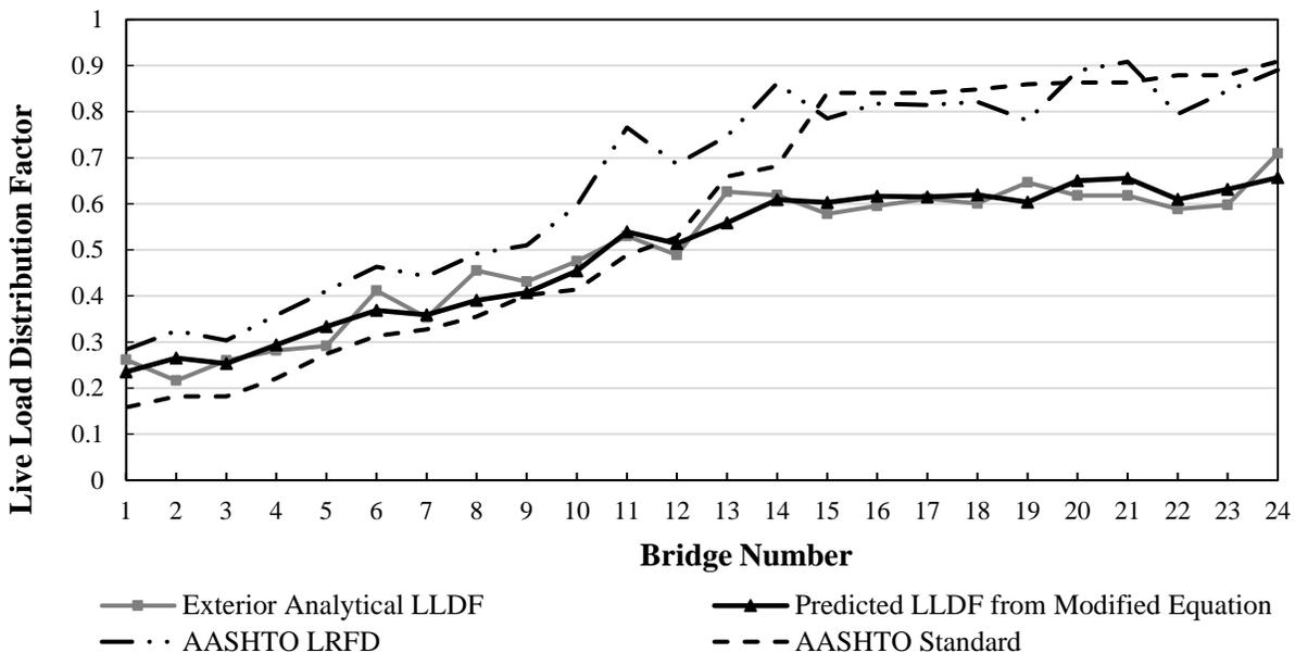
**Figure 24. Exterior analytical LLDFs with 121 farm vehicles – multiple traffic lane steel-concrete bridges**
