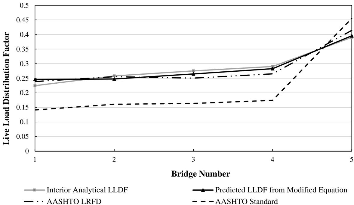
**Figure 23. Interior analytical LLDFs with 121 farm vehicles - one traffic lane steel-concrete bridges**
