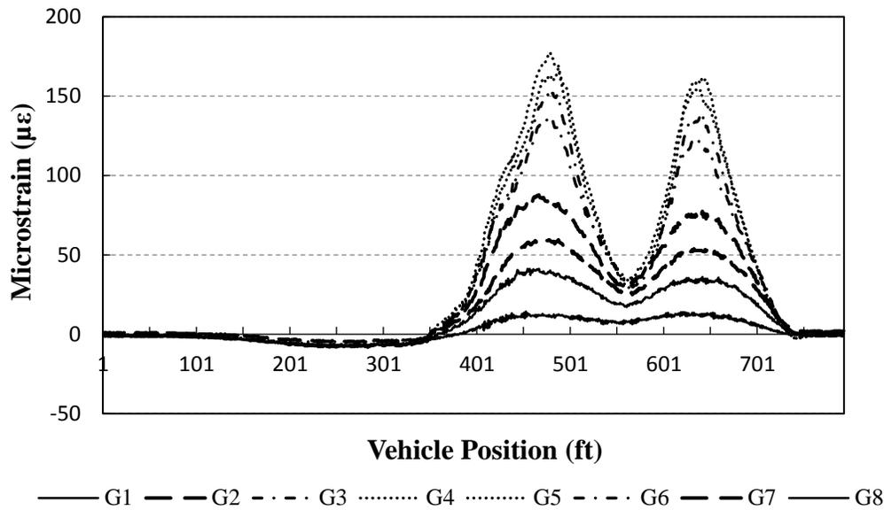
(b) Strain plot for all girders of a representative bridge under semi-truck loading
