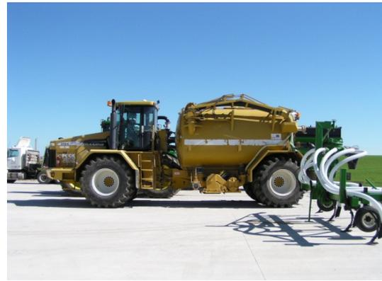
(c2) TerraGator with dual-wheel front axle
