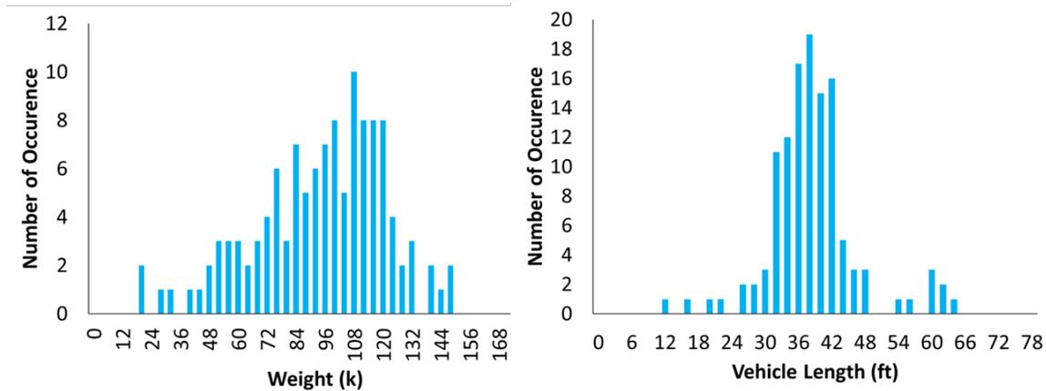
**Figure 10. Histograms of vehicle inventory with reference to weight and length**
