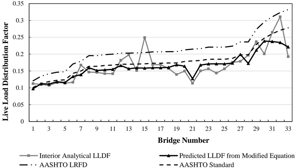
**Figure 40. Interior analytical LLDFs with 121 farm vehicles – one-way traffic lane timber-timber bridges**
