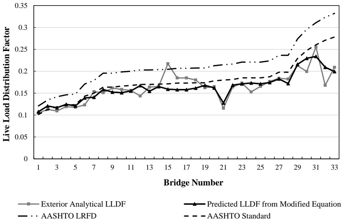
**Figure 39. Exterior analytical LLDFs with 121 farm vehicles – one-way traffic lane timber-timber bridges**
