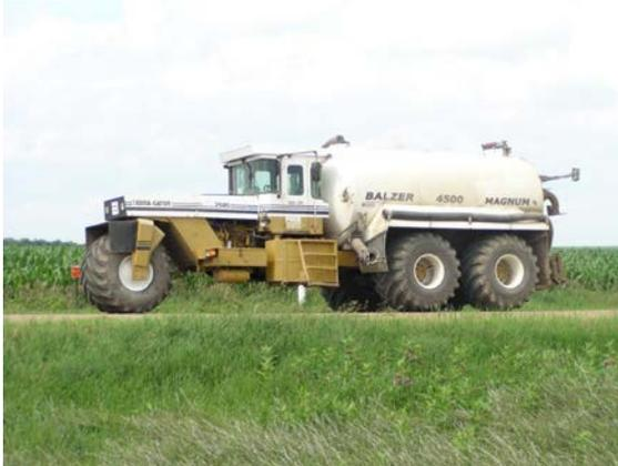
(c1) TerraGator with single-wheel front axle
