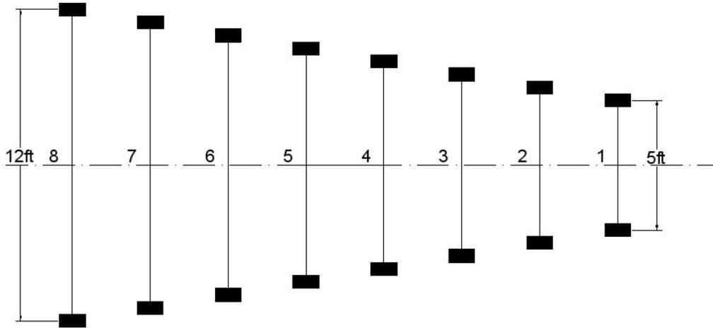
**Figure 14. Footprints of eight axles with varying gauge widths of 5 ft to 12 ft**
