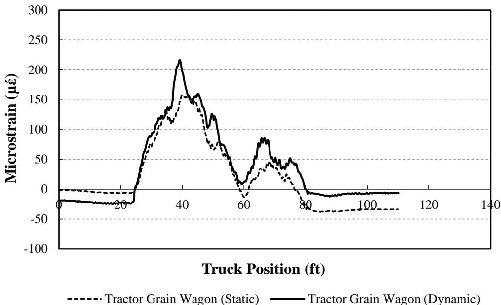
**Figure 8. Comparison plot between dynamic and static strain for a representative girder**
