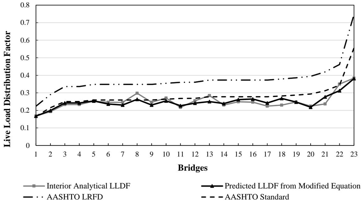
**Figure 32. Interior analytical LLDFs with 121 farm vehicles – one-way traffic lane steel-timber bridges**
