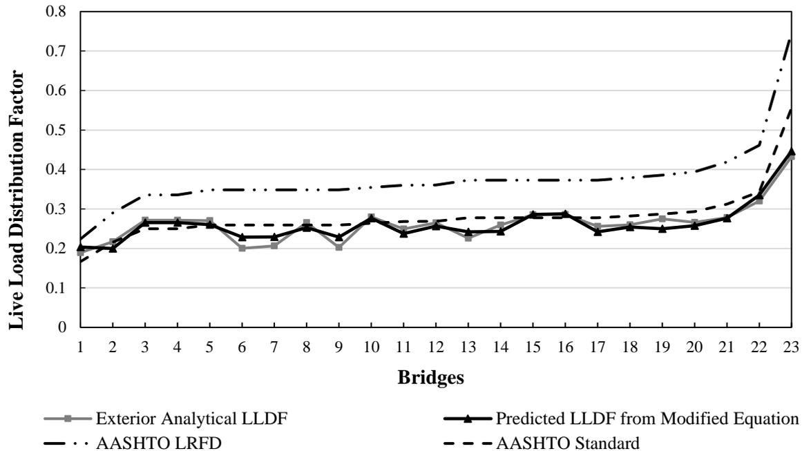
**Figure 31. Exterior analytical LLDFs with 121 farm vehicles – one-way traffic lane steel-timber bridges**
