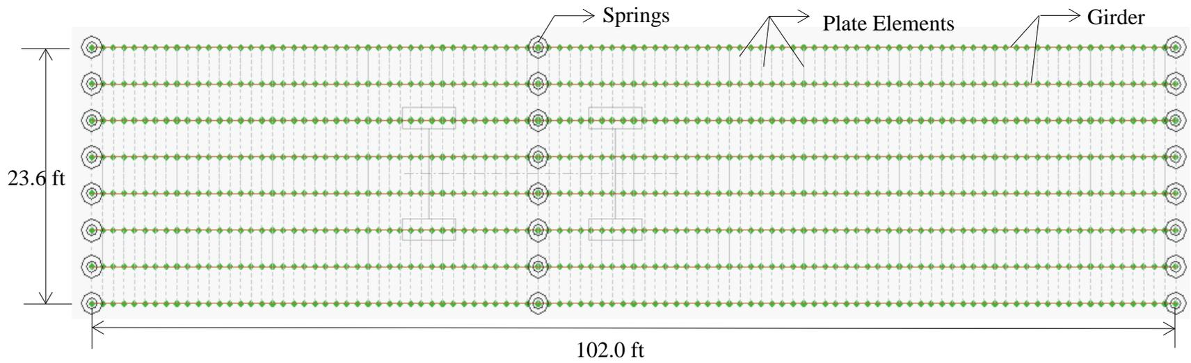
**Figure 9. Finite element bridge model**
