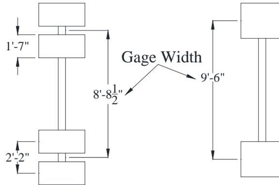
**Figure 12. Axle gauge width measurement for two types of axles**
