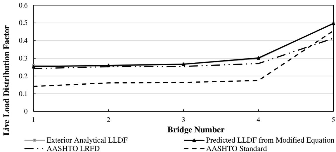
**Figure 22. Exterior analytical LLDFs with 121 farm vehicles - one-way traffic lane steel-concrete bridges**
