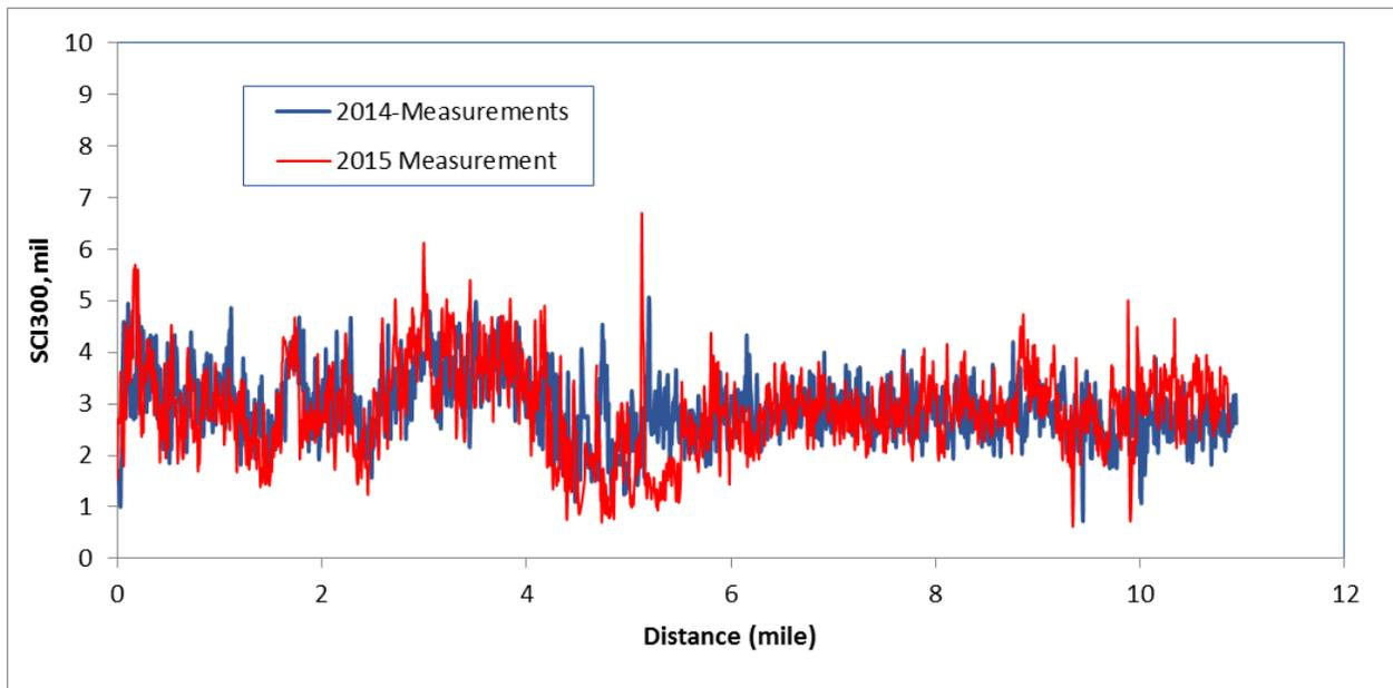
**Figure 10. Temperature corrected repeated TSD tests (SCI300) on Champaign CH1**
