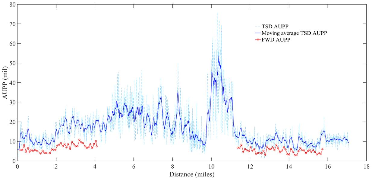
**Figure 16 Comparison of TSD AUPP and FWD AUPP on SR29 East**
