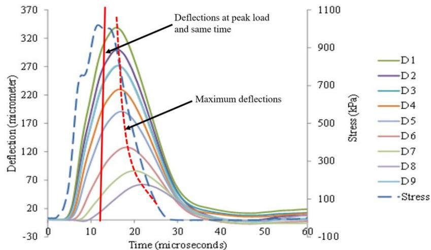
**Figure 17 Example of FWD time history from LTPP section 169034 taken from Chatti et al. (2017)**
