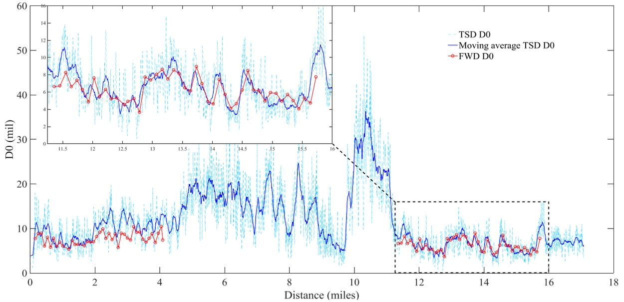
**Figure 15 Comparison of TSD D0 and FWD D0 on R29 East (<https://goo.gl/maps/UmevQei4yYk>)**
