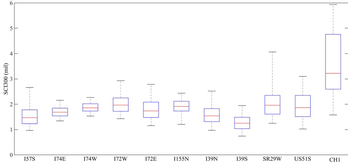
**Figure 9. SCI300 box of tested roads in 2015.**
