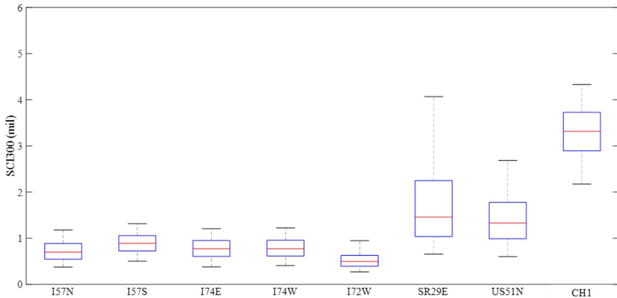
**Figure 8. SCI300 box plot of tested roads in 2014.**
