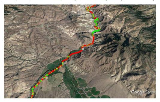
Figure 5. Detail example of estimated structural condition: US93 south near Ellis (© 2016 Google).
