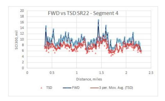
Figure 11. Comparison of TSD SCI300 and FWD SCI300 on SR 22 Segment 4
