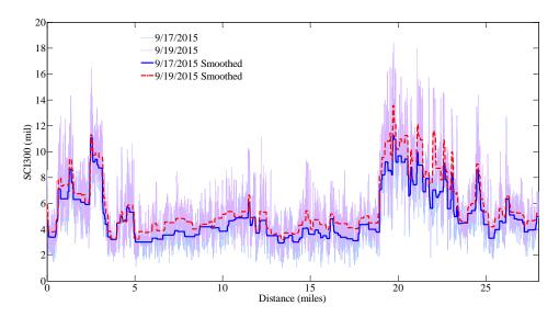
Figure 8. Temperature corrected repeated TSD tests (SCI300) on a stretch of SR28N (https://goo.gl/maps/wJ7yQpWEXo82).
