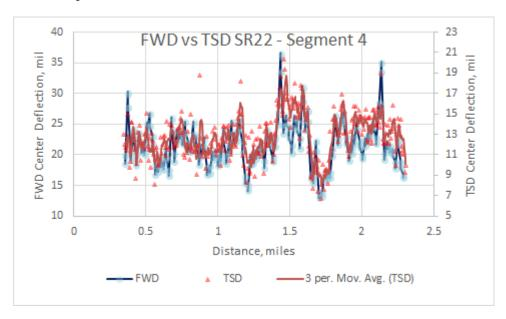
Figure 10. Comparison of TSD D0 and FWD D0 on SR 22 Segment 4
