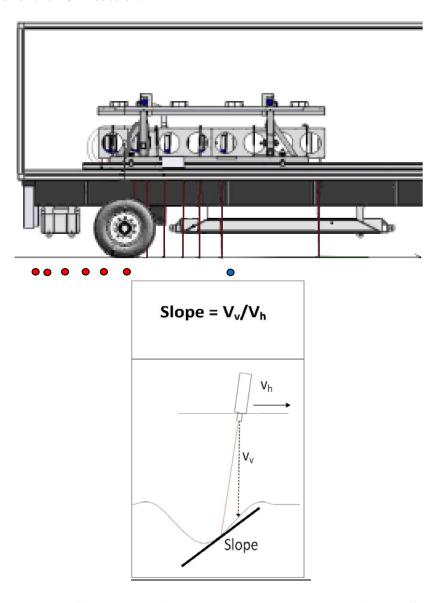
Figure 2. Schematic of the measurement principle of the TSD.
