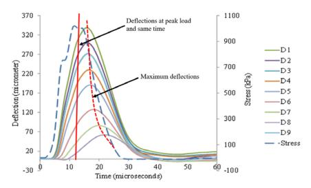
Figure 12 Example of FWD time history from LTPP section 169034 taken from Chatti et al. (2017)
