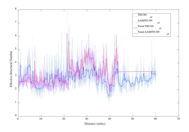
Figure 15 Example of calculated effective structural number on US93 south (see Figure 16 or following link <a href="https://goo.gl/maps/vXkXU5nFM4r">https://goo.gl/maps/vXkXU5nFM4r</a>)
