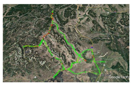
Figure 4. Color-coded estimated structural condition of tested pavements in 2015 with Good (green), Fair (yellow), and Poor (red) ratings (© 2016 Google Image Landsat / Copernicus).
