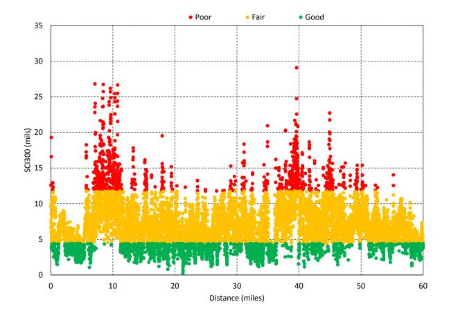
Figure 14 Classification of structural condition on US93 south based on percentile: 25<sup>th</sup> percentile and lower represents good structural condition and 90<sup>th</sup> percentile and higher represents poor structural condition
