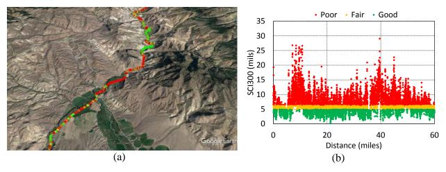
Figure 13. Identified Strong (green) and Weak (red) sections on US93 south based on thresholds obtained from Table 2: (a) Google Earth plot (© 2016 Google); (b) figure plot
