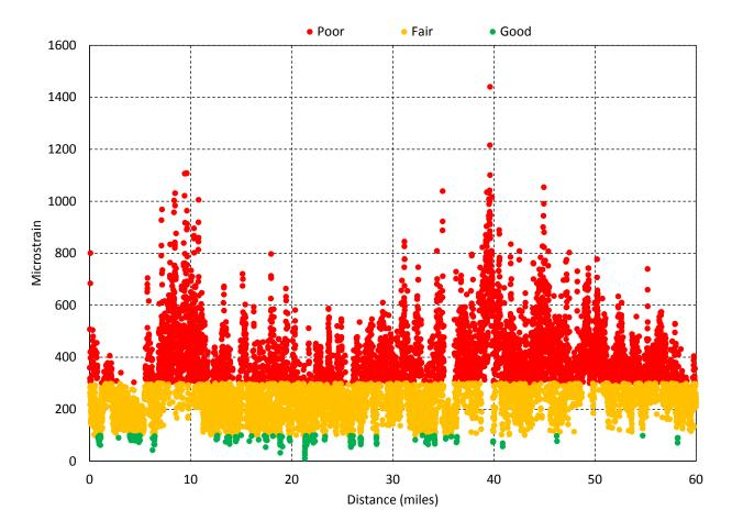
Figure 18. Estimated tensile strain at bottom of asphalt layer on US93 south.
