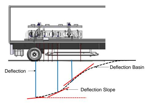
Figure 3. Relationship between the deflection basin, deflection, and deflection slope.
