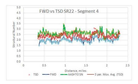
Figure 17. Comparison of Structural number computed from TSD and FWD on SR 22 Segment 4
