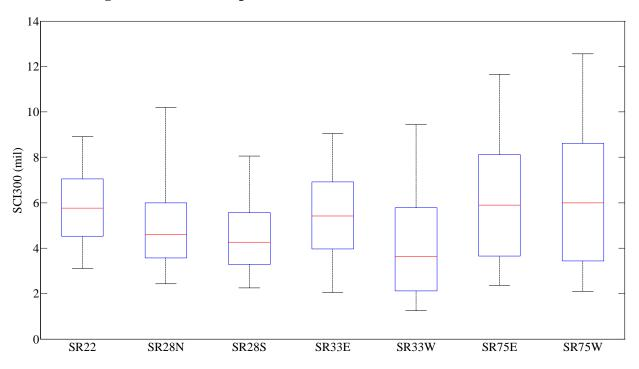
Figure 7. SCI300 box plot of state routes tested in 2015.
