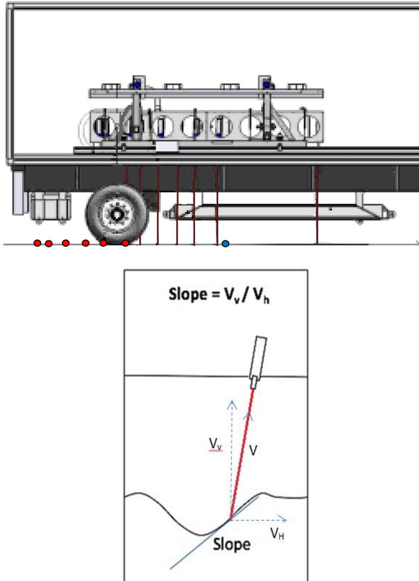
**Figure 2. Schematic of the measurement principle of the TSD (Krarup 2012 and modified from Flintsch et al. 2013).**
