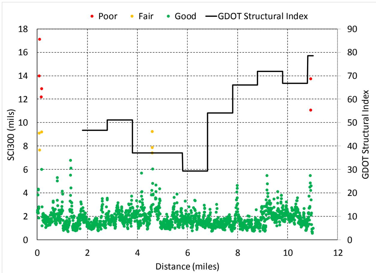
Figure 12 Comparison on SR74 in Fayette County between TSD SCI300 measured in 2015 and Structural Index obtained from surface distresses (<https://goo.gl/maps/azJkphpKdBo>)
