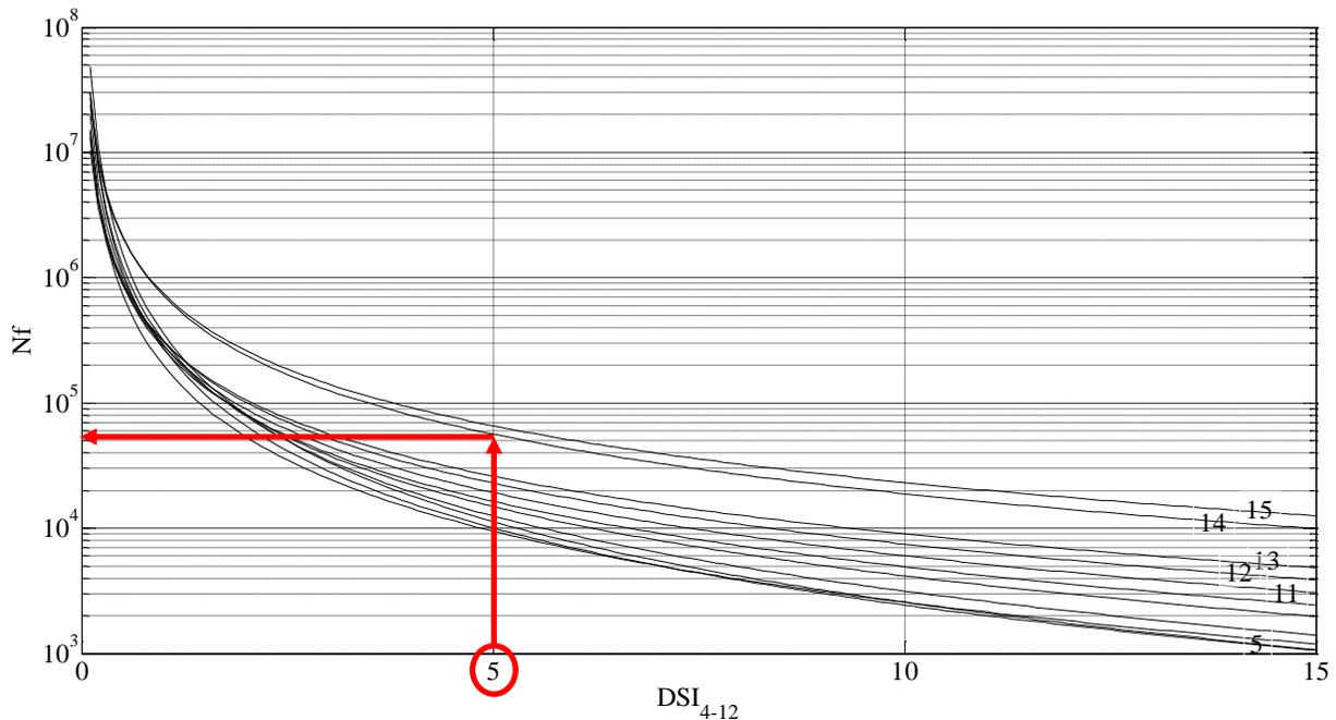
**Figure 20. Fatigue life curves for TSD DSI.**
