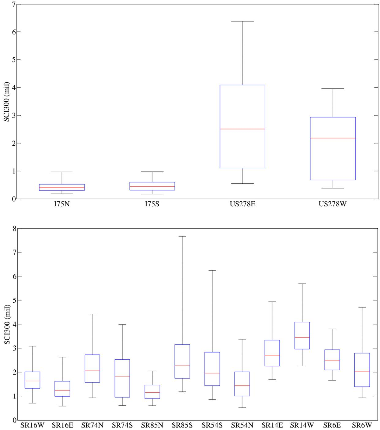
**Figure 8. SCI300 box plot of tested roads in 2014.**
