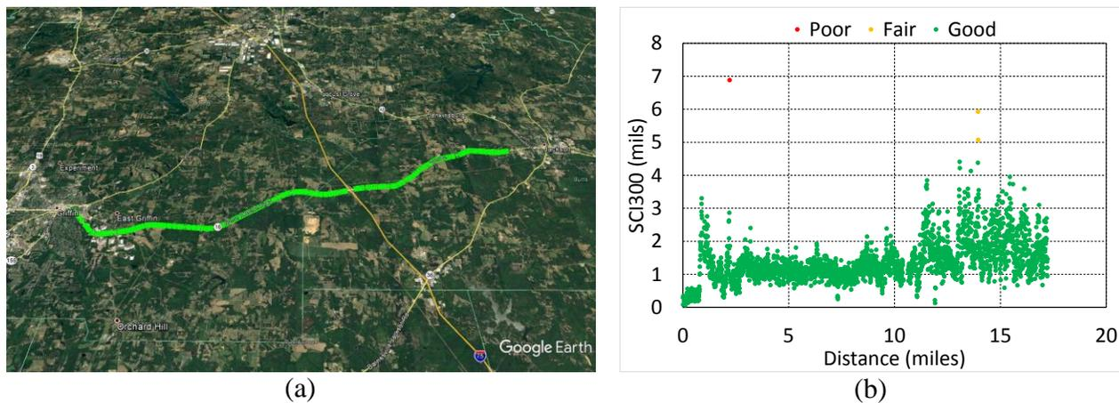
**Figure 13. Identified Strong (green) and Weak (red) sections on SR16 east based on thresholds obtained from Table 2: (a) Google Earth plot (© 2016 Google Image Landsat / Copernicus); (b) figure plot**
