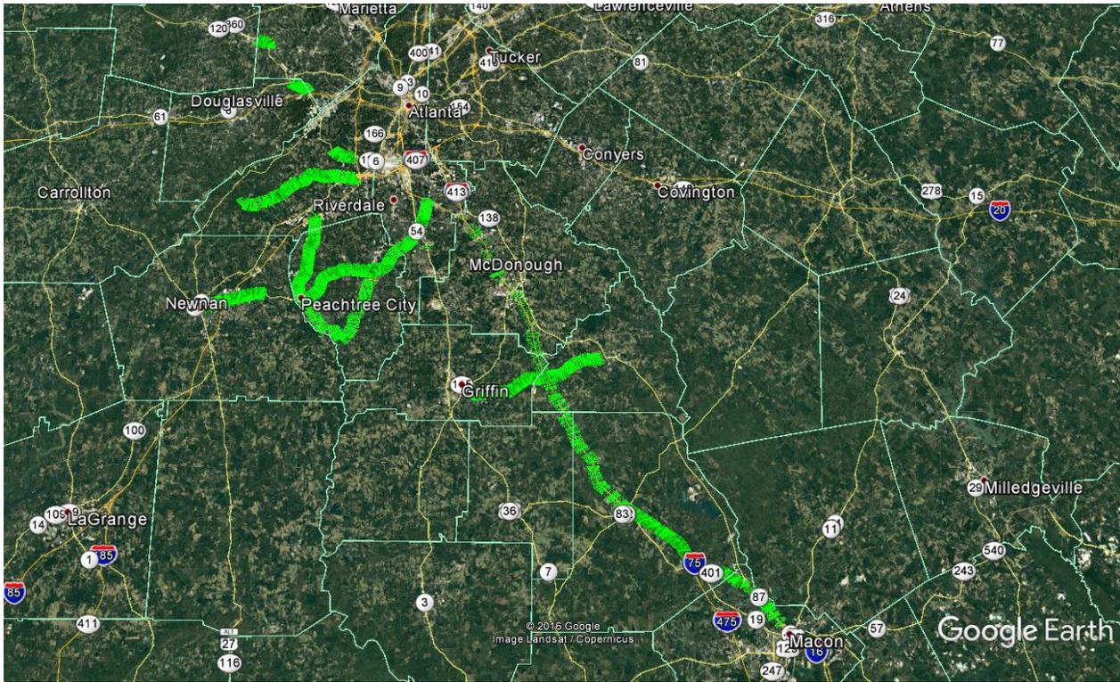
**Figure 6. Color-coded estimated structural condition of tested roads in 2015 with Good (green), Fair (yellow), and Poor (red) ratings (© 2016 Google Image Landsat / Copernicus).**
