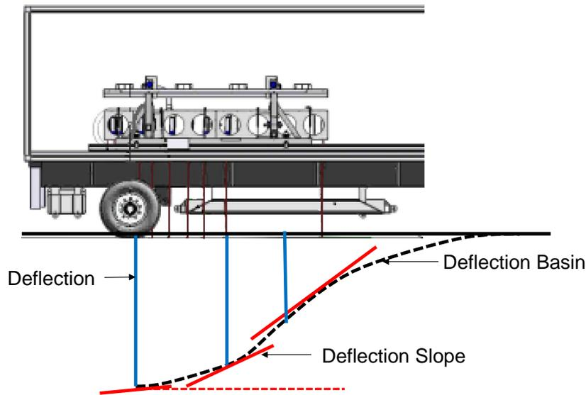
**Figure 3. Relationship between the deflection basin, deflection, and deflection slope (modified from Krarup 2012).**
