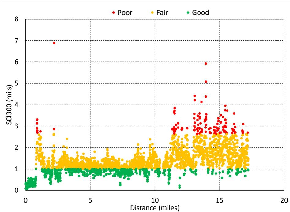
**Figure 14 Classification of structural condition on SR16 East based on percentile: 25<sup>th</sup> percentile and lower represents good structural condition and 90<sup>th</sup> percentile and higher represents poor structural condition**
