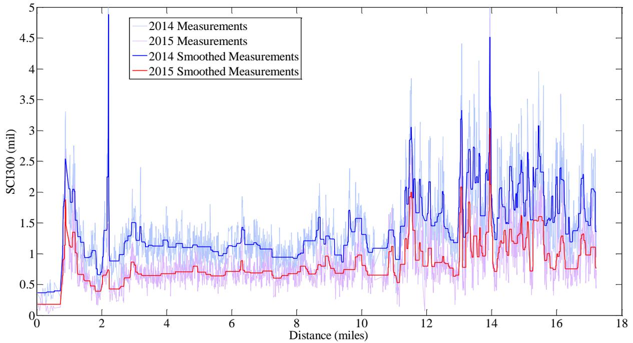
**Figure 10. Temperature corrected repeated TSD tests (SCI300) on SR16E**
