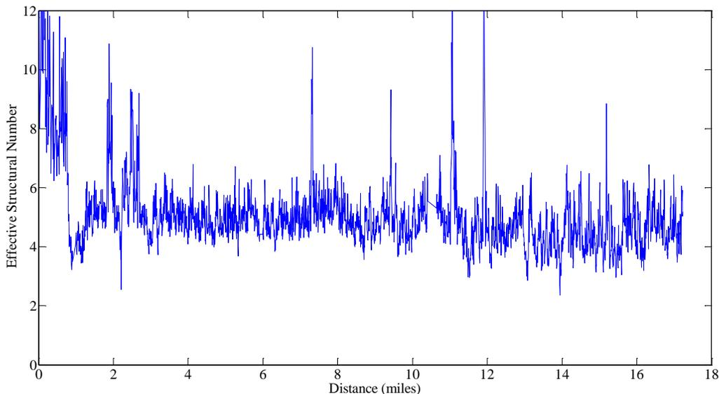
**Figure 16 Effective Structural Number on SR16E calculated from measurements collected in 2015**
