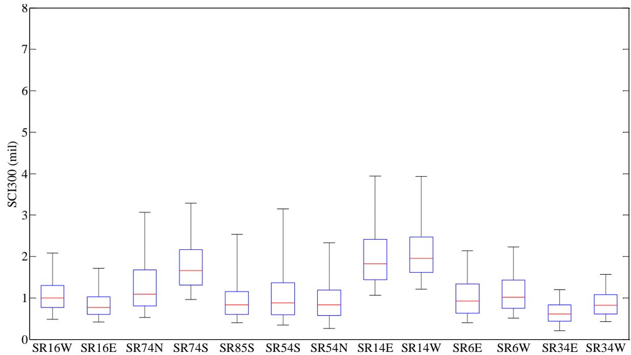
**Figure 9. SCI300 box of tested roads in 2015.**
