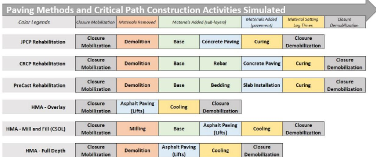
For example, a paving job featuring CRCP Rehabilitation includes a total of 7 critical path activities within a working window (illustrated below). Note that in this hypothetical CRCP paving job, certain critical path activities feature slack times or lag times (2, 3, 4, 5).
