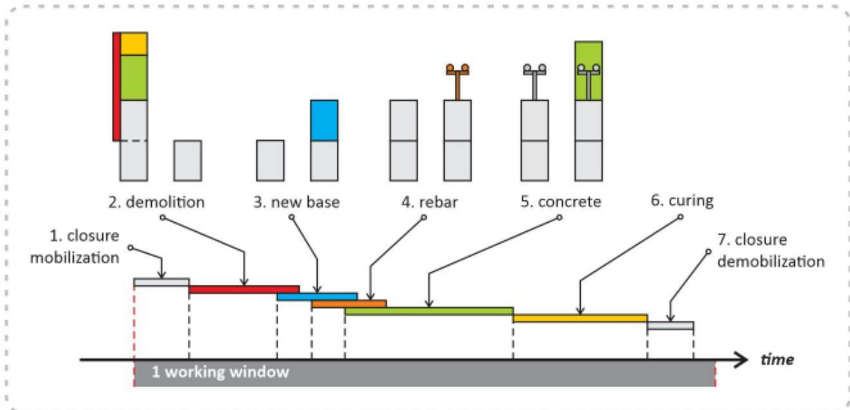
Although the sequence of construction activities depends on the paving method, Road Scheduler assumes closures include a closure mobilization and demobilization activity (activities 1 and 7). Otherwise, other critical path tasks within the closure can be a construction activity (activities 2-5) or a lag activity (activity 6).
