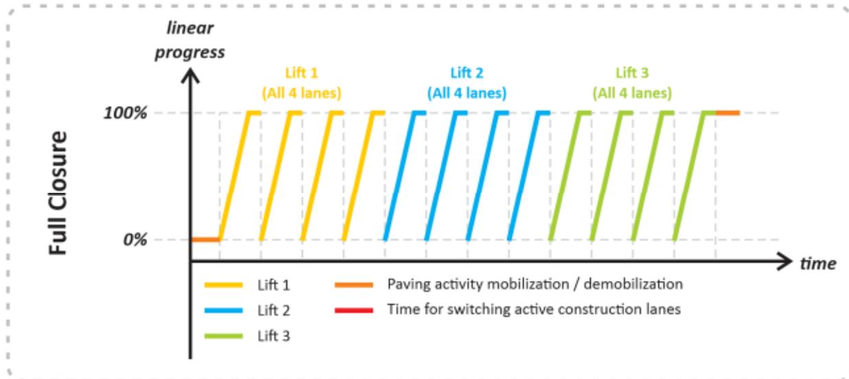
Each lift must have at least 1 additional adjacent lane available for a material supply truck. To represent this, Road Scheduler typically 'skips' lanes when it sequences lifts; for example, the lane sequence for the first lift may be 1, 3, 2, 4 so that the supply lanes are 2, 4, 1, 3 respectively. This pattern maximizes the amount of cooling time for a given lane and lift until a paver needs to begin the next lift layer.
