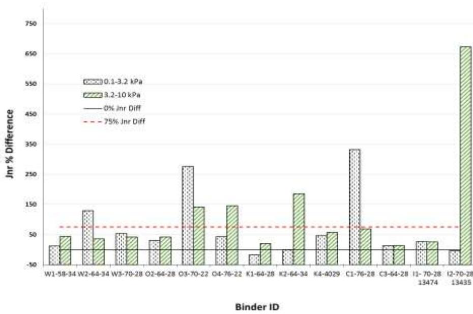
**Figure 10. Values of % Jnr Diff values for each Pooled Fund binder. Where 0.1-3.2 kPa data represents the % Jnr Diff between stress levels of 0.1 and 3.2 and 3.2-10 kPa data represents the % Jnr Diff between stress levels of 3.2 and 10 kPa.**
