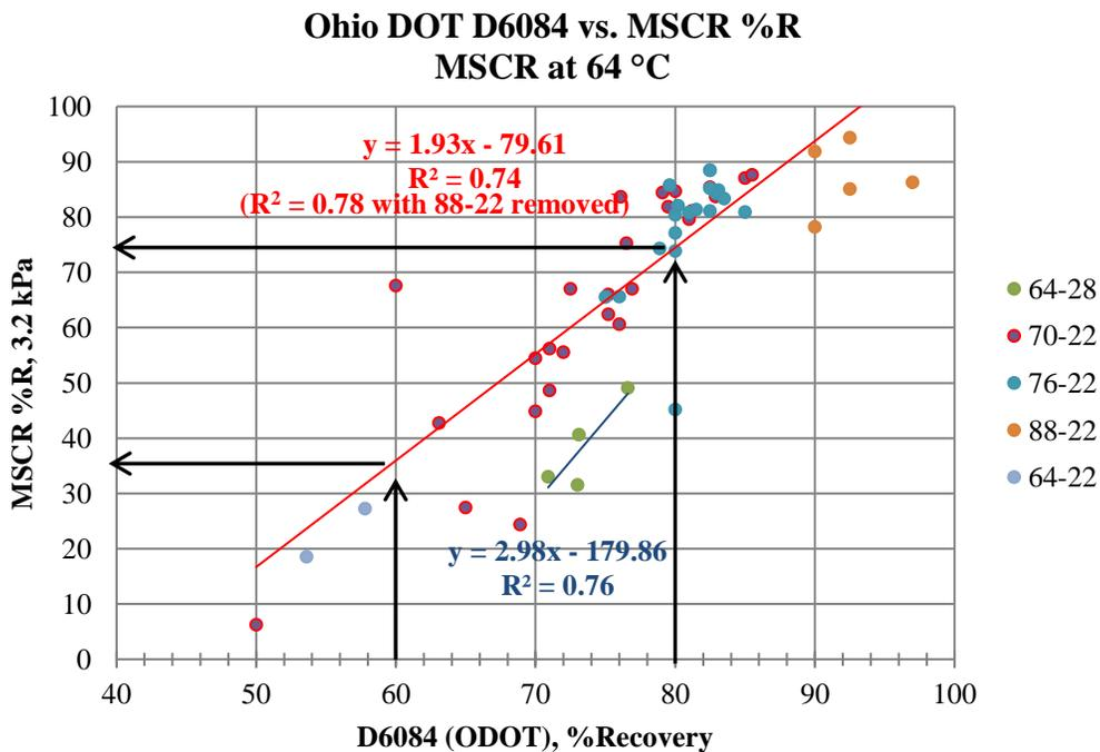
**Figure 3. Correlation of elastic recovery to %R for KDOT and ODOT**
