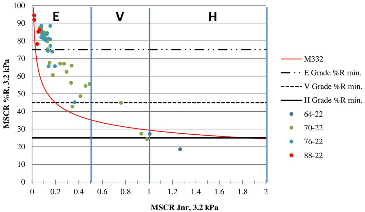
Figure 7. KDOT and ODOT MSCR data on M332 chart
