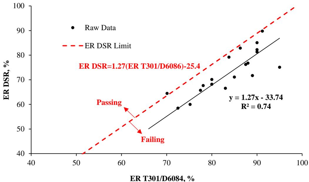
**Figure 6. Correlation between ER T301/D6084 and ER DSR (TP123 method B) with recommended limitation for potential ER DSR specification.**
