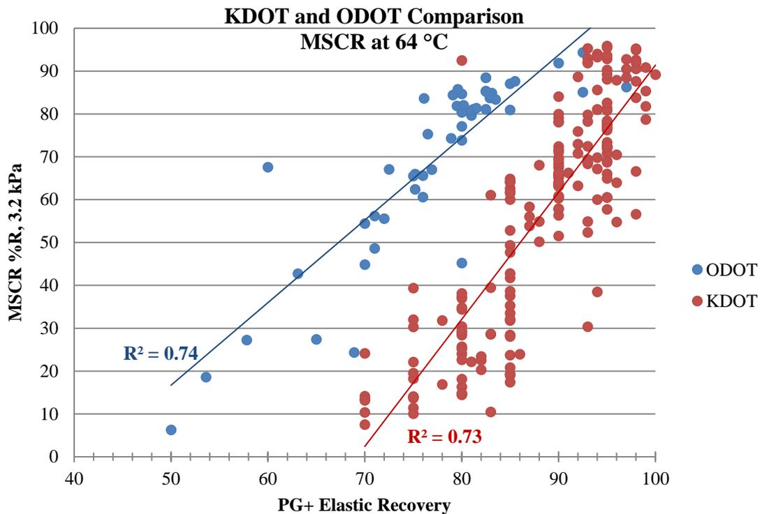
Figure 4. Comparison of KDOT and ODOT data showing effect of PG+ elasticity method.
