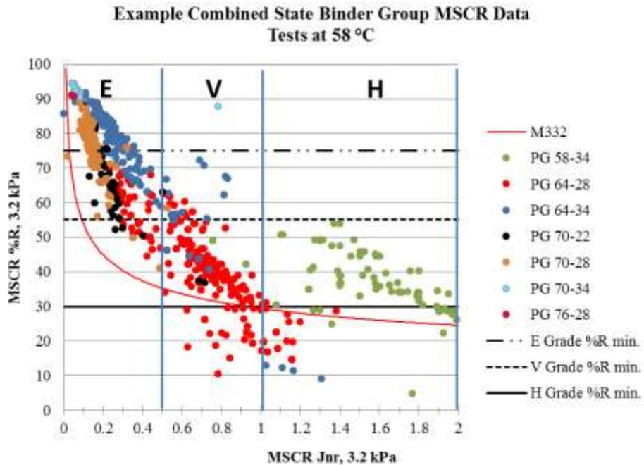
**Figure 8. Combined State Binder Group example data (adapted from [4]).**
