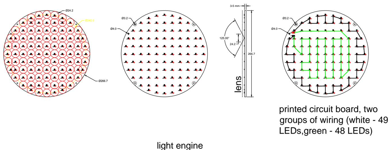
a total of 97 LEDs directly mounted on a 3-5 mm thick MPCB board serving as the passive heat exchanger. The 97 LEDs in a total of approximately 20-26 W are wired in two groups in parallel, connected to 110 V.
