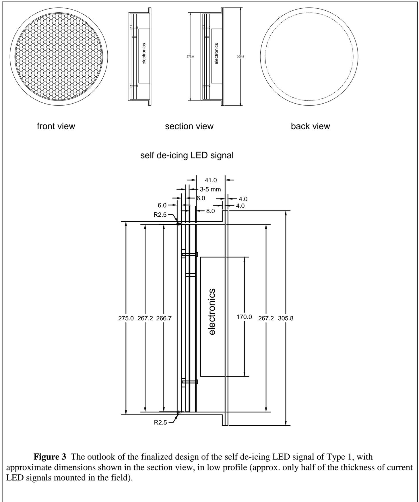
**Figure 3** The outlook of the finalized design of the self de-icing LED signal of Type 1, with approximate dimensions shown in the section view, in low profile (approx. only half of the thickness of current LED signals mounted in the field).
