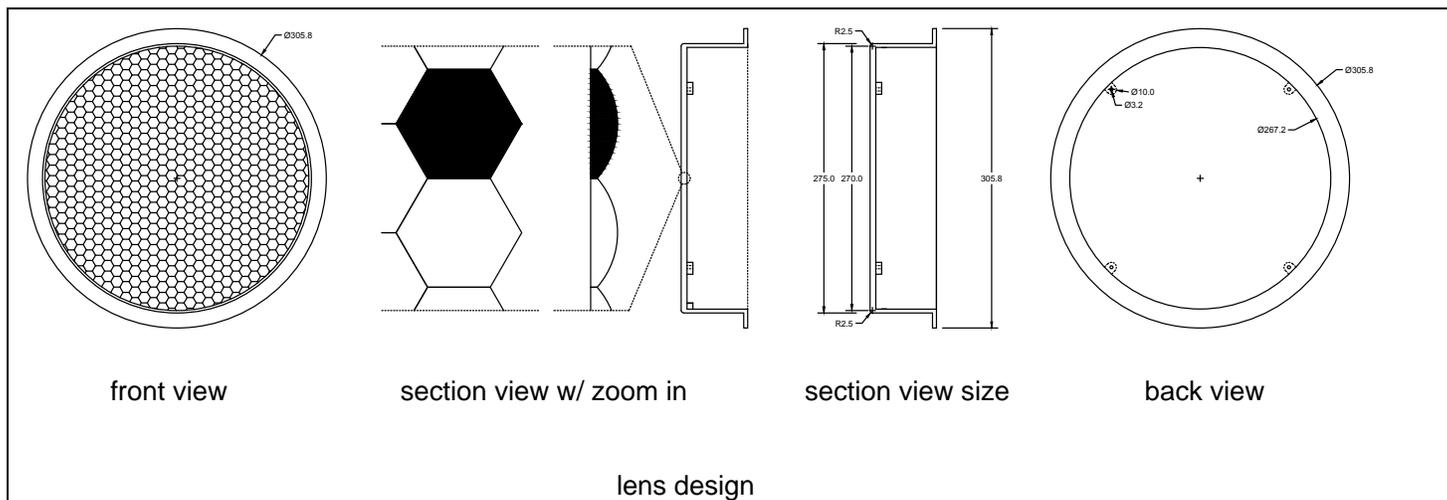
**Figure 4** The detail of the new lens design of the self de-icing LED signal of Type 1. In this design, the lens adopts a whole piece design with smooth and flat outside surface and hundreds of small plano-convex lenses on the inside surface to focus the light serving as a collimator lens. This design allows a small gap between the LEDs and the lens as small as ¼ inch for enhanced thermal performance.
