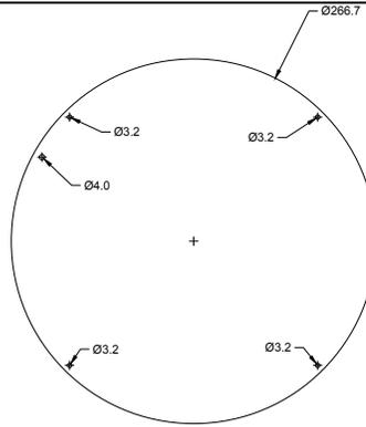
passive heat exchanger (the aluminum back plate of the MPCB board)
