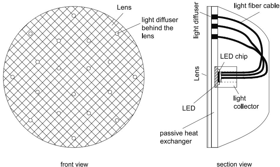
**Figure 2** Type 2 signal deploying the architecture of “Heated Lens Lighting Arrangement” (non-provisional patent application No. PCT/US14/53503) using a single high-power color LED module, a light collector and multiple light fibers.
