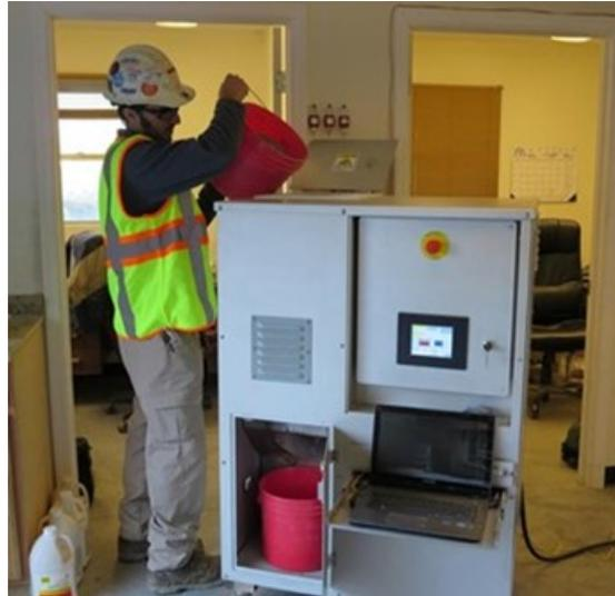
**Figure 2.2: Operator Introducing Aggregate into SLT for Scanning**
