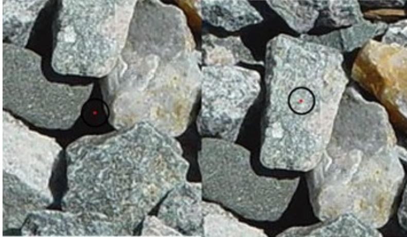
**Figure 4.1: Target Orifice (Outer Circle) and Laser Shot (Red Dot Inside Circle) – Magnified Photo of ~½ Inch Diameter Aggregate**
