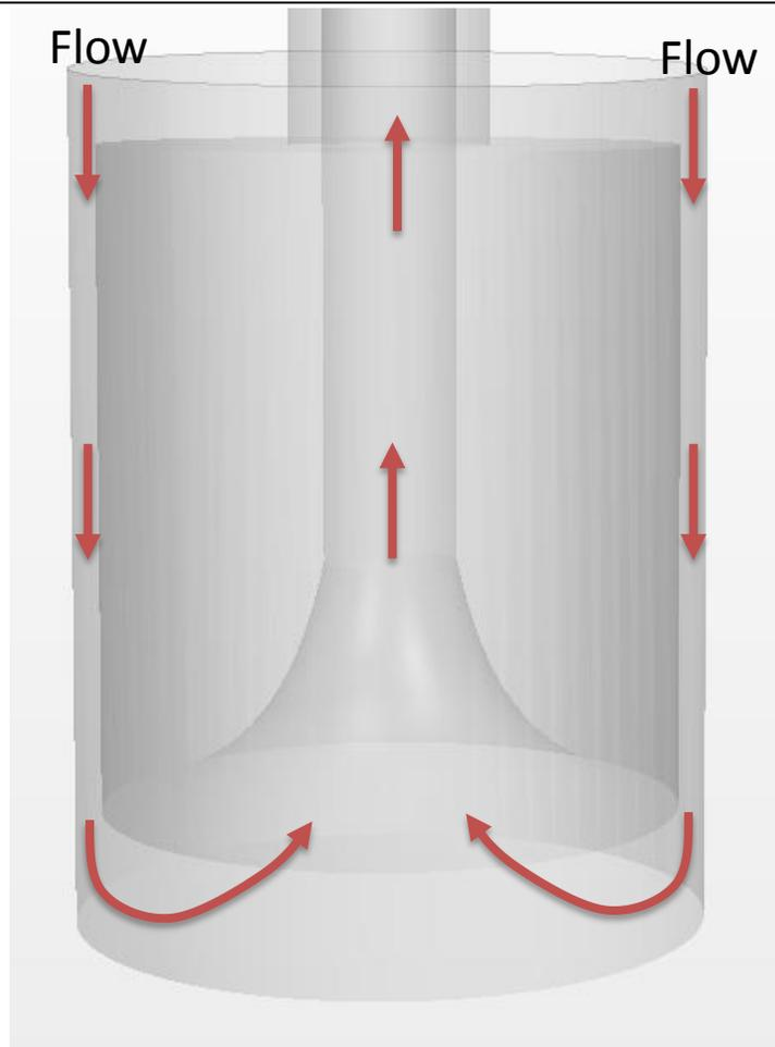
Geometry of the ISTD erosion head
