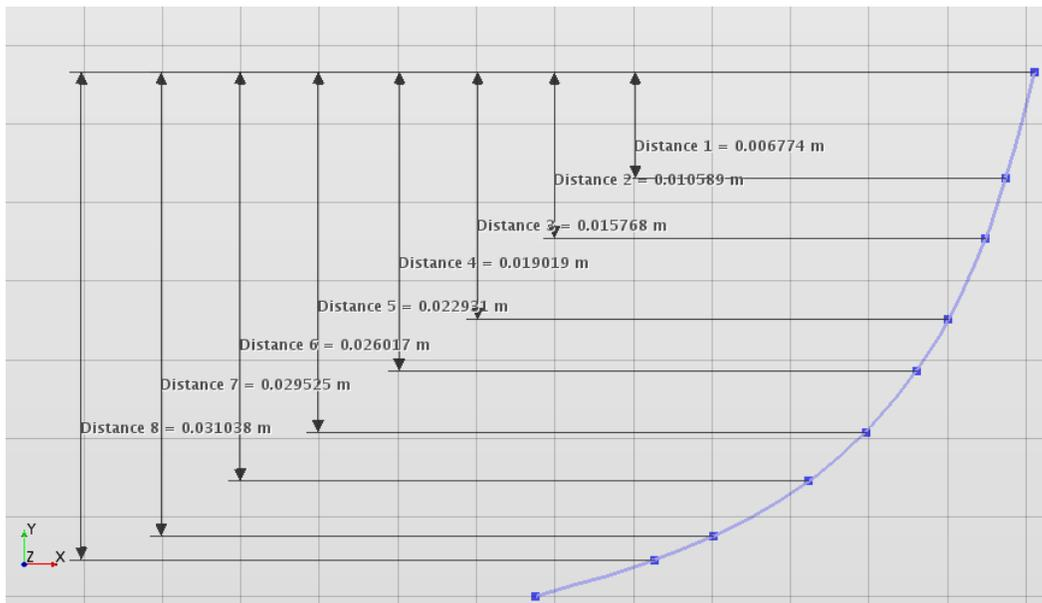
The spline function with eight parameters selected for the erosion head
