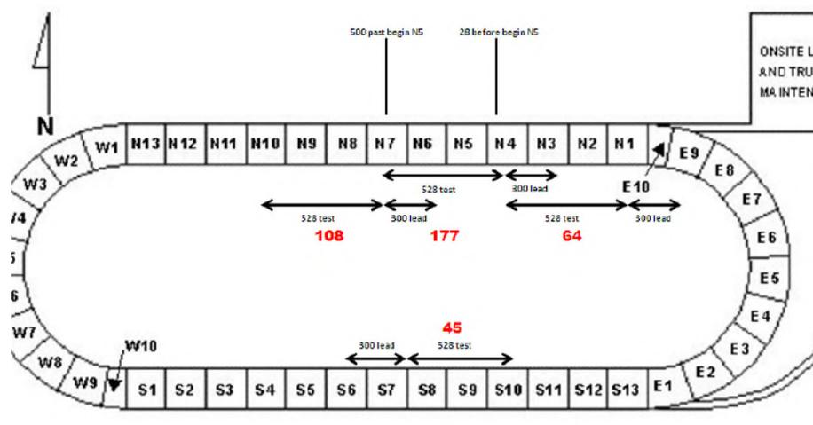
Figure 4.4. Location of profiler test sections on the NCAT test track (Powell, 2012).
