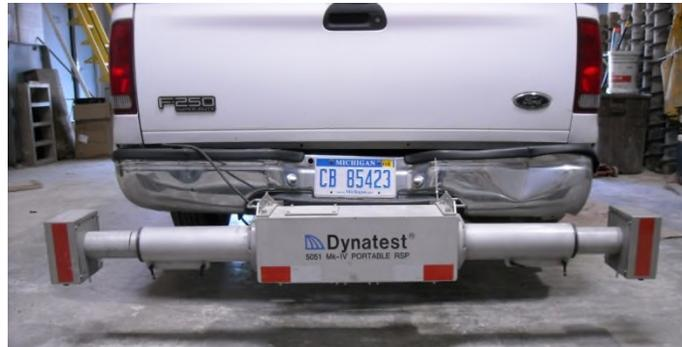
Figure 2.4. Portable profiler mounted on the back of a vehicle.
