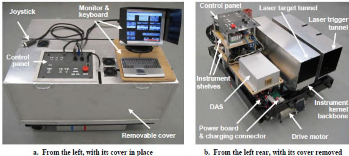
Figure 2.11. Benchmark profiler with and without cover in place (Winkler et al., 2013).
