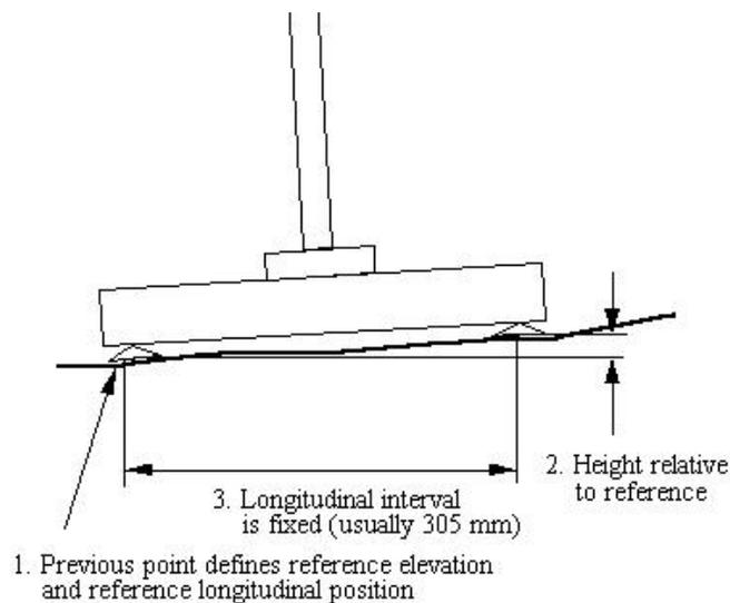
Figure 2.7. Elevation measurements by Dipstick. (Karamihas and Sayers, 1998).
