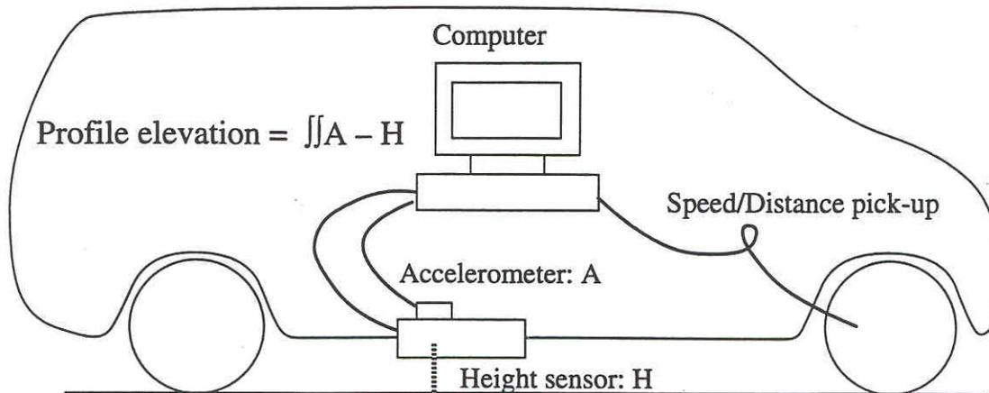
Figure 2.1. Components of an inertial profiler (Sayers and Karamihas, 1998).
