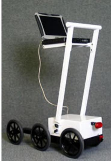
Figure 2.9. SSI CS 8800 Walking Profiler.
