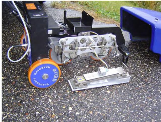
Figure 2.6. ARRB walking profiler.
