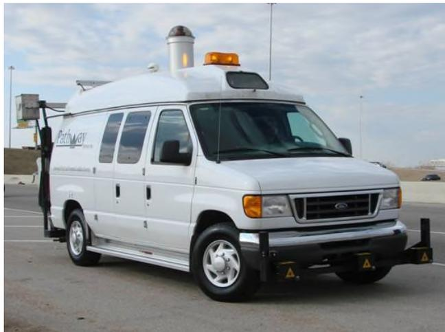
Figure 2.16. Pathway multi-function data collection equipment.
