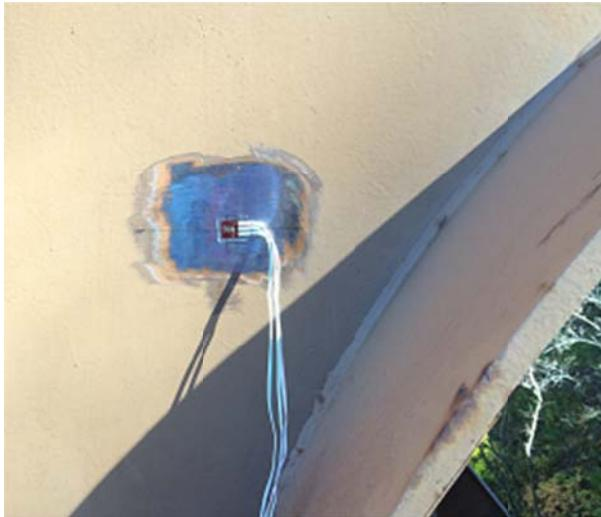
**Figure 3.2-5.** Triaxial strain gage at girder-knee joint.
