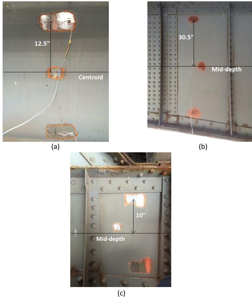
**Figure 4.2-2.** Location of gages for field test. (a) Uniaxial weldable strain gages at floor beam #5, centerline of the bridge. (b) Uniaxial strain gages at bascule's girder web, 65.375 in. from floor beam No.2 towards centerline of lift span. (c) Triaxial glued strain gages at tail beam, 21.5 in. from tail beam end (tail beam bearing on approach span is at top right).
