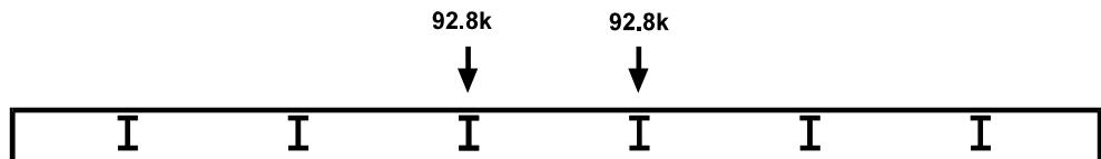
**Figure 9.4-5.** OSOW stringer reactions as loads on floor beam.
