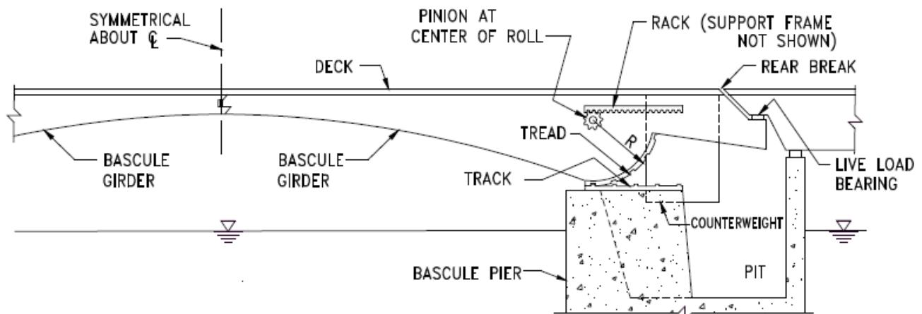
**Figure 4.1-1.** Double leaf Rolling Bascule Bridge configuration. Reprinted from WisDOT Structures Inspection Manual.
