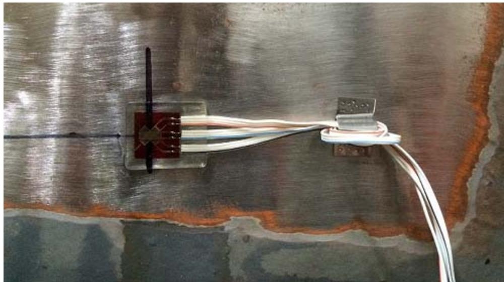
**Figure 4.2-6.** Triaxial strain gage at tail beam.
