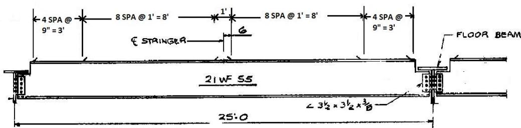
(b) Stringer-floor beam connection elevation view and shear connector spacing
