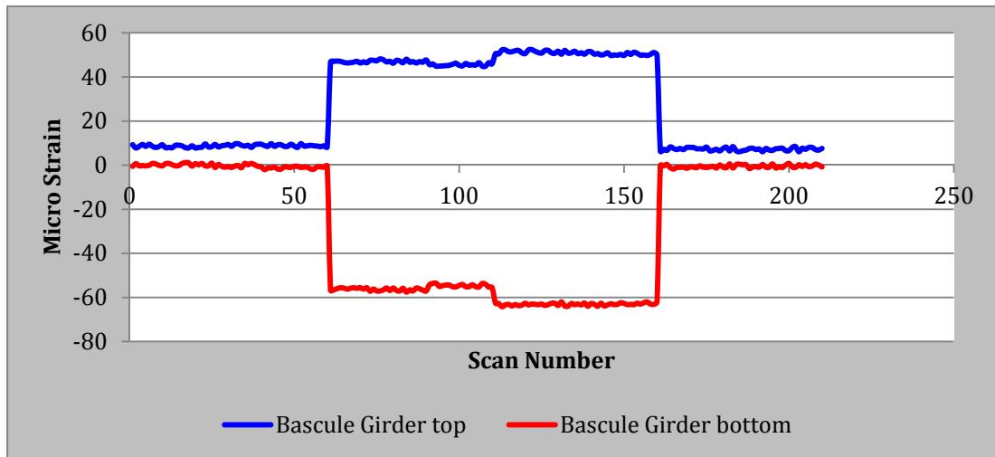
**Figure 4.2-8.** Strain gage from bascule girder.
