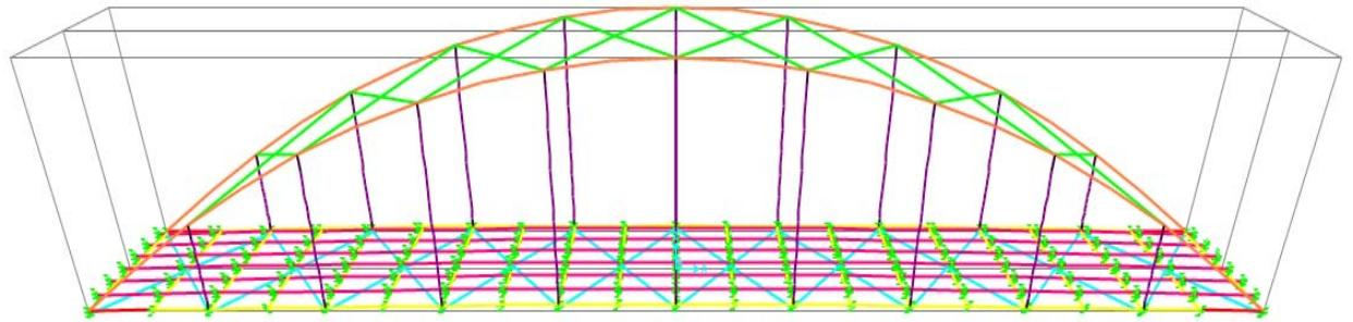
**Figure 6.3-1.** 3D FEM model of Cameron Ave Bridge
