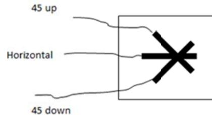
**Figure 3.2-7.** Rosette strain gage.
