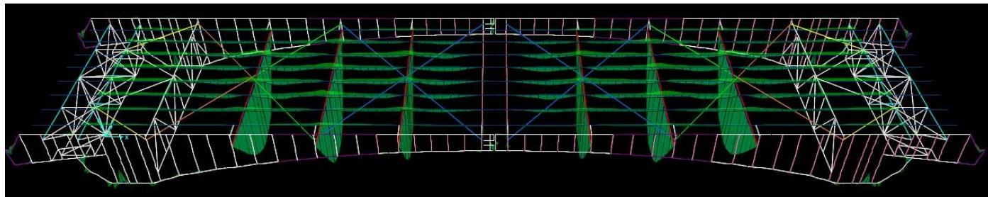
**Figure 4.4-1.** Moment envelope of critical members under OSOW/HL-93 truck combinations.
