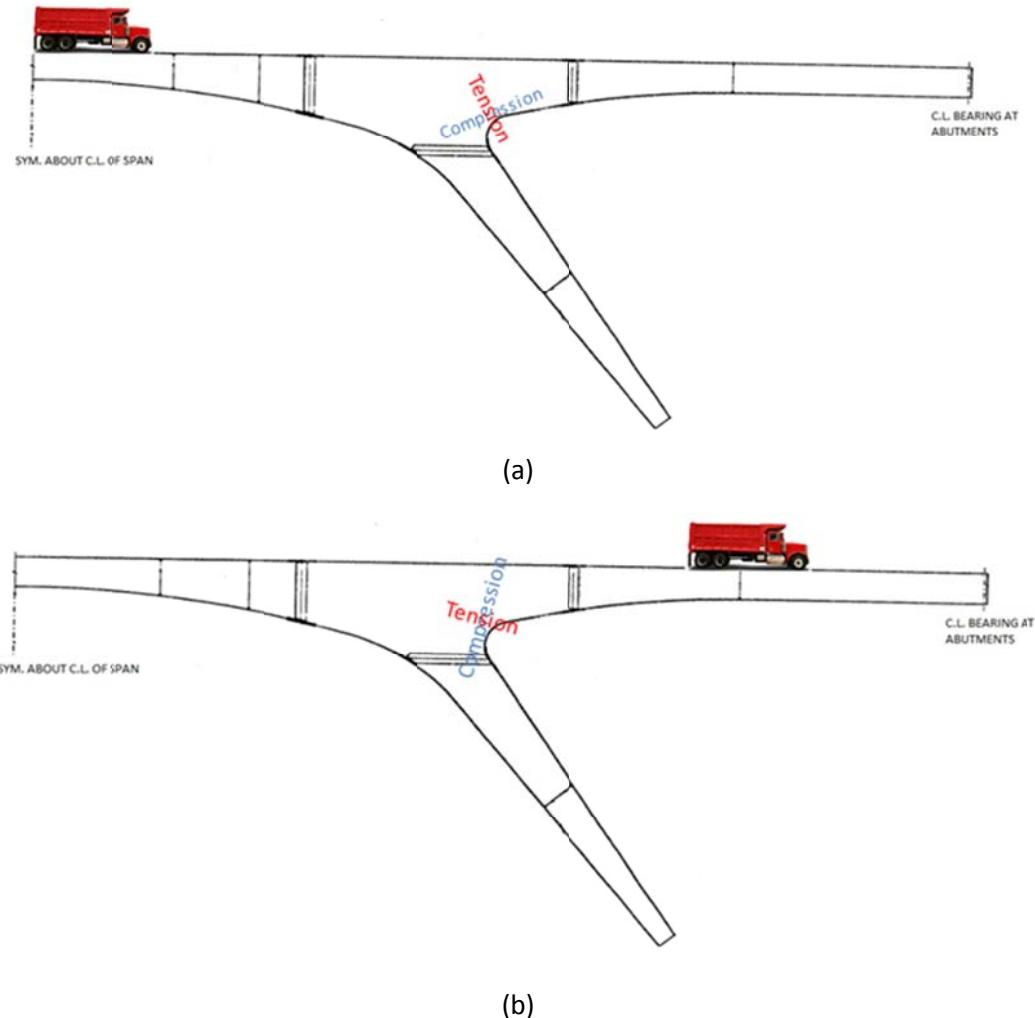
**Figure 3.2-8.** Direction of principal stresses at girder-knee point under loaded dump trucks. (a) Trucks at midspan (Position 1) and (b) trucks at 60 ft. from south abutment (Position 2).
