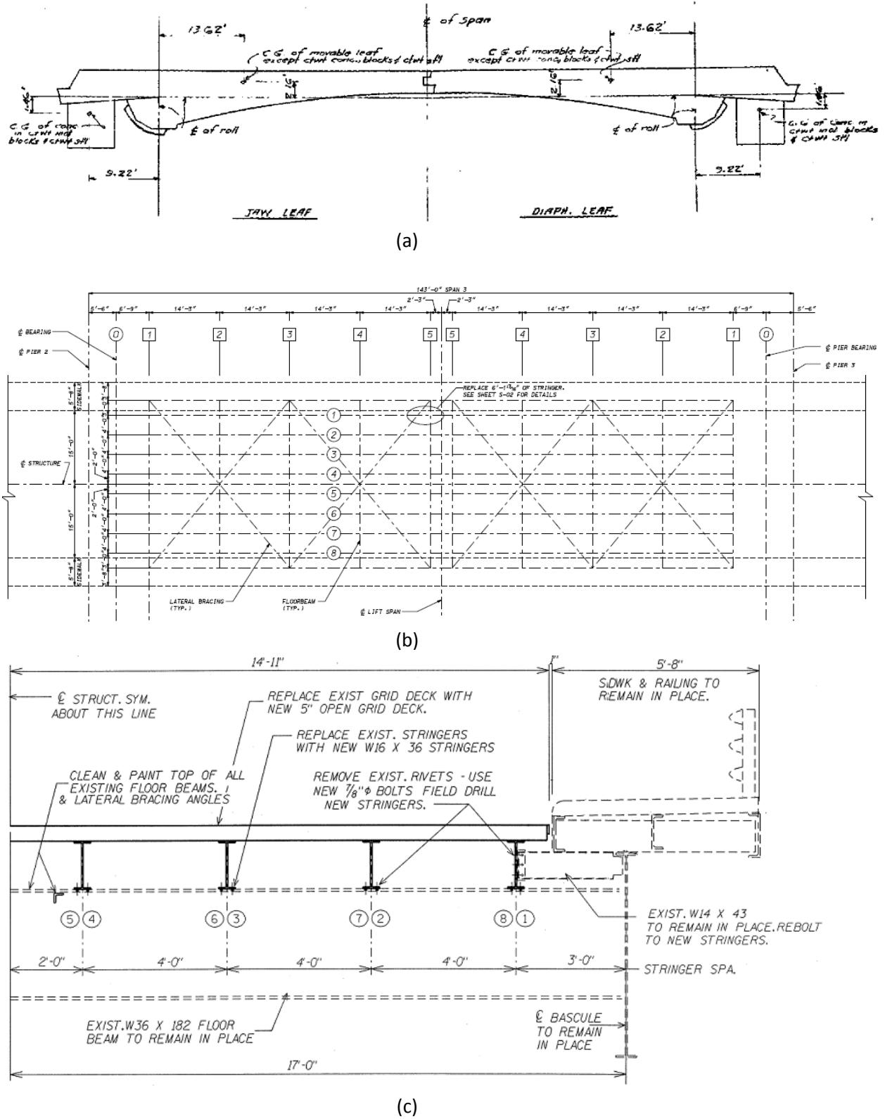
**Figure 4.1-3.** Marinette Bridge plans. (a) Elevation view with North to right (b) Framing plan. (c) Cross sectional view (half of the bridge). Adapted from WisDOT HSI database [10]
