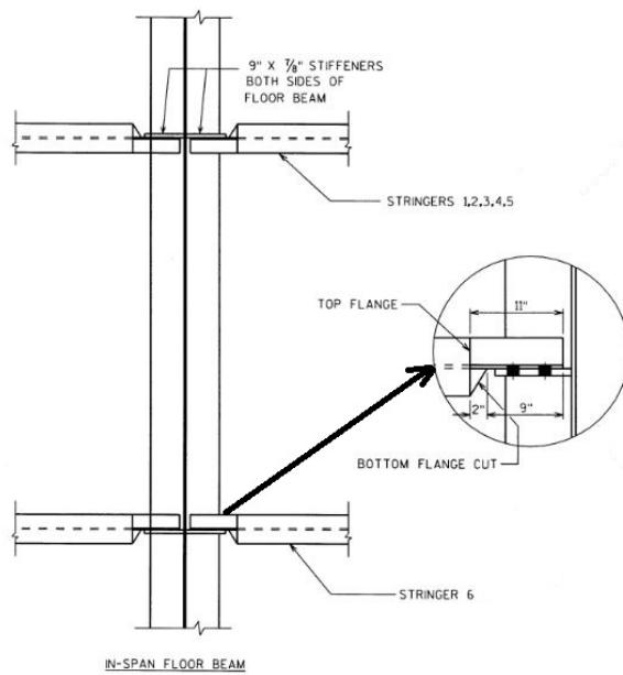
(b) Stringer and floor beam connection (plan view)
