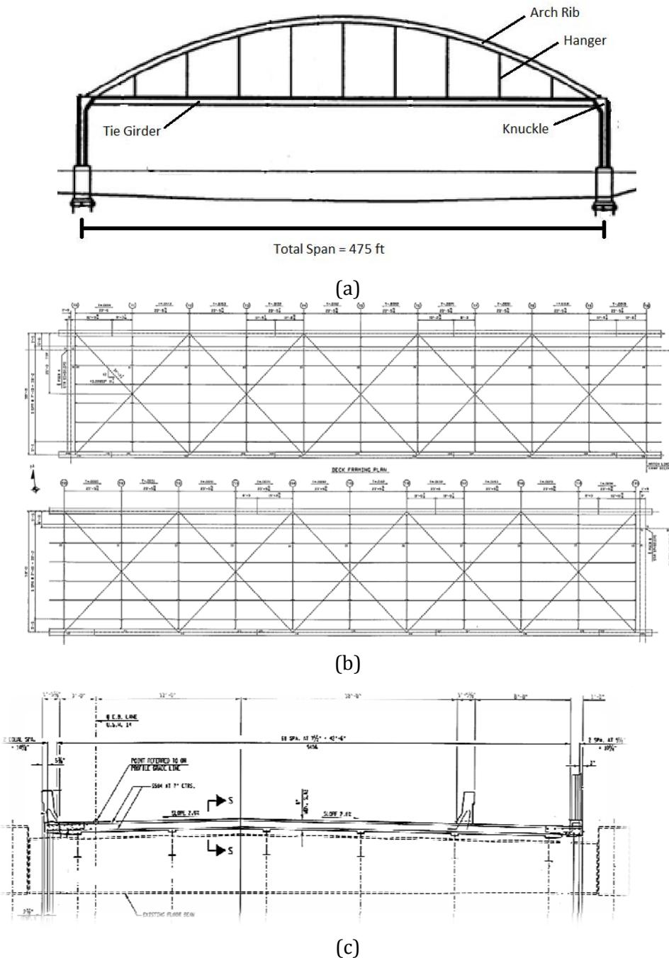
Figure 6.1-2. Plans of La Crosse Bridge structural components (a) Elevation view (b) Framing Plan (Upper is west half span, lower east half span) (c) Cross Section
