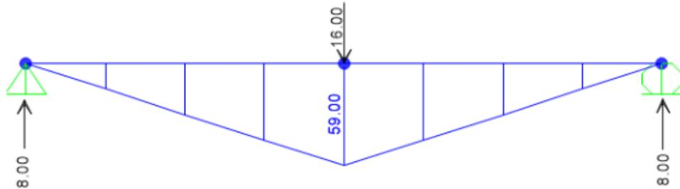
**Figure 9.3-1.** Moment with HL-93 wheel line load on a stringer span.
