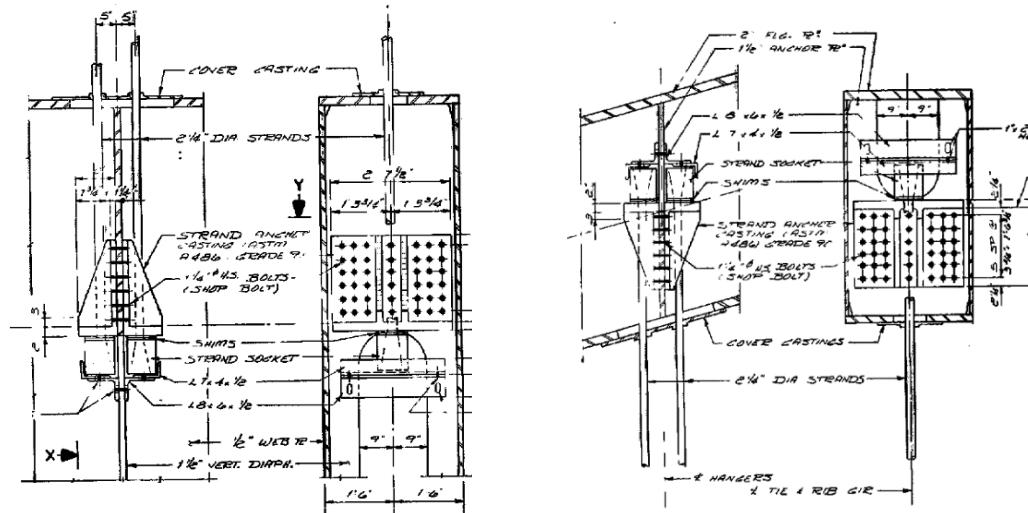
**Figure 8.1-3.** Connection details between hanger and girder (left), and arch (right).
