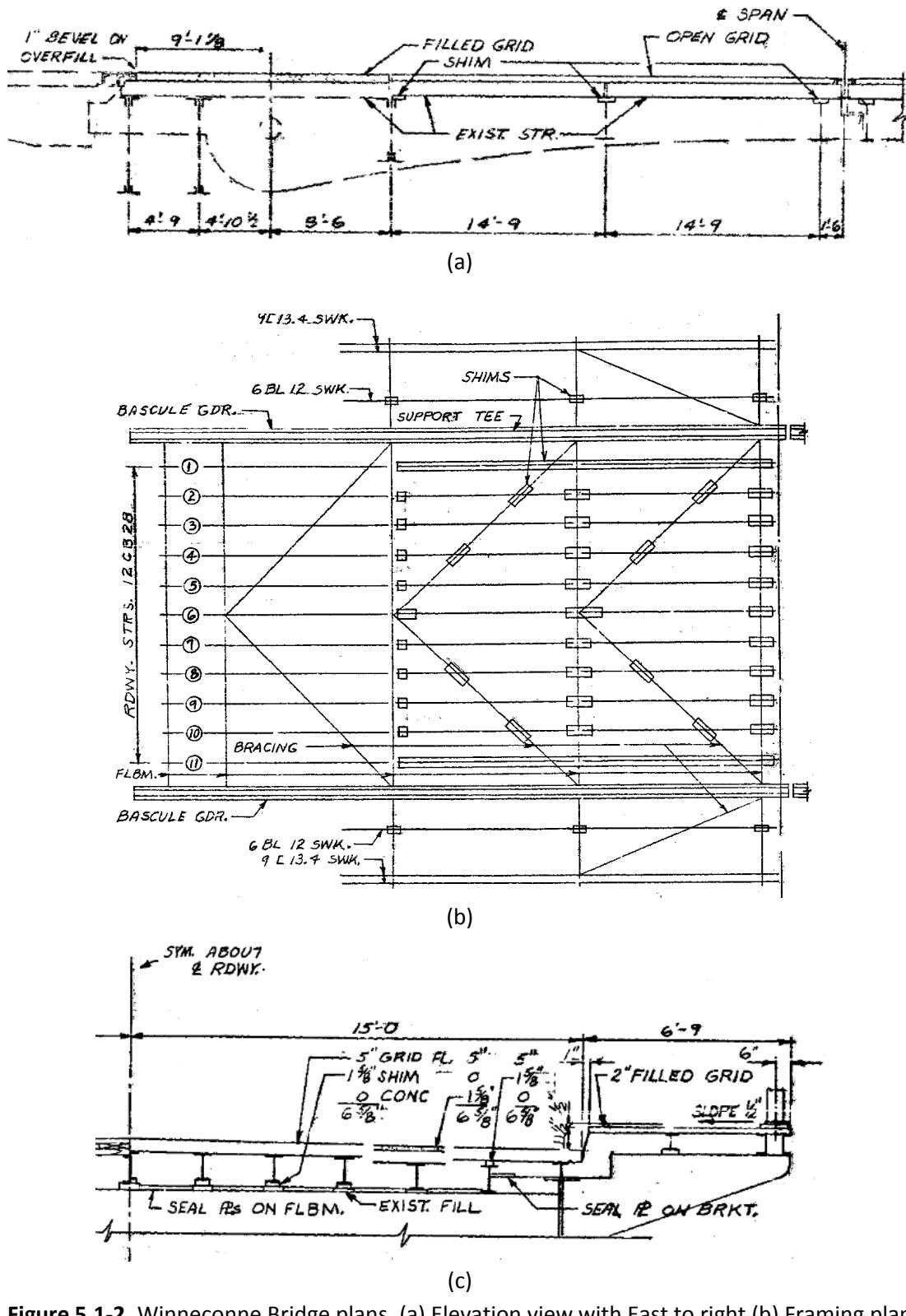
**Figure 5.1-2.** Winneconne Bridge plans. (a) Elevation view with East to right (b) Framing plan (half of bridge total span). (c) Cross sectional view (half of the bridge). Adapted from WisDOT HSI database [10].
