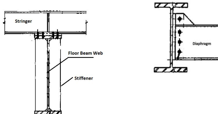
**Figure 8.1-5.** Floor beam and stringer, stringer and diaphragm connection details.
