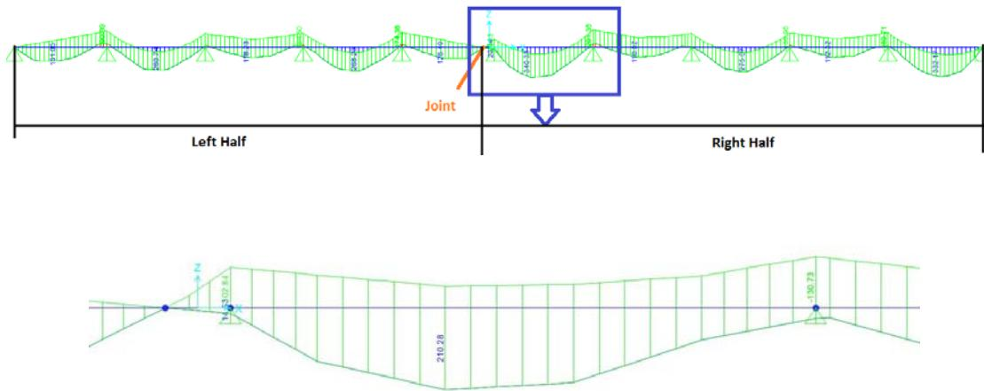
**Figure 9.6-1.** Moment envelope from HL-93 wheel line on continuous stringers and variation in 6<sup>th</sup> span with maximum positive moment.
