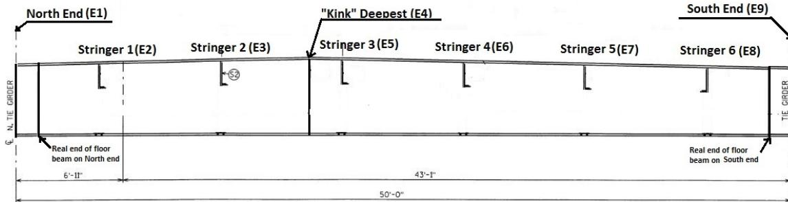
**Figure 6.3-2.** Floor beam frame element definition (Elevation view)
