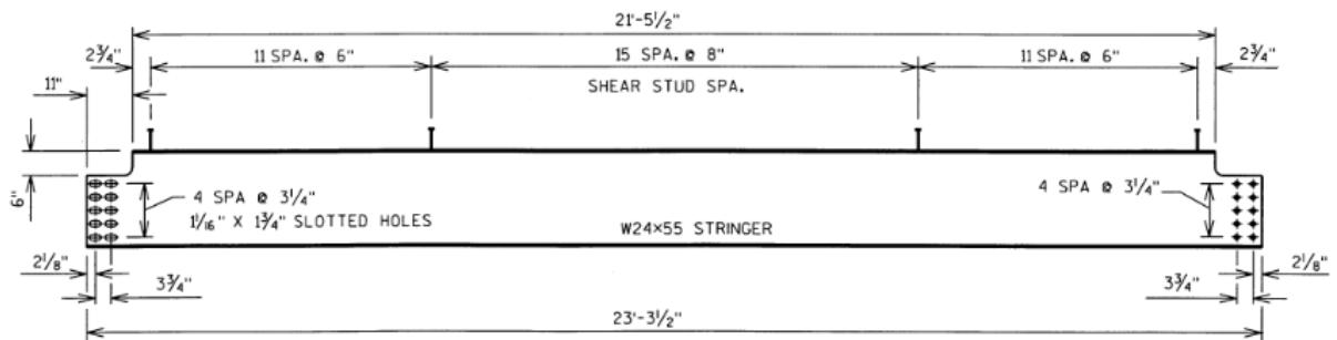
(a) Shear connection (studs) spacing on the stringers
