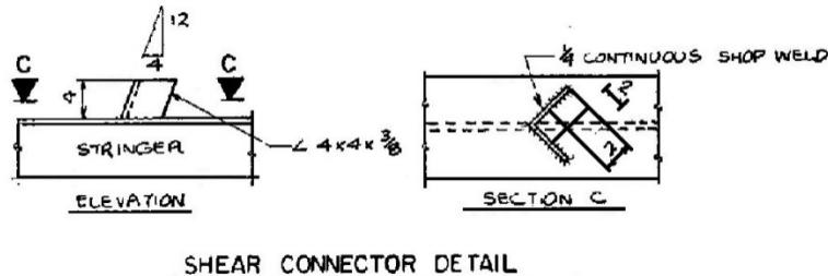
(c) Angle connector details (elevation and plan views)
