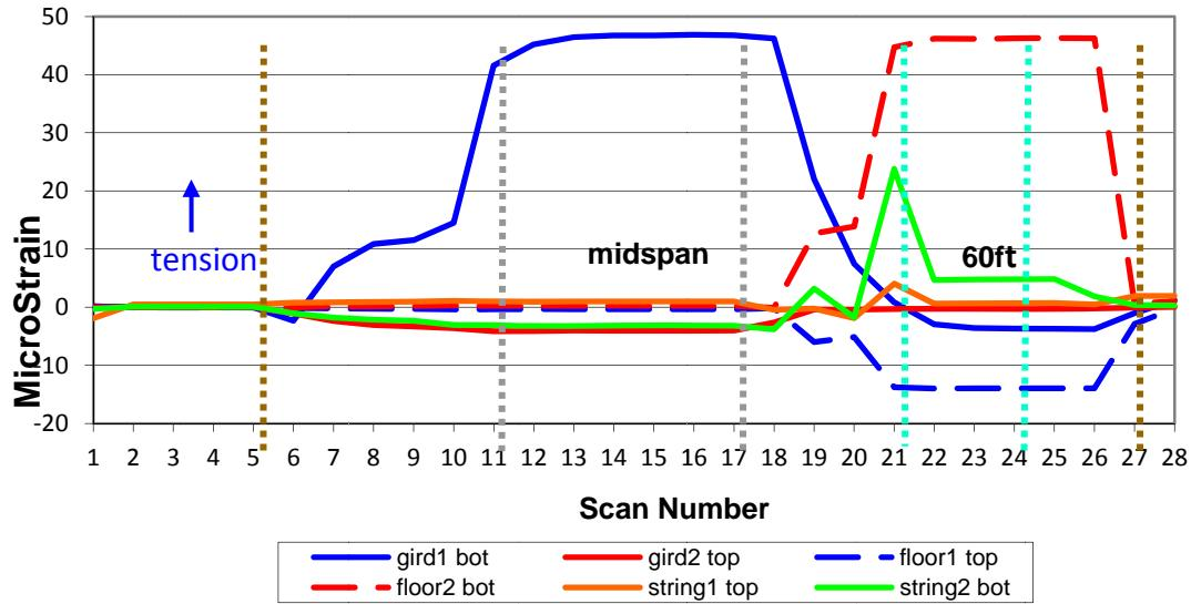
**Figure 3.2-6.** Strain gage values from field test.
