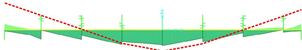
**Figure 9.5-4.** Comparison of 3D FEM predicted floor beam moment diagram (solid green) with a moment diagram from the fixed end simplified analysis (red dash) for the Dual500-2 OSOW truck loading.
