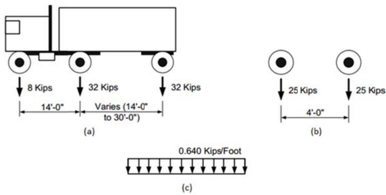
**Figure 2.1-3.** AASHTO HL-93 (a) design truck, (b) design tandem and (c) design lane.
