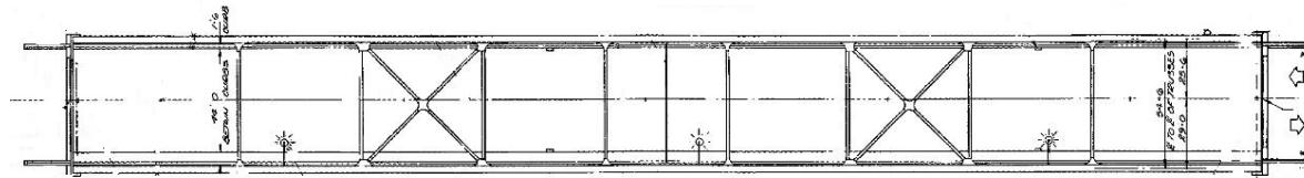
**Figure 7.1-7.** Arch bracing pattern - plan view.
