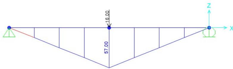
**Figure 9.2-1.** HL93 Wheel line moment diagram. Stringer moment is 57ft\*k multiplied by the AASHTO factor 0.73 = 42ft\*k.
