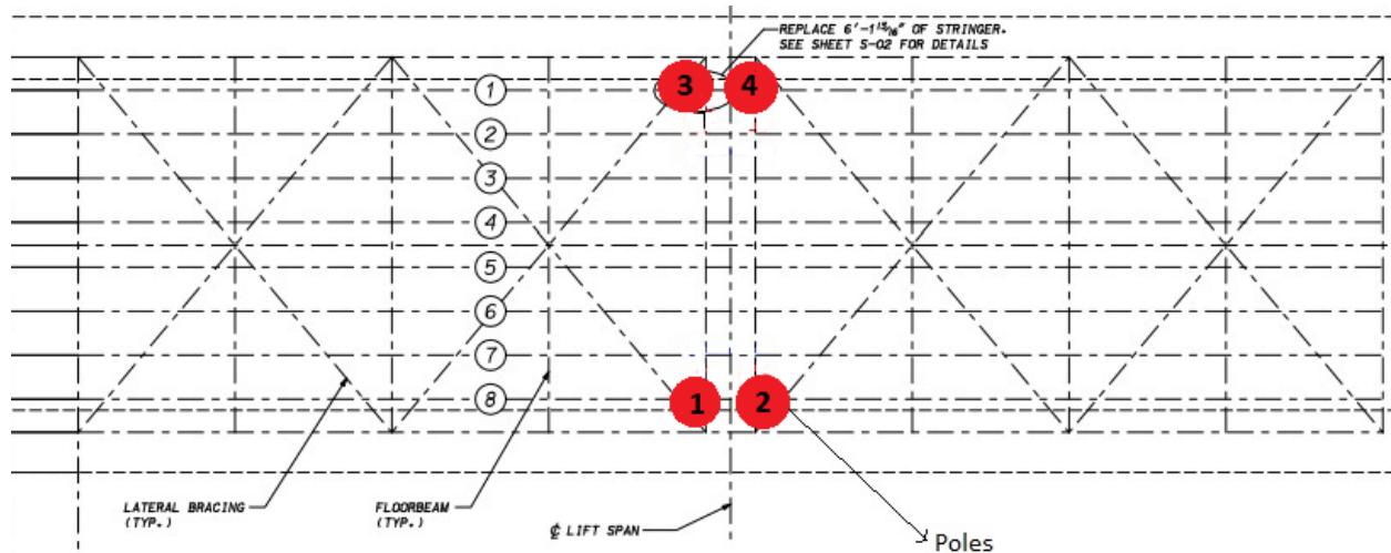
**Figure 4.2-3.** Deflection target locations during the bridge test.
