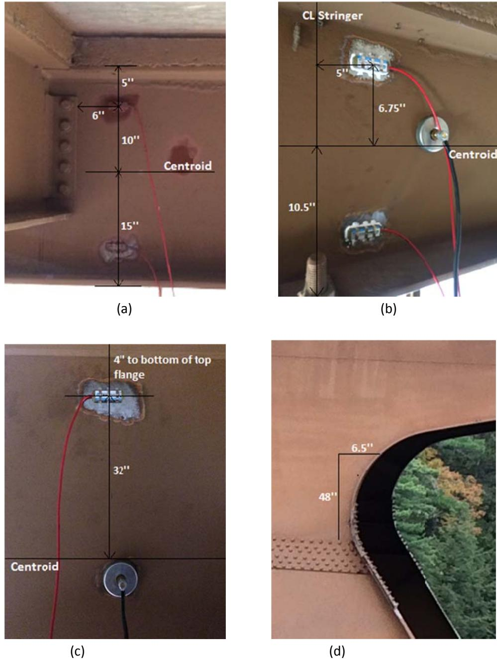
**Figure 3.2-2.** Location of gages for field test. (a) Vibrating strain gages at floor beam #14, 6 in. from stringer #2 web connection. (b) Vibrating strain gages at stringer #2, 115 in. from F.B #14. (c) Vibrating strain gage at girder, 90 in. south from bridge centerline. (d) Triaxial strain gage at knee-column, approximately 966 in. from south abutment and 135 in. from girder top flange.
