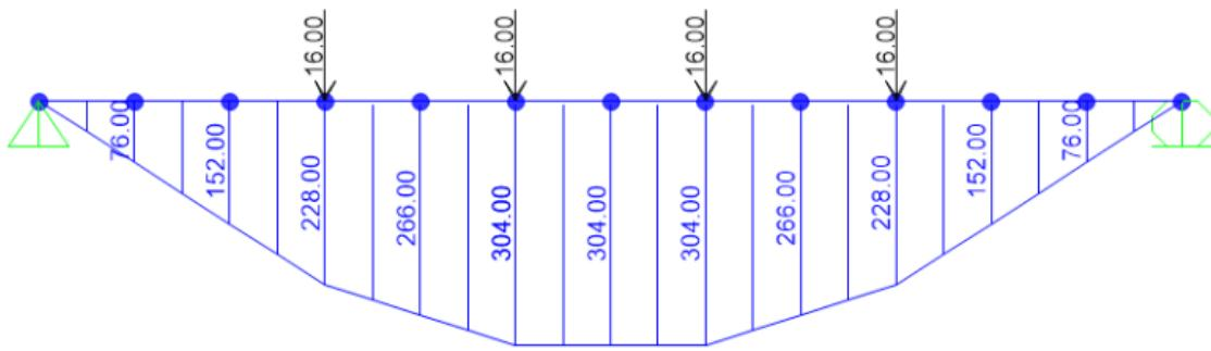
**Figure 9.3-3.** HL93 predicted floor beam moment diagram.
