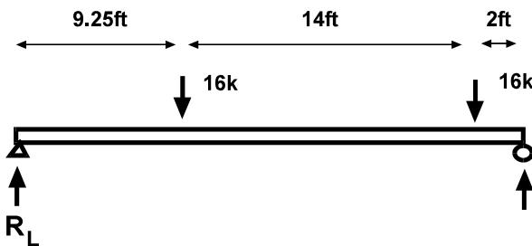
Figure 9.4-1. HL-93 truck position to cause max moment in stringer.
