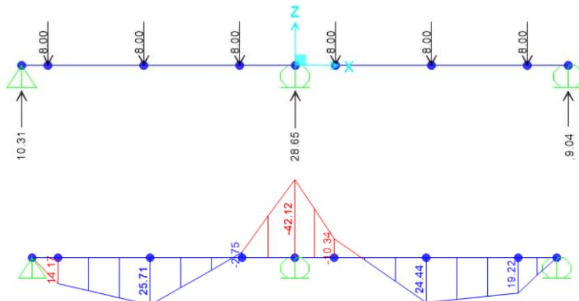
**Figure 9.2-2.** Dual500-2 Wheel line moment diagram with min negative moment over support. Stringer moment predicted as -42ft\*k multiplied by 0.74 factor = -31.2ft\*k. Alternate distribution factor of 1.5 would give -63ft-k.
