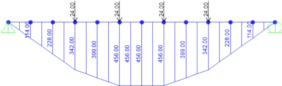
**Figure 9.3-4.** Predicted Dual500-6 induced floor beam moment diagram.
