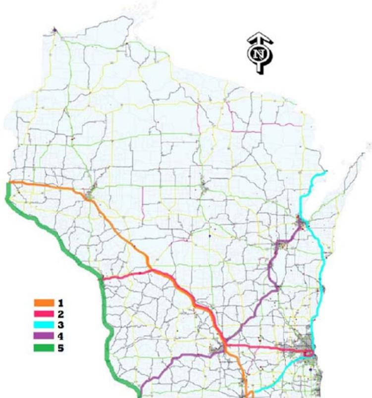
**Figure 1.2-1.** Critical routes for OSOW truck permitting in Wisconsin.
