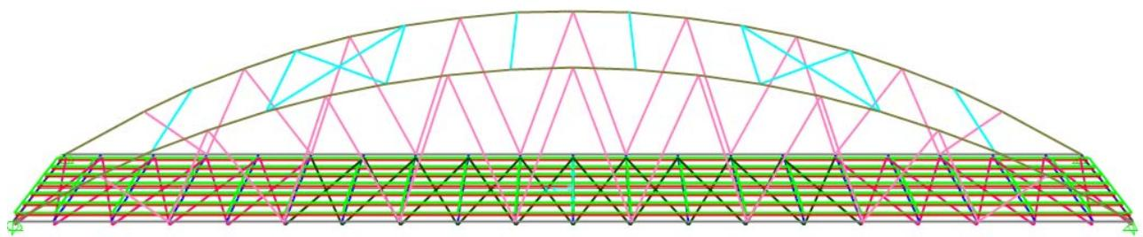
**Figure 7.2-1.** 3D finite-element-model of the Chippewa River Memorial Bridge.
