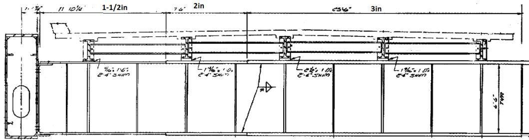
**Figure 8.1-4.** Typical Floor Beam Elevation View, 1/2 span.
