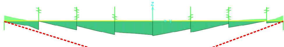
**Figure 9.5-5.** Comparison of 3D FEM predicted floor beam moment diagram (solid green) with a moment diagram from the pin ended simplified analysis (red dash) for the Dual500-2 OSOW truck loading.
