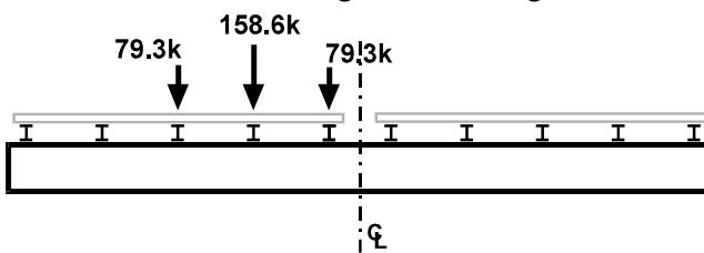
**Figure 9.6-3.** Simulated Dual500-2 loading on a Frigo floor beam.
