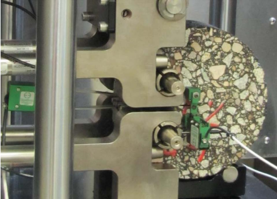
**Figure 3.43 DC(T) Test Configuration – Closer View**
