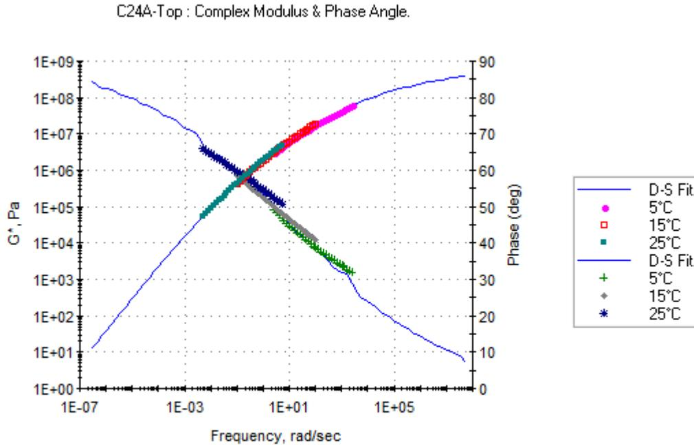
**Figure 3.11 Example Mastercurve Generated from DSR Temperature-Frequency Sweep Testing**
