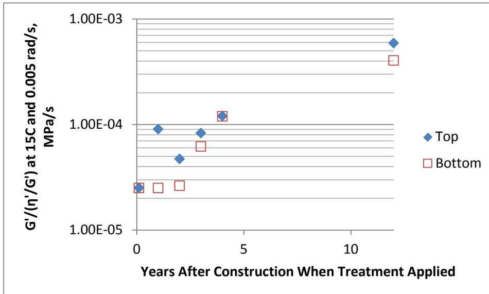
Figure 4.33  $G''/(\eta'G')$  Parameter as a Function of Time When Sealing Occurred
