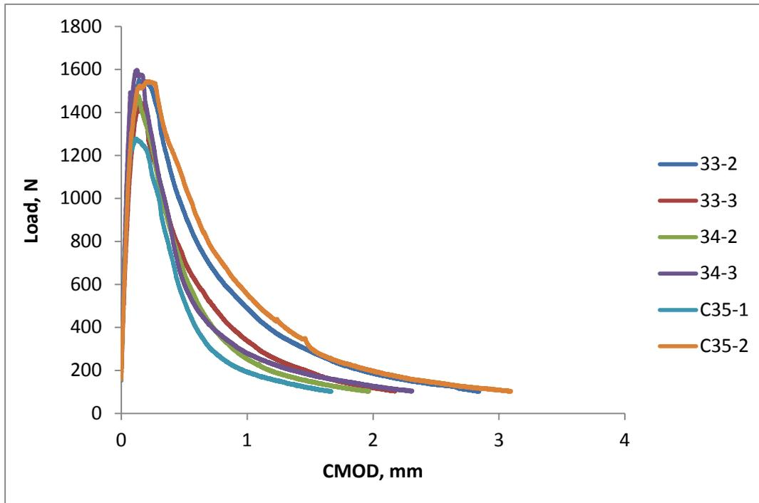
Figure 3.46 DC(T) Load vs. CMOD Curves for Cells 33-35
