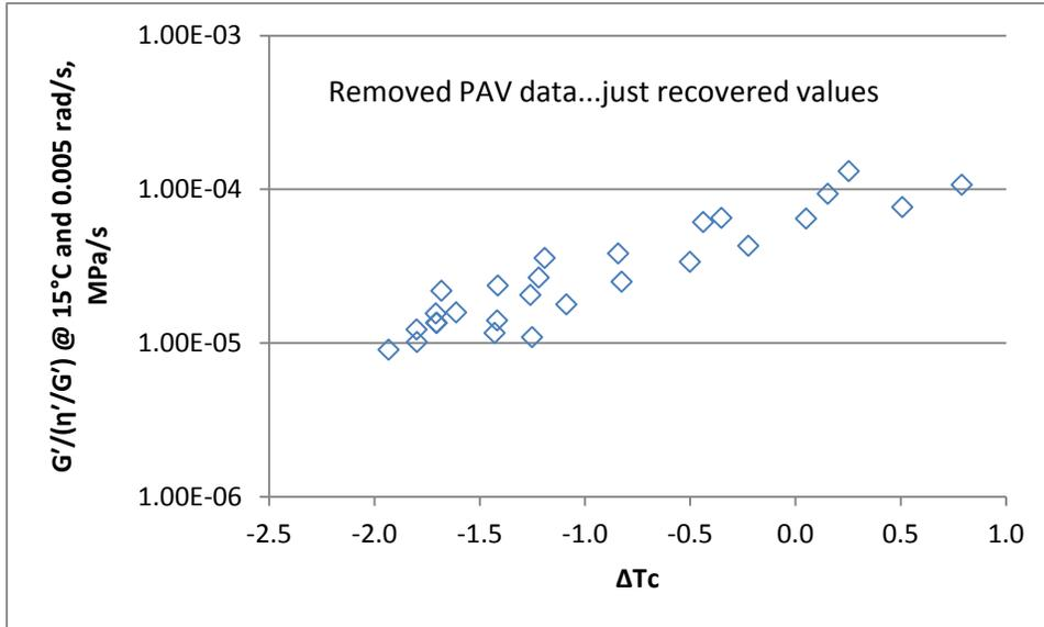
**Figure 3.25 Comparison of  $G' / (\eta' / G')$  and  $\Delta T_c$  – Recovered Binder Data**
