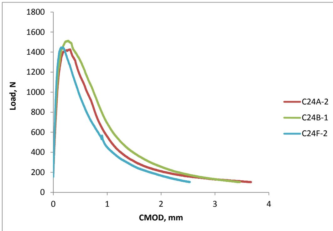
**Figure 3.45 DC(T) Load vs. CMOD Curves for Cell 24**
