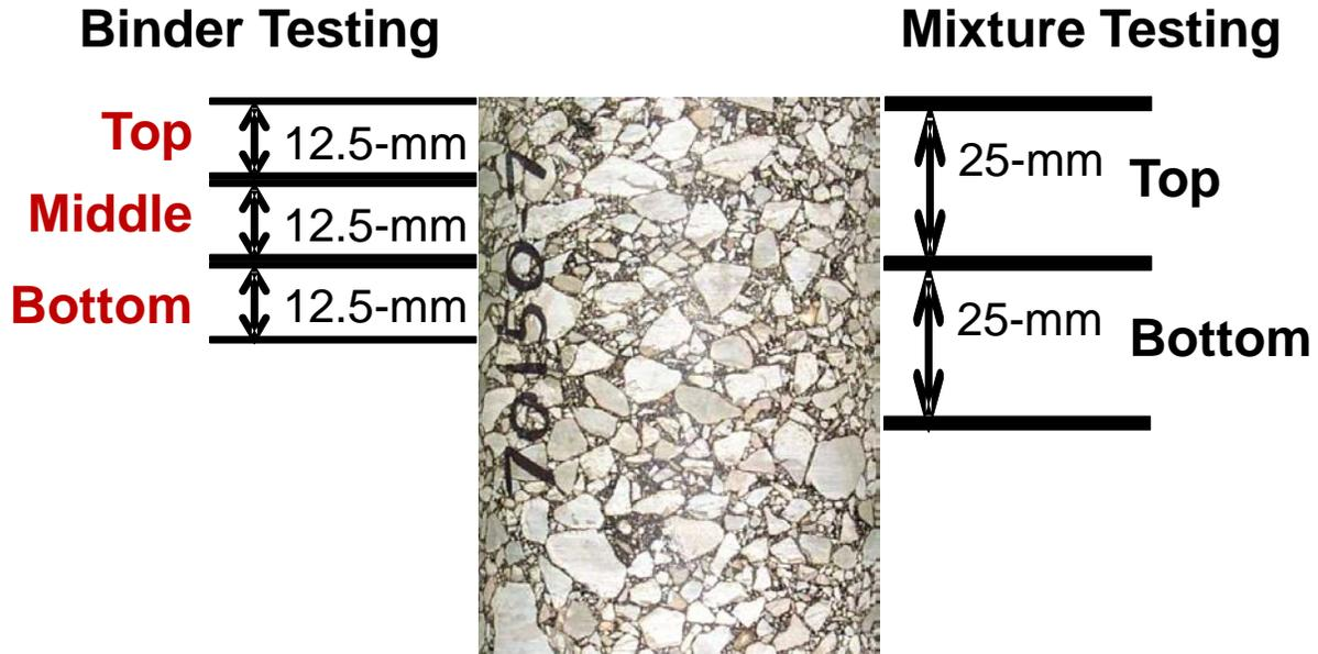
Figure 4.21 Layer Designations for Binder and Mixture Testing
