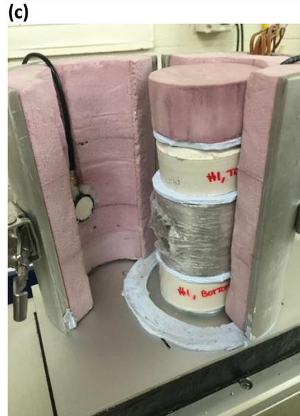
Figure 8 - Current Testing States (a) Sorption samples conditioning at 50% relative humidity (b) Sample labeling convention cut and cored LGCC sample (c) LGCC Test Setup.
