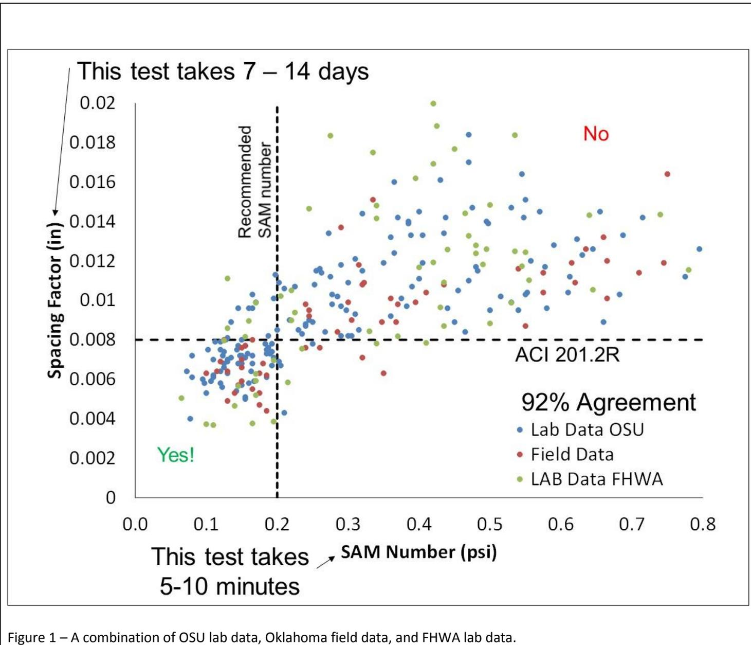
Figure 1 – A combination of OSU lab data, Oklahoma field data, and FHWA lab data.
