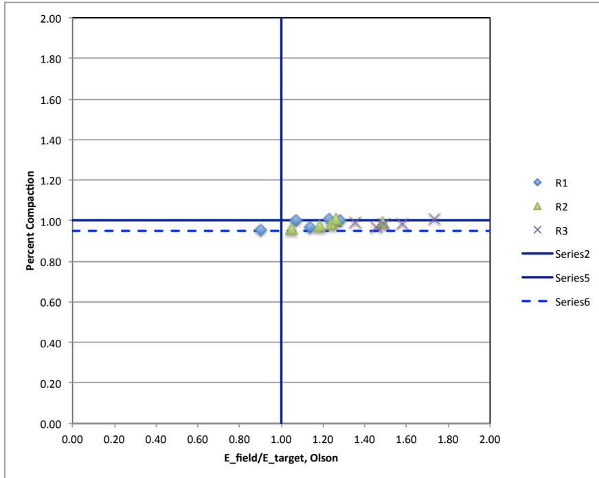
Figure 16- PC vs. Field to Target modulus ratio for Olson LWD.
