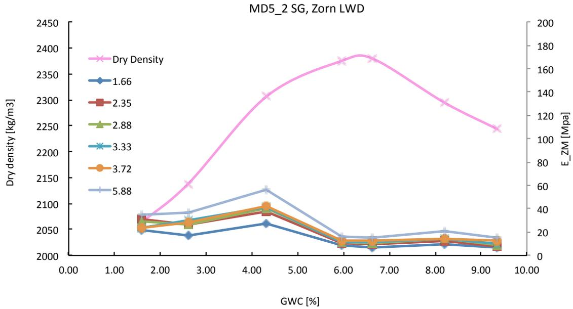
Figure 7- Zorn LWD modulus on Proctor mold for different stress states (P/Pa) and Dry Density versus GWC.
