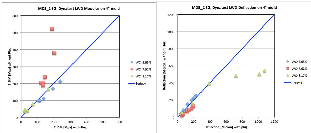
Figure 21. Measured modulus and deflection on 4 inch Proctor mold for Dynatest LWD with and without plug.
