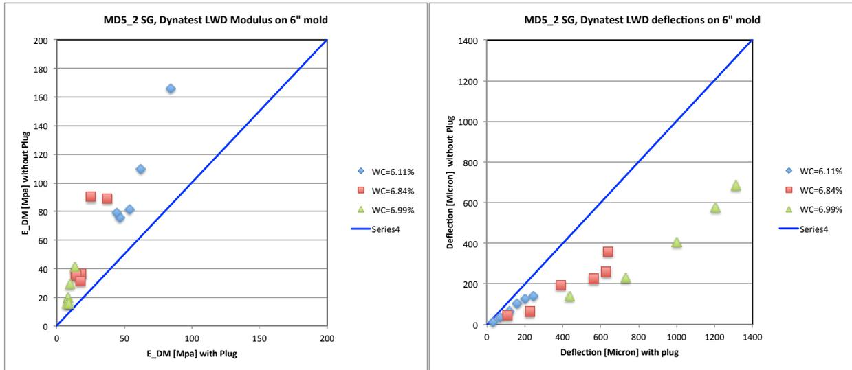
Figure 23. Measured modulus and deflection on 6 inch Proctor mold for Dynatest LWD with and without plug.
