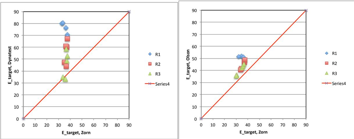
Figure 18- LWDs calculated Target modulus correlation.
