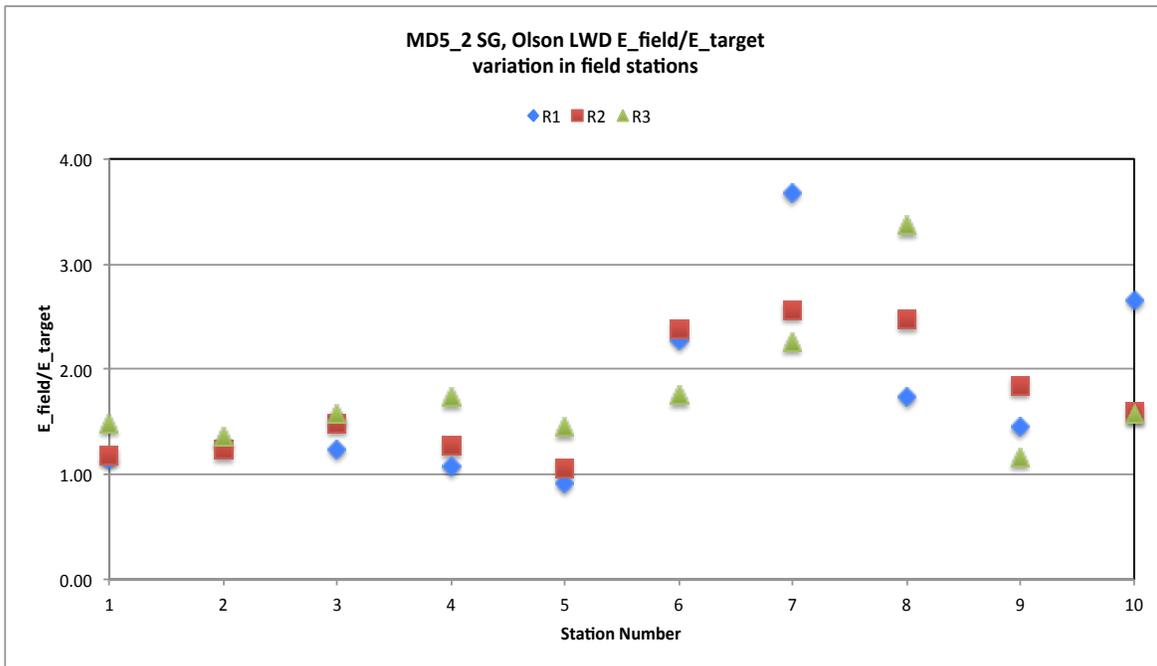
Figure 13- Measured field modulus to calculated target modulus ratio: Olson LWD.
