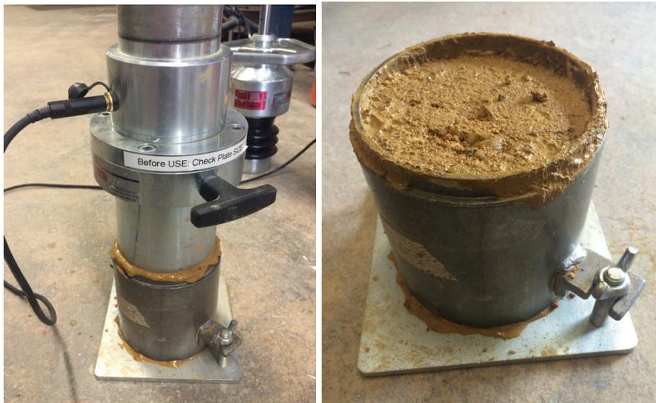
Figure 45- Permanent deformation and unlevelled surface in the 4 inch mold after testing with Zorn LWD.
