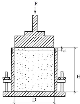
Figure 2- Schematic of LWD testing on Proctor mold. (Tefa, 2015).
