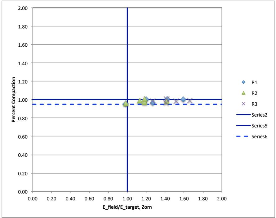
Figure 14- PC vs. Field to Target modulus ratio for Zorn LWD.
