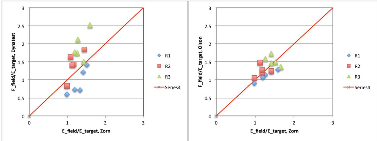
Figure 19- LWDs Field to Target modulus correlation.
