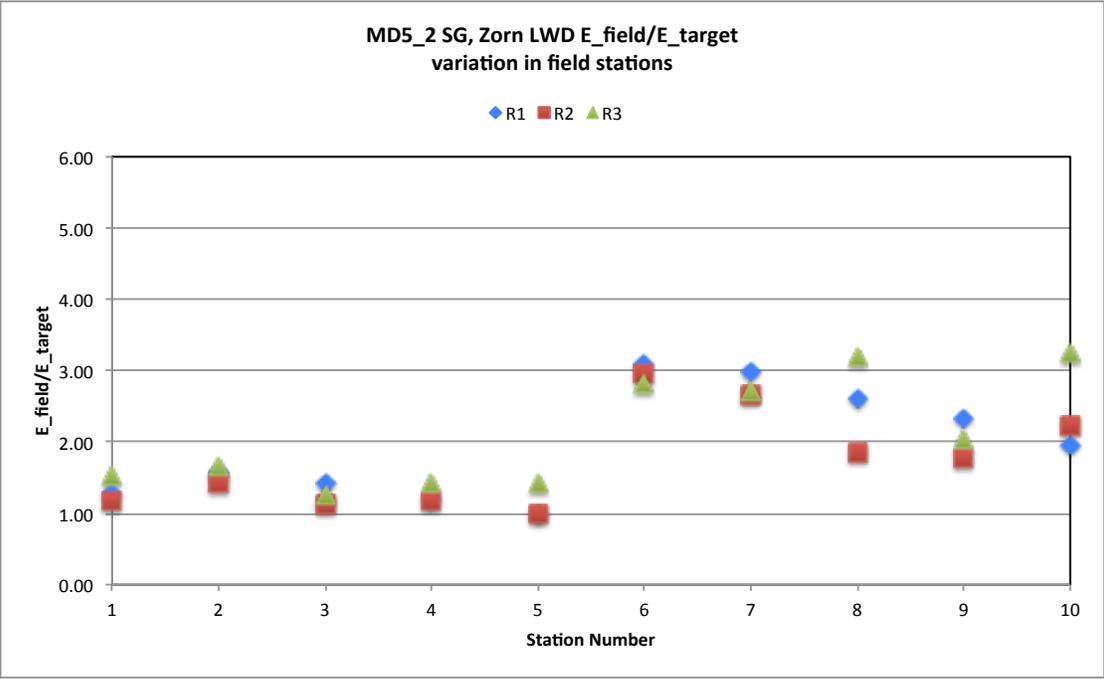
Figure 11- Measured field modulus to calculated target modulus ratio: Zorn LWD.
