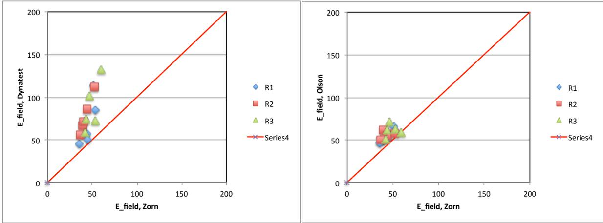
Figure 17- LWDs Field measured modulus correlation.
