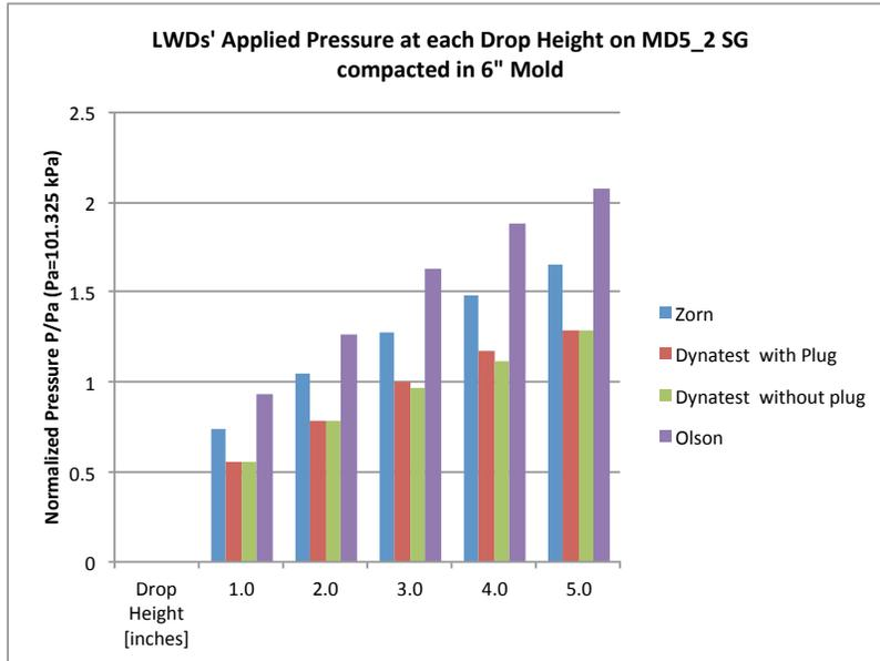
Figure 22- Applied pressure on 6 inch Proctor Mold for Zorn, Olson, and Dynatest LWDs (Dynatest with and without plug).
