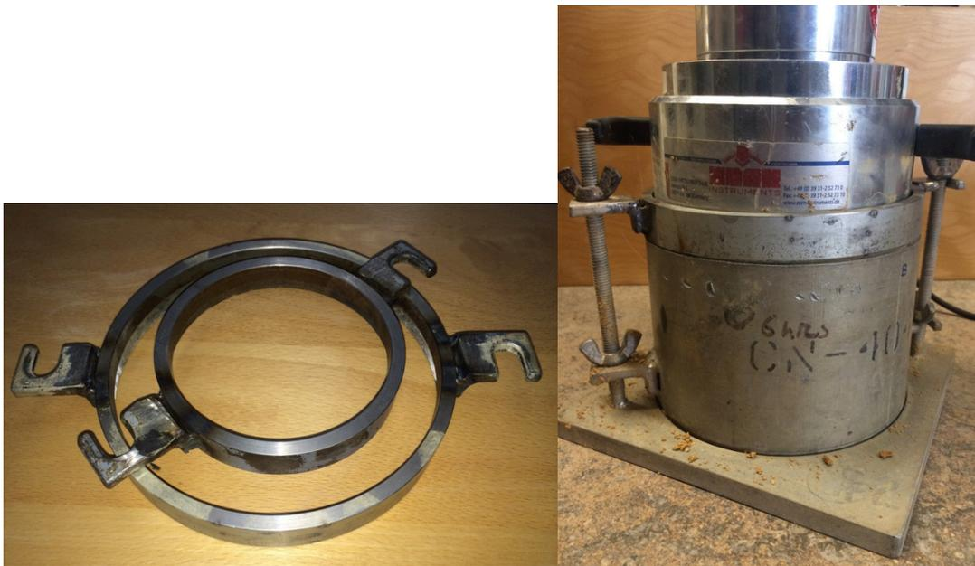
Figure 44- Collar designed for 4 inch and 6 inch molds.
