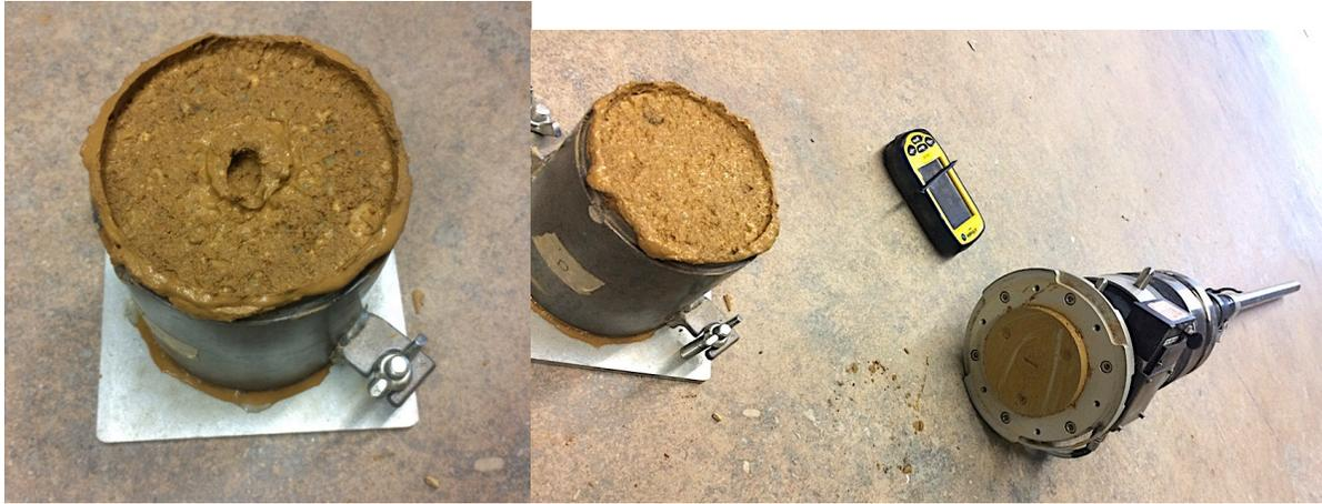
Figure 10- Measuring deflection directly on top of soil versus plate deflection using Plugin with Dynatest LWD
