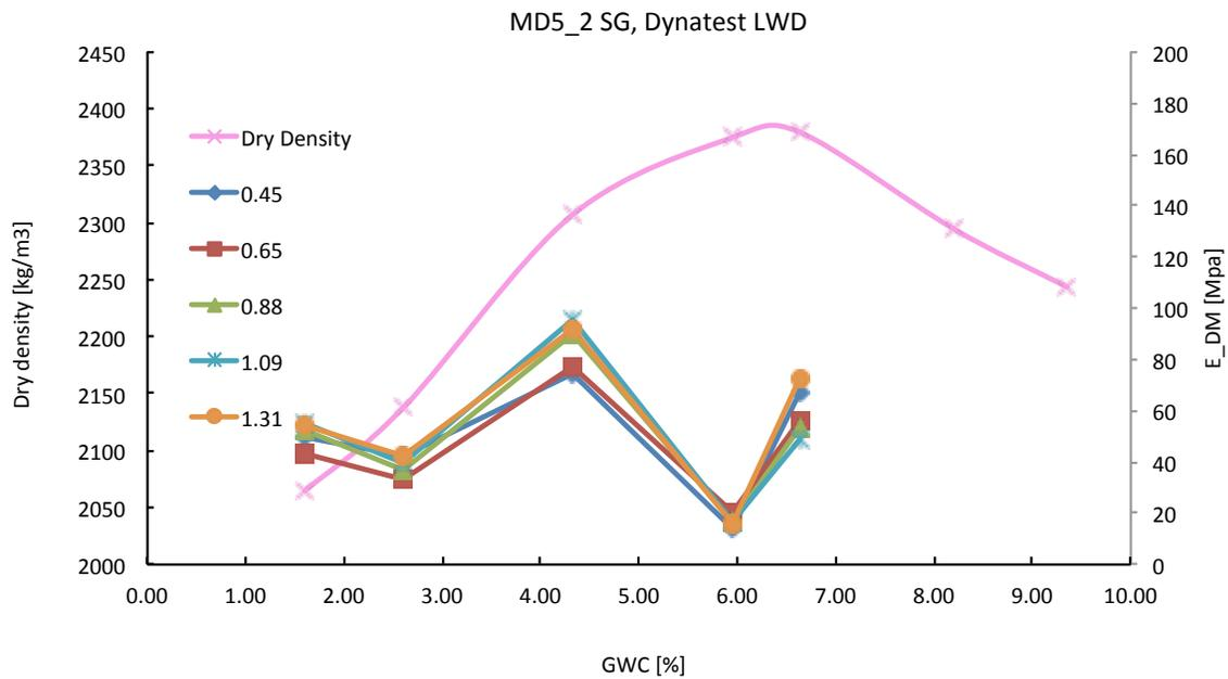
Figure 8- Dynatest LWD modulus on Proctor mold for different stress states (P/Pa) and Dry Density versus GWC.
