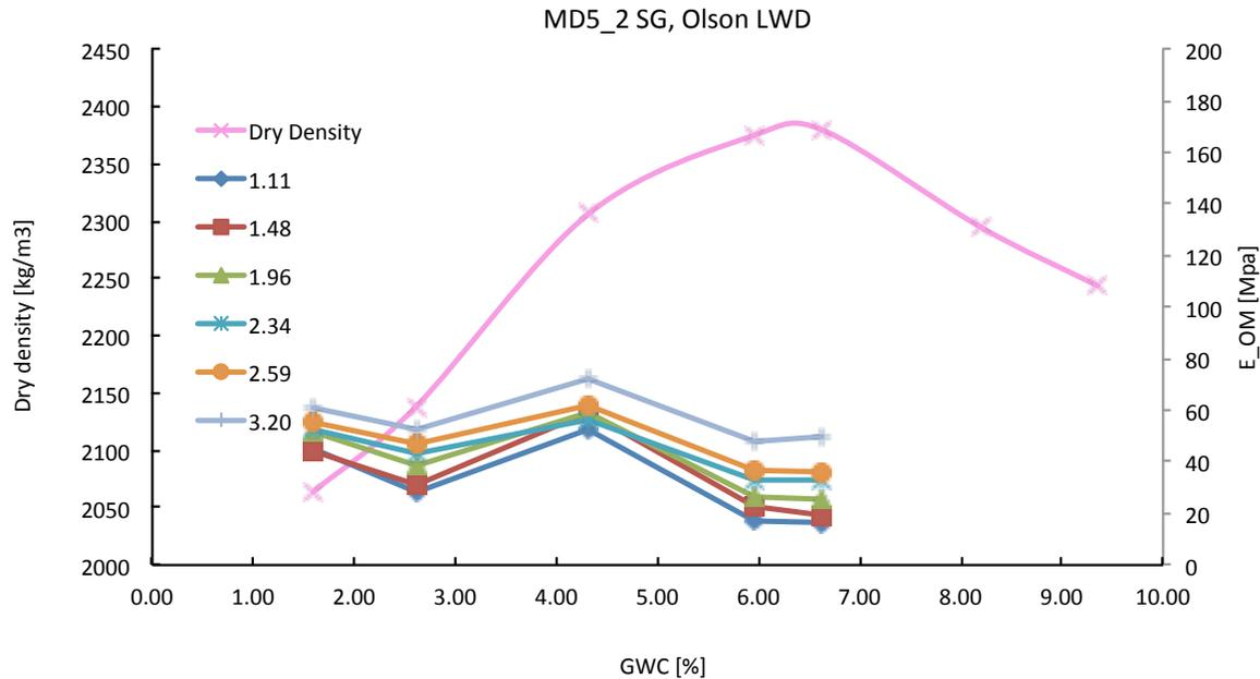
Figure 9- Olson LWD modulus on Proctor mold for different stress states (P/Pa) and Dry Density versus GWC.
