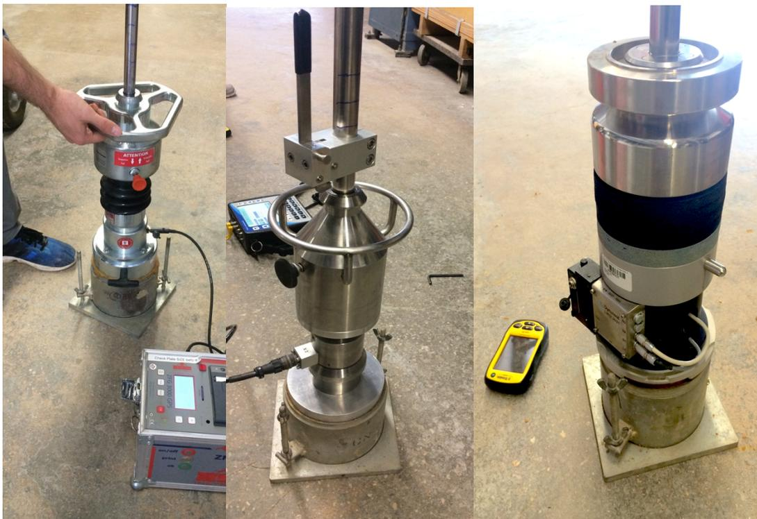
Figure 1- Zorn, Olson and Dynatest LWDs on 6 inch Proctor molds.
