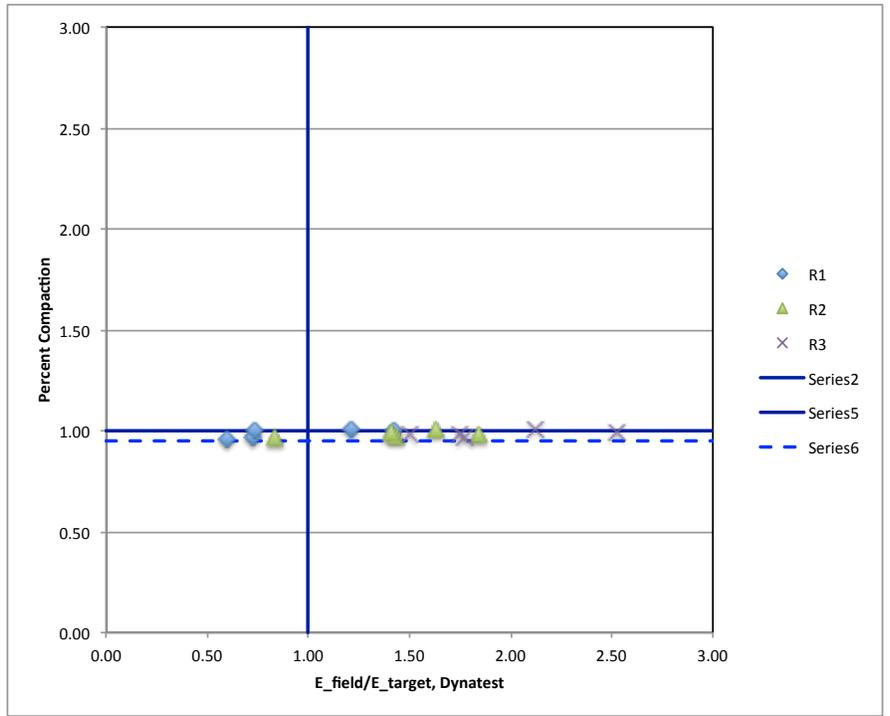
Figure 15- PC vs. Field to Target modulus ratio for Dynatest LWD.
