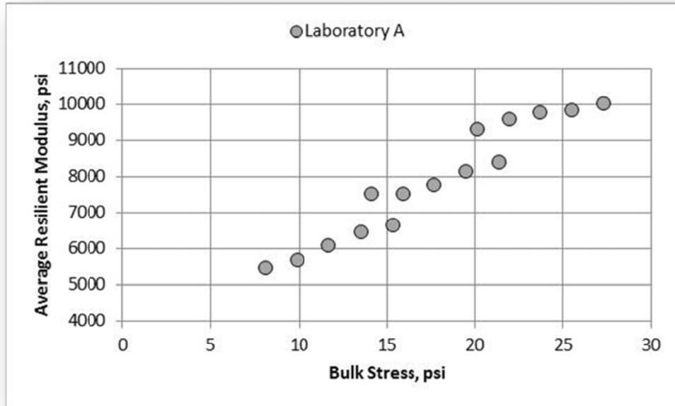
**Figure 92. A-2-4 Soil (NCAT Subgrade), Laboratory A, Resilient Modulus**
