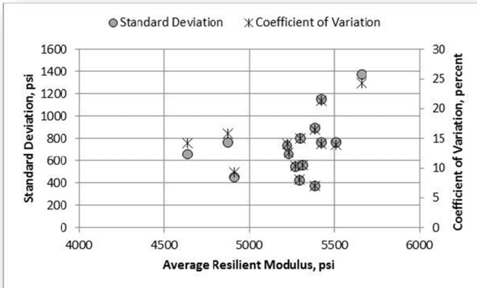
Figure 91. A-7-6 Soil, Laboratory I, Standard Deviation and Coefficient of Variation
