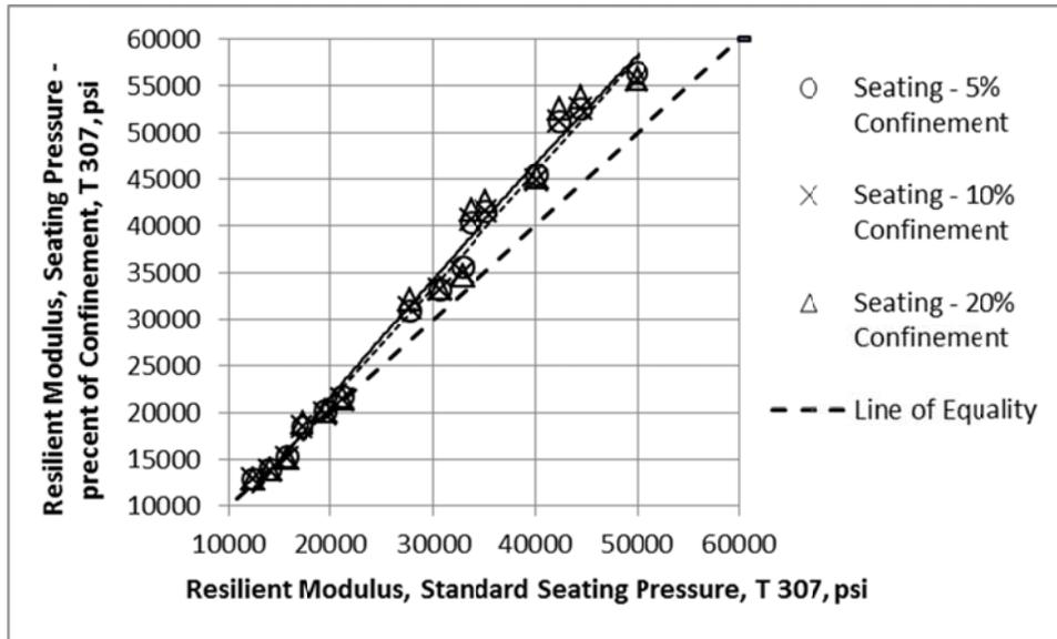
Figure 5. Effect of Seating Load on Resilient Modulus for the GAB Material, AASHTO T 307
