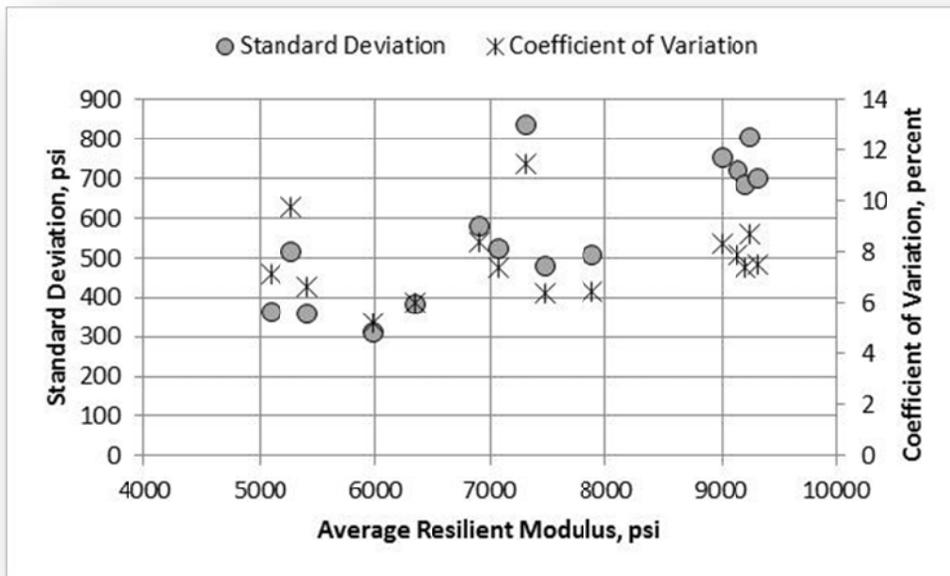
Figure 103. A-2-4 Soil (NCAT Subgrade), Laboratory F, Standard Deviation and Coefficient of Variation
