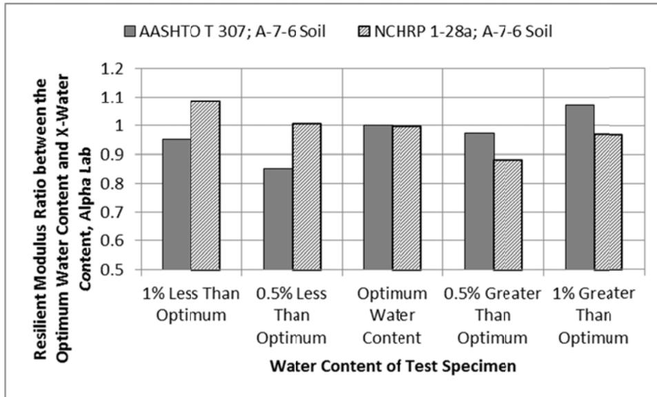
Figure 33. Effect of Water Content on Resilient Modulus Ratio; Alpha Laboratory
