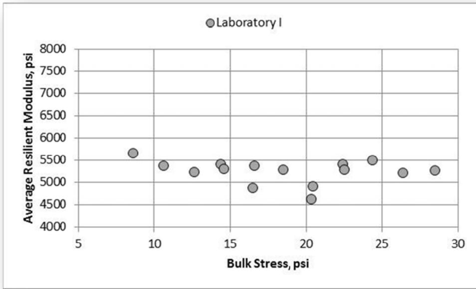
Figure 90. A-7-6 Soil, Laboratory I, Resilient Modulus
