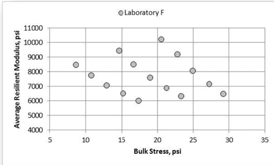
Figure 82. A-7-6 Soil, Laboratory F, Resilient Modulus
