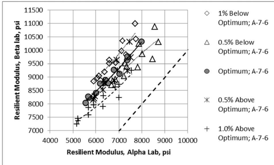
**Figure 36. Comparison of Resilient Modulus between the Alpha and Beta Laboratories; A-7-6 Soil**
