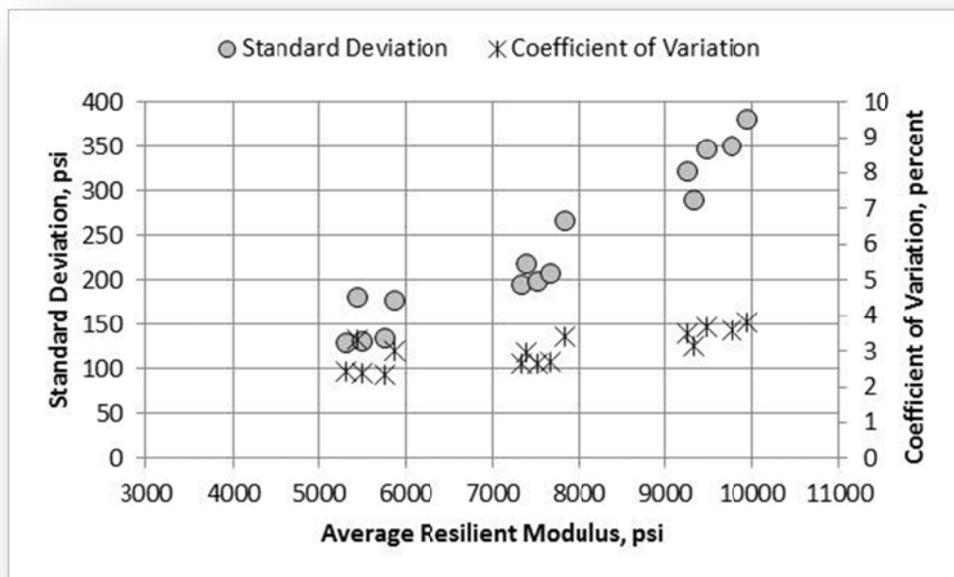
Figure 111. A-2-4 Soil (Low Plasticity), Laboratory A, Standard Deviation and Coefficient of Variation
