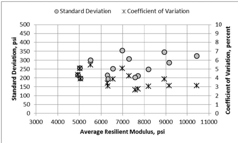
**Figure 53. Variation of Resilient Modulus Values for Different Stress States as Measured by Laboratory H for the Georgia A-2-4 Silty Sand Soil**
