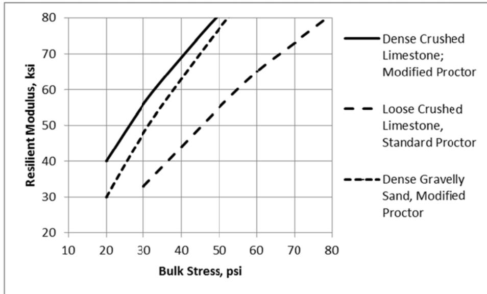
**Figure 65. Some Typical Resilient Modulus Test Results from the Corp of Engineers**
