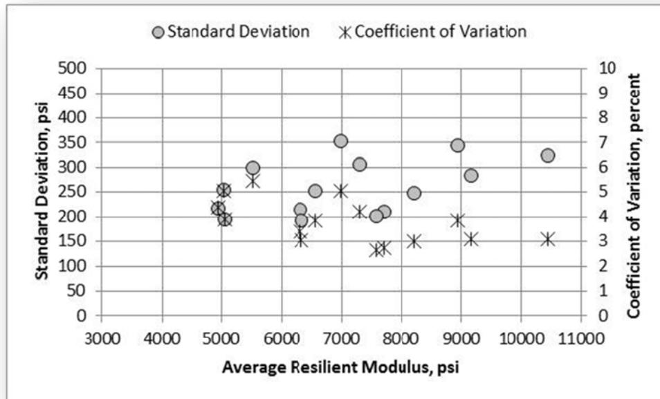
Figure 119. A-2-4 Soil (Low Plasticity), Laboratory H, Standard Deviation and Coefficient of Variation
