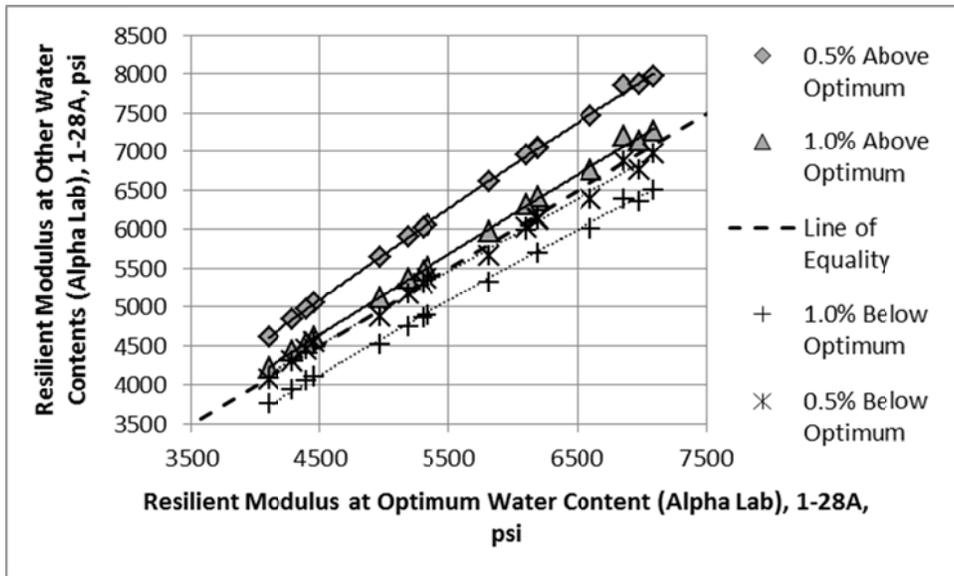
Figure 29. Effect of Water Content on Resilient Modulus Measured in accordance with NCHRP 1-28a Procedures for the A-7-6 Soil, Alpha Laboratory
