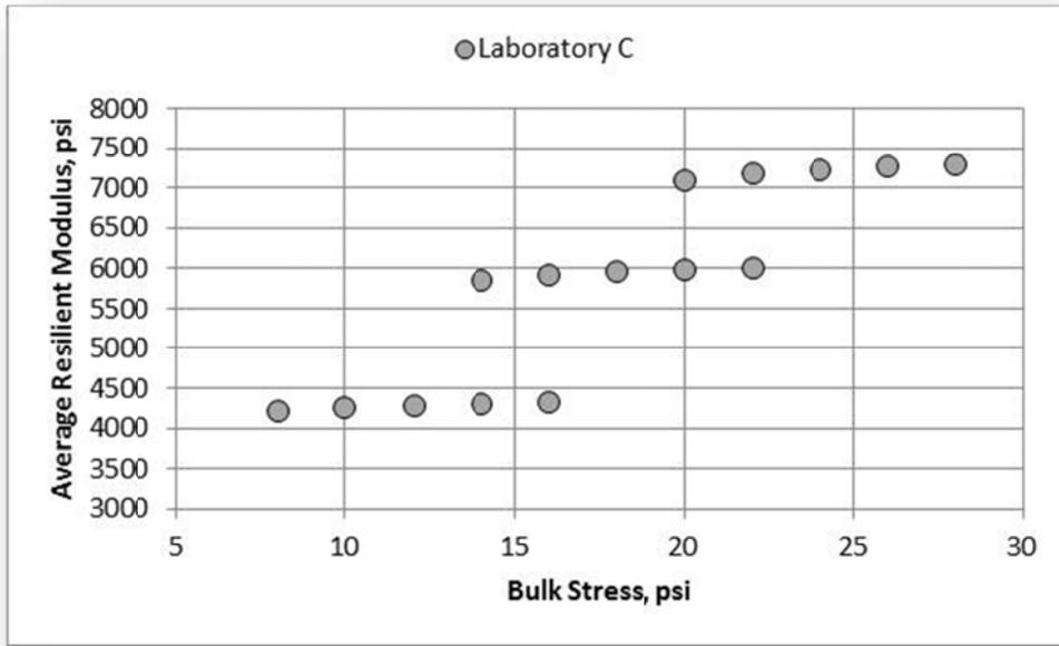
Figure 96. A-2-4 Soil (NCAT Subgrade), Laboratory C, Resilient Modulus
