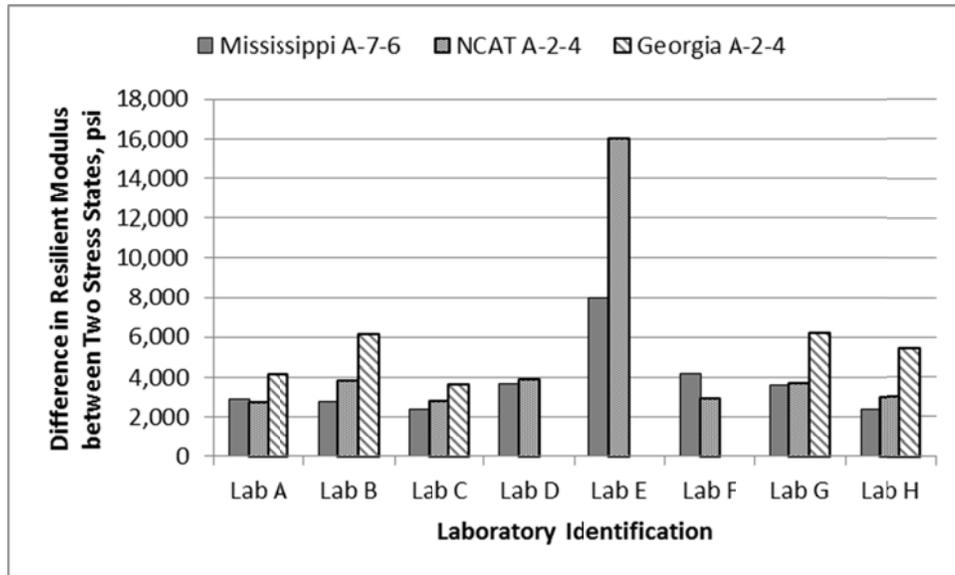
**Figure 54. Average Difference in Resilient Modulus between Two Stress States**
