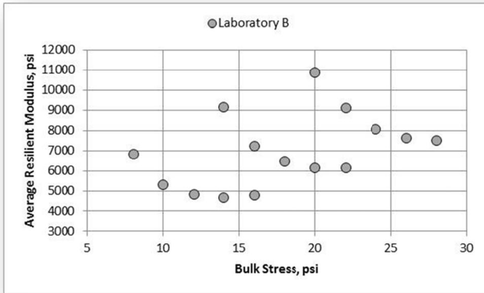
Figure 112. A-2-4 Soil (Low Plasticity), Laboratory B, Resilient Modulus
