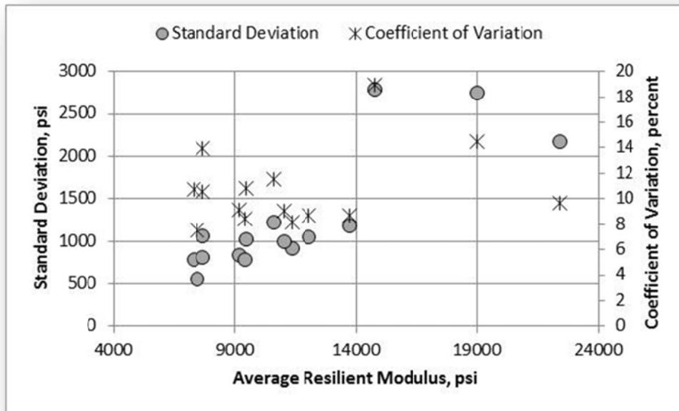
Figure 101. A-2-4 Soil (NCAT Subgrade), Laboratory E, Standard Deviation and Coefficient of Variation
