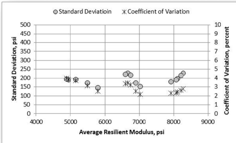
Figure 77. A-7-6 Soil, Laboratory C, Standard Deviation and Coefficient of Variation
