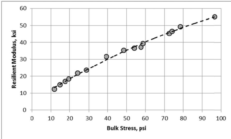
**Figure 63. Crushed Gravel Aggregate Base; Repeated Load Resilient Modulus Tests
