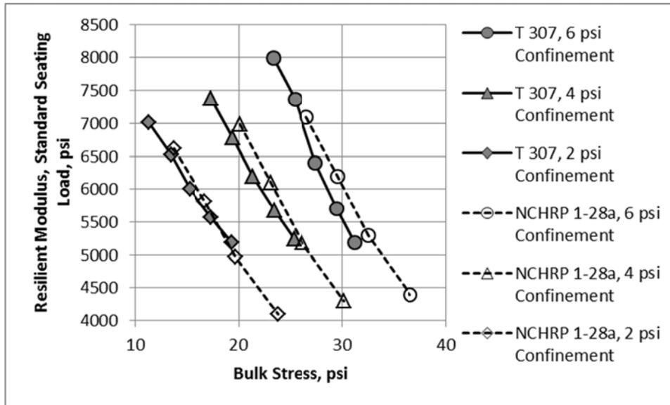
**Figure 9. Resilient Modulus Measured in Accordance with AASHTO T 307 and NCHRP 1-28a Procedures Using the Standard Seating Loads Designated by each Procedure for the A-7-6 Soil**
