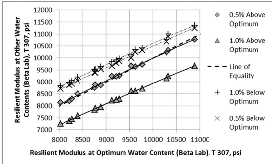
**Figure 30. Effect of Water Content on Resilient Modulus Measured in Accordance with AASHTO T 307 for the A-7-6 Soil, Beta Laboratory**
