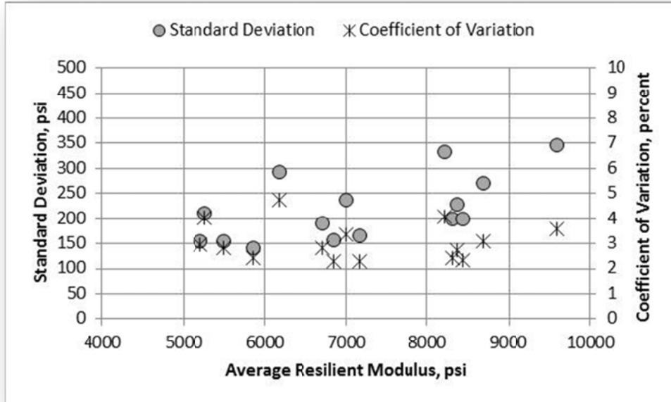
Figure 95. A-2-4 Soil (NCAT Subgrade), Laboratory B, Standard Deviation and Coefficient of Variation
