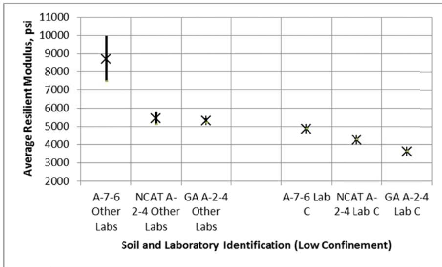
**Figure 56. Average Resilient Modulus Measured at Low Confinement (2 psi) and 4 psi Vertical Stress for the Different Embankment Soils**
