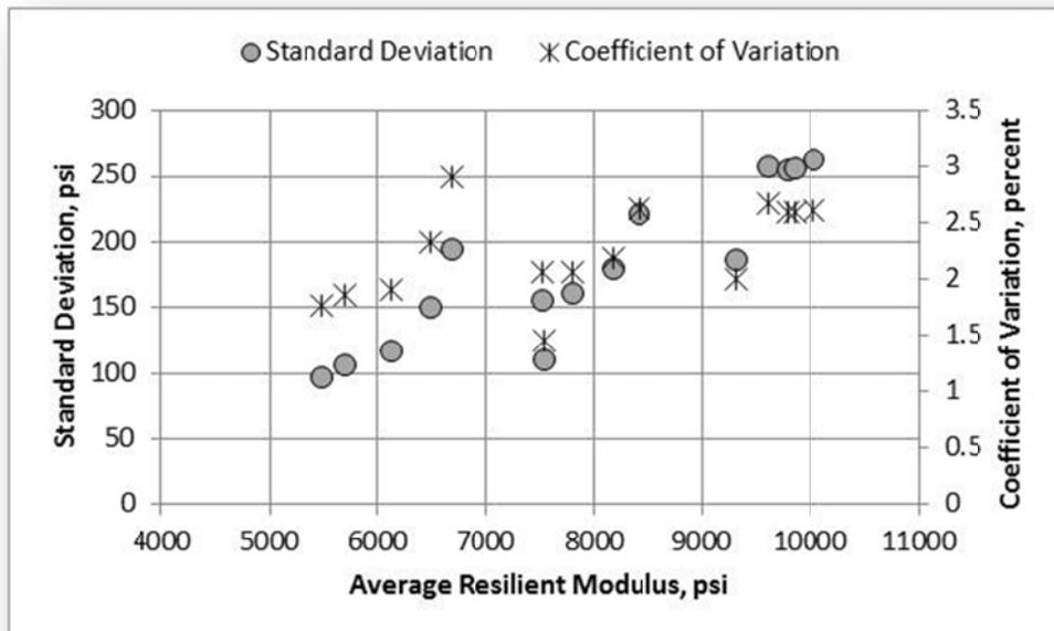
**Figure 93. A-2-4 Soil (NCAT Subgrade), Laboratory A, Standard Deviation and Coefficient of Variation**
