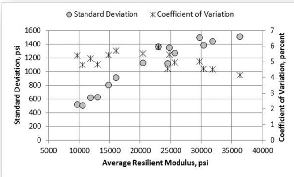
Figure 125. GAB Material, Laboratory B, Standard Deviation and Coefficient of Variation
