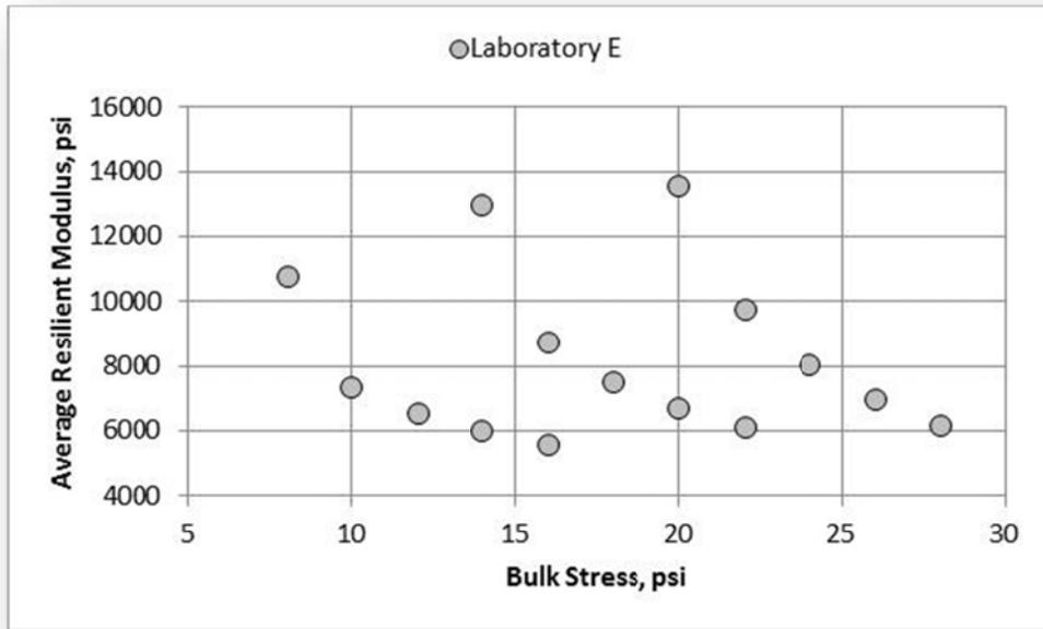
Figure 80. A-7-6 Soil, Laboratory E, Resilient Modulus
