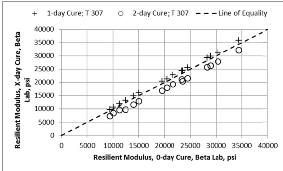
**Figure 19. Effect of Curing Time on Resilient Modulus (Equivalent Stress States) for the GAB Material, Beta Laboratory**
