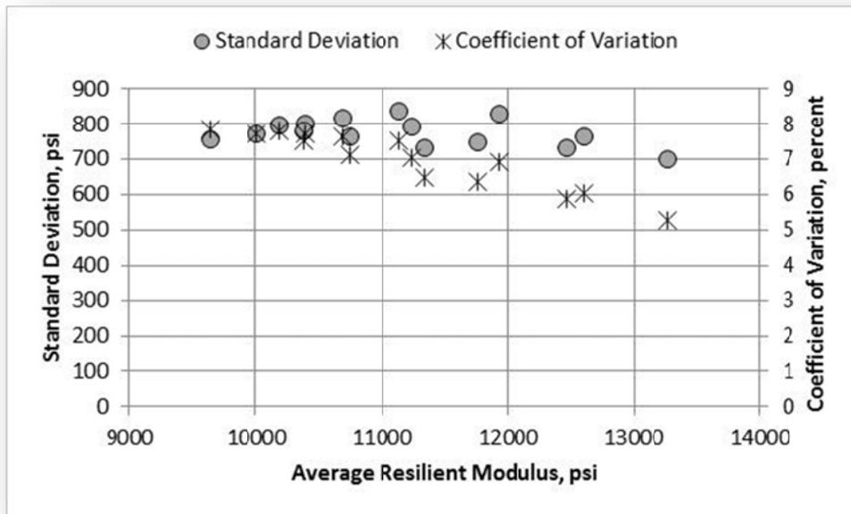
**Figure 85. A-7-6 Soil, Laboratory G, 95 percent Compaction, Standard Deviation and Coefficient of Variation**
