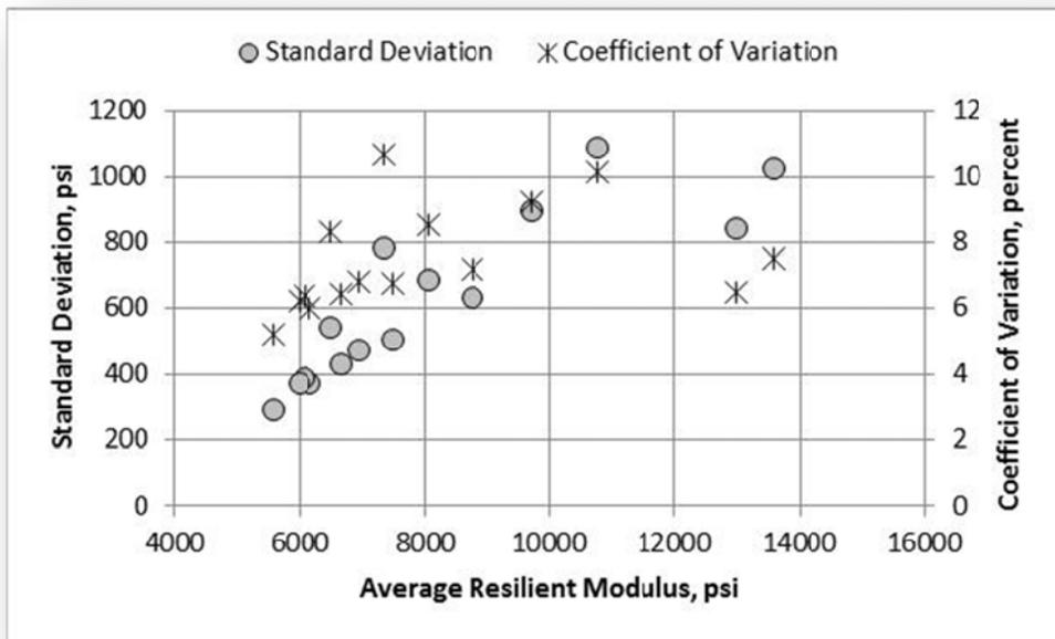
Figure 81. A-7-6 Soil, Laboratory E, Standard Deviation and Coefficient of Variation
