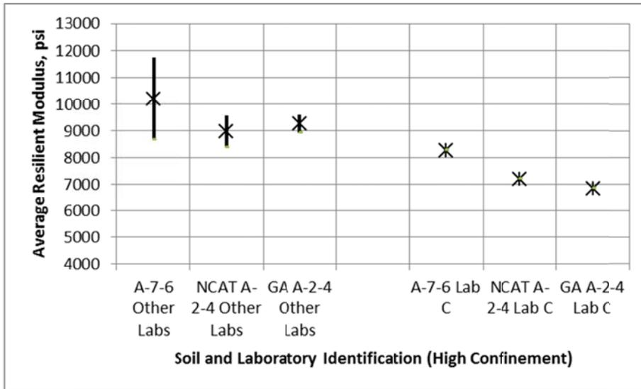
**Figure 55. Average Resilient Modulus Measured at High Confinement (6 psi) and 4 psi Vertical Stress for the Different Embankment Soils**
