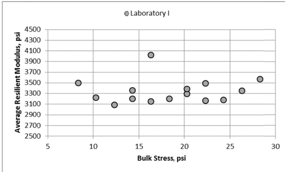
**Figure 50. Resilient Modulus Values Measured by Laboratory I as a Function of Stress State for the Georgia A-2-4 Silty Sand Soil**
