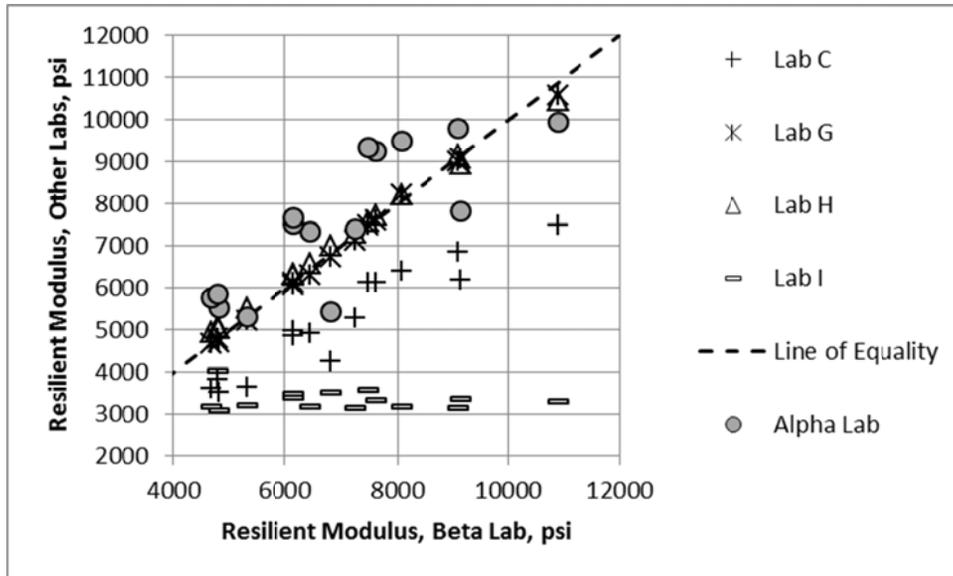
Figure 40. Resilient Moduli Reported from all Laboratories for the Georgia A-2-4 Soil
