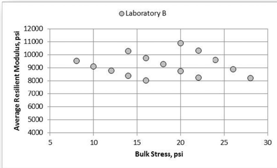
Figure 74. A-7-6 Soil, Laboratory B, Resilient Modulus
