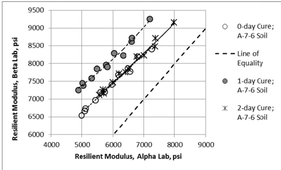
**Figure 24. Comparison of Resilient Modulus Measured by the Alpha and Beta Laboratories in Accordance with AASHTO T 307 for Different Curing Times; A-7-6 Soil**
