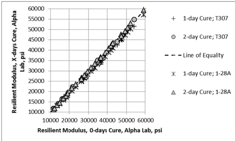
**Figure 18. Effect of Curing Time on Resilient Modulus (Equivalent Stress States) for the GAB Material, Alpha Laboratory**
