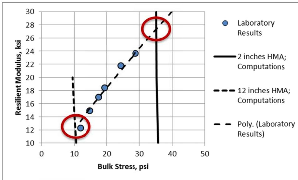
**Figure 68. Graphical Determination of the Design Resilient Modulus for the Crushed Gravel Aggregate Base**
