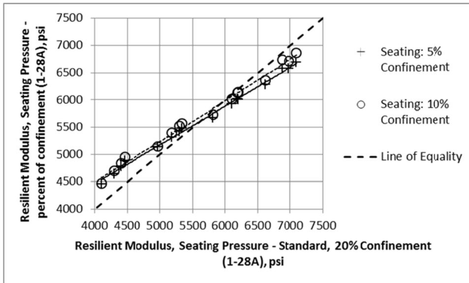
Figure 6. Effect of Seating Load on Resilient Modulus, NCHRP 1-28a
