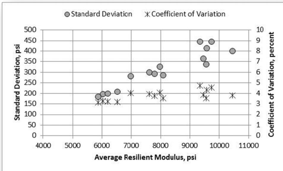
Figure 99. A-2-4 Soil (NCAT Subgrade), Laboratory D, Standard Deviation and Coefficient of Variation
