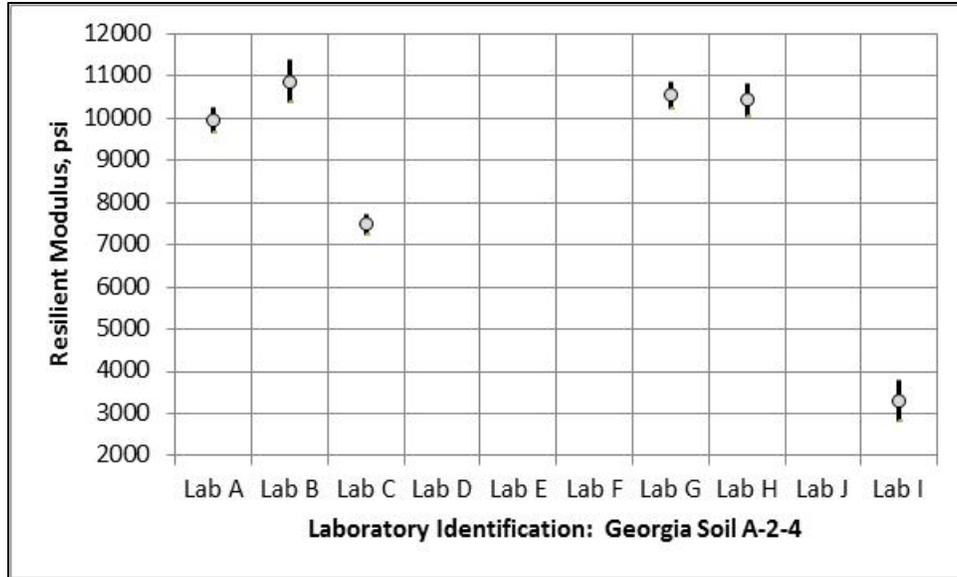
**Figure 46. Difference in Resilient Modulus for the Georgia A-2-4 Soil; All Participating Laboratories**
