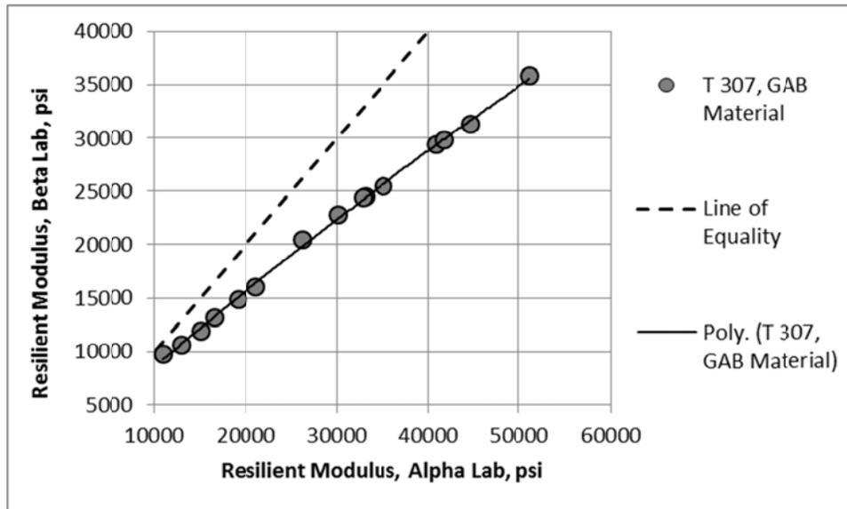
**Figure 37. Comparison of Resilient Modulus between the Alpha and Beta Laboratories; GAB Material**
