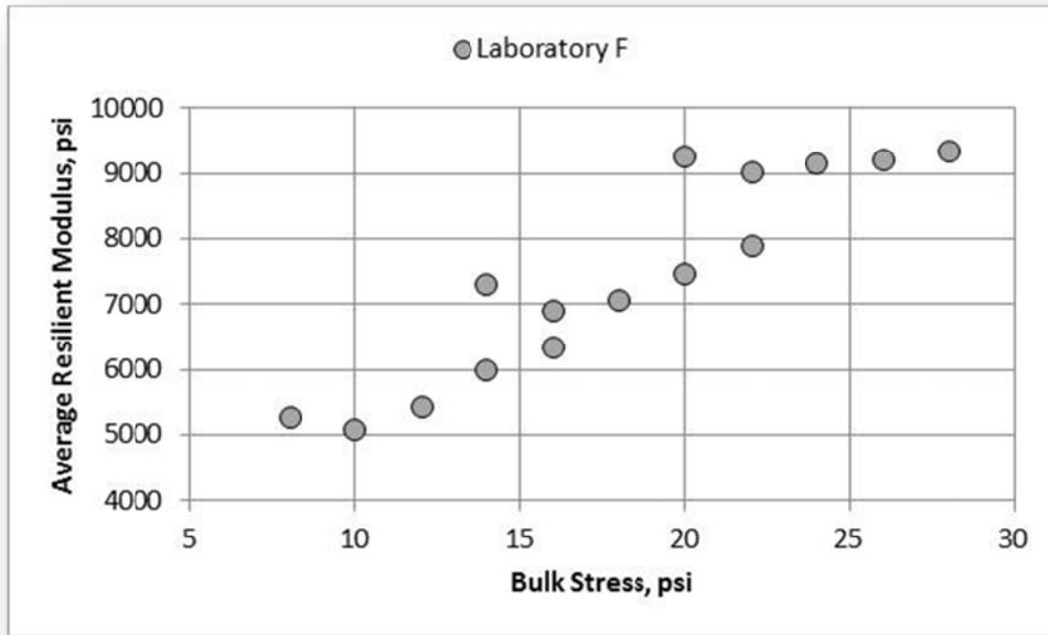
Figure 102. A-2-4 Soil (NCAT Subgrade), Laboratory F, Resilient Modulus
