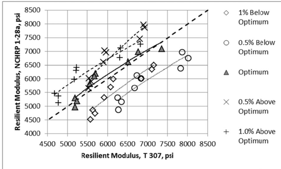
**Figure 35. Comparison of Resilient Modulus for Varying Water Contents: AASHTO T 307 and NCHRP 1-28a**
