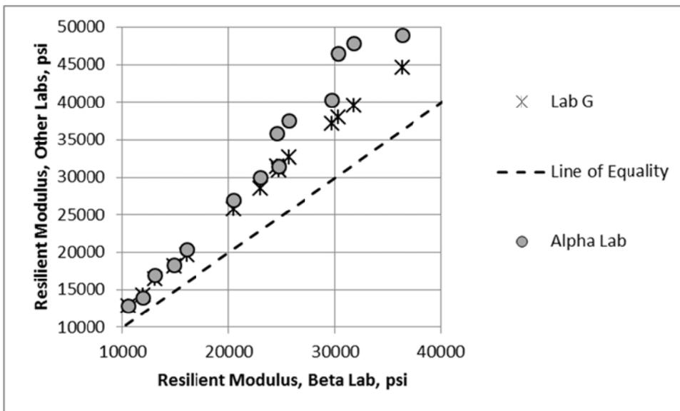
Figure 41. Resilient Moduli Reported from all Laboratories for the GAB Material
