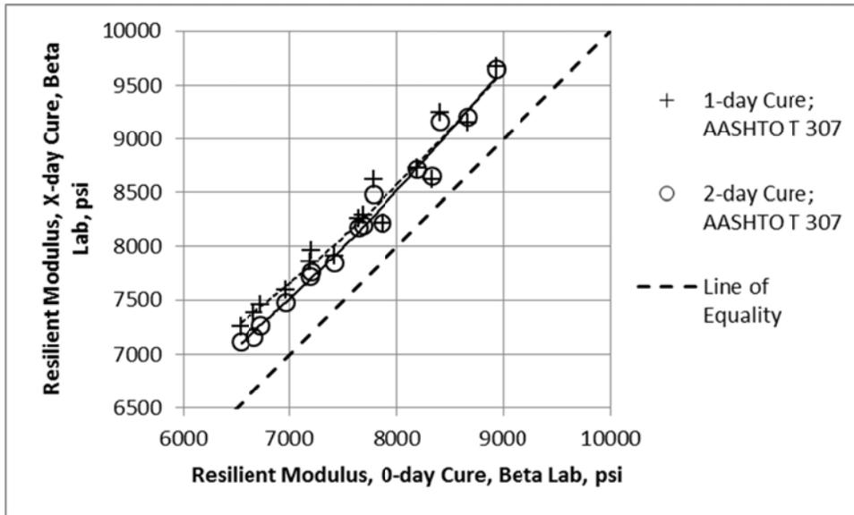
**Figure 17. Effect of Curing Time on Resilient Modulus at Equivalent Stress States for the A-7-6 Soil, Beta Laboratory**
