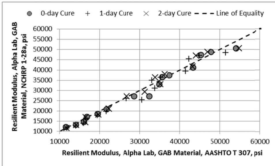
**Figure 23. Comparison of Resilient Modulus Measured by the Alpha Laboratory in Accordance with AASHTO T 307 and NCHRP 1-28a for Different Curing Times, GAB Material**
