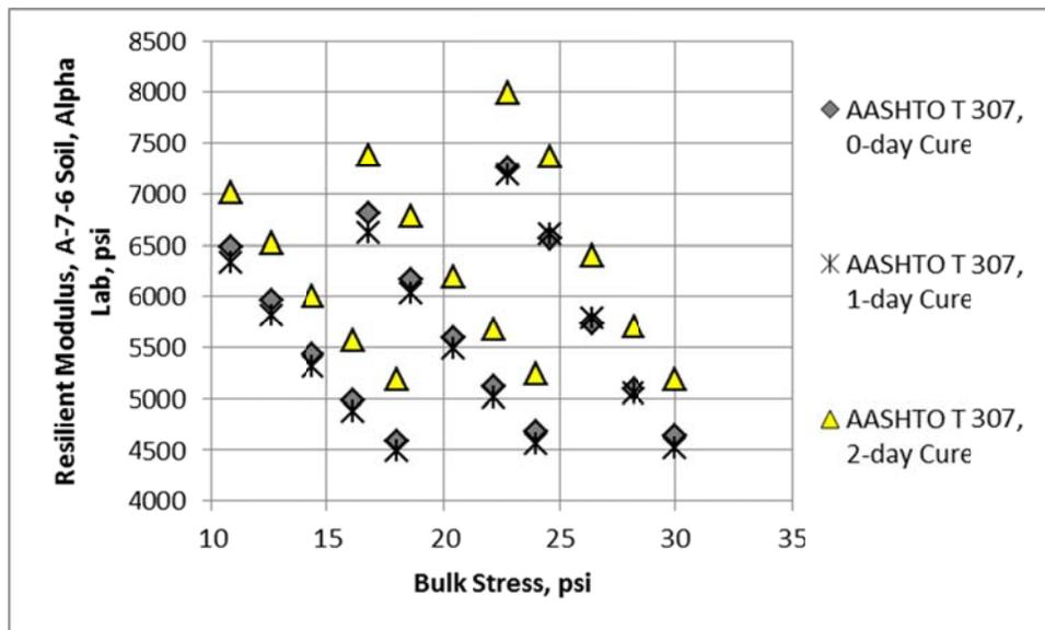
**Figure 12. Resilient Modulus for the A-7-6 Soil Measured by the Alpha Laboratory for different Curing Times, AASHTO T 307**
