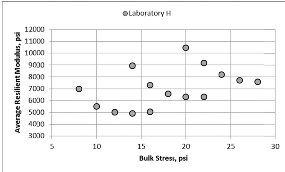
**Figure 52. Resilient Modulus Values Measured by Laboratory H as a Function of Stress State for the Georgia A-2-4 Silty Sand Soil**
