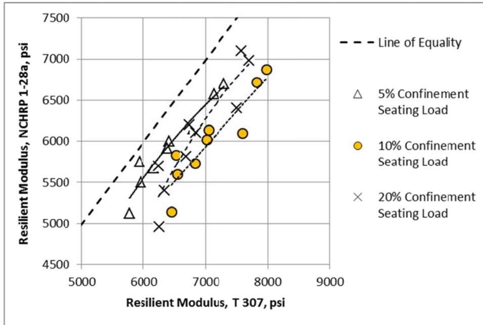
**Figure 11. Comparison of Resilient Modulus between AASHTO T 307 and NCHRP 1-28a for the Same Seating Load**
