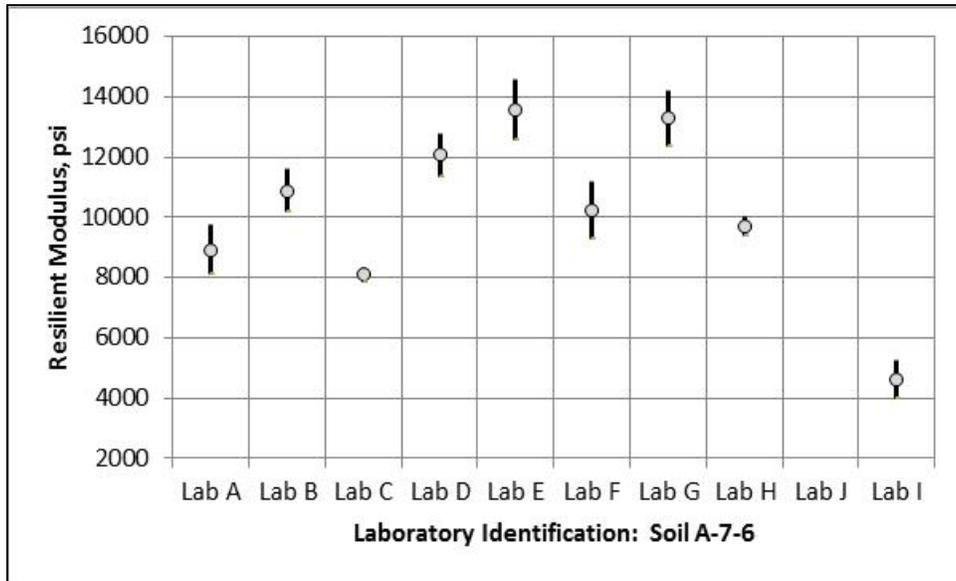
**Figure 42. Difference in Resilient Modulus for the A-7-6 Soil; All Participating Laboratories**
