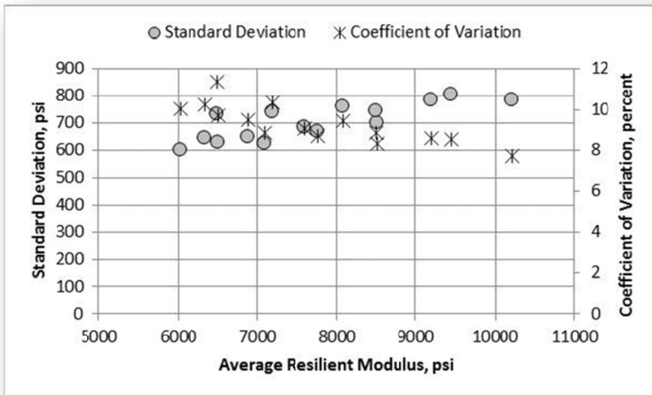
Figure 83. A-7-6 Soil, Laboratory F, Standard Deviation and Coefficient of Variation
