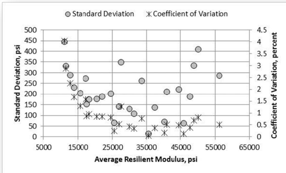
Figure 123. GAB Material, Laboratory A, Standard Deviation and Coefficient of Variation
