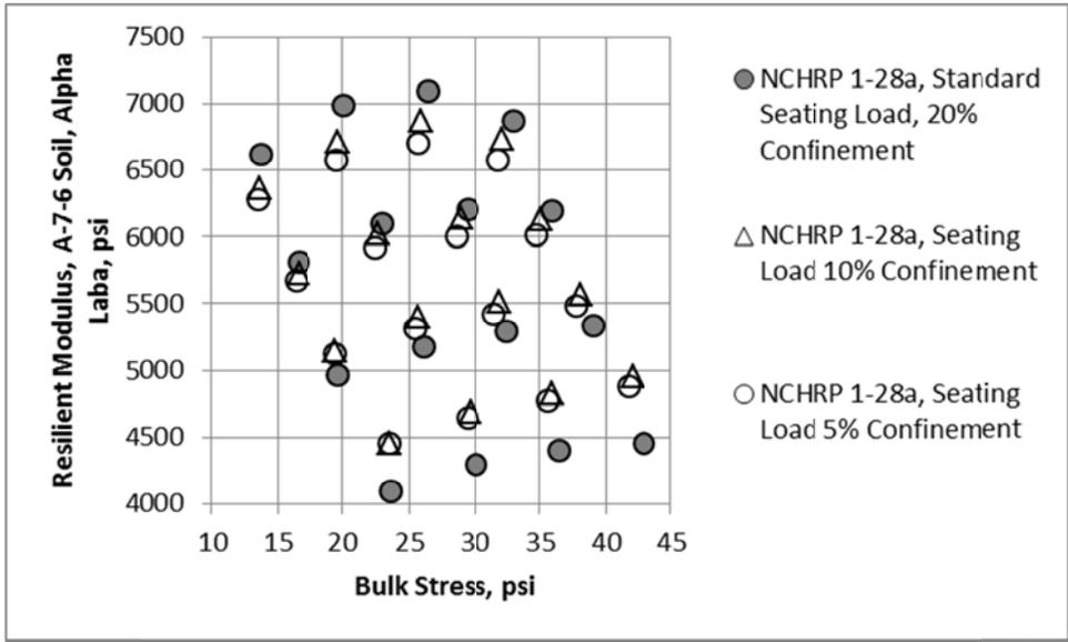
**Figure 2. Resilient Modulus for the A-7-6 Soil Measured by the Alpha Laboratory for different Seating Loads, NCHRP 1-28a**
