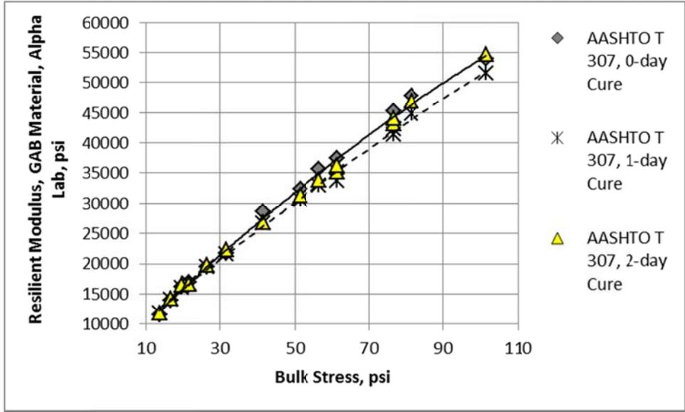
Figure 14. Resilient Modulus for the GAB Material Measured by the Alpha Laboratory for different Curing Times, AASHTO T 307
