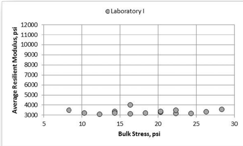
Figure 120. A-2-4 Soil (Low Plasticity), Laboratory I, Resilient Modulus
