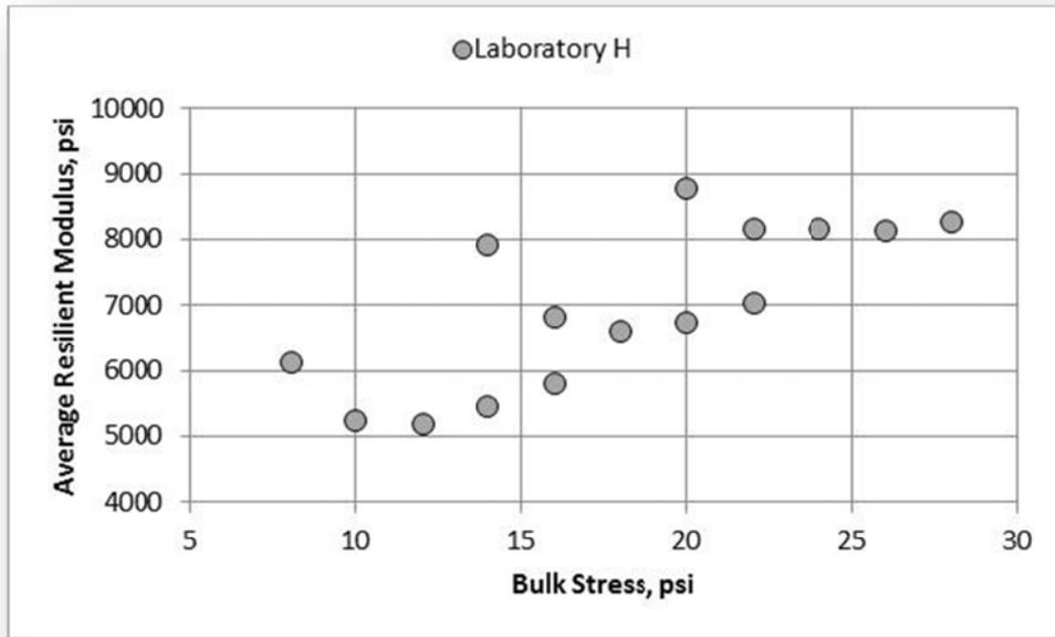
Figure 106. A-2-4 Soil (NCAT Subgrade), Laboratory H, Resilient Modulus
