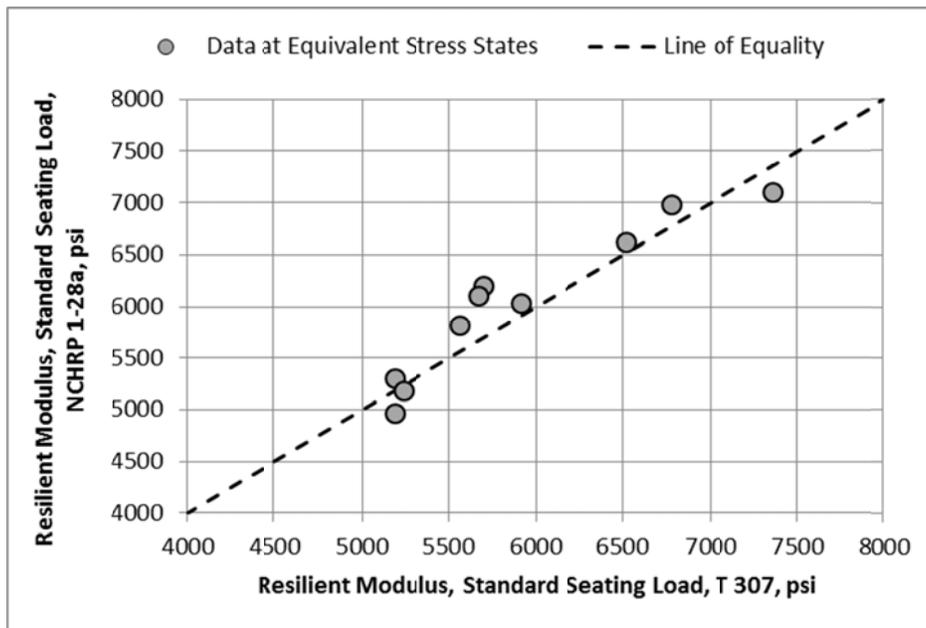
**Figure 10. Comparison of Resilient Modulus at Equivalent Stress States between AASHTO T 307 and NCHRP 1-28a Using the Standard Seating Loads Designated by each Procedure**
