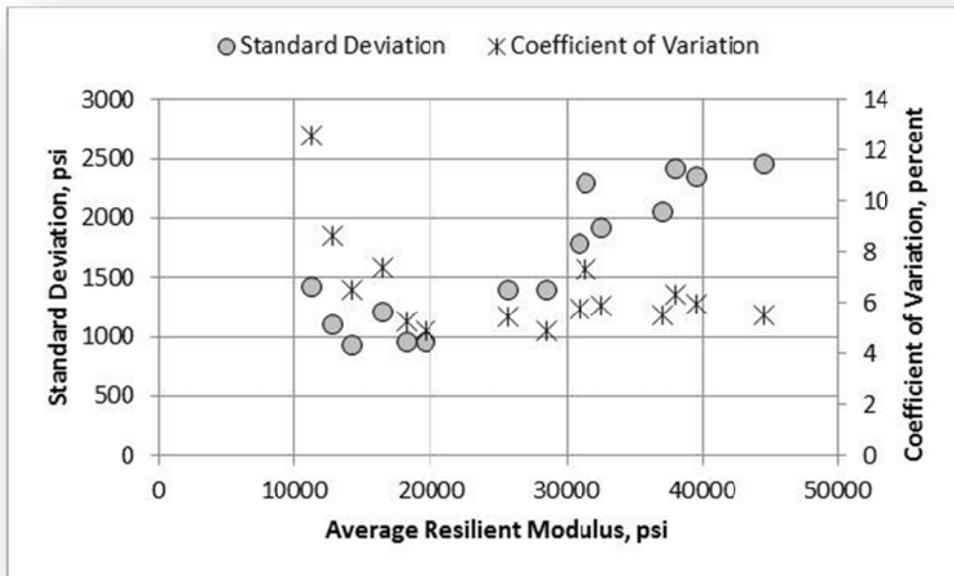
Figure 127. GAB Material, Laboratory G, Standard Deviation and Coefficient of Variation
