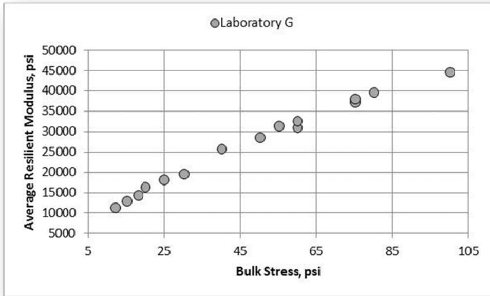
Figure 126. GAB Material, Laboratory G, Resilient Modulus
