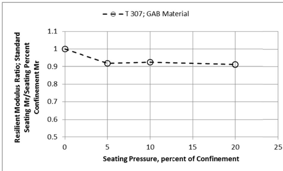
Figure 8. Effect of Seating Load on the Resilient Modulus Ratio, GAB Material (for AASHTO T 307, “0” is the standard seating load)
