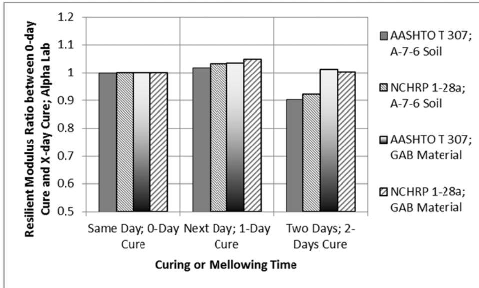
**Figure 20. Effect of Curing Time on Average Resilient Modulus Ratio (Equivalent Stress States) for the A-7-6 Soil and GAB Material, Alpha Laboratory**
