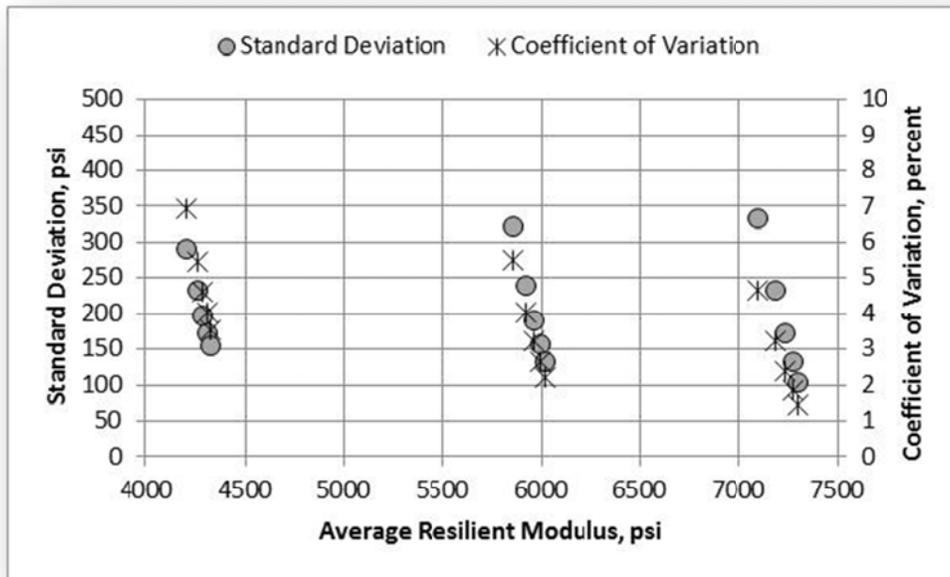
Figure 97. A-2-4 Soil (NCAT Subgrade), Laboratory C, Standard Deviation and Coefficient of Variation
