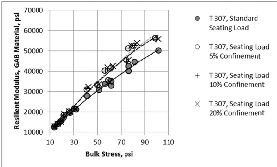
Figure 3. Resilient Modulus for the GAB Material Measured by the Alpha Laboratory for different Seating Loads, AASHTO T 307
