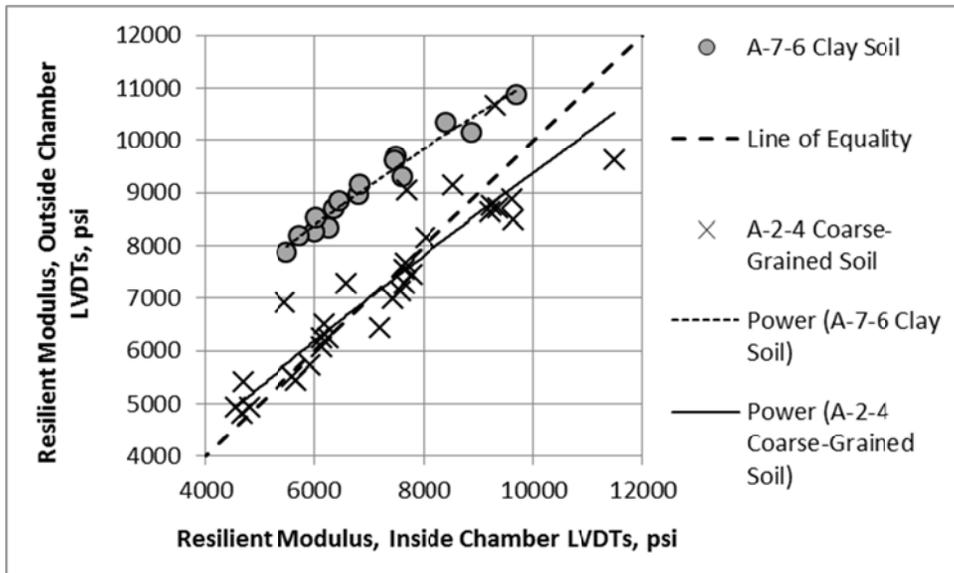
Figure 58. Comparison of Resilient Modulus Measured with different Locations of the LVDTs between All Participating Laboratories
