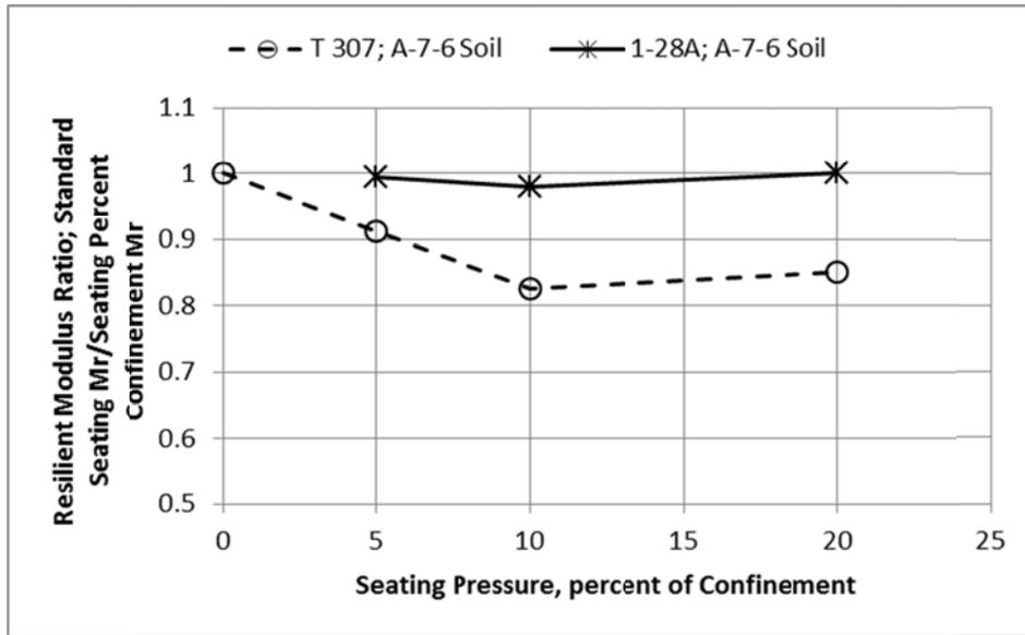
Figure 7. Effect of Seating Load on the Resilient Modulus Ratio; A-7-6 Soil (for AASHTO T 307, “0” is the standard seating load)
