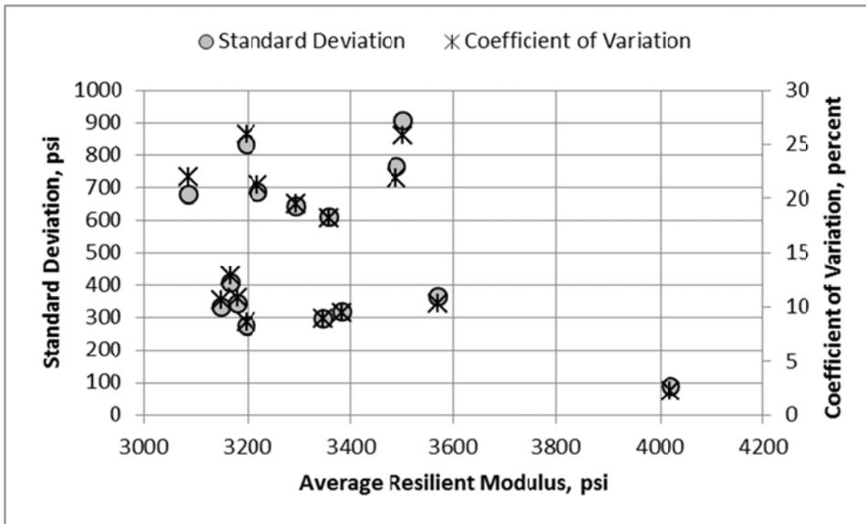
**Figure 51. Variation of Resilient Modulus Values for Different Stress States as Measured by Laboratory I for the Georgia A-2-4 Silty Sand Soil**
