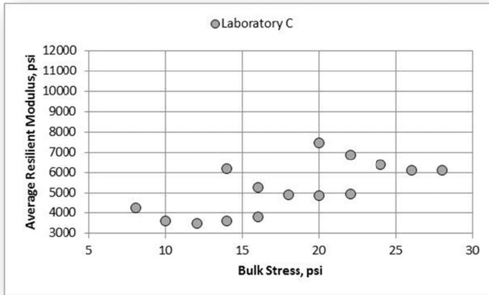
Figure 114. A-2-4 Soil (Low Plasticity), Laboratory C, Resilient Modulus
