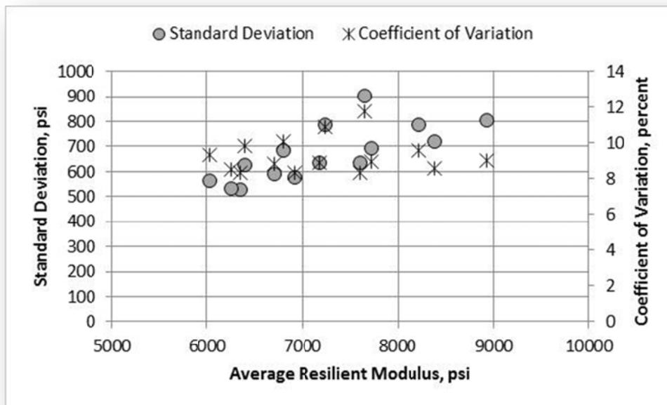
Figure 73. A-7-6 Soil, Laboratory A, Standard Deviation and Coefficient of Variation
