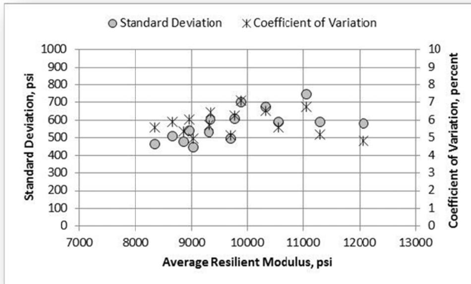
Figure 79. A-7-6 Soil, Laboratory D, Standard Deviation and Coefficient of Variation
