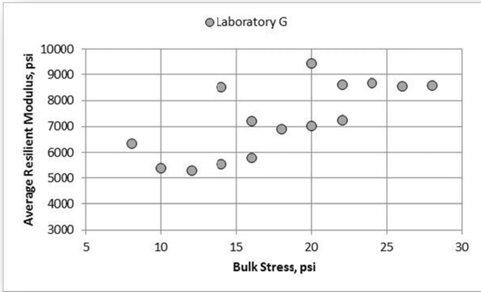
Figure 104. A-2-4 Soil (NCAT Subgrade), Laboratory G, Resilient Modulus
