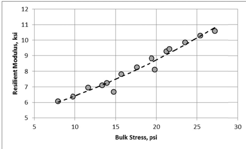
**Figure 61. A-7-5 Fine-Grained Clay Soil; Repeated Load Resilient Modulus Tests
