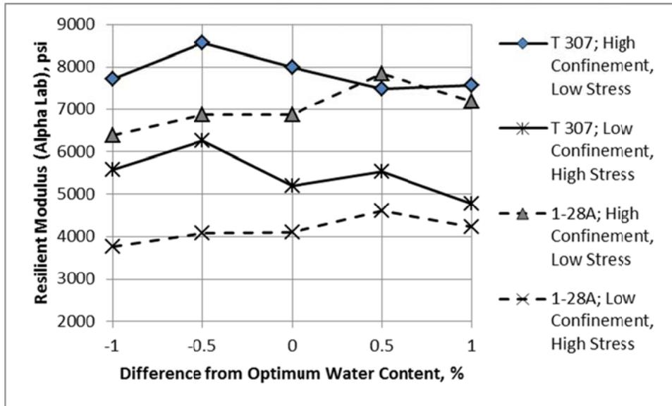
**Figure 31. Effect of Water Content on Resilient Modulus at Equivalent Stress States; Alpha Laboratory**
