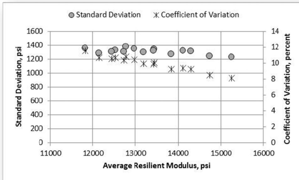
Figure 87. A-7-6 Soil, Laboratory G, 100 percent Compaction, Standard Deviation and Coefficient of Variation
