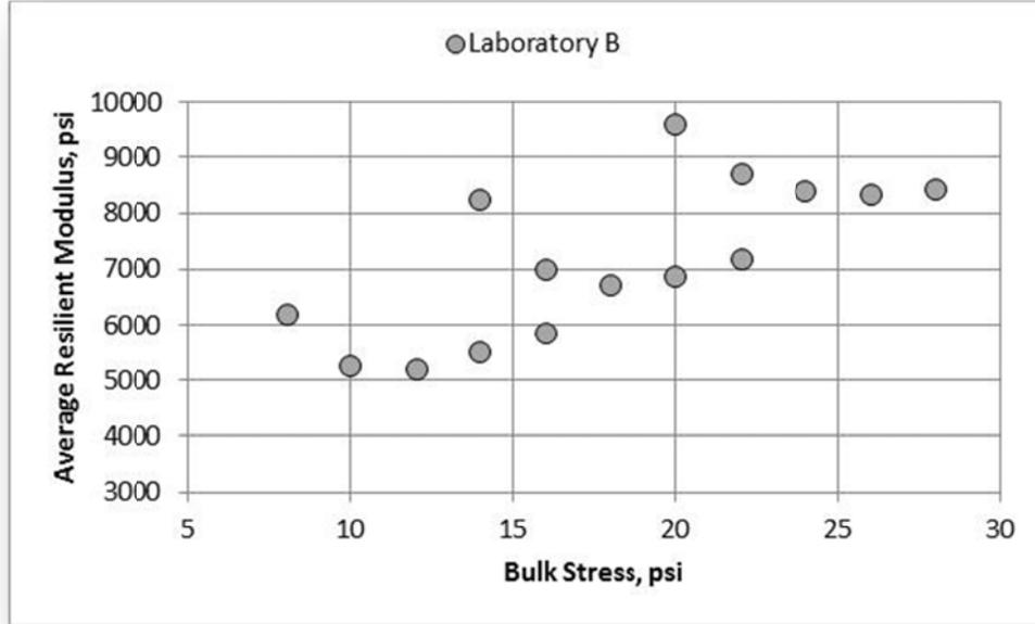
Figure 94. A-2-4 Soil (NCAT Subgrade), Laboratory B, Resilient Modulus
