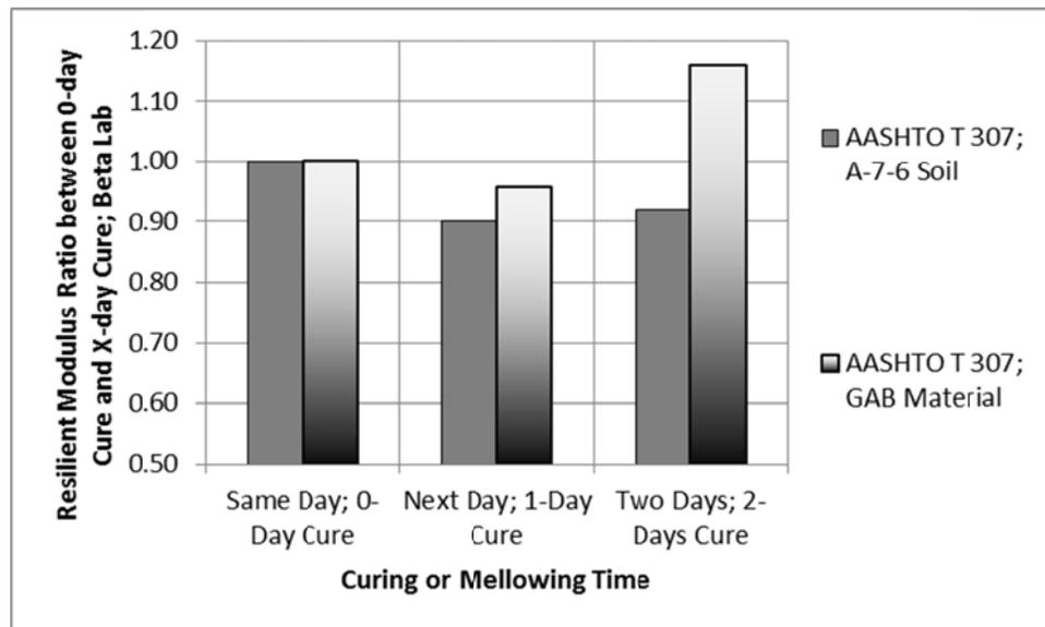
**Figure 21. Effect of Curing Time on Average Resilient Modulus Ratio (Equivalent Stress States) for the A-7-6 Soil and GAB Material, Beta Laboratory**
