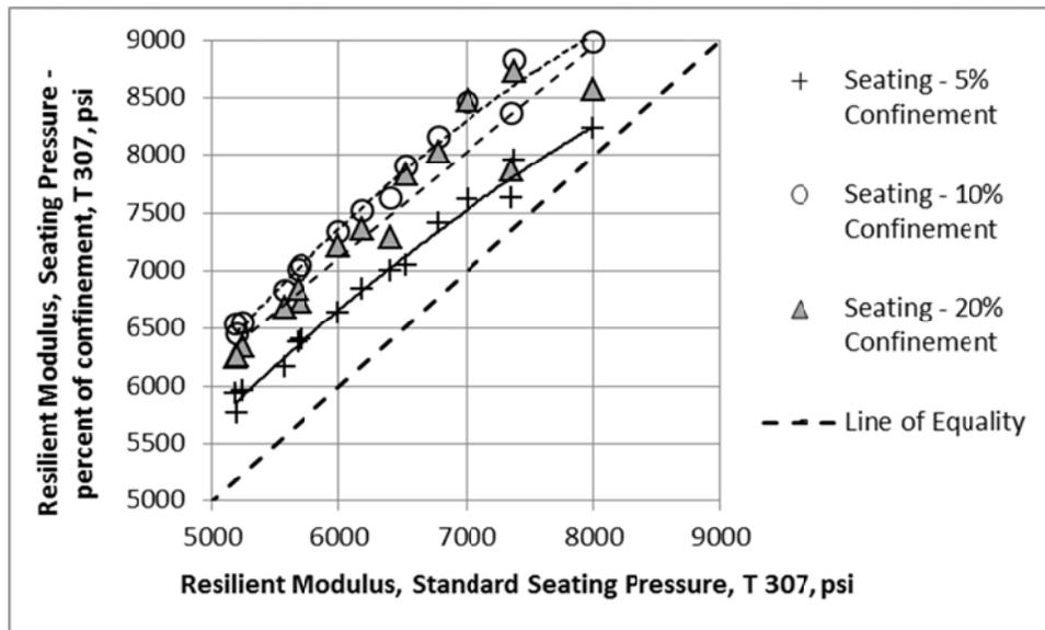
Figure 4. Effect of Seating Load on Resilient Modulus for the A-7-6 Soil, AASHTO T 307
