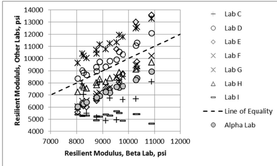
**Figure 38. Resilient Moduli Reported from all Laboratories for the A-7-6 Soil**
