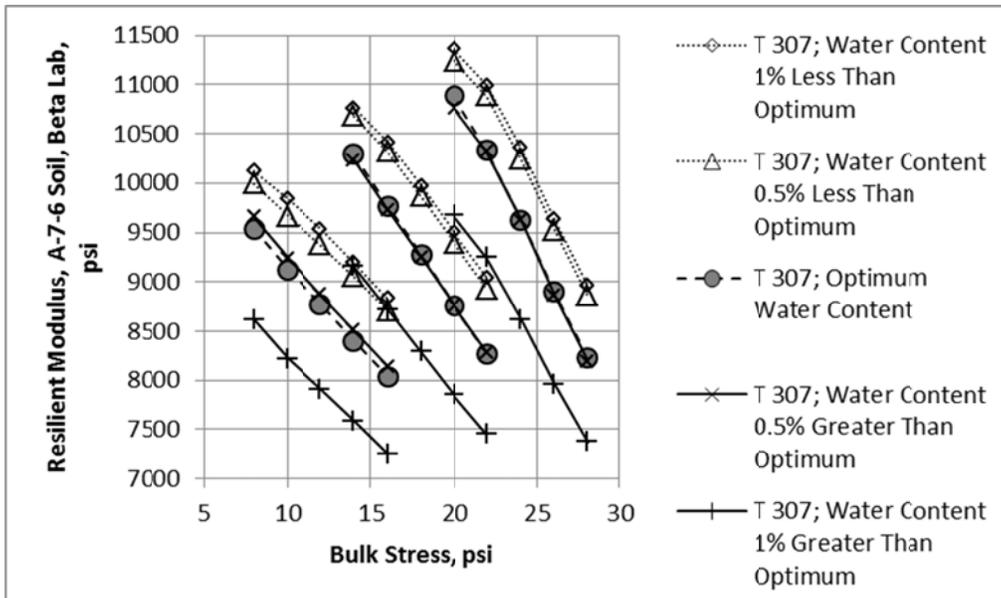
Figure 27. Resilient Modulus Measured on the A-7-6 Soil for Different Water Contents; Beta Laboratory
