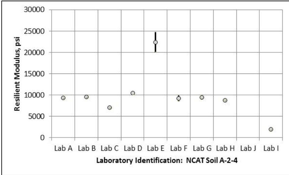
**Figure 44. Difference in Resilient Modulus for the NCAT A-2-4 Soil; All Participating Laboratories**
