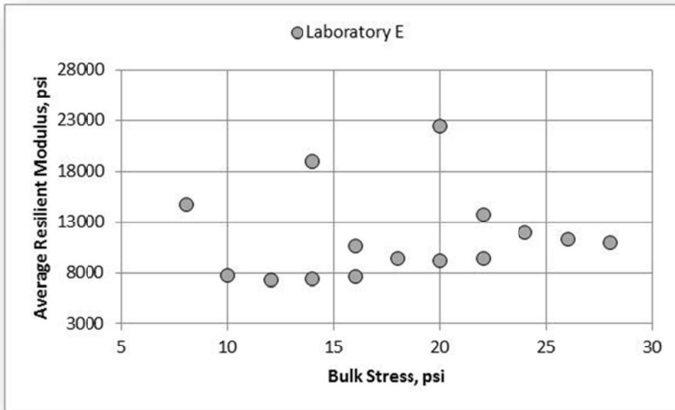
Figure 100. A-2-4 Soil (NCAT Subgrade), Laboratory E, Resilient Modulus
