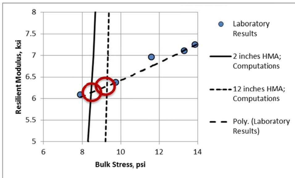
**Figure 66. Graphical Determination of the Design Resilient Modulus for the A-7-5 Fine-Grained Clay Soil**
