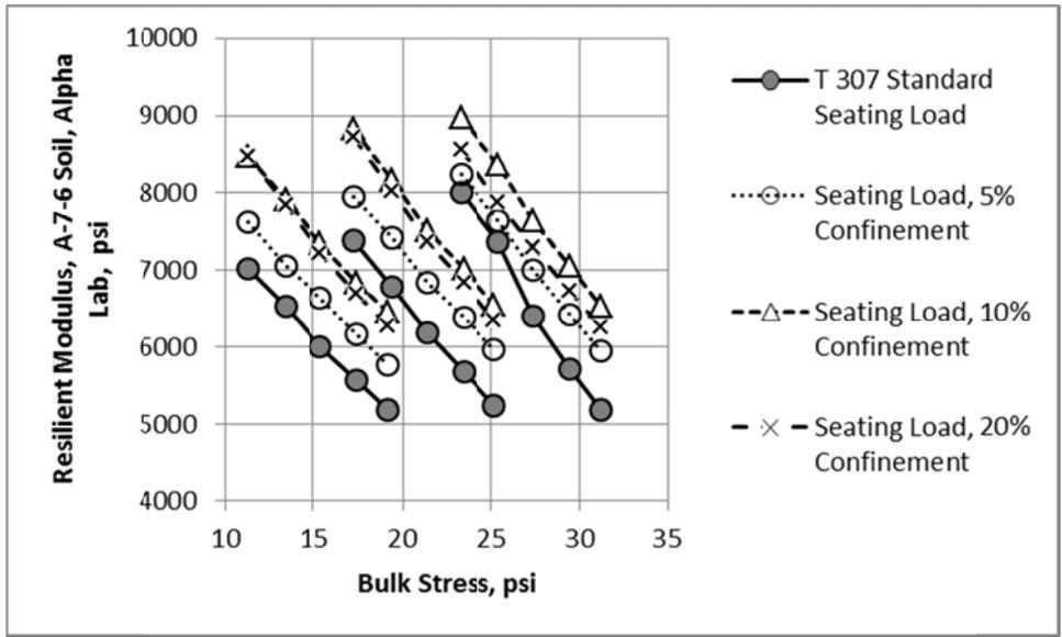
**Figure 1. Resilient Modulus for the A-7-6 Soil Measured by the Alpha Laboratory for different Seating Loads, AASHTO T 307**
