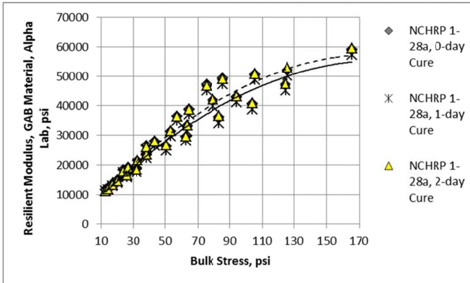
Figure 15. Resilient Modulus for the GAB Material Measured by the Alpha Laboratory for different Curing Times, NCHRP 1-28a
