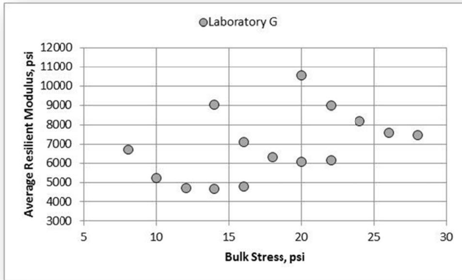
Figure 116. A-2-4 Soil (Low Plasticity), Laboratory G, Resilient Modulus
