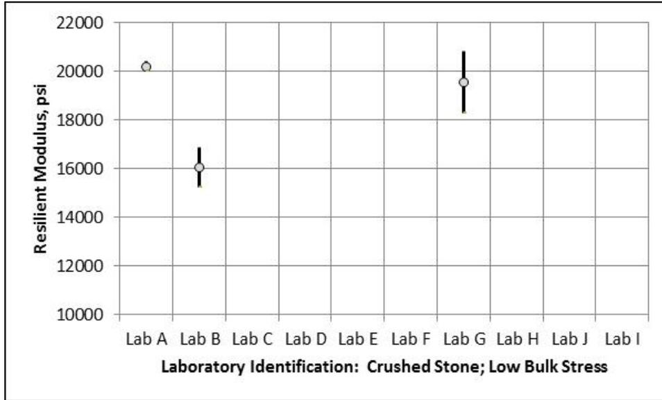
**Figure 48. Difference in Resilient Modulus for the Crushed Stone Base Material; All Participating Laboratories, Low Bulk Stress Level**
