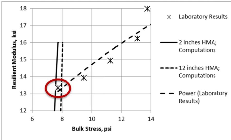
**Figure 67. Graphical Determination of the Design Resilient Modulus for the A-1-b Coarse-Grained Sandy Soil**
