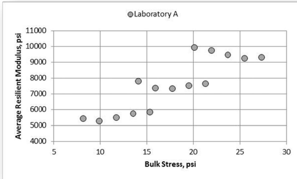
Figure 110. A-2-4 Soil (Low Plasticity), Laboratory A, Resilient Modulus
