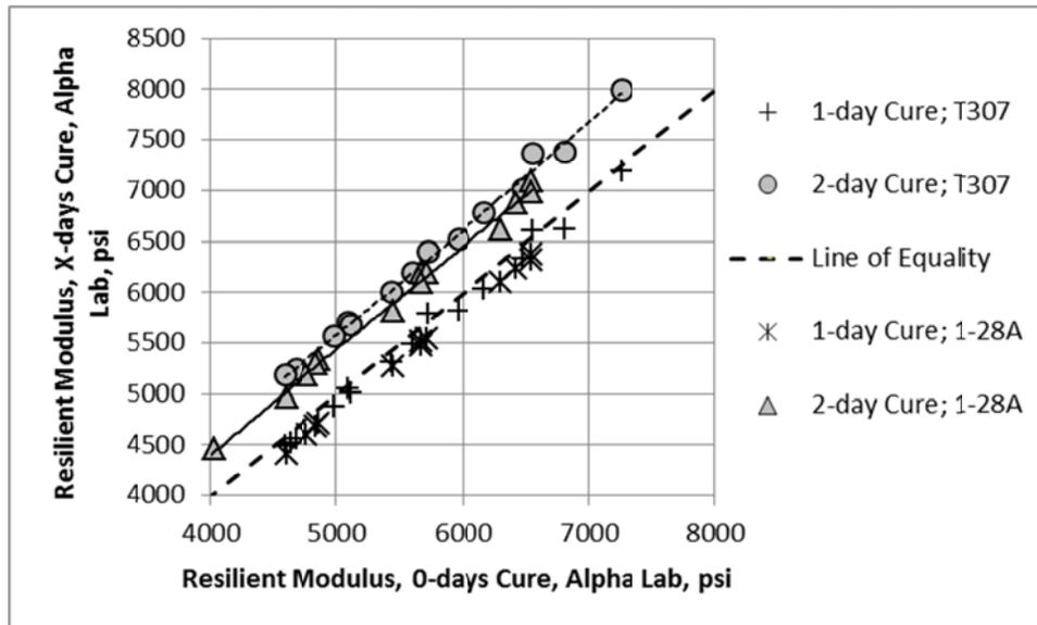
Figure 16. Effect of Curing Time on Resilient Modulus at Equivalent Stress States for the A-7-6 Soil, Alpha Laboratory
