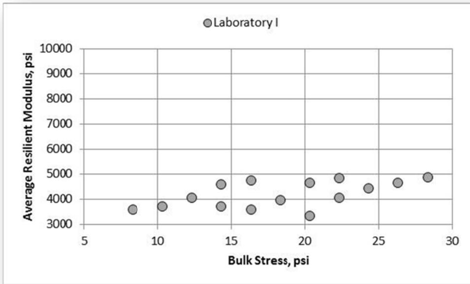
Figure 108. A-2-4 Soil (NCAT Subgrade), Laboratory I, Resilient Modulus
