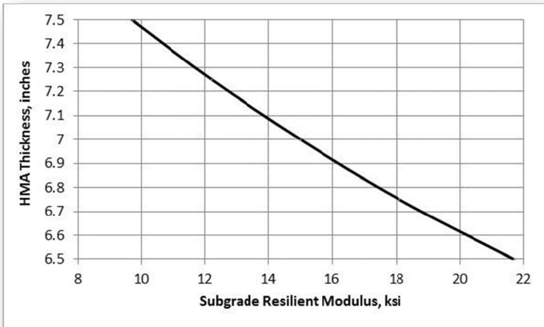
**Figure 71. Graphical Determination of the Maximum Change in Resilient Modulus of the A-1-b Soil Requiring Less Than 0.5 inches Change in HMA Thickness**
