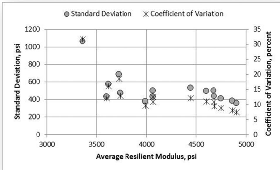
Figure 109. A-2-4 Soil (NCAT Subgrade), Laboratory I, Standard Deviation and Coefficient of Variation
