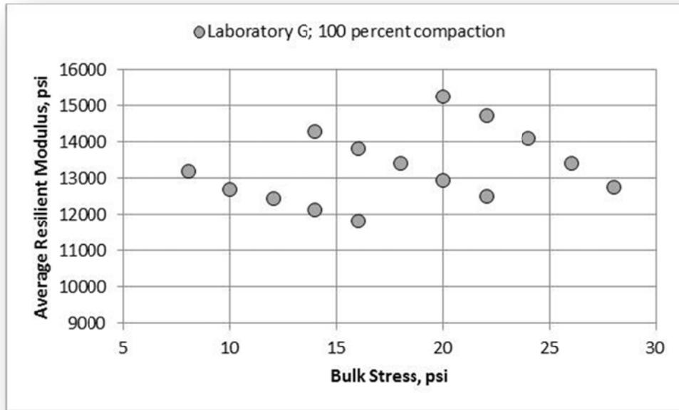
Figure 86. A-7-6 Soil, Laboratory G, 100 percent Compaction, Resilient Modulus
