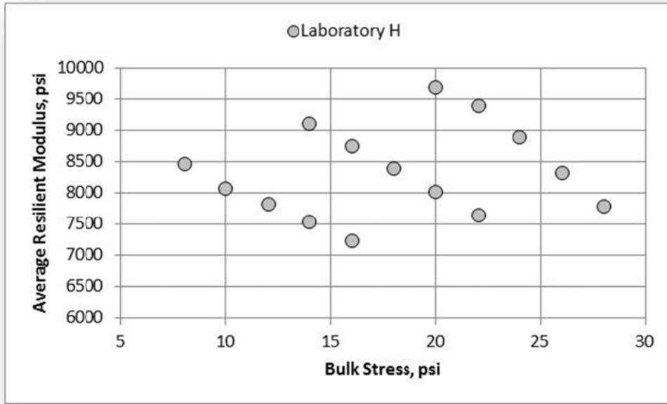
Figure 88. A-7-6 Soil, Laboratory H, Resilient Modulus
