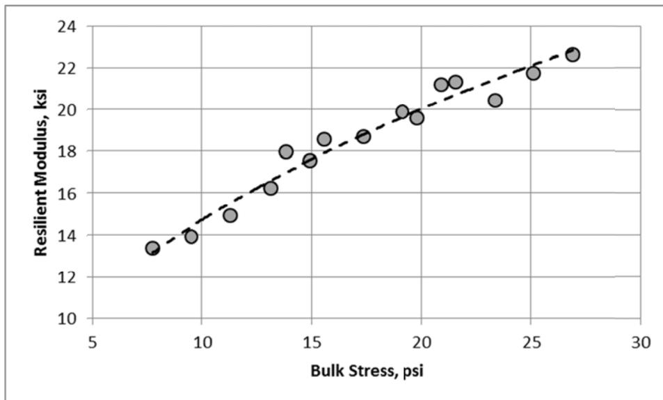
**Figure 62. A-1-b Coarse-Grained Sandy Soil; Repeated Load Resilient Modulus Tests
