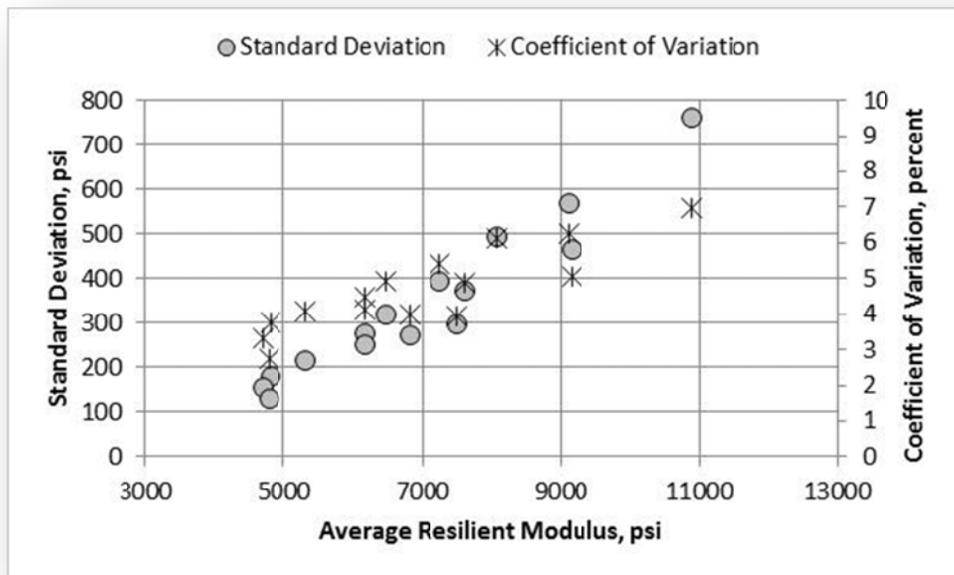
Figure 113. A-2-4 Soil (Low Plasticity), Laboratory B, Standard Deviation and Coefficient of Variation
