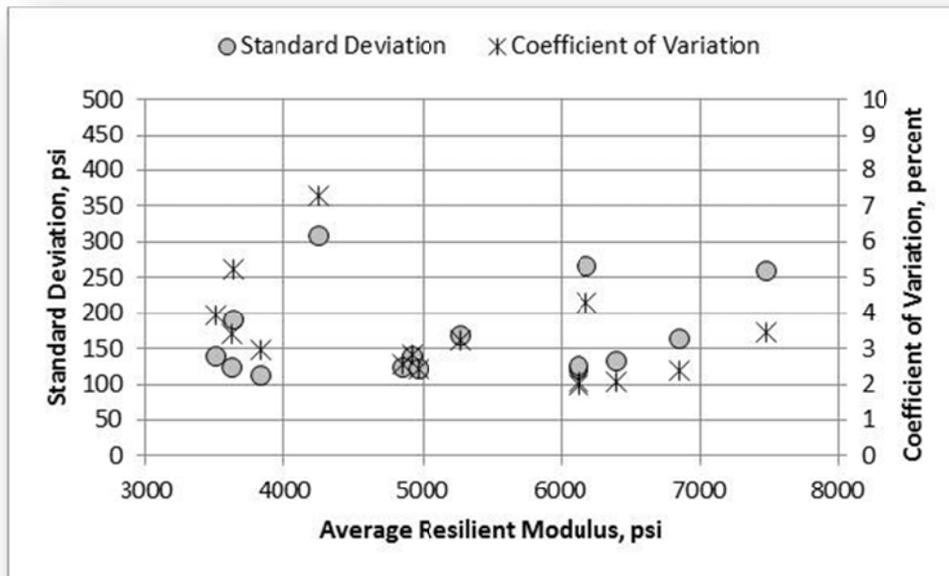
Figure 115. A-2-4 Soil (Low Plasticity), Laboratory C, Standard Deviation and Coefficient of Variation
