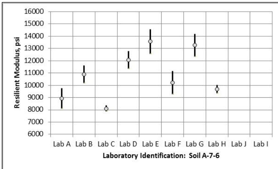
**Figure 43. Difference in Resilient Modulus for the A-7-6 Soil; Excludes Laboratory I**
