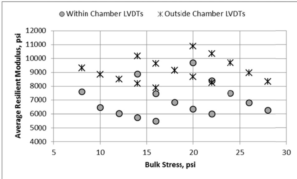
Figure 57. Comparison of Resilient Modulus Measured with different Locations of the LVDTs between Two Laboratories
