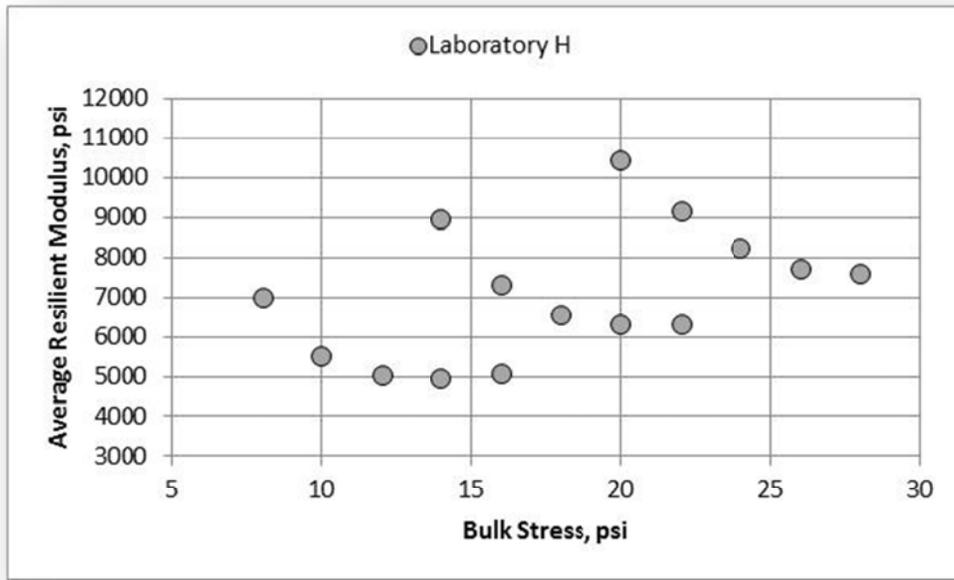
Figure 118. A-2-4 Soil (Low Plasticity), Laboratory H, Resilient Modulus
