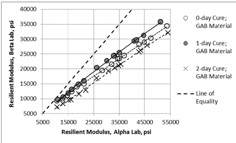
**Figure 25. Comparison of Resilient Modulus Measured by the Alpha and Beta Laboratories in Accordance with AASHTO T 307 for Different Curing Times; GAB Material**
