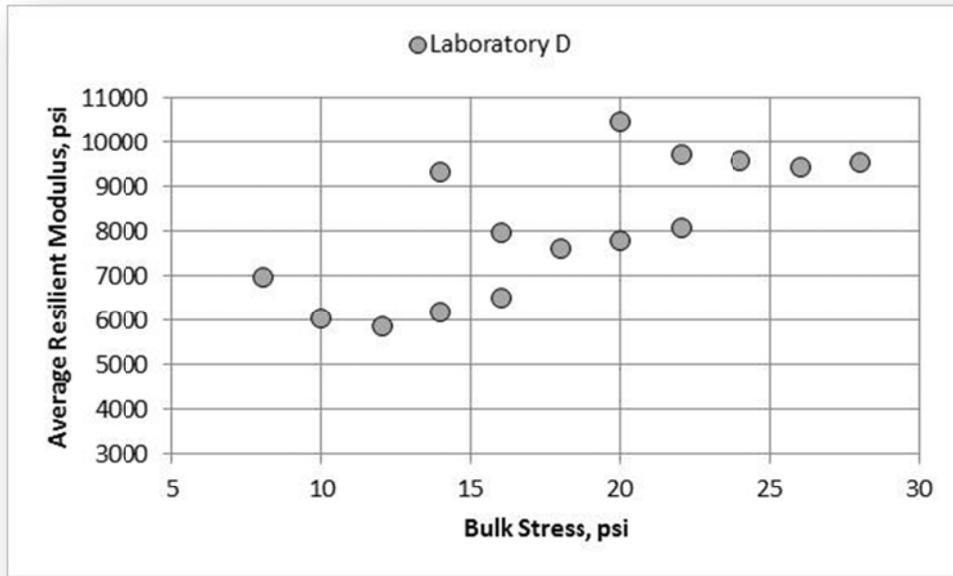
Figure 98. A-2-4 Soil (NCAT Subgrade), Laboratory D, Resilient Modulus
