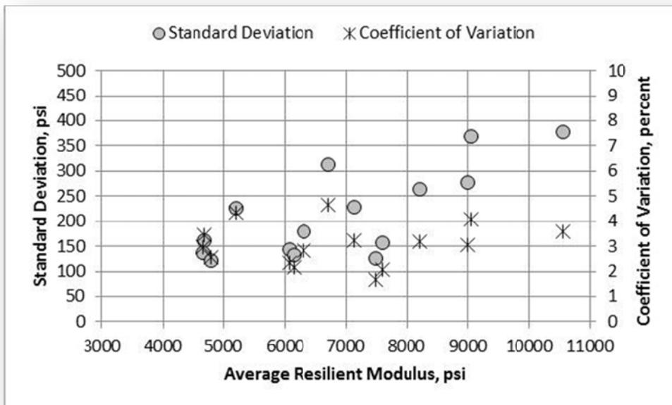
Figure 117. A-2-4 Soil (Low Plasticity), Laboratory G, Standard Deviation and Coefficient of Variation
