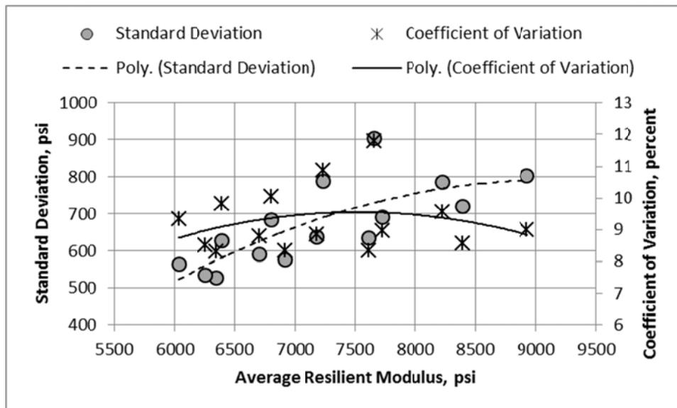
**Figure 60. Single Operator Standard Deviation and Coefficient of Variation over a Range of Resilient Moduli; Laboratory A, A-7-6 Soil**
