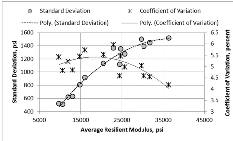
**Figure 59. Single Operator Standard Deviation and Coefficient of Variation over a Range of Resilient Moduli; Laboratory B, GAB Material**
