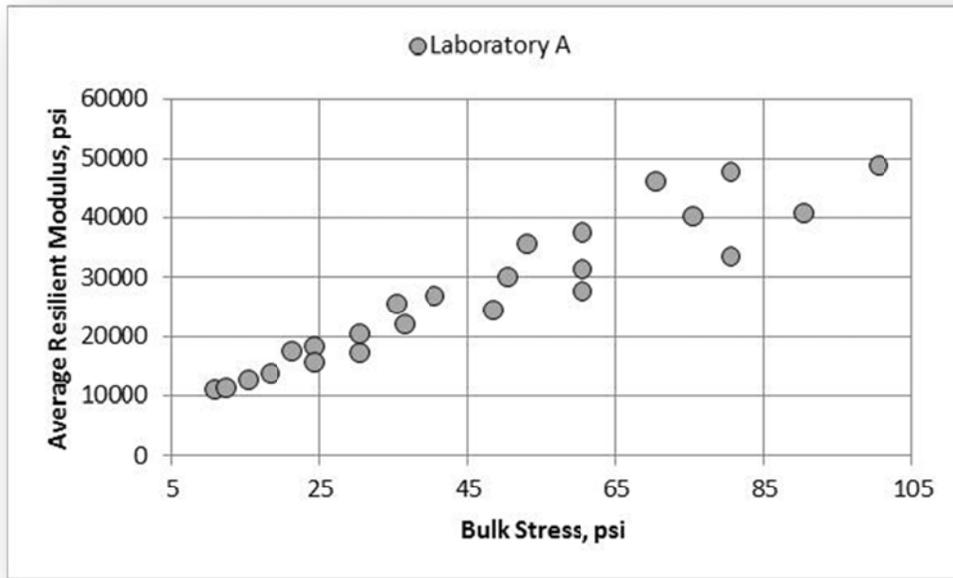
Figure 122. GAB Material, Laboratory A, Resilient Modulus
