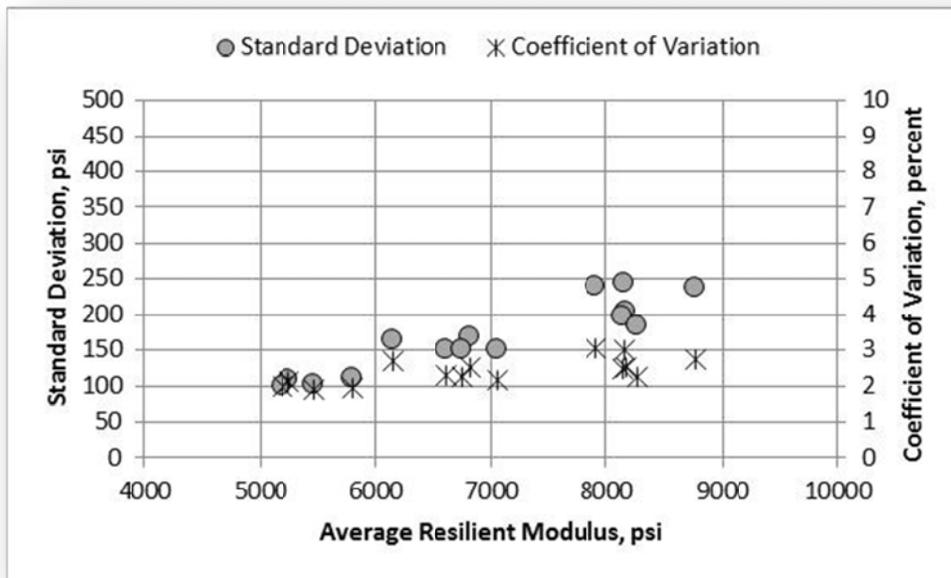
Figure 107. A-2-4 Soil (NCAT Subgrade), Laboratory H, Standard Deviation and Coefficient of Variation
