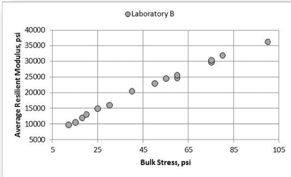
Figure 124. GAB Material, Laboratory B, Resilient Modulus
