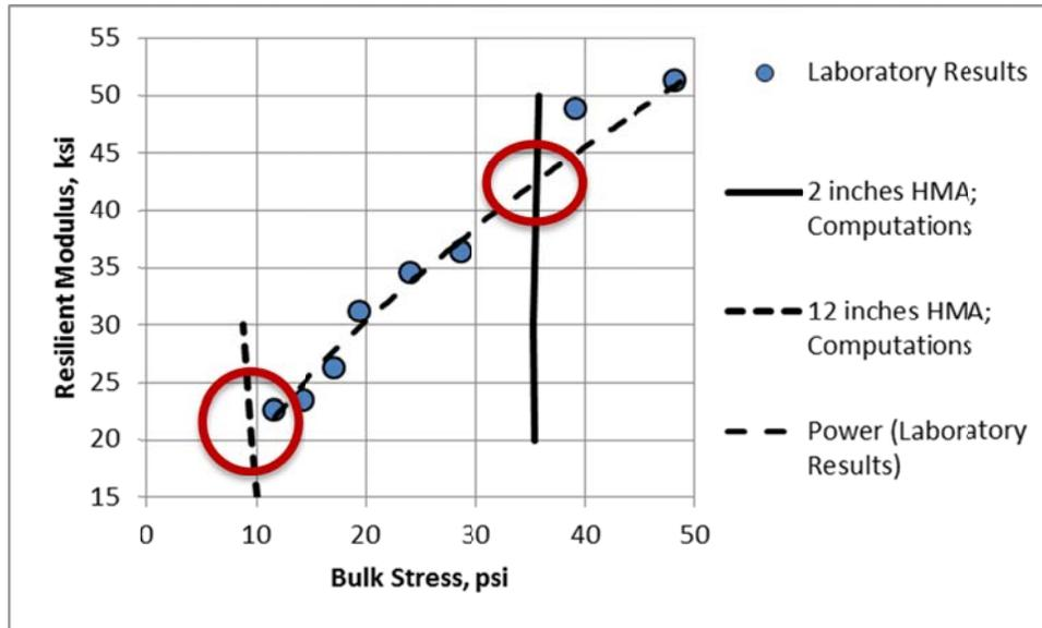
**Figure 69. Graphical Determination of the Design Resilient Modulus for the Crushed Stone Aggregate Base**
