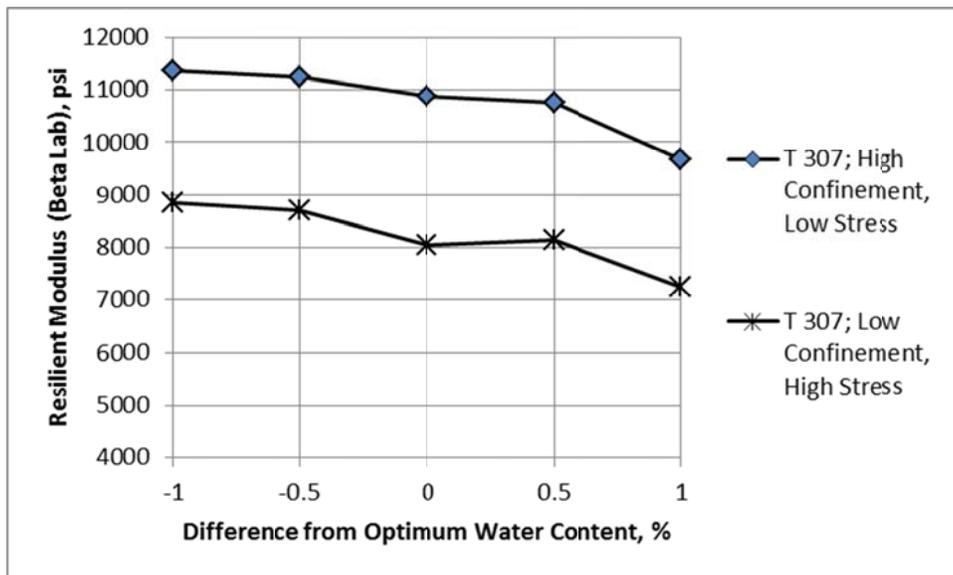
**Figure 32. Effect of Water Content on Resilient Modulus at Equivalent Stress States; Beta Laboratory**
