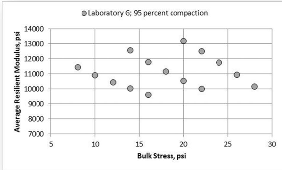
**Figure 84. A-7-6 Soil, Laboratory G, 95 percent Compaction, Resilient Modulus**
