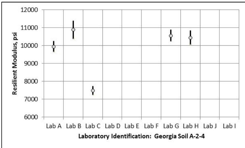
**Figure 47. Difference in Resilient Modulus for the Georgia A-2-4 Soil; Excludes Laboratory I**
