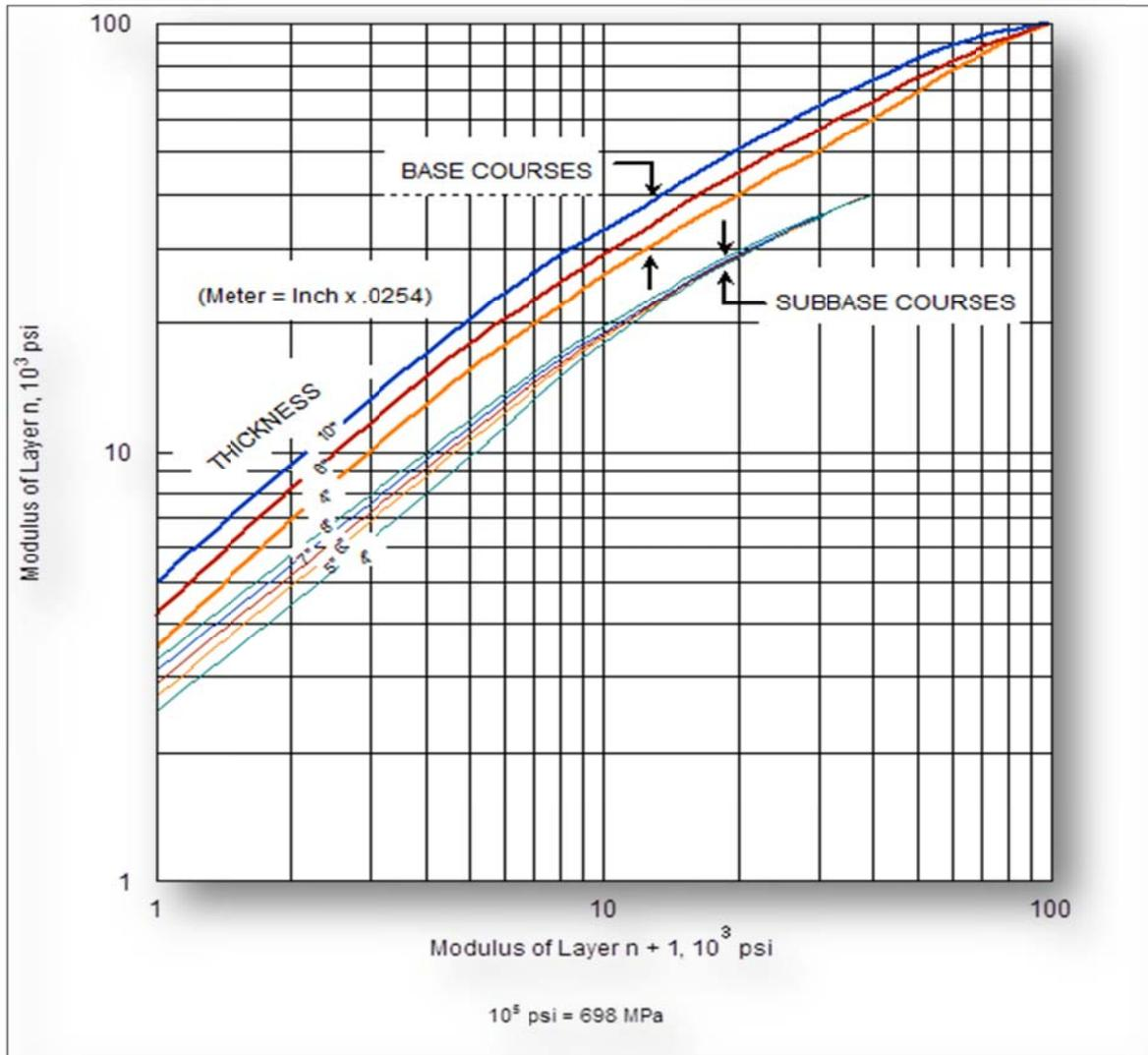
**Figure 70. Limiting Modulus Criteria of Unbound Aggregate Base and Subbase Layers (Baker and Brabston, 1975)**
