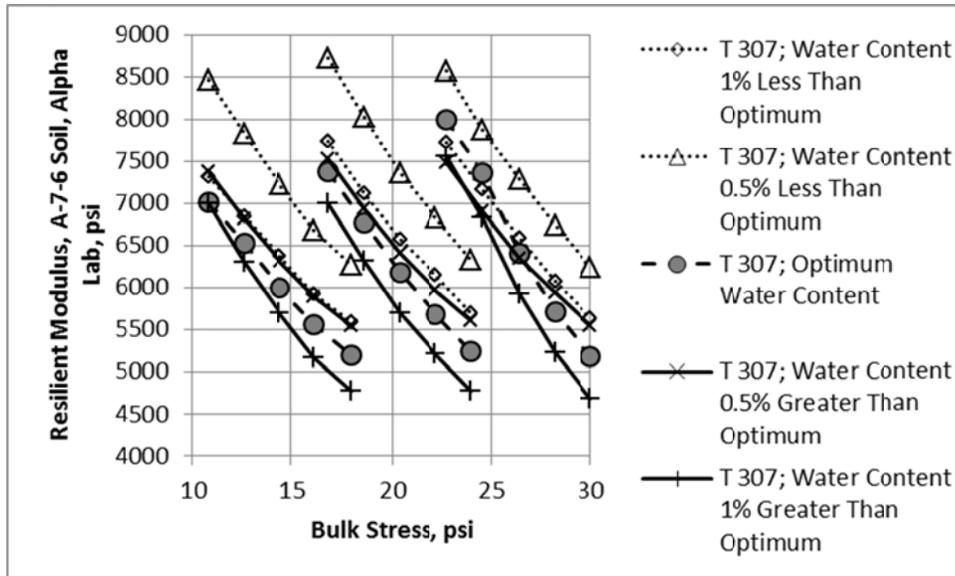
Figure 26. Resilient Modulus Measured on the A-7-6 Soil for Different Water Contents; Alpha Laboratory
