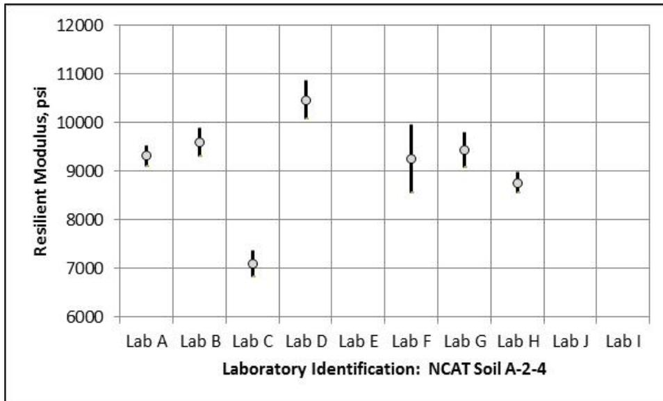
**Figure 45. Difference in Resilient Modulus for the NCAT A-2-4 Soil; Excludes Laboratories E and I**
