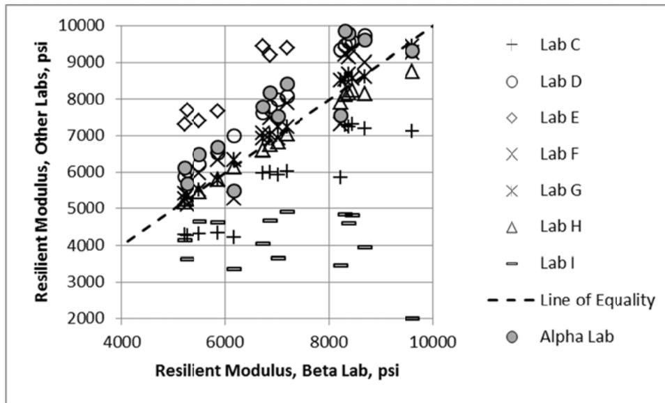
**Figure 39. Resilient Moduli Reported from all Laboratories for the NCAT A-2-4 Soil**
