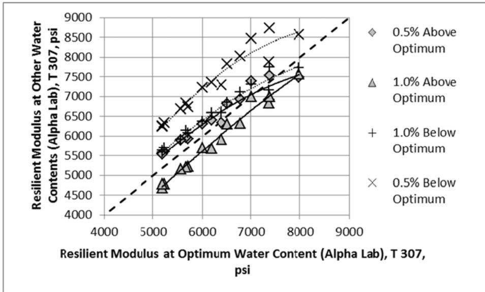
Figure 28. Effect of Water Content on Resilient Modulus Measured in accordance with AASHTO T 307 for the A-7-6 Soil, Alpha Laboratory
