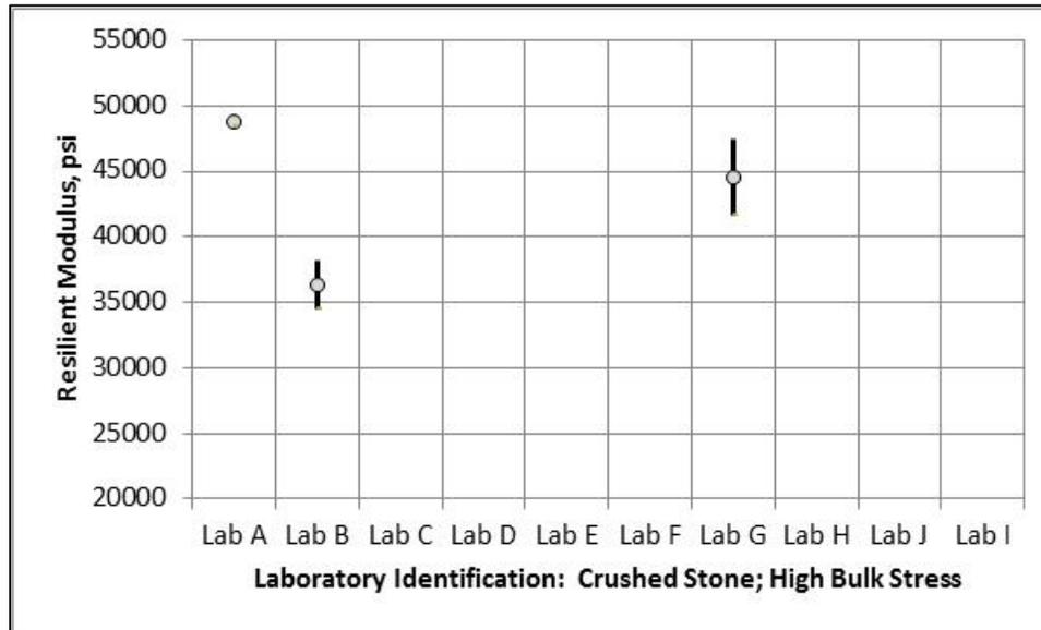
**Figure 49. Difference in Resilient Modulus for the Crushed Stone Base Material; All Participating Laboratories, High Bulk Stress Level**
