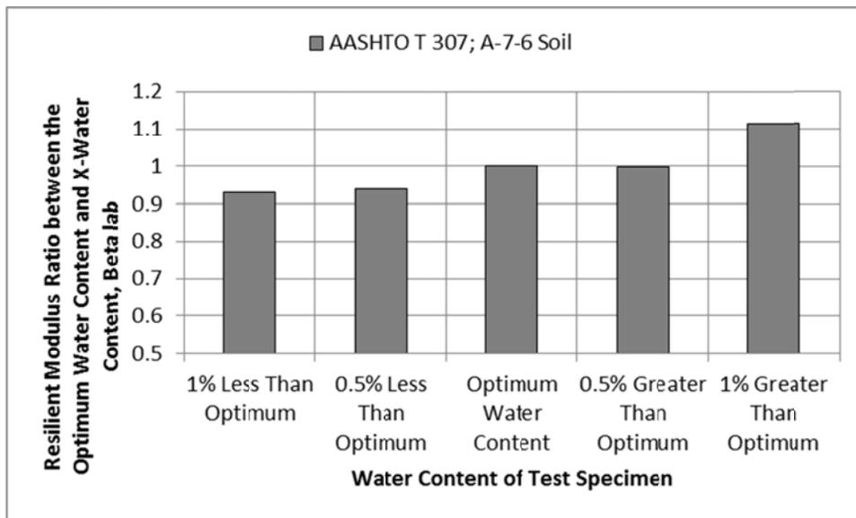
Figure 34. Effect of Water Content on Resilient Modulus Ratio; Beta Laboratory
