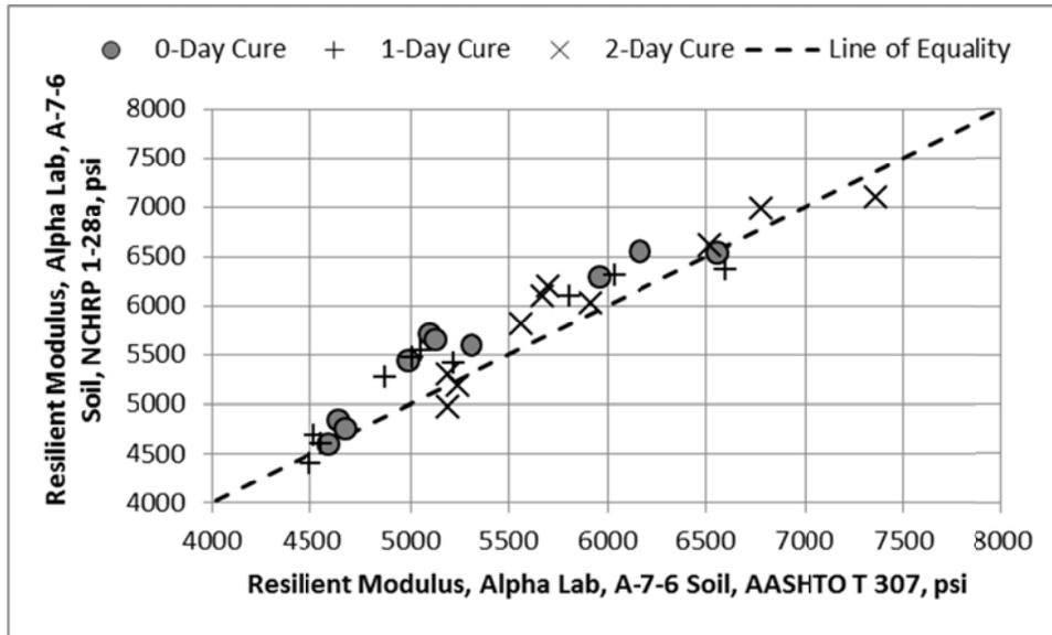
**Figure 22. Comparison of Resilient Modulus Measured by the Alpha Laboratory in Accordance with AASHTO T 307 and NCHRP 1-28a for Different Curing Times, A-7-6 Soil**
