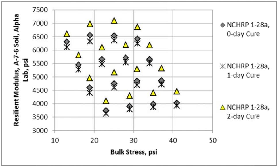
Figure 13. Resilient Modulus for the A-7-6 Soil Measured by the Alpha Laboratory for different Curing Times, NCHRP 1-28a
