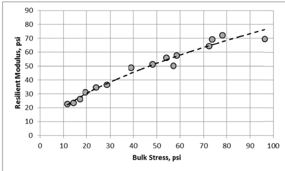
**Figure 64. Crushed Stone Aggregate Base; Repeated Load Resilient Modulus Tests
