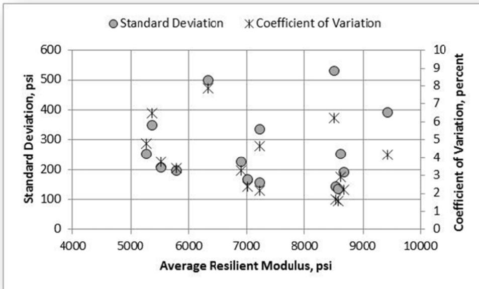
Figure 105. A-2-4 Soil (NCAT Subgrade), Laboratory G, Standard Deviation and Coefficient of Variation
