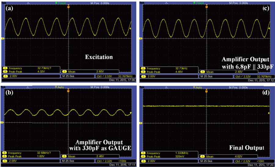
Fig. 6 Test results for the C-Strain Sensor with 330 pF as the nominal capacitance for the AC Wheatstone bridge. (a) external excitation signal; (b) the amplifier output without capacitance change; (c) the amplifier output with 6.8 pF capacitance change; (d) the final output with 6.8 pF capacitance change.
