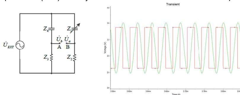
Fig. 3 The AC Wheatstone bridge and the waveforms used in C-Strain board.
