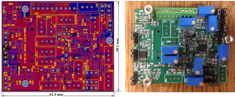
Fig. 2 PCB design and the fabricated C-strain board.
