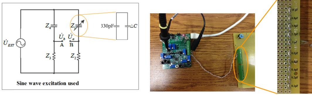
Fig. 5 Test setup for the C-strain sensor (left is the AC Wheatstone bridge configuration used in the sensor for the test).
