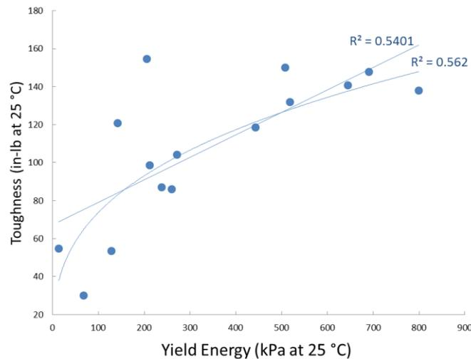
Figure 12. Toughness and Yield Energy at 25 °C for WCTG binder set.
