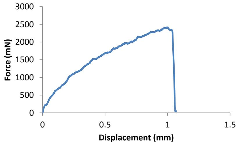
Figure 8.1. Graph. BBR-SENB typical force-displacement curve
