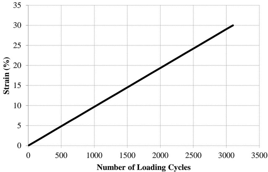
**Figure 2– Loading scheme for amplitude sweep test**
