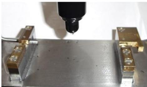
Figure 6.3. Photograph. Beam supports to ensure notch alignment
