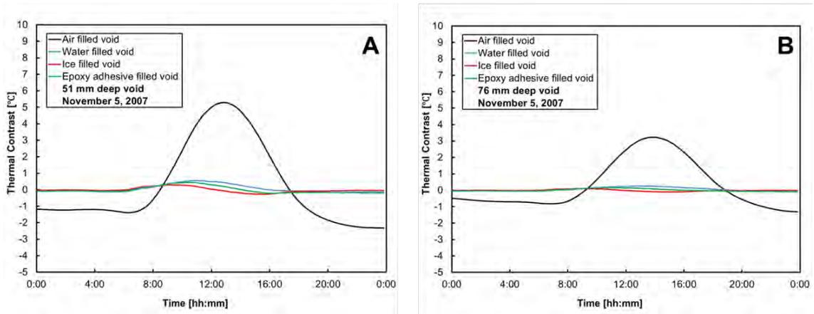
**Figure 17: Results from a computer model of filled voids**
