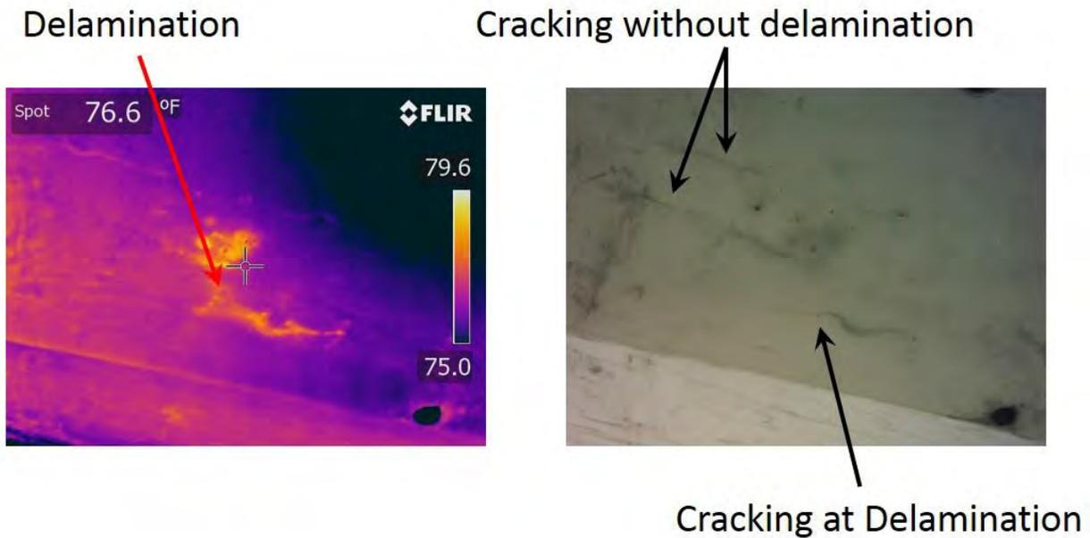
**Figure 38: IR (A) and digital (B) image of a possible parge coat delamination**
