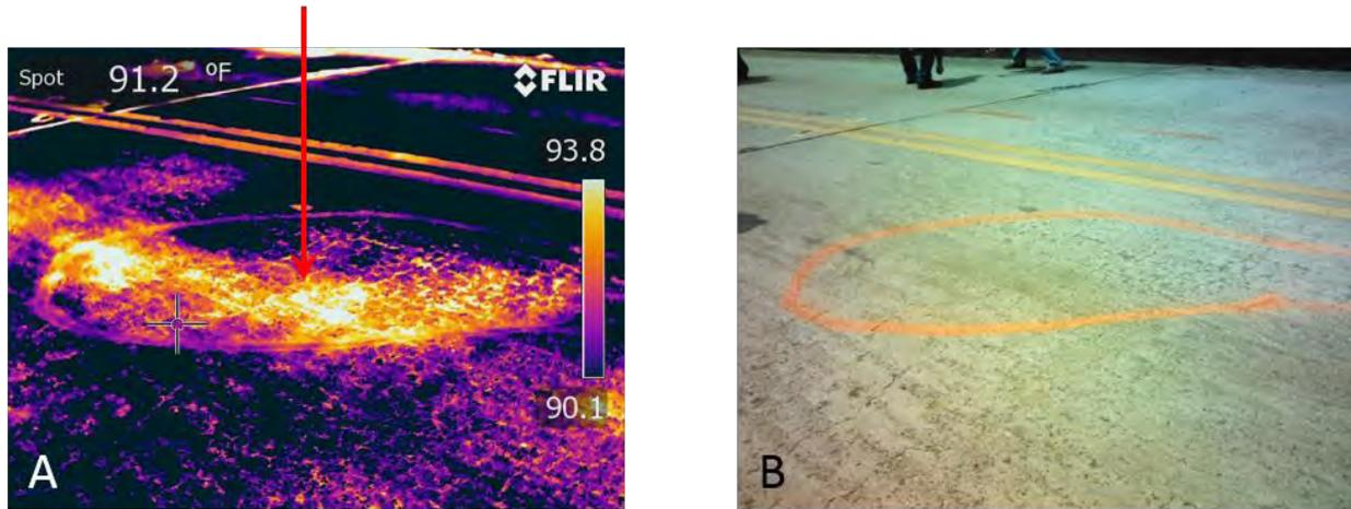
**Figure 29: IR (A) and digital (B) images of a deck delamination over a railroad on Dames Ferry Rd.**
