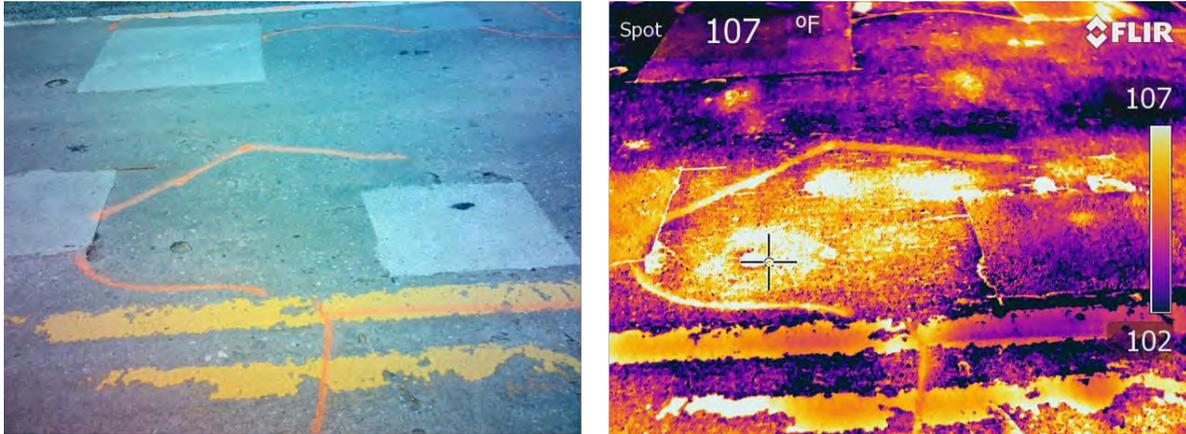
Figure 3: Standard and IR photos of bridge deck delamination (Barnesville, Georgia)
