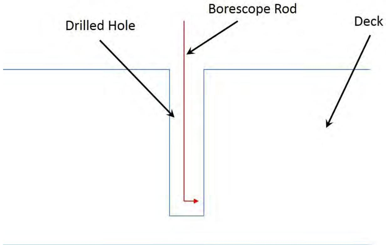
**Figure 23: Schematic diagram of how the borescope is used**
