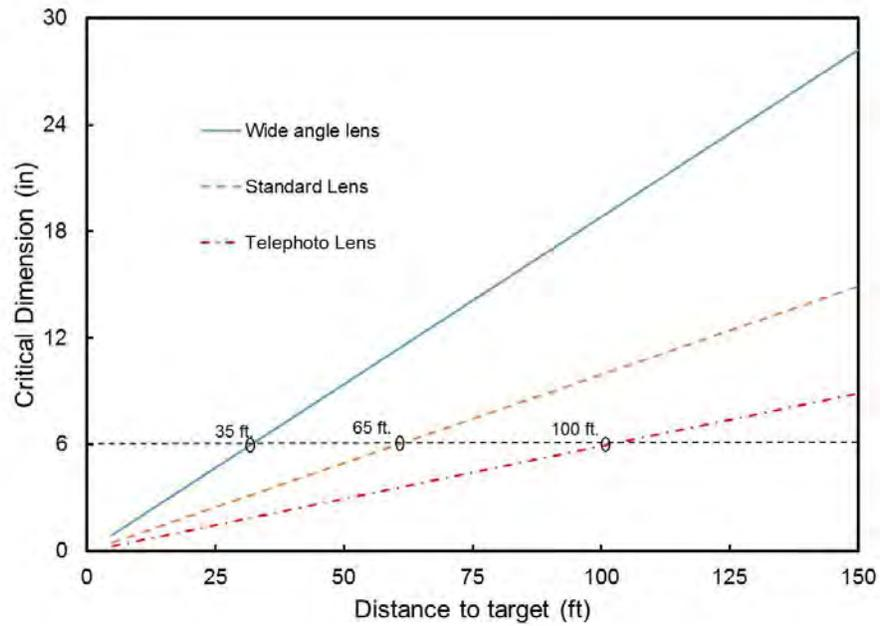
Figure A3. Graph showing critical dimension as a function of distance.
