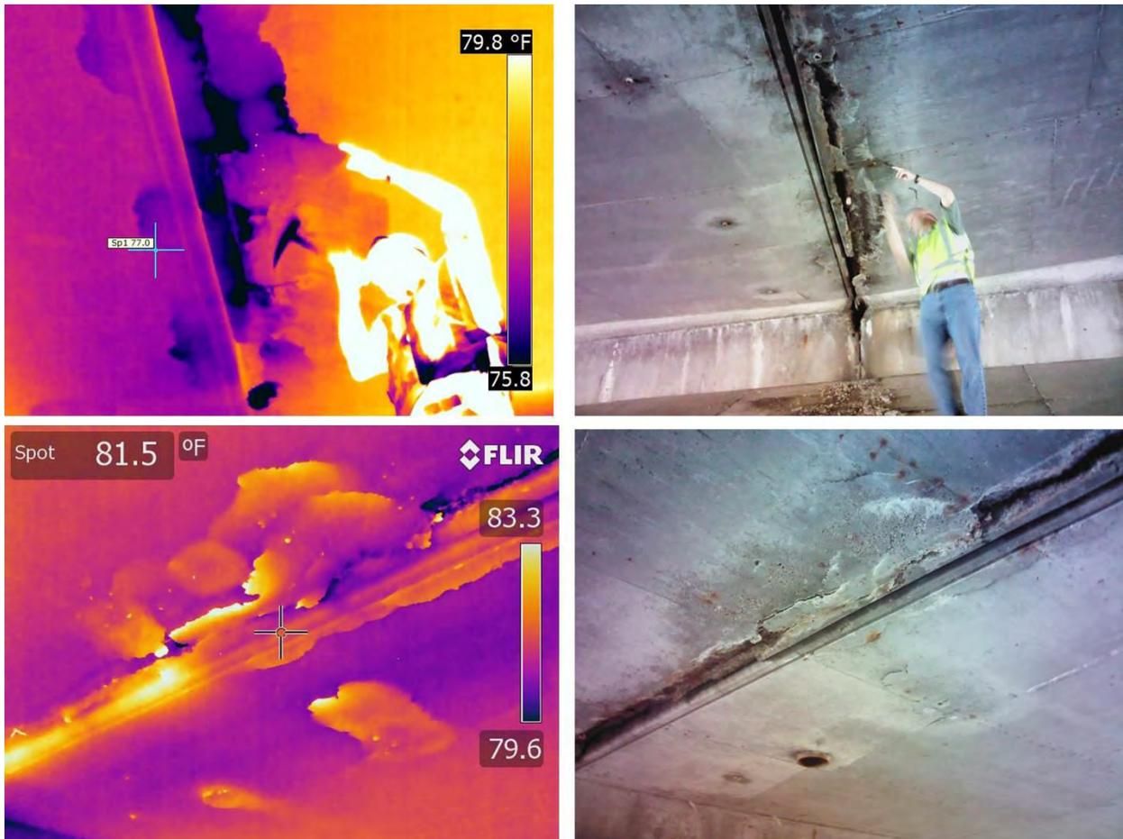
**Figure 50: Thermal images showing damage along a longitudinal joint in a 159 ft. wide slab bridge**
