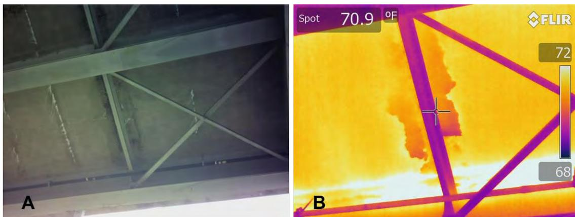
**Figure 9: Delamination with some spalling by a cross brace in the soffit**
