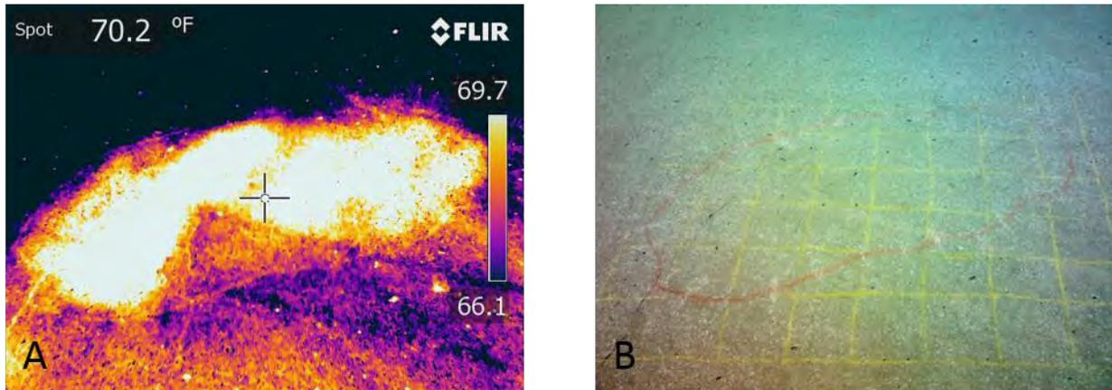
**Figure 2: Infrared (A) and digital (B) images of a deck delamination in Kansas City**
