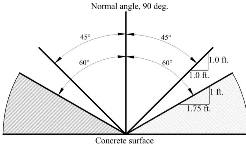
**Figure A1. Schematic diagram of observation angles.**
