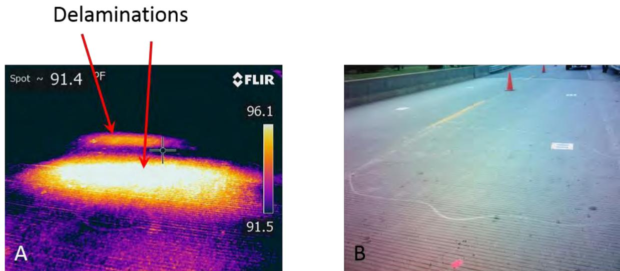
**Figure 19: Infrared (A) and Digital (B) images of a deck delamination in Lamoni, IA**
