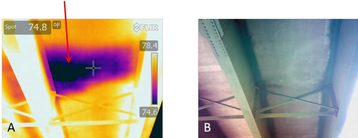
**Figure 20: Infrared (A) and Digital (B) images from the soffit of the delamination in Figure**
