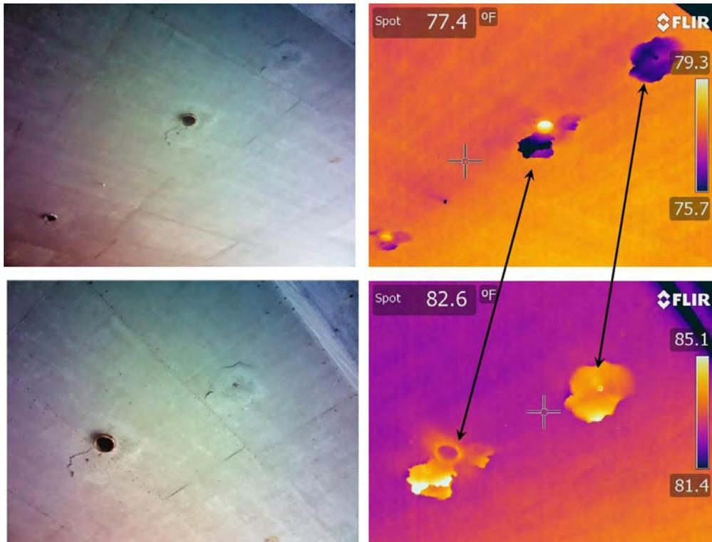
**Figure 49: Thermal images of delaminations in the soffit of a wide slab bridge, showing morning (top) and afternoon (bottom) results**
