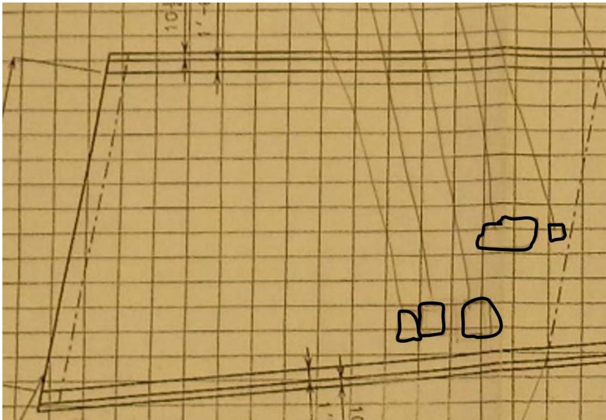
**Figure 1: Chain drag results for the North span of Bridge A0295**
