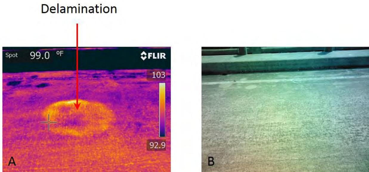
**Figure 45: Infrared (A) and digital (B) images of a deck delamination in Florida**
