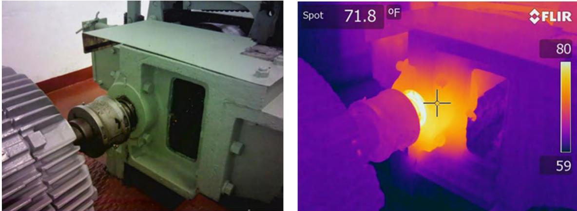
Figure 21: Standard and IR photos of Lewis and Clark River drawbridge mechanism (Astoria, Oregon)
