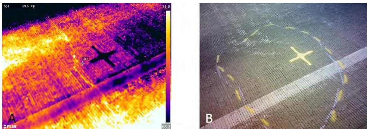
**Figure 15: Thermal image showing an area of deck repaired by epoxy injection**
