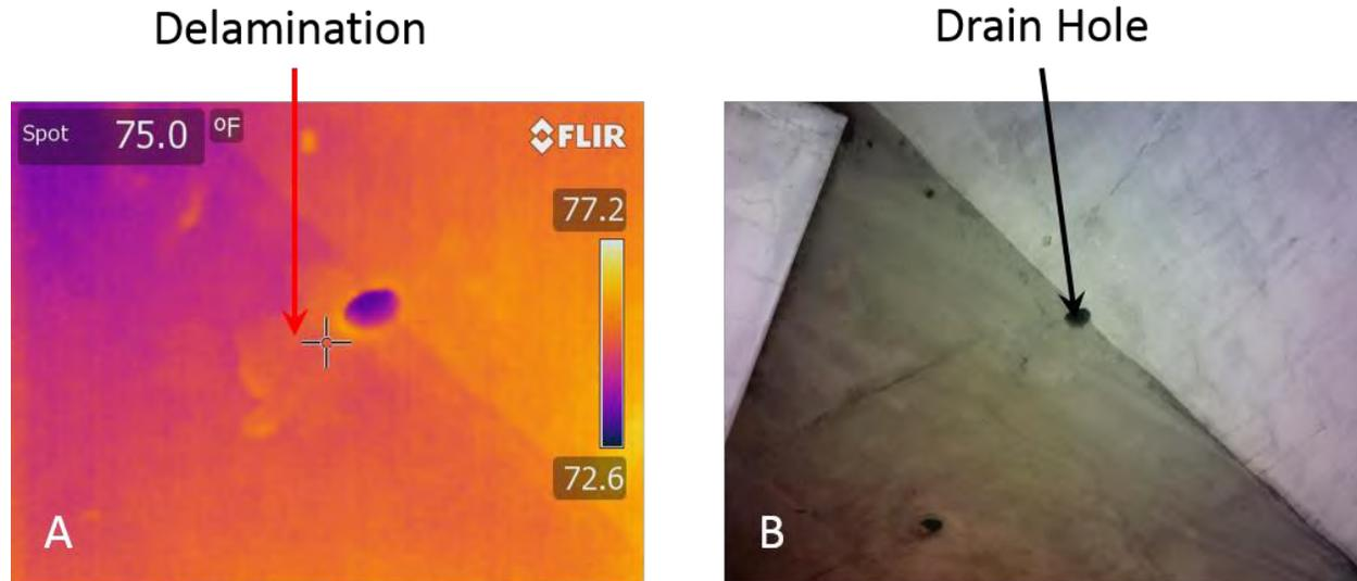
**Figure 37: Thermal image (A) and digital image (B) of a drain delamination**
