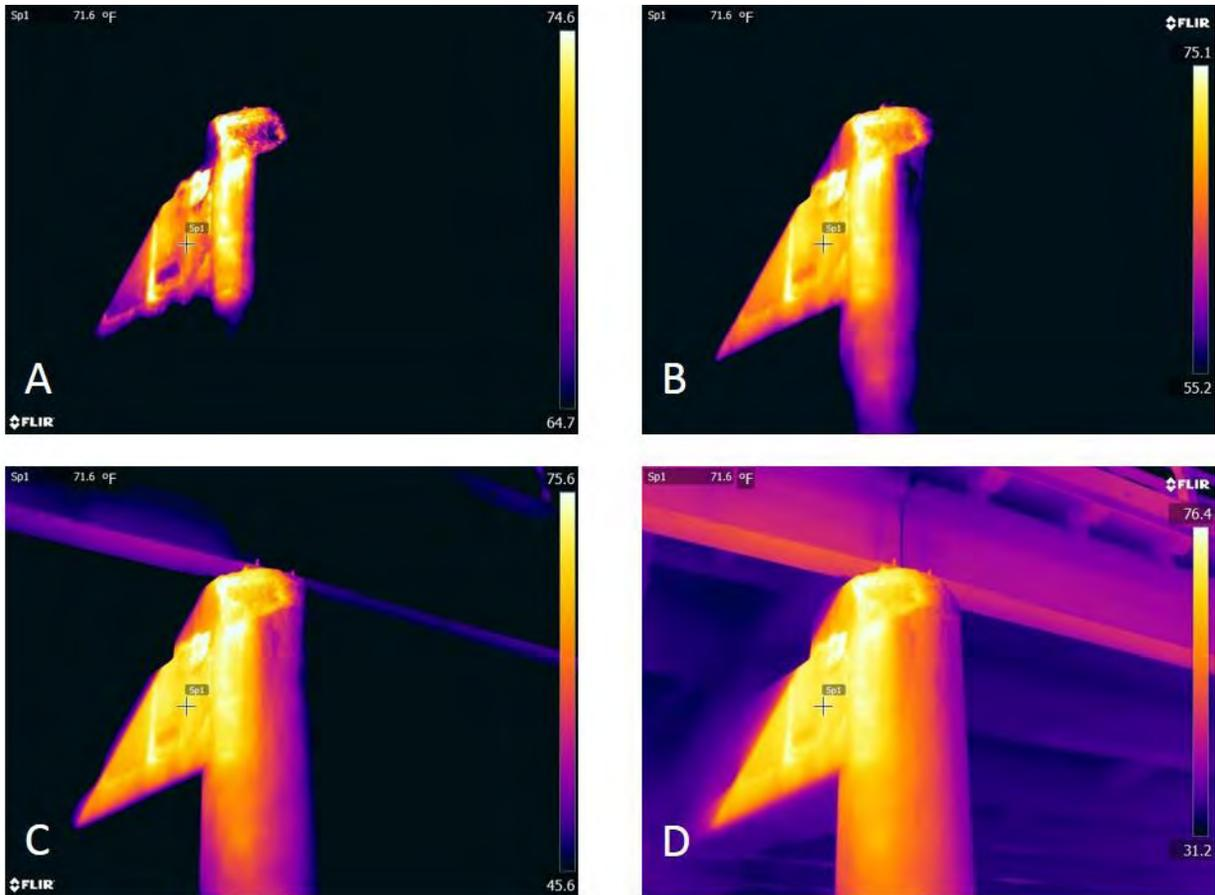
**Figure 44: Illustration of how thermal gradient can affect an image**
