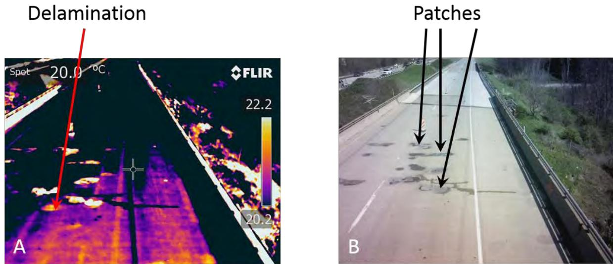
**Figure 33: IR (A) and digital (B) images from a boom of a deck in Pennsylvania**
