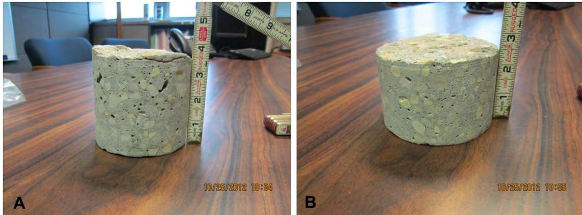
**Figure 16: Cores from the delaminations in the deck**
