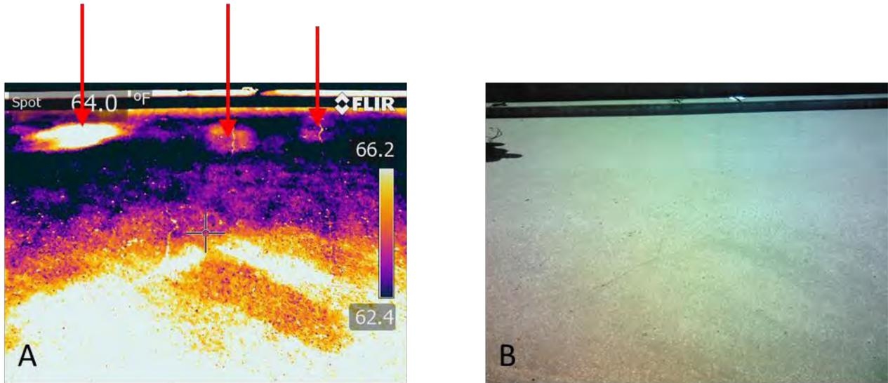
**Figure 3: Infrared (A) and Digital (B) images of a group of delaminations in Kansas City**
