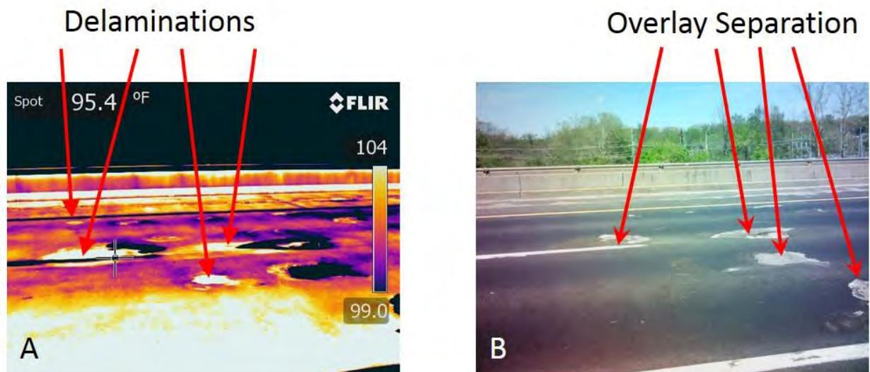
**Figure 5: Infrared (A) and Digital (B) images of Providence Rd. Bridge (northbound) over Hinkson Creek**
