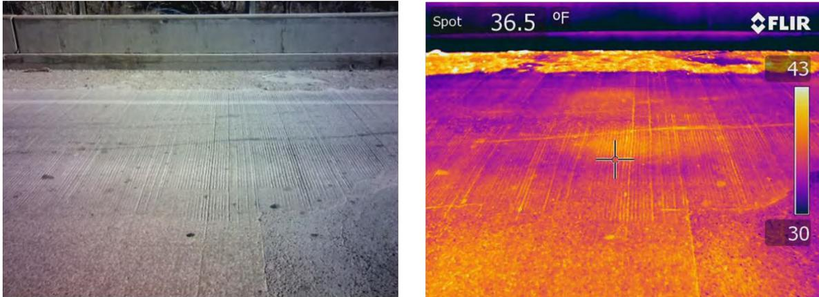
Figure 5: Standard and IR photos of bridge deck delamination (Vinton, Iowa)
