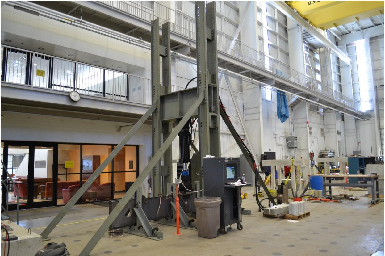
**Figure 4: Axial test setup precrack test frame**
