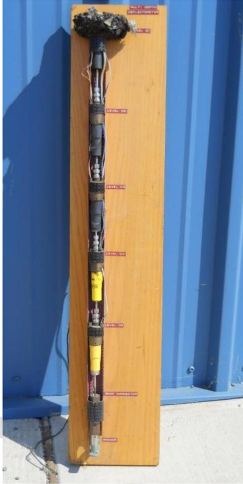
Figure F-22. A model multi-depth deflectometer (MDD), showing five modules.
