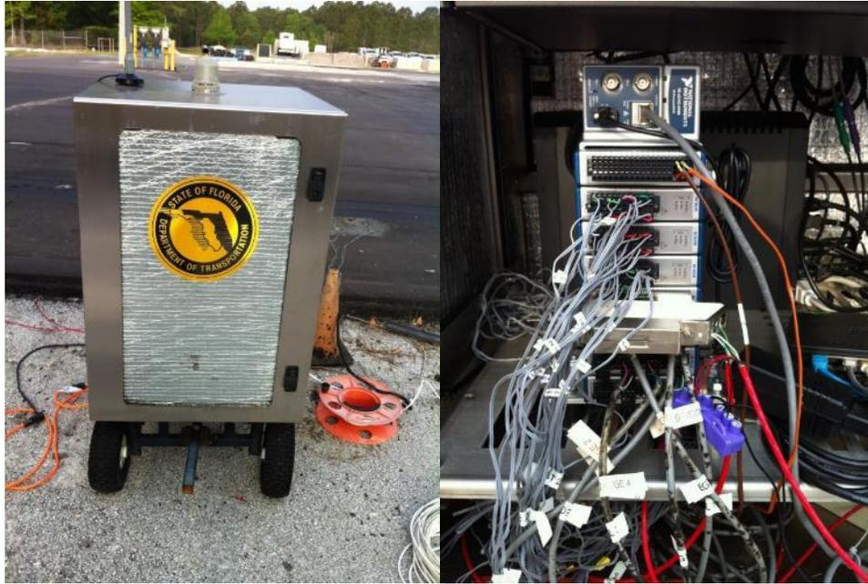
**Figure E-10. Mobile DAQ system.**
