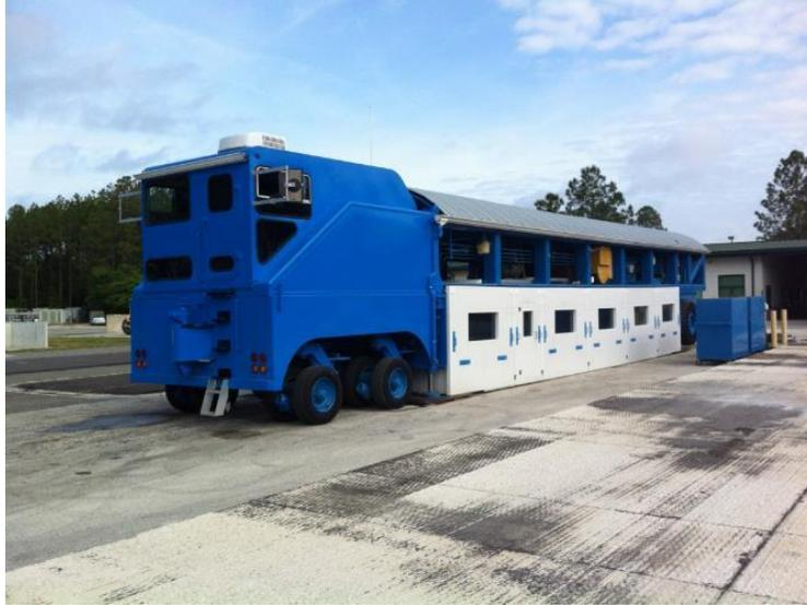
**Figure E-2. Insulated panels on HVS.**
