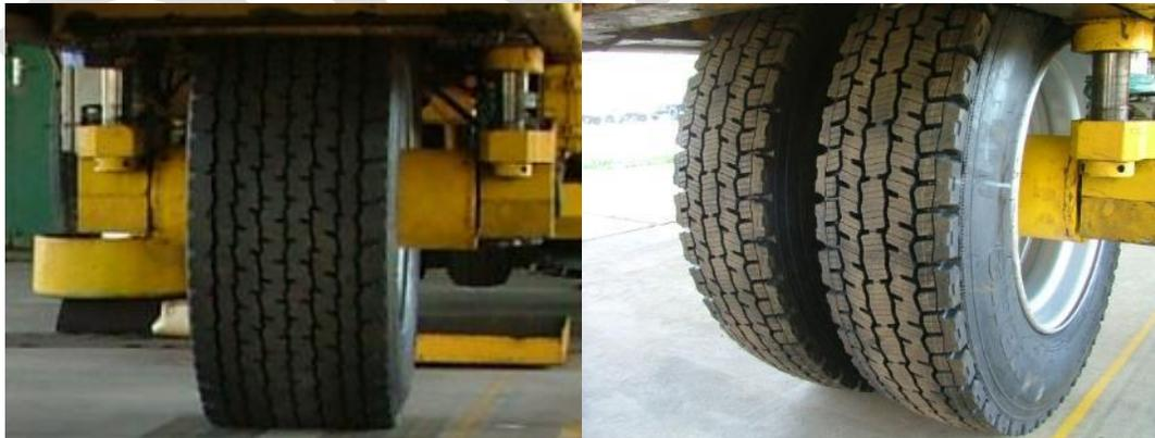
Figure 3-3. Test tires: WBT and DTA.
