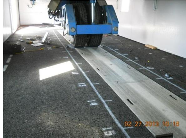
(b). Interior view of the temperature control chamber while validating HVS half-axle load
