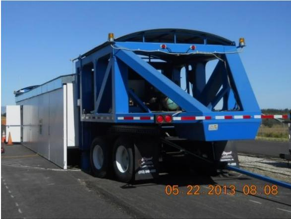
(a). Overall view of the HVS with temperature control chamber
