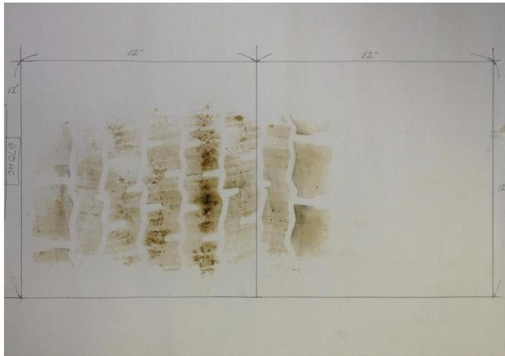
**Figure F-30. New-generation wide-base tire footprint.**
