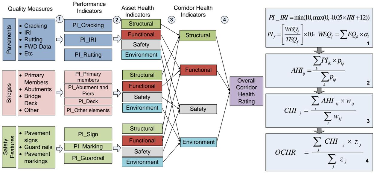
**FIGURE 2 Performance aggregation framework and computation steps.**
