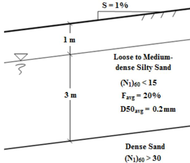
**Figure 2-2 Soil profile used for the lateral spread displacement comparison study.**
