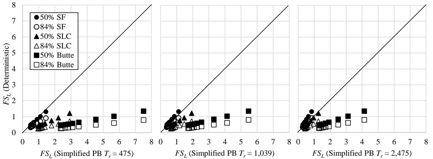
**Figure 2-5 Comparison of deterministic and simplified performance-based values of  $FS_L$ .**
