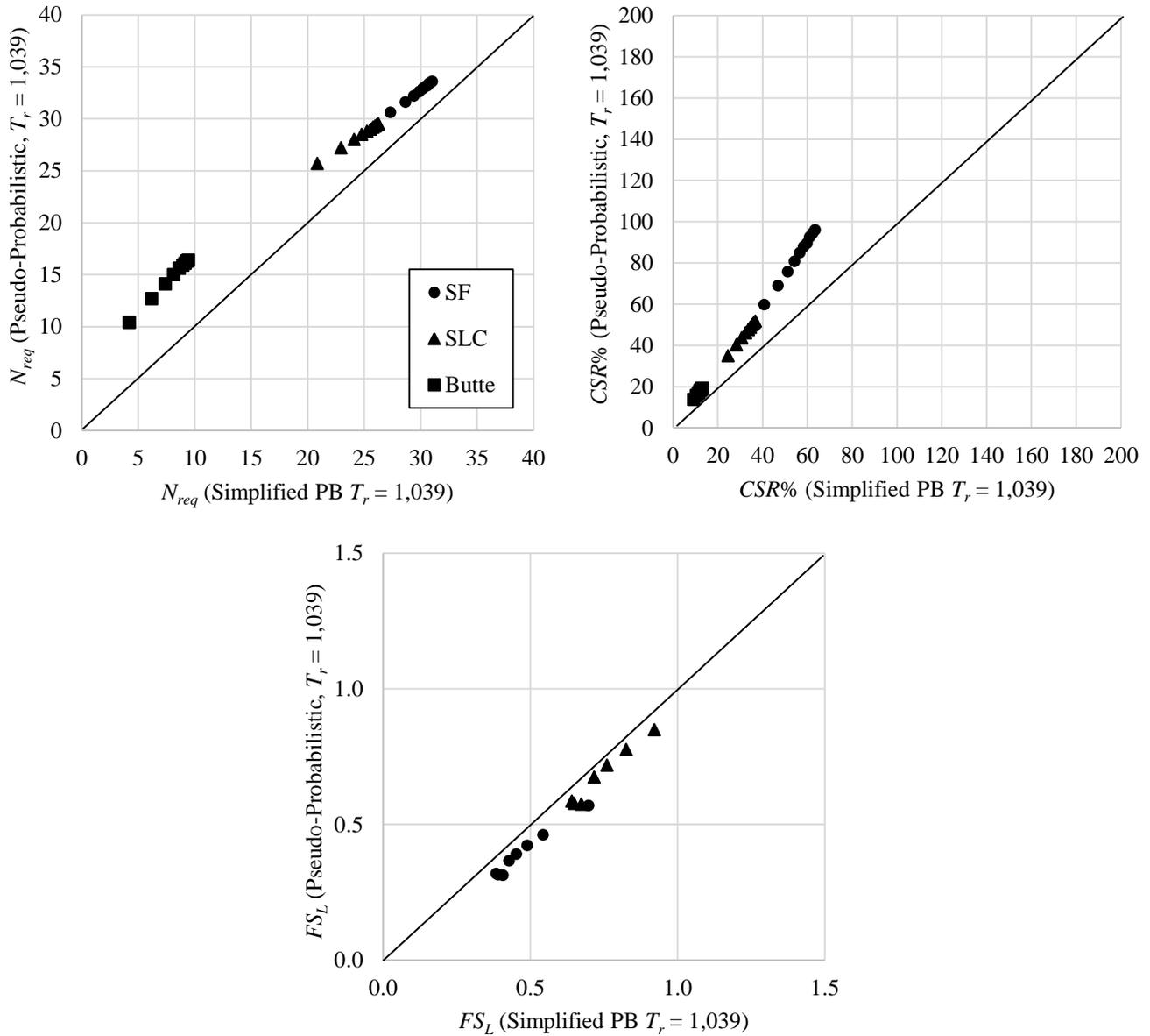
**Figure 2-3 Comparison of pseudo-probabilistic and simplified performance-based values of  $N_{req}$ , CSR%, and  $FS_L$ .**
