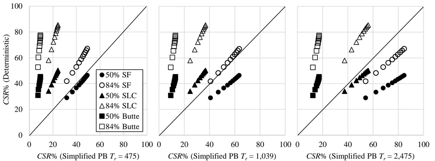
**Figure 2-6 Comparison of deterministic and simplified performance-based values of  $CSR\%$ .**
