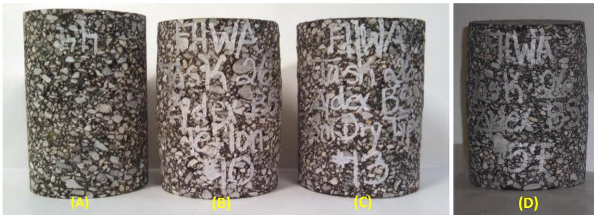
**Figure 3 Comparison of (A) Untested Flow Number Specimens, (B) Specimen Tested Using Single-Layer Teflon, (C) Specimen Tested Using Spray Silicone, and (D) Specimen Tested Using Double-Layer Teflon**
