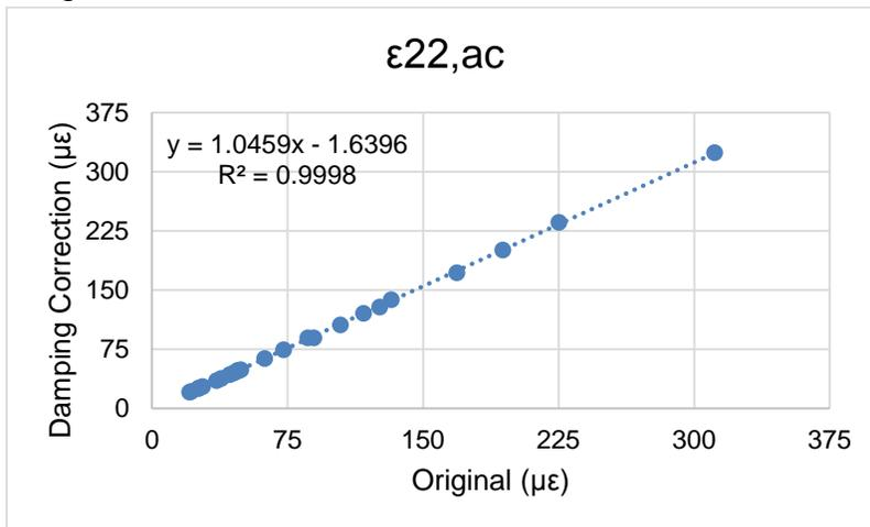
Figure B-5. Vertical compressive strain in the AC layer.
