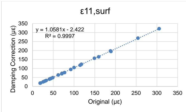
Figure B-1. Longitudinal strain at the AC surface.
