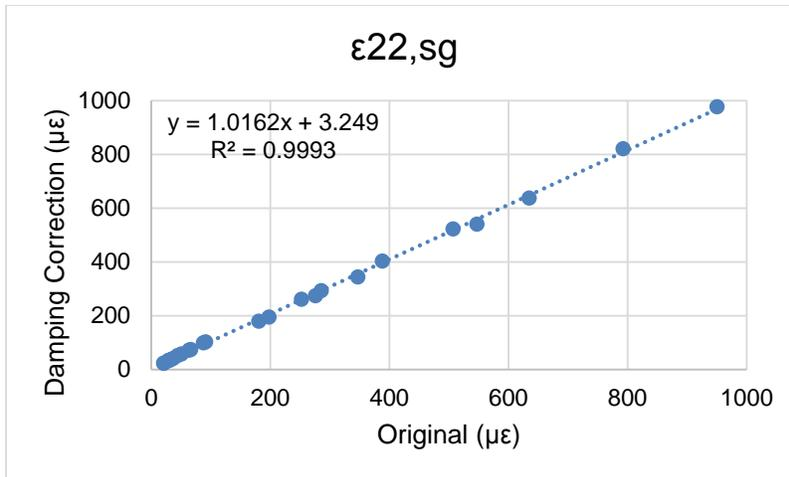
Figure B-7. Vertical compressive strain in the subgrade layer.
