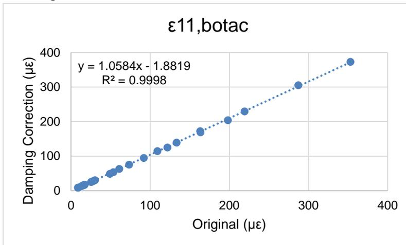
Figure B-3. Longitudinal strain at the bottom of the AC.
