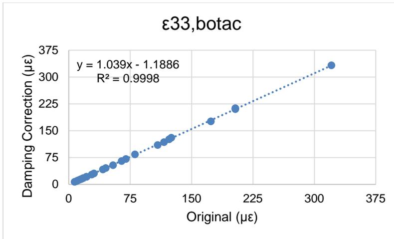
Figure B-4. Transverse strain at the bottom of the AC.
