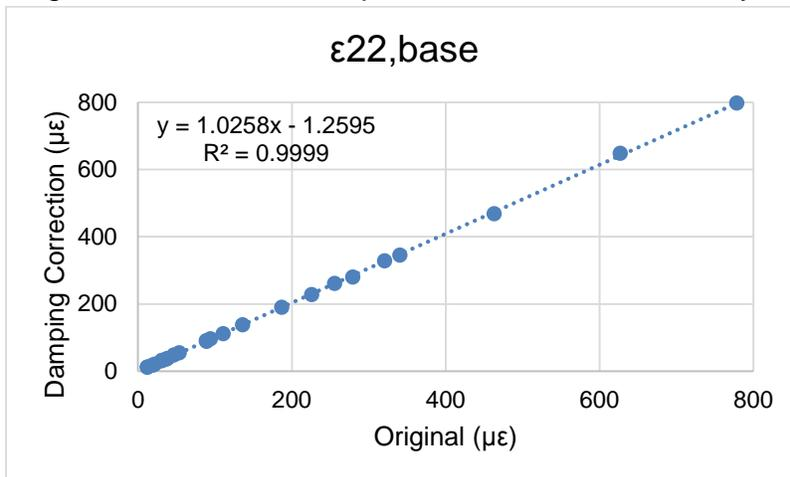
Figure B-6. Vertical compressive strain in the base layer.
