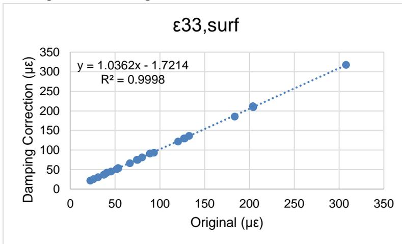
Figure B-2. Transverse strain at the AC surface.
