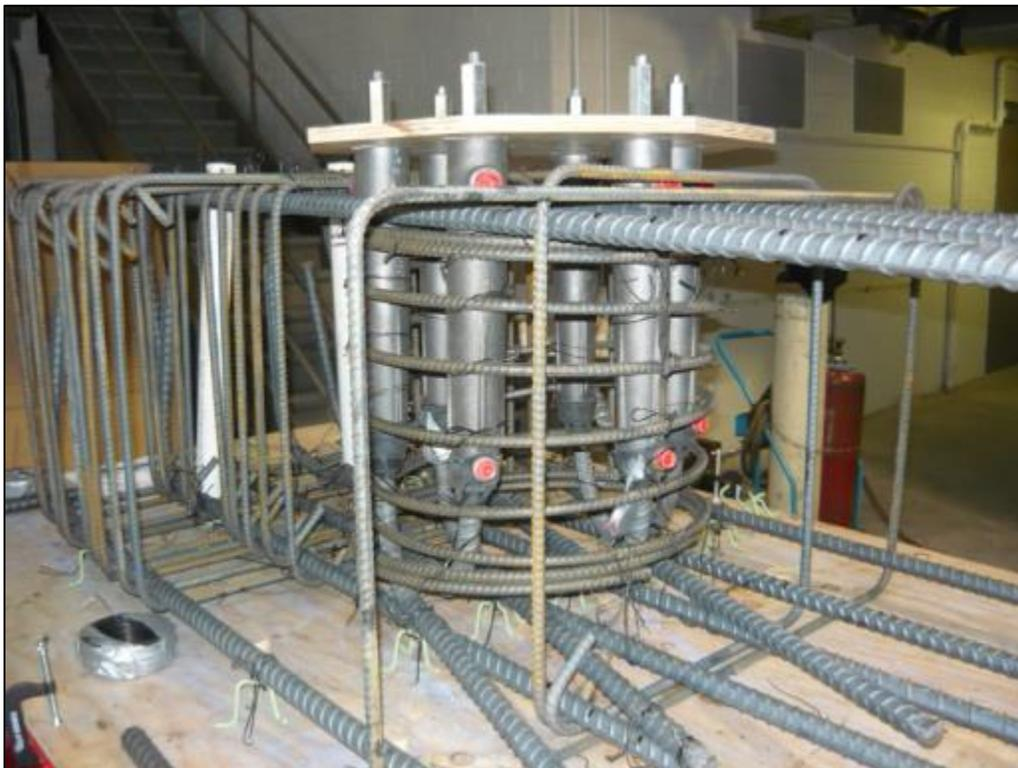
Figure 2-10. GGSS-2 precast footing core rebar cage.
