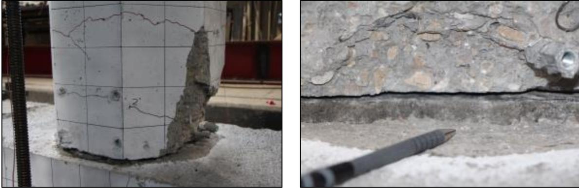
Figure 4-48. Damage state for FGSS-3 at end of test: cracks and spalling, permanent gap.
