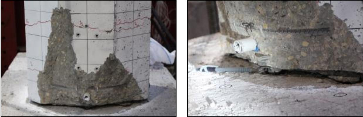
(b) Damage state at 8% drift ratio: cracks and spalling, fractured bar, and exposed rebar cage.
