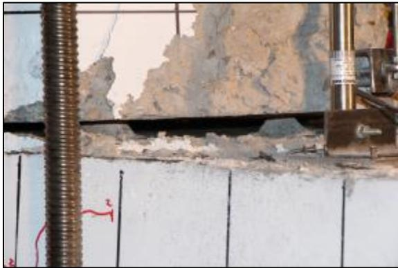
(c) Bar pull-out during 6% drift ratio.
