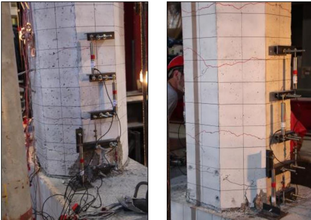
Figure 4-46. Damage state for FGSS-3 at 4% drift ratio.
