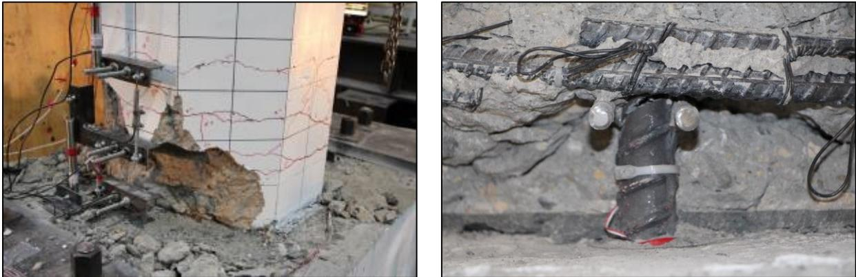
(b) Damage state at 7% drift ratio: cracks, spalling, fractured bar, and exposed rebar cage.
