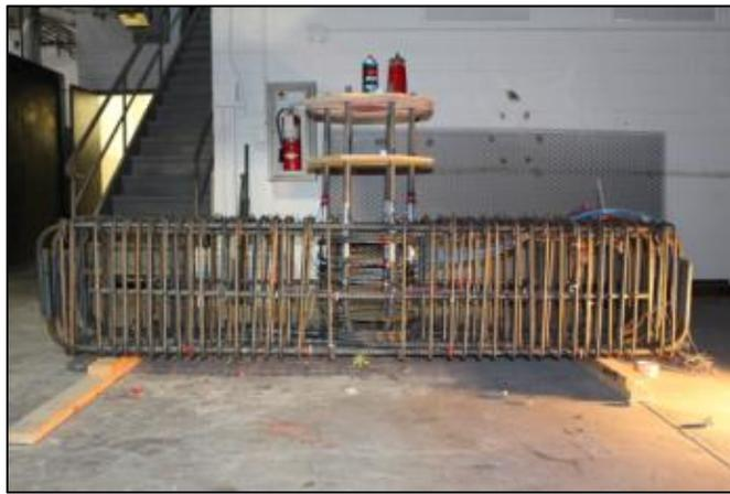
(b) Cap beam rebar cage.
