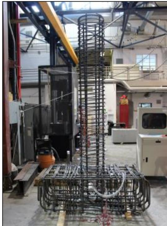
(b) Rebar cage ready to cast concrete.
