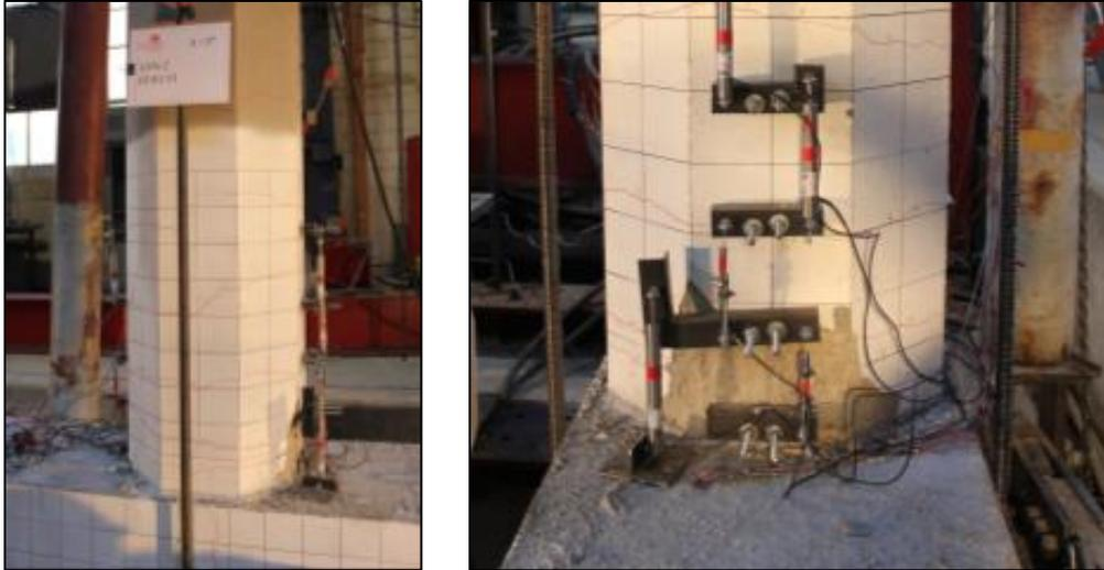
(a) Damage state at 3% drift ratio: cracks and spalling.
