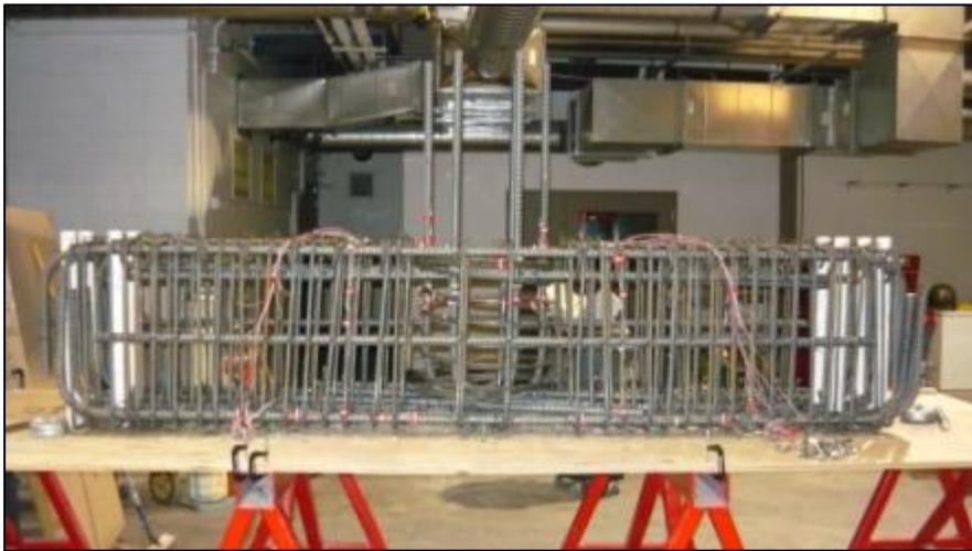
(b) Cap beam rebar cage.
