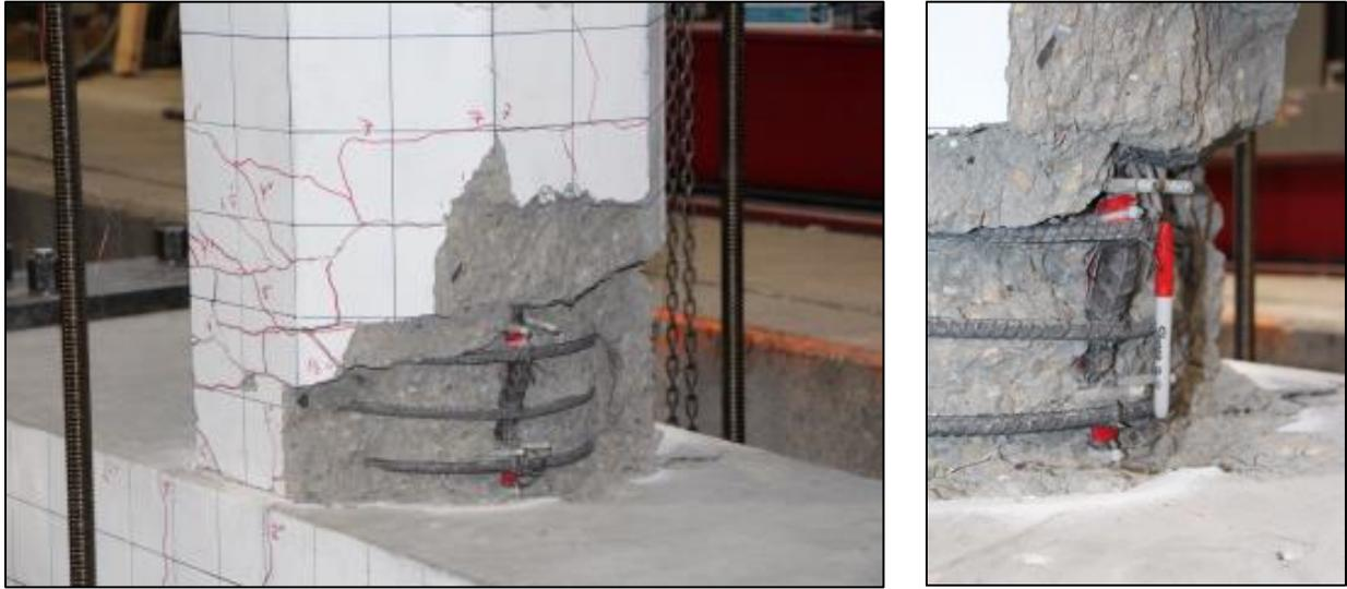
Figure 4-57. Damage state for FGSS-CIP at end of test: cracks and spalling, rebar buckling and fracture.
