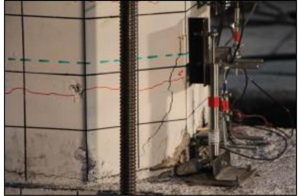
(b) Damage state at 3% drift ratio.
