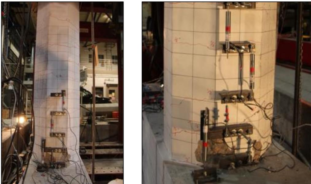
Figure 4-54. Damage state for FGSS-CIP at 3% drift ratio.
