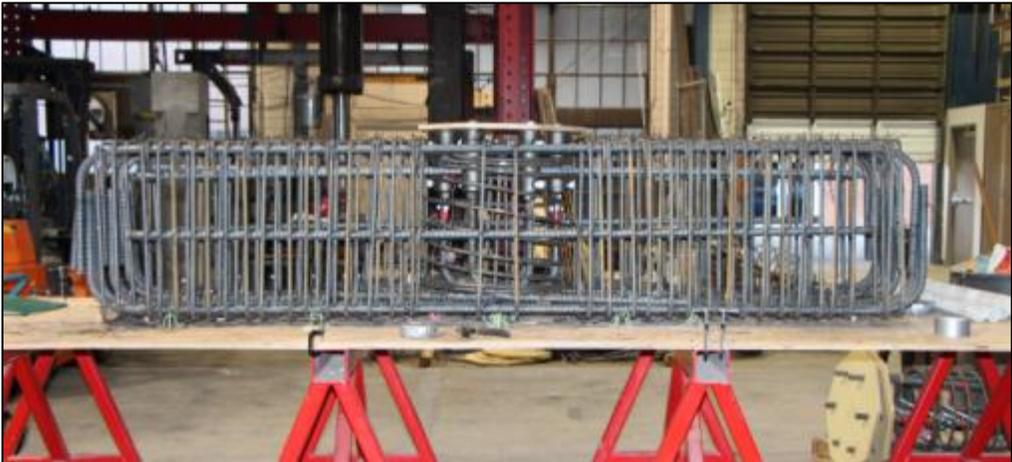
(b) Cap beam rebar cage.
