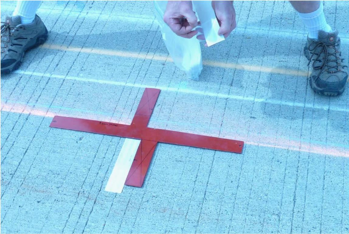
**Figure B-8. ICC SurPRO 4000 pavement marking template.**
