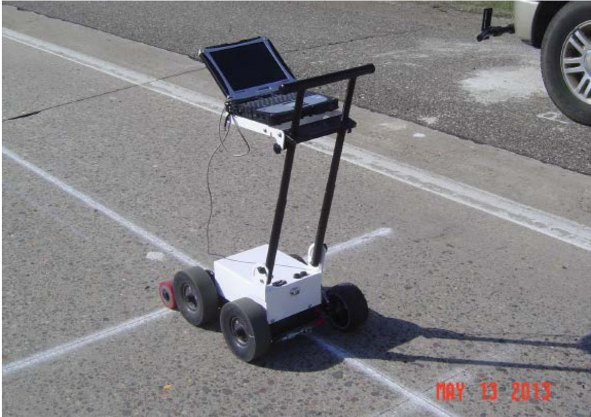
**Figure B-1. SSI SC8800 Walking Profiler.**
