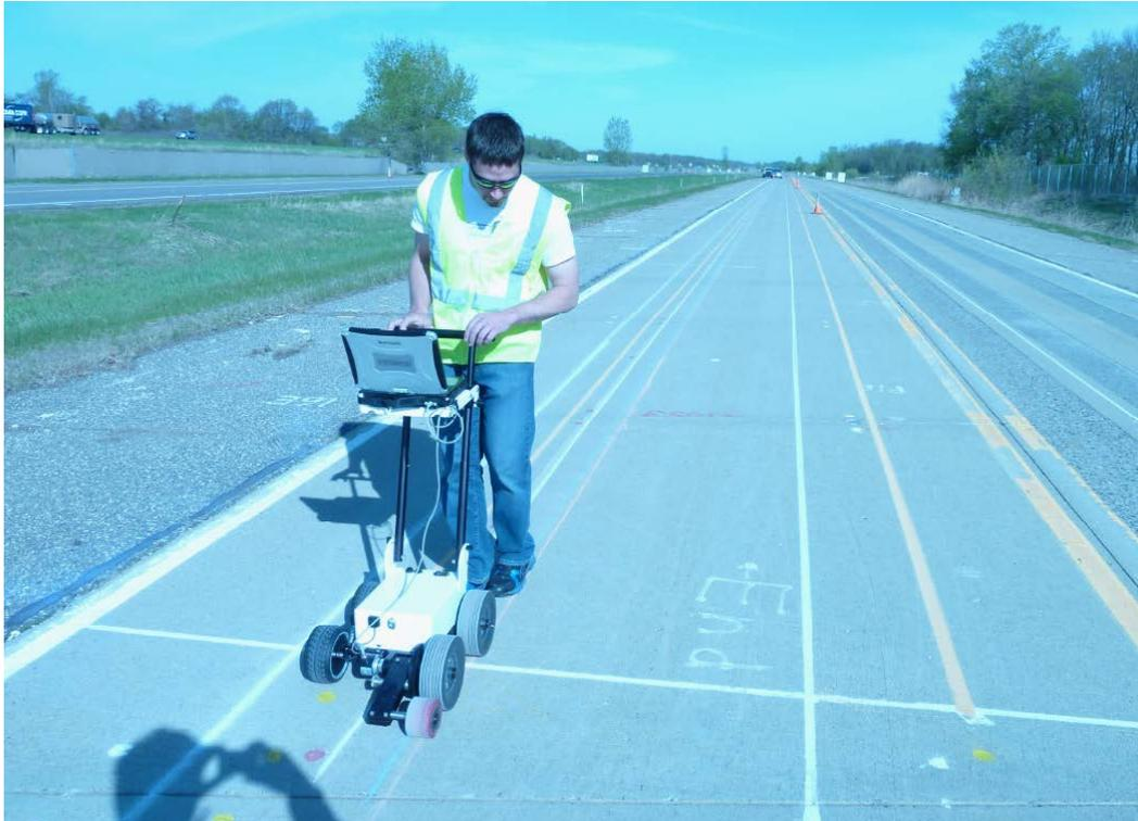
**Figure B-3. SSI SC8800 Walking Profiler on transverse tining.**
