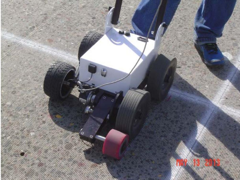
**Figure B-2. SSI SC8800 Walking Profiler, close-up.**
