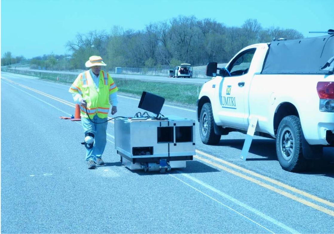
**Figure B–10. Benchmark Profiler cart at the chip seal section.**
