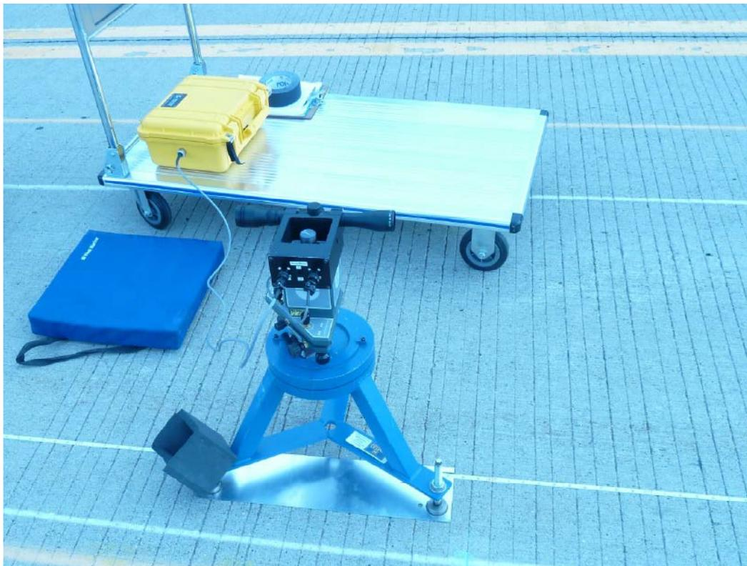
**Figure B-13. Benchmark Profiler reference laser stand and power supply.**
