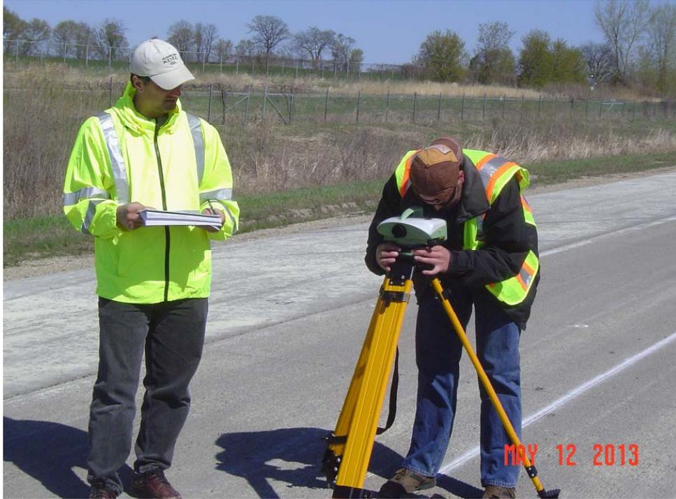
**Figure B-14. Leica DNA 03 level.**
