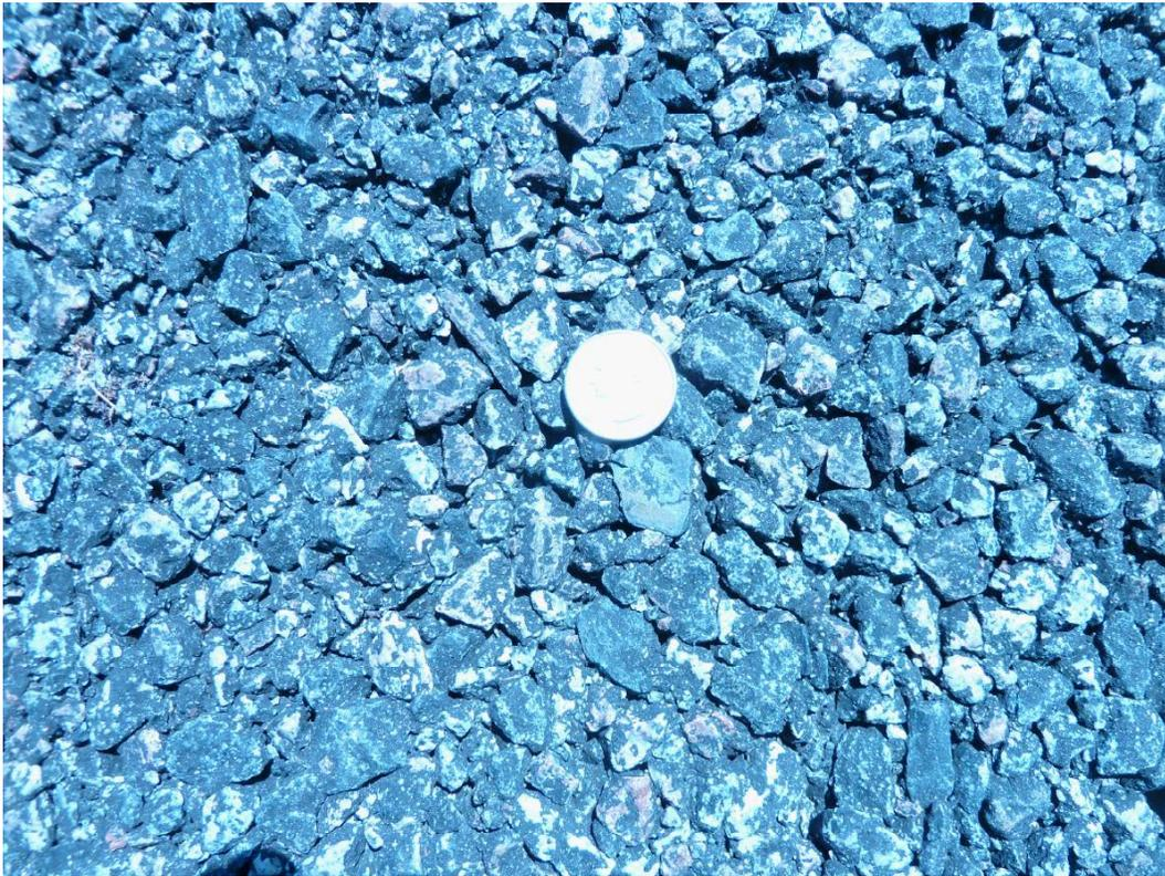
**Figure A-6. Pervious hot mix asphalt texture.**
