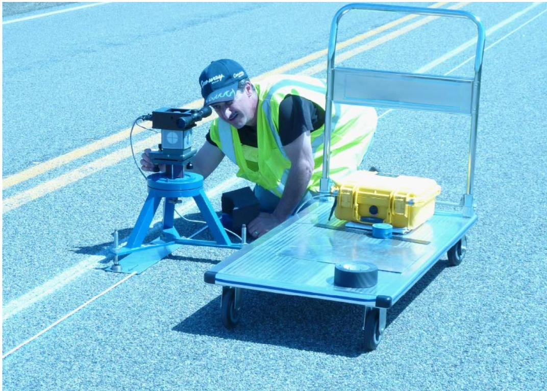
**Figure B–11. Benchmark Profiler reference laser alignment.**
