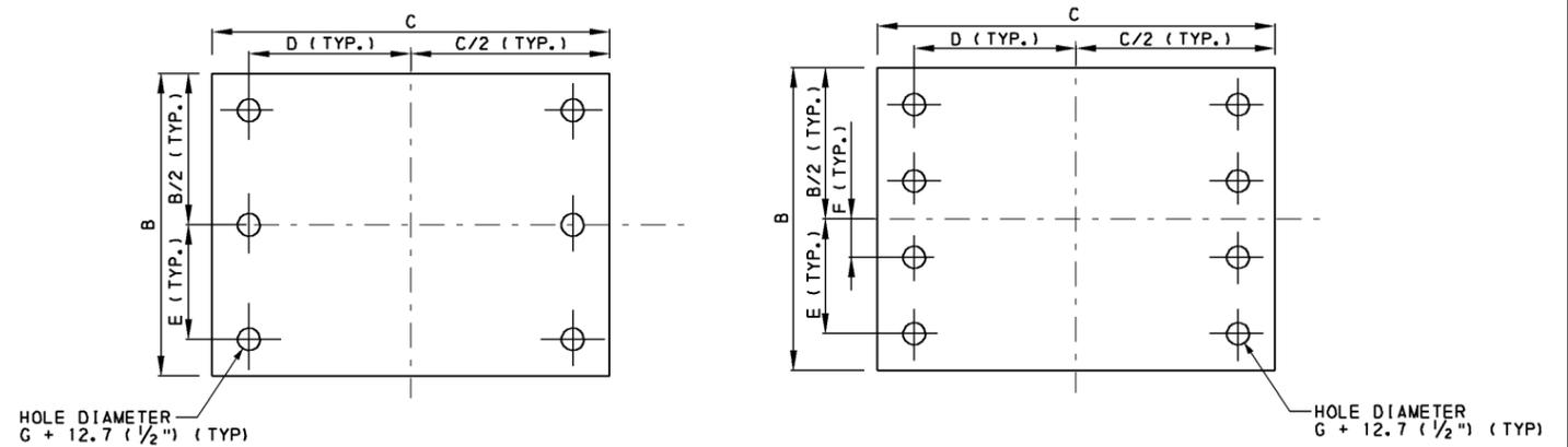
**ANCHOR BOLT LOCATION PLAN - 6 AND 8 ANCHOR BOLTS**
