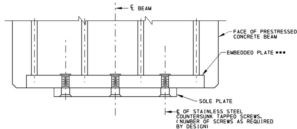
\* NUMBER OF STUDS OR ANCHORS AS REQUIRED BY DESIGN. SPACED AS REQUIRED TO MISS STRAND PATTERN
