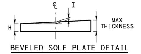
\* - BEARING HEIGHT INCLUDES 1/8" BEDDING MATERIAL. EFFECTS OF BEVELED SOLE PLATE ARE NOT INCLUDED. IF BEVELED SOLE PLATE IS USED CALCULATE INCREASED BEARING HEIGHT ACCORDINGLY.
