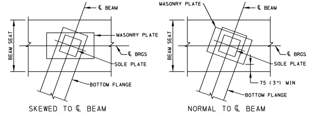
**SOLE AND MASONRY PLATE ORIENTATION OPTIONS**
