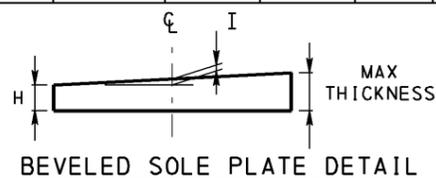
\*- BEARING HEIGHT INCLUDES 3.2 BEDDING MATERIAL. EFFECTS OF BEVELED SOLE PLATE ARE NOT INCLUDED. IF BEVELED SOLE PLATE IS USED CALCULATE INCREASED BEARING HEIGHT ACCORDINGLY.
