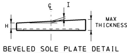
\* - BEARING HEIGHT INCLUDES 3.2 (1/8") BEDDING MATERIAL. EFFECTS OF BEVELED SOLE PLATE ARE NOT INCLUDED. IF BEVELED SOLE PLATE IS USED CALCULATE INCREASED BEARING HEIGHT ACCORDINGLY.
