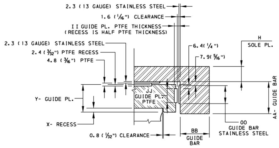
ALTERNATE GUIDE BAR FABRICATION DETAIL
