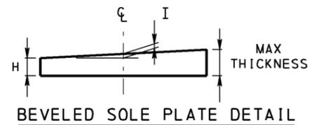
\* - BEARING HEIGHT INCLUDES 1/8" BEDDING MATERIAL. EFFECTS OF BEVELED SOLE PLATE ARE NOT INCLUDED. IF BEVELED SOLE PLATE IS USED CALCULATE INCREASED BEARING HEIGHT ACCORDINGLY.
