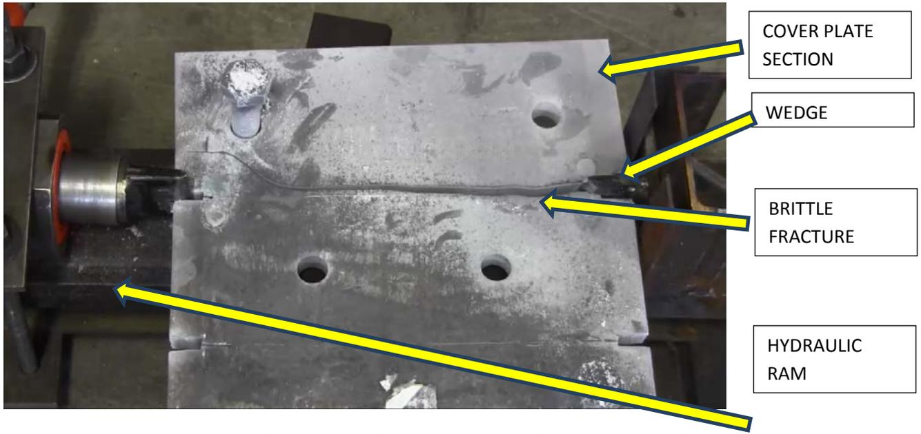
Figure 2: Test setup for evaluation of driven wedge method for producing brittle fracture
