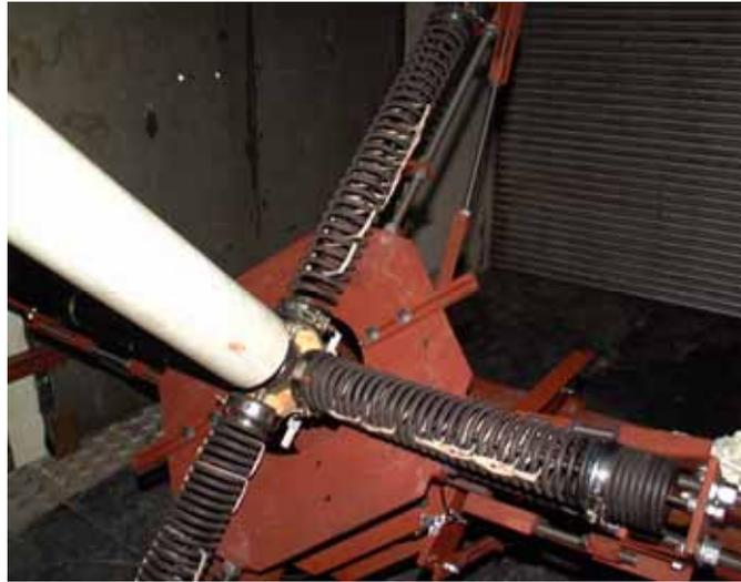
**Figure 46. Photo. Elastic bands on the spring coils.**
