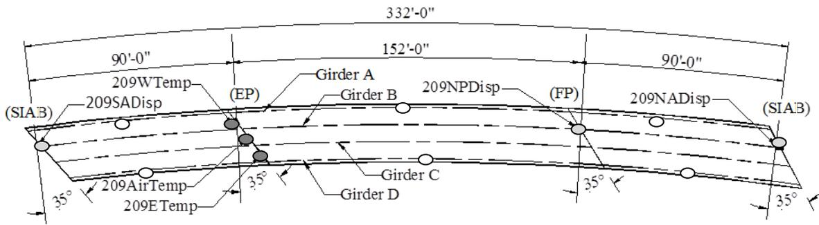
**Figure 5.22. Bridge 209 instrumentation**
