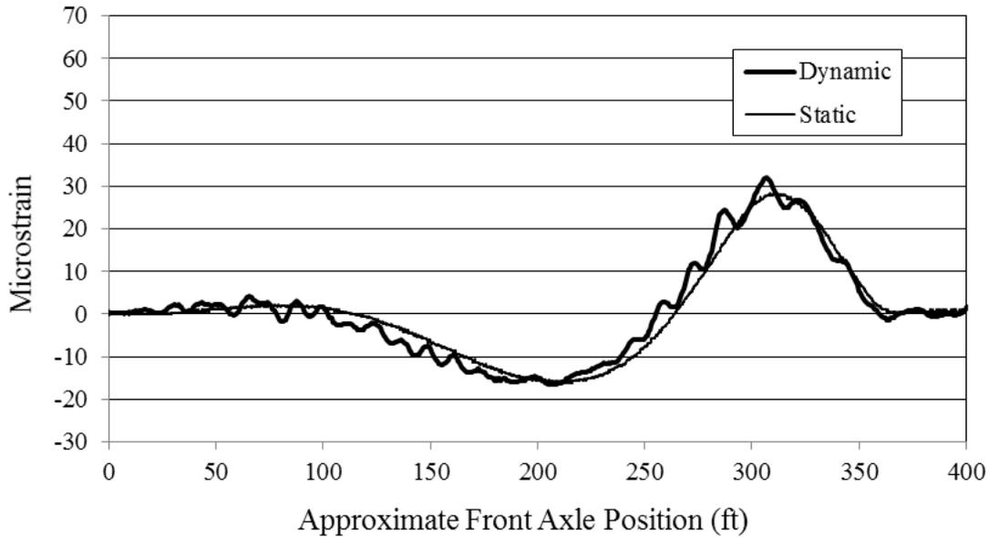
**Figure 7.18. Superimposed static and dynamic load strains**
