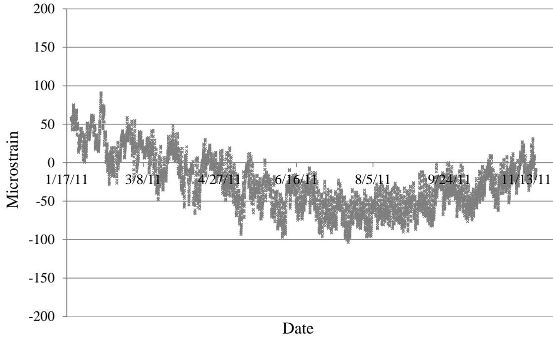
**Figure 6.7. Top flange east strain gauge reading**
