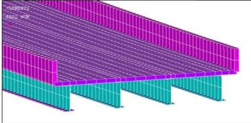
**Figure 8.9. Typical meshed cross section with parapets**
