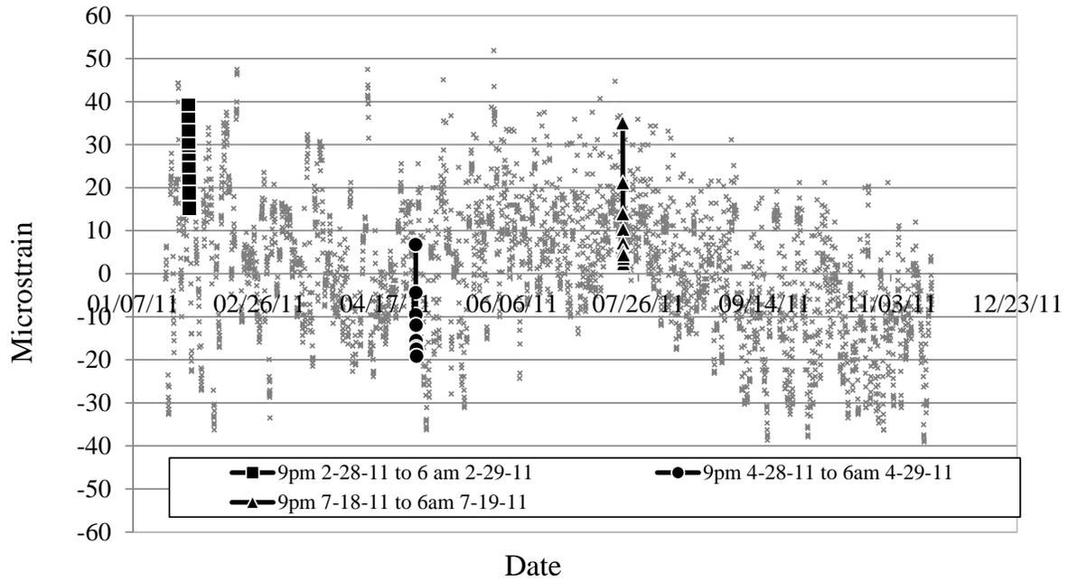
**Figure 6.11. Major axis bending versus time**
