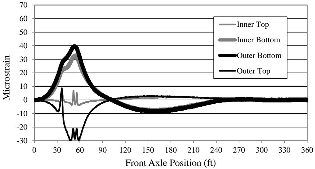
**Figure 7.6. Bridge 309-S2 Girder B strain (LP2)**
