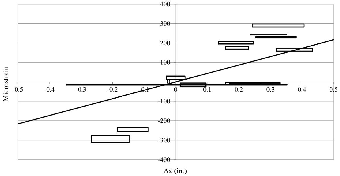
**Figure 6.103. SAHP6 weak axis bending strain versus displacement**
