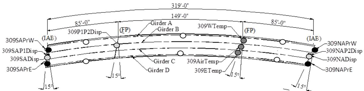
**Figure 5.23. Bridge 309 instrumentation**
