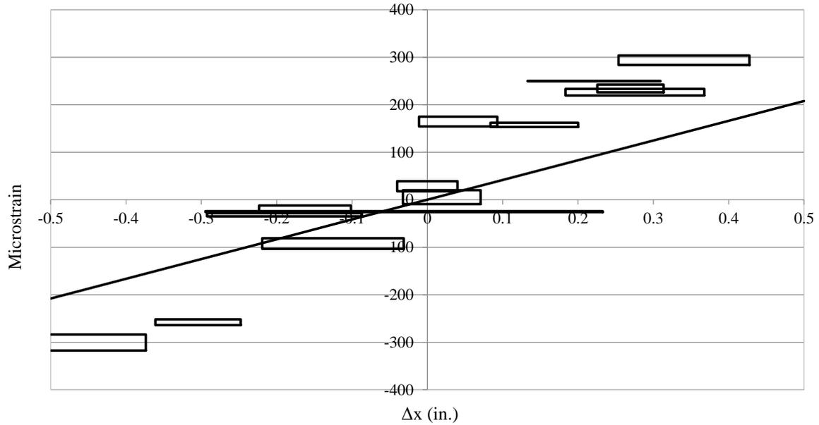
**Figure 6.105. NAHP4 weak axis bending strain versus displacement**
