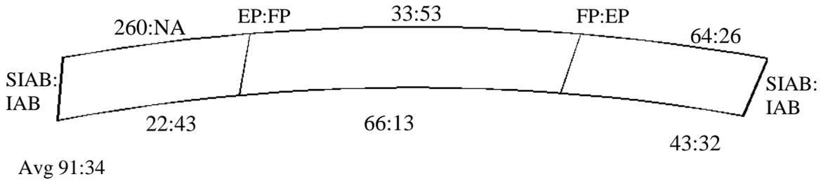
**Figure 6.38. Bridge 209:2208 lateral bending moment top flange**
