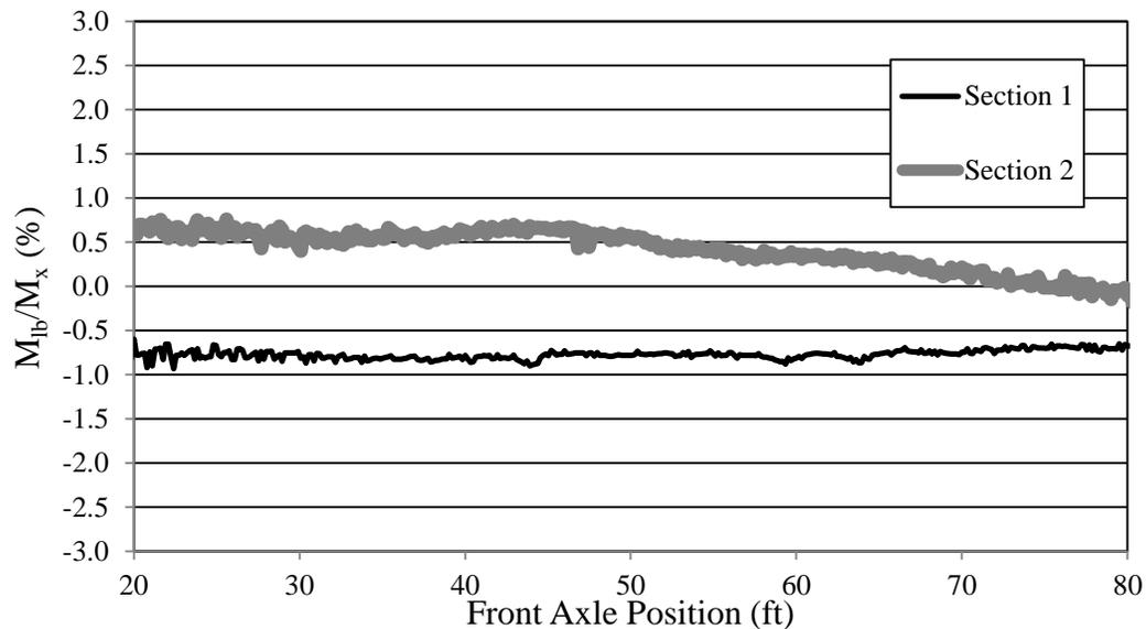
**Figure 7.38. Bridge 309 Girder A ratio of  $M_{lb}/M_x$**
