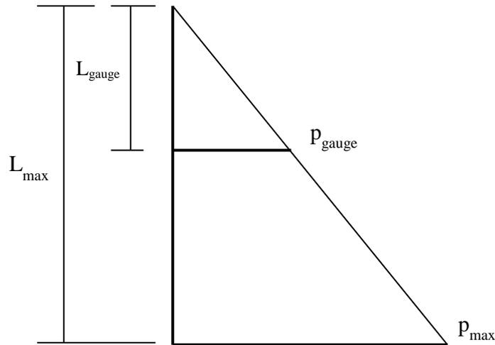
**Figure 6.52. Assumed backfill passive stress distribution**
