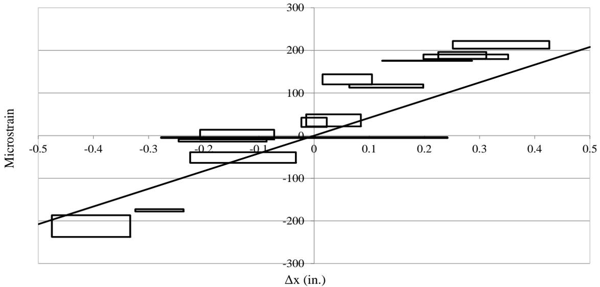
**Figure 6.101. SAHP1 weak axis bending strain versus displacement**
