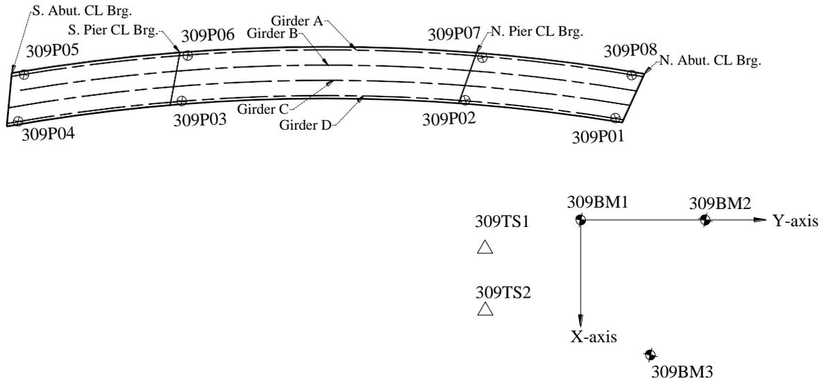
**Figure 5.28. Bridge 309 reflector, TS, and BM locations**
