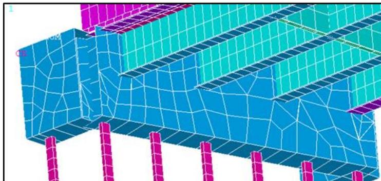
**Figure 8.10. Meshed girders and abutment**
