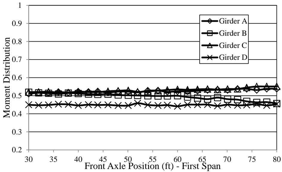
**Figure 7.35. Bridge 309-S2 moment distributions versus truck position**
