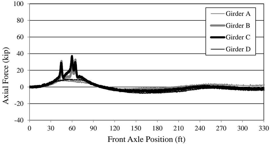
**Figure 7.27. Bridge 309-S1 axial forces in girders (LP3)**
