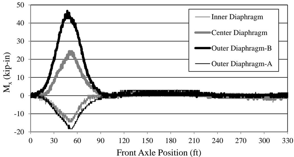
**Figure 7.29. Bridge 309 strong axis moments in diaphragms (LP3)**
