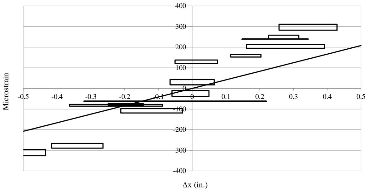
**Figure 6.104. NAHP1 weak axis bending strain versus displacement**
