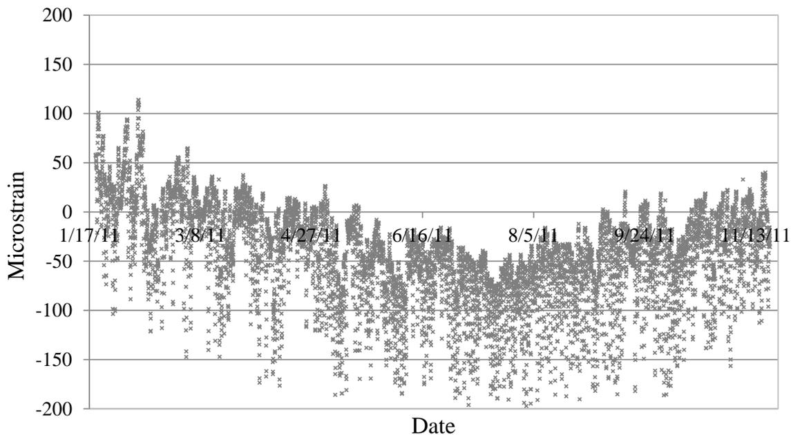
**Figure 6.6. Bottom flange east strain gauge reading**
