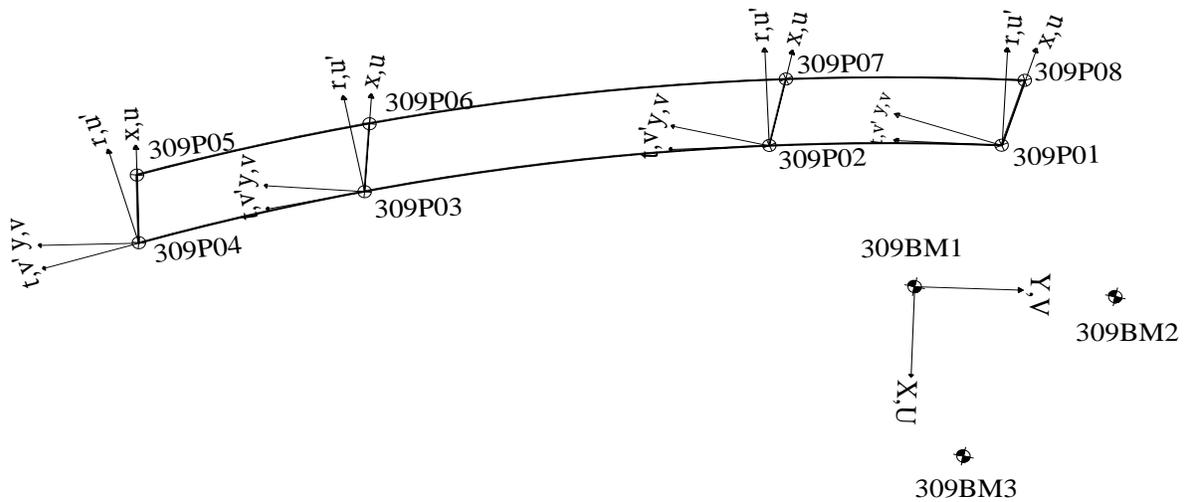
**Figure 6.53. Local abutment and pier coordinate systems**
