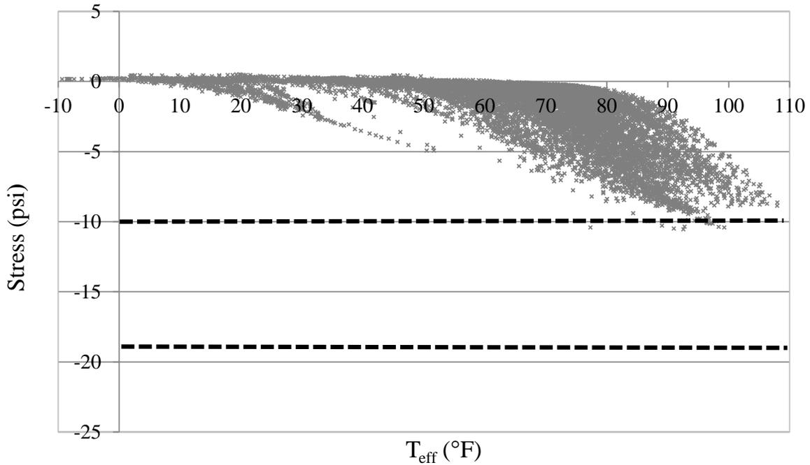
**Figure 6.50. Southwest abutment backwall pressure versus effective temperature**
