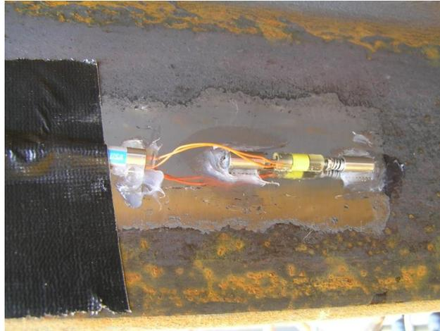
**Figure 5.17. Vibrating-wire strain gauge**
