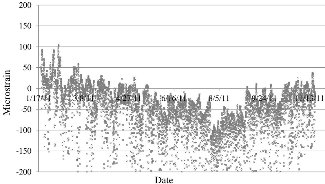
**Figure 6.9. Bottom flange west strain gauge reading**
