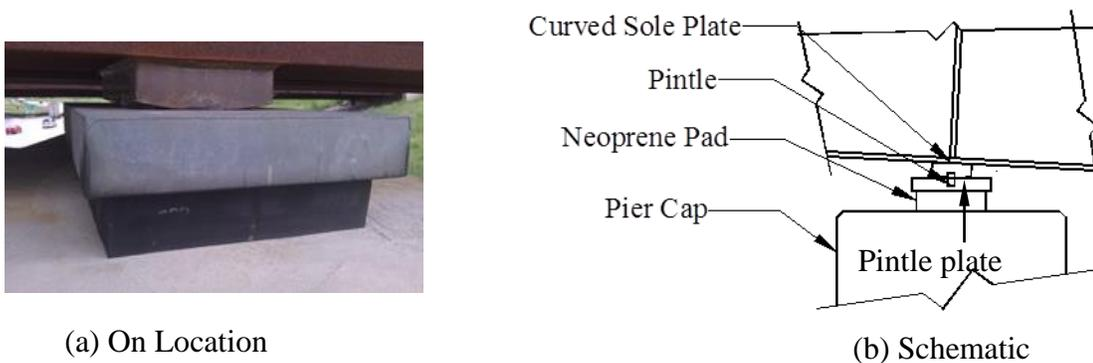
**Figure 5.10. Expansion pier bearing**
