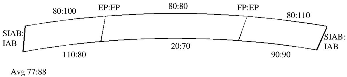
**Figure 6.23. Bridge 209:2208 strong axis bending strain range**
