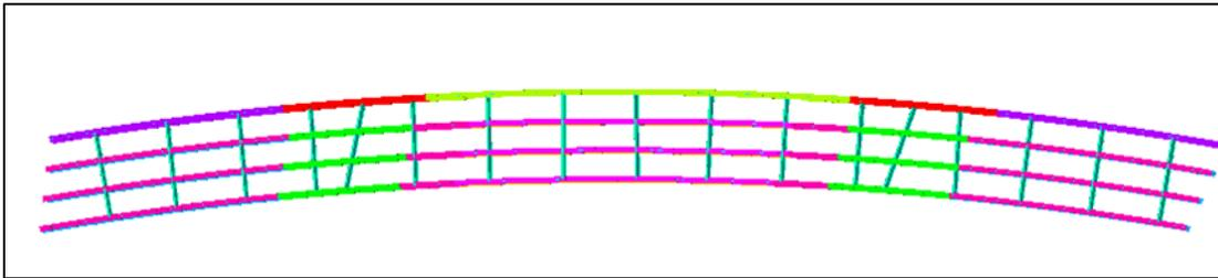
**Figure 8.8. Meshed changes in girder bottom flange thicknesses**
