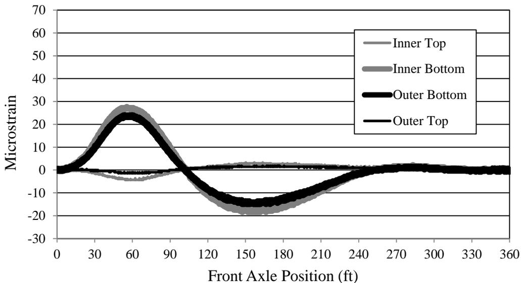
Figure 7.1. Bridge 309-S1 Girder A strain (LP2)
