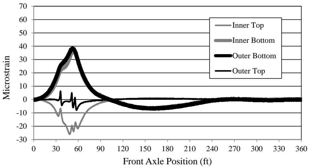
**Figure 7.7. Bridge 309-S2 Girder C strain (LP2)**
