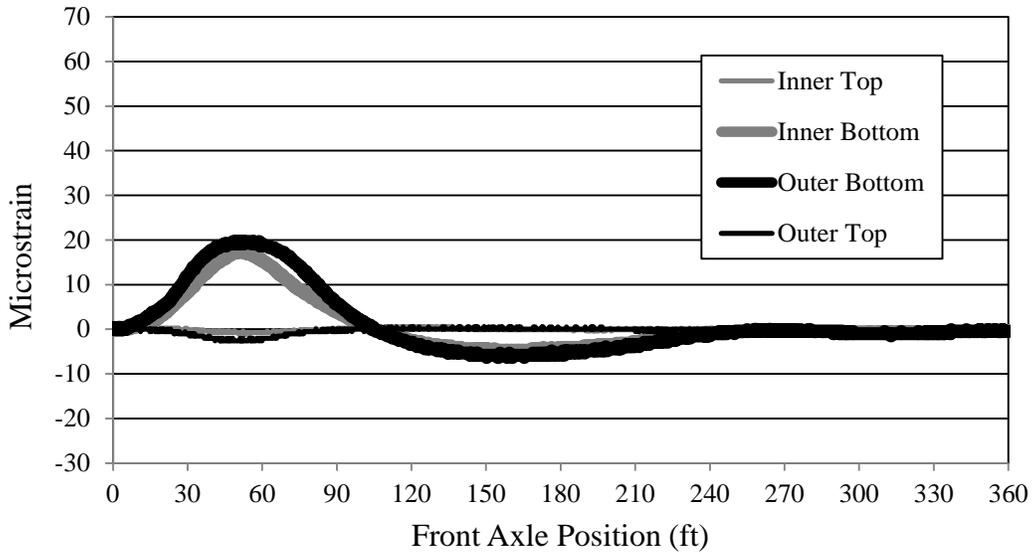
**Figure 7.8. Bridge 309-S2 Girder D strain (LP2)**
