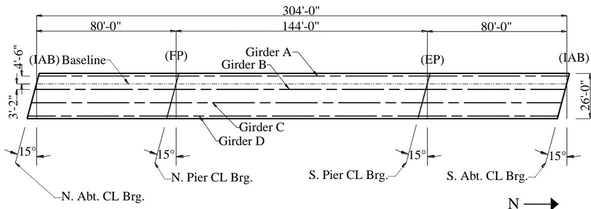
**Figure 5.7. Bridge 2408 plan view**
