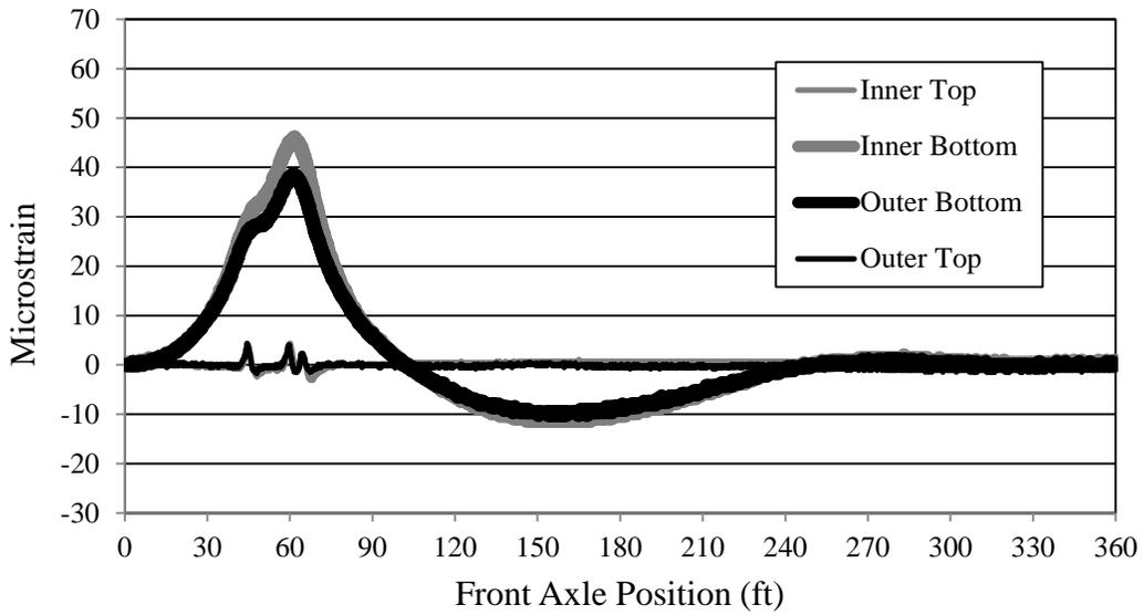
**Figure 7.3. Bridge 309-S1 Girder C strain (LP2)**
