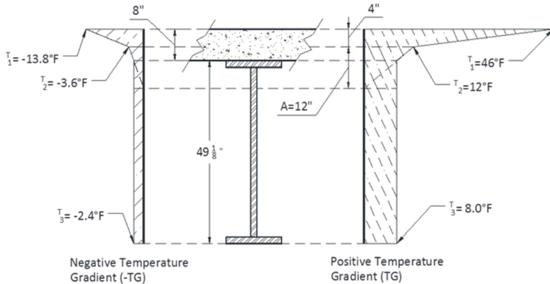
**Figure 8.25. Temperature gradient**
