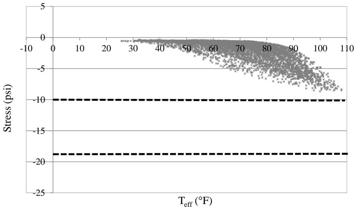
**Figure 6.48. Northwest abutment backwall pressure versus effective temperature**
