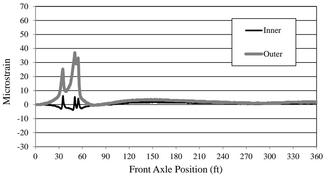
**Figure 7.12. Girder B-S2 top flange strain (LP3)**
