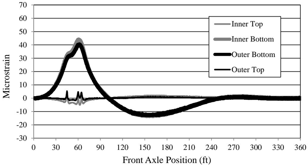
**Figure 7.2. Bridge 309-S1 Girder B strain for (LP2)**
