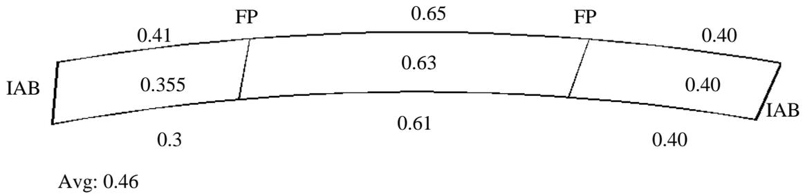
**Figure 6.62. Bridge 309 change in length per span**
