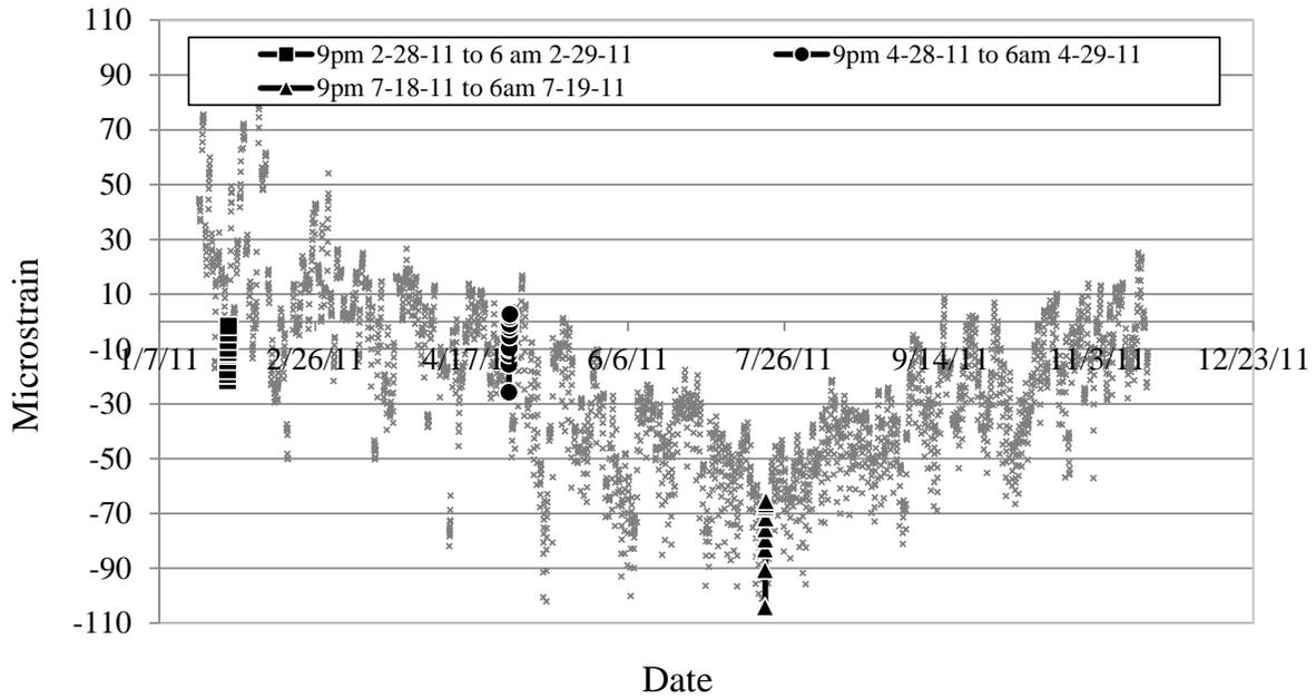
**Figure 6.10. Axial strain versus time**
