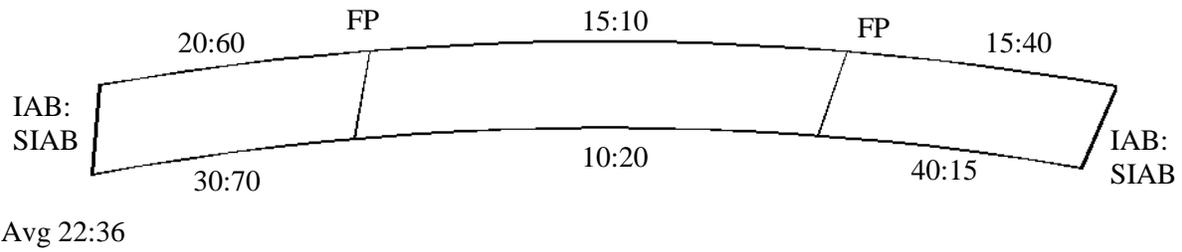
**Figure 6.25. Bridge 309:2308 lateral bending strain top flange**
