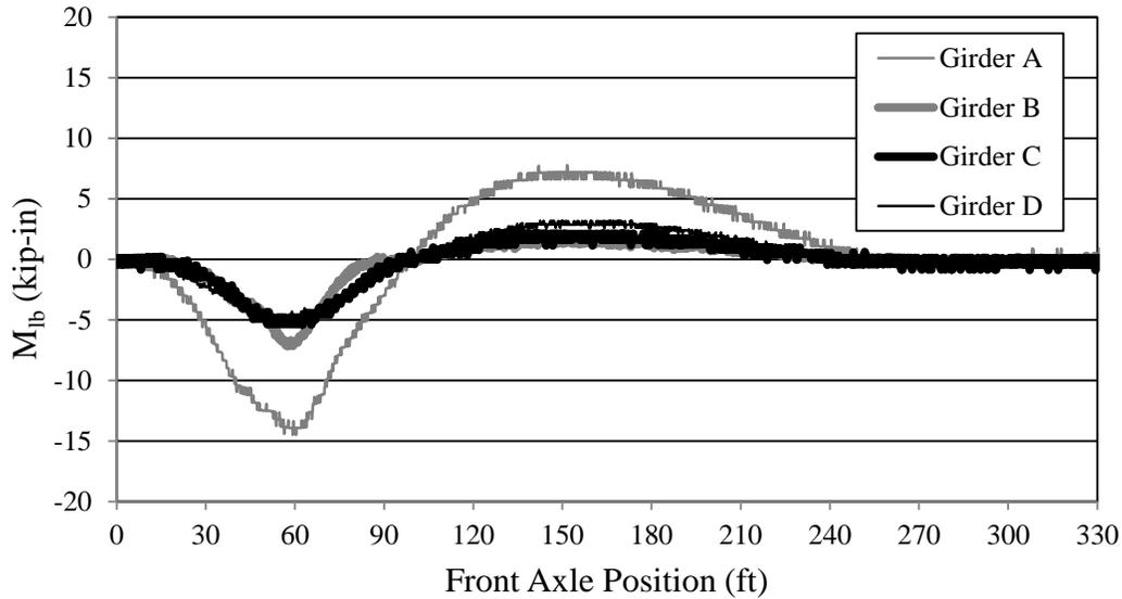
**Figure 7.24. Bridge 309-S1 lateral bottom flange moments (LP3)**
