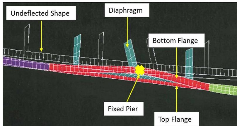
**Figure 8.31. Girder A deflected shape due to T(+)**
