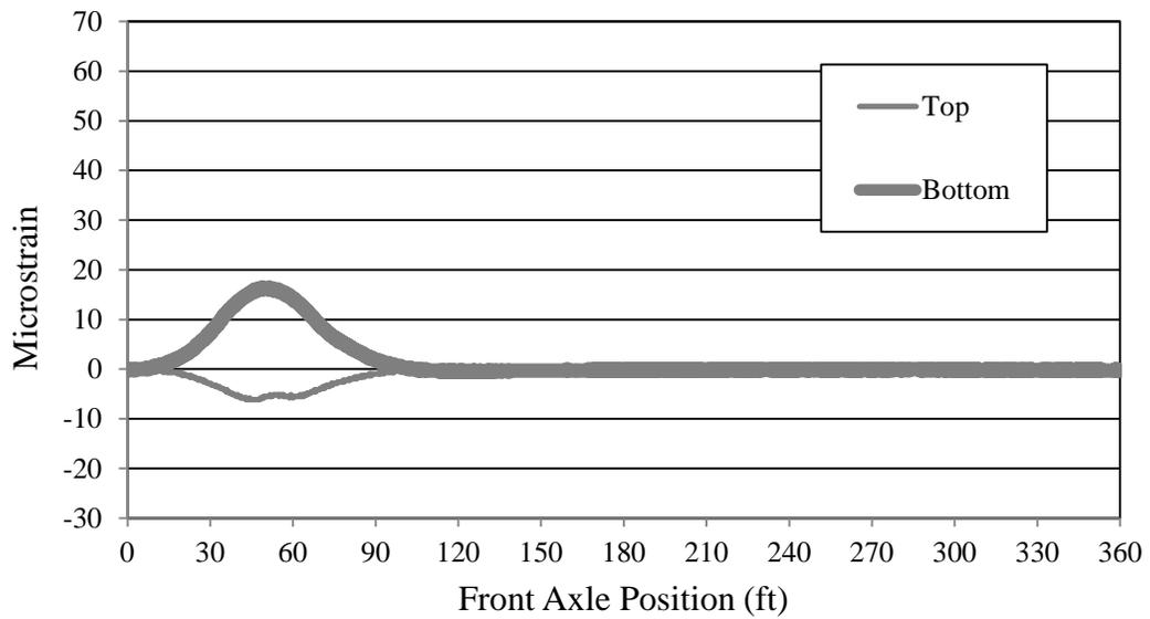
**Figure 7.14. Bridge 309 center diaphragm strain (LP2)**
