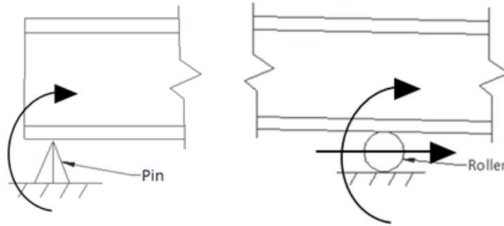
**Figure 8.12. Simply supported abutment (left) and pier (right)**
