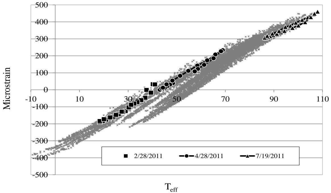
**Figure 6.46. Typical internal minor axis bending strain**
