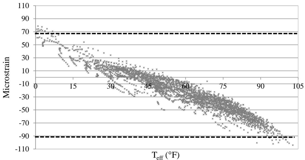
**Figure 6.18. Strain range calculation – axial strain example**
