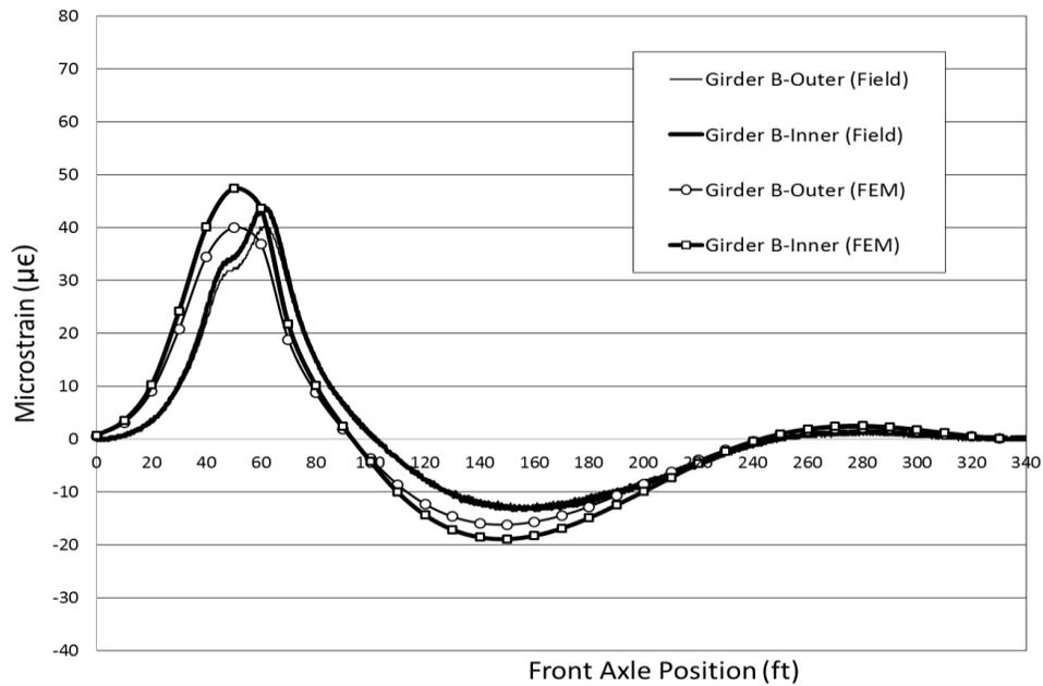
**Figure 8.15. Center path at Section 1 Girder B**
