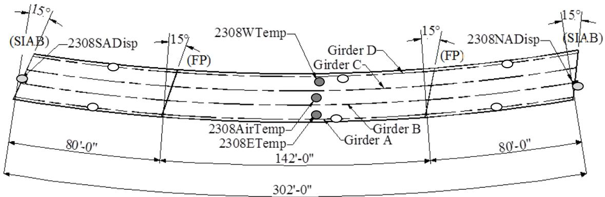
**Figure 5.25. Bridge 2308 instrumentation**
