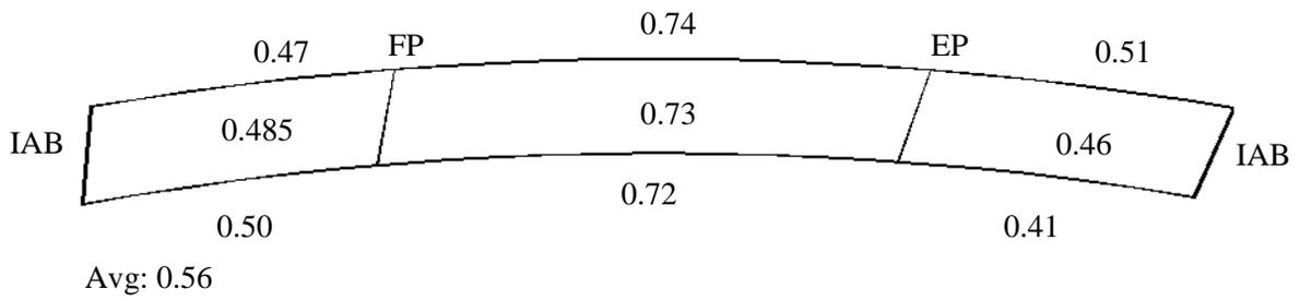
**Figure 6.63. Bridge 2208 change in length per span**
