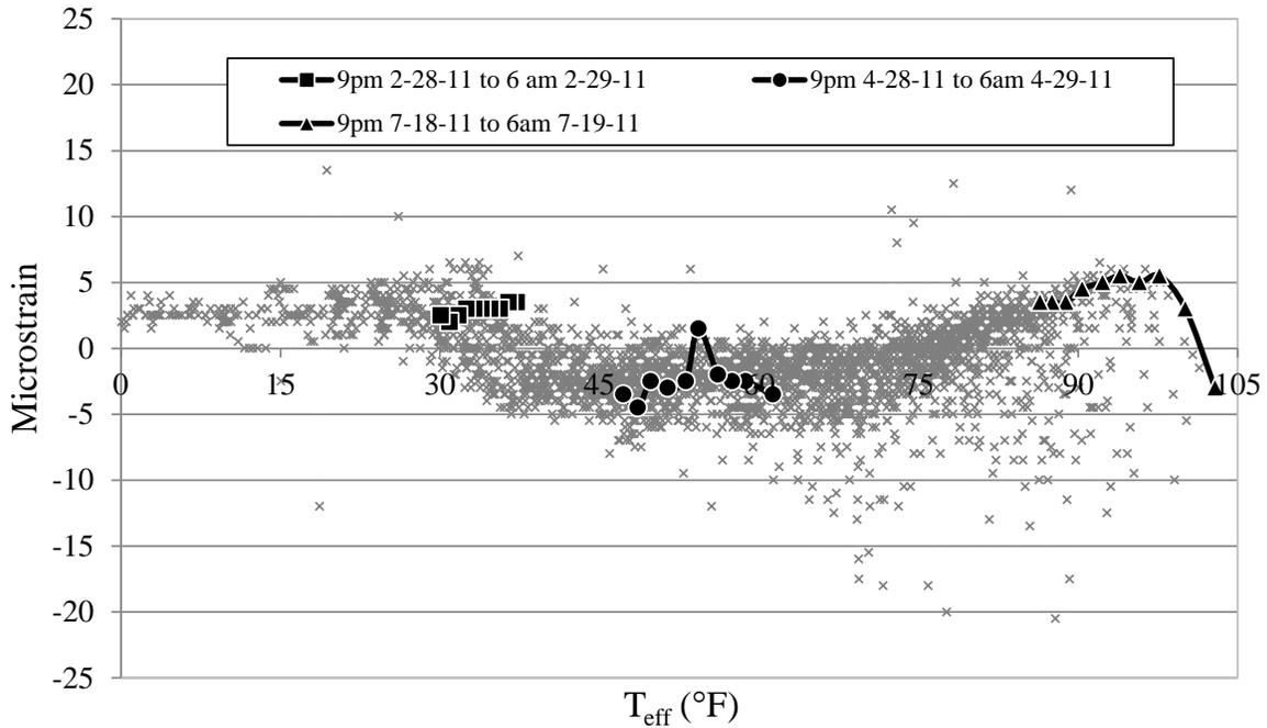
**Figure 6.16. Top flange lateral bending versus  $T_{eff}$**
