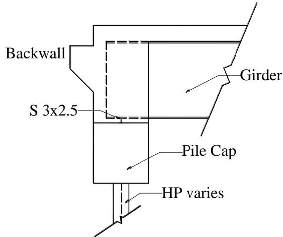
**Figure 5.13. Integral abutment Section A-A**
