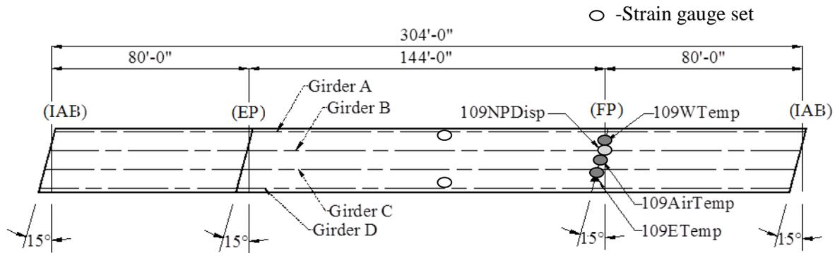
**Figure 5.21. Bridge 109 instrumentation**
