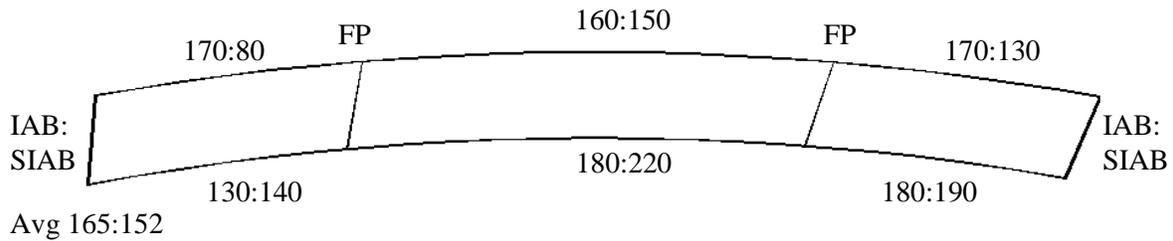
**Figure 6.19. Bridge 309:2308 axial strain range**
