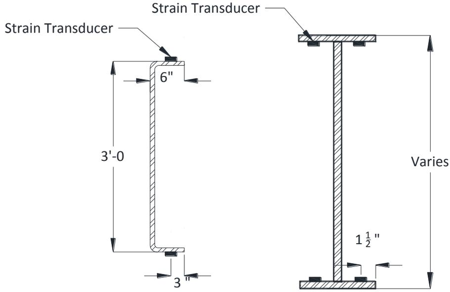
**Figure 5.37. I-girder and diaphragm strain transducer detail**
