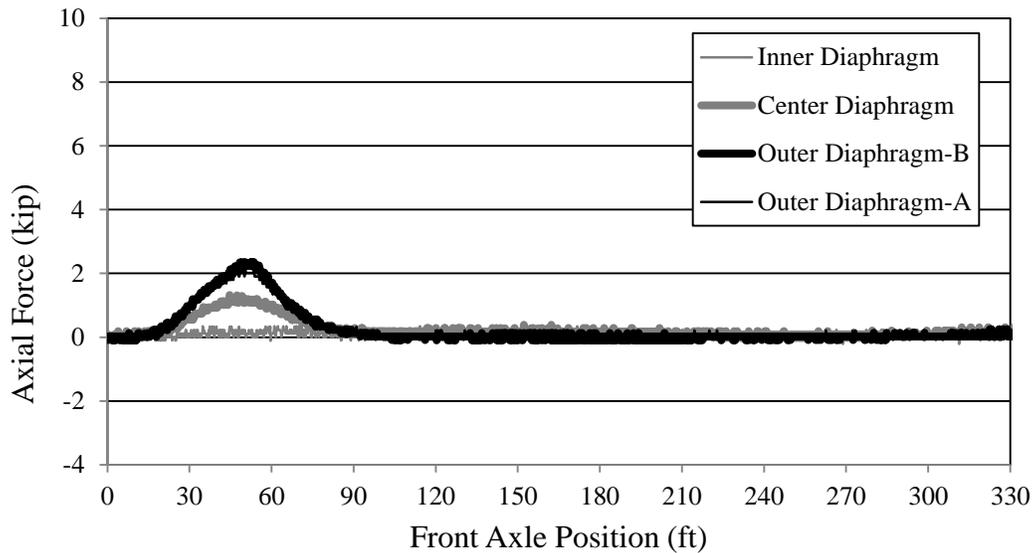
**Figure 7.30. Bridge 309 axial forces in diaphragms (LP3)**
