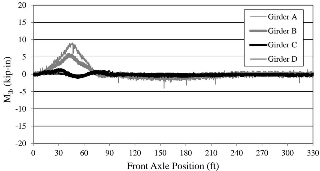
**Figure 7.25. Bridge 309-S2 lateral bottom flange moments (LP3)**
