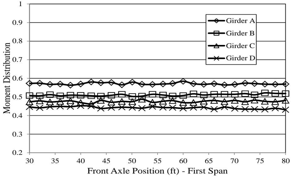
**Figure 7.34. Bridge 309-S1 moment distributions versus truck position**
