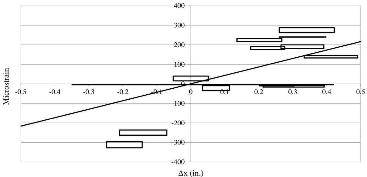
**Figure 6.102. SAHP4 weak axis bending strain versus displacement**
