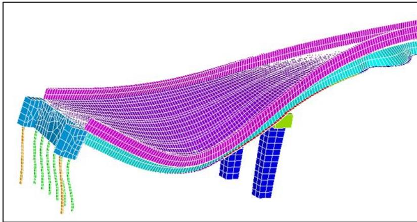
**Figure 8.13. Deflected shape for outer truck position**
