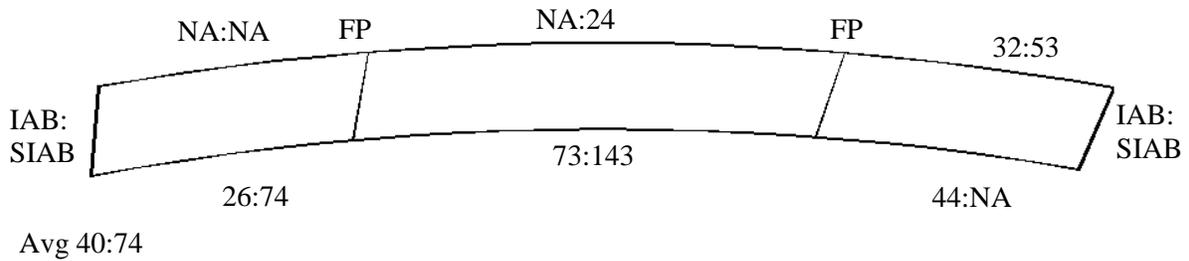
**Figure 6.40. Bridge 309:2308 lateral bending strain bottom flange**
