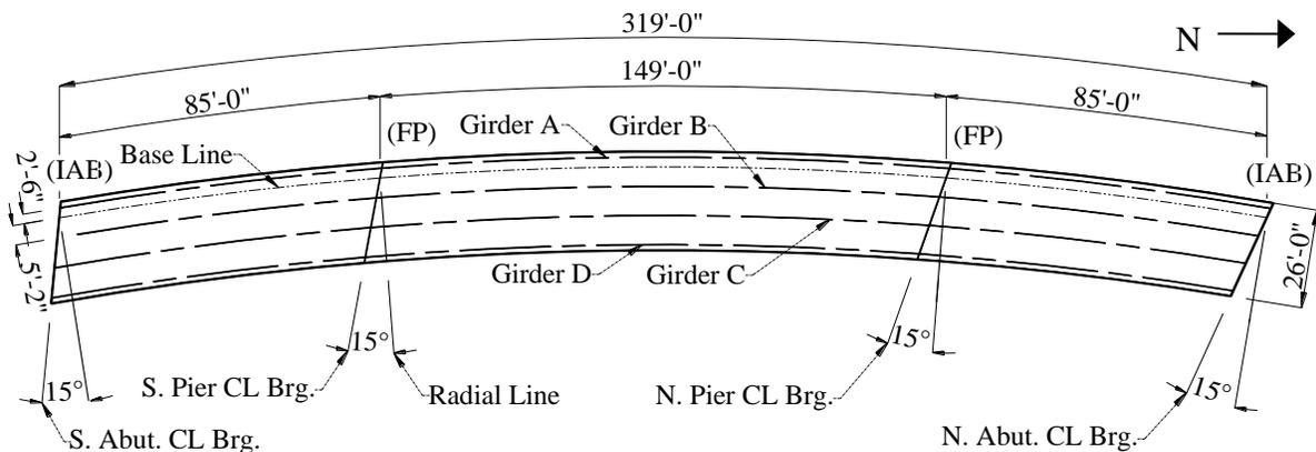
**Figure 5.4. Bridge 309 plan view**
