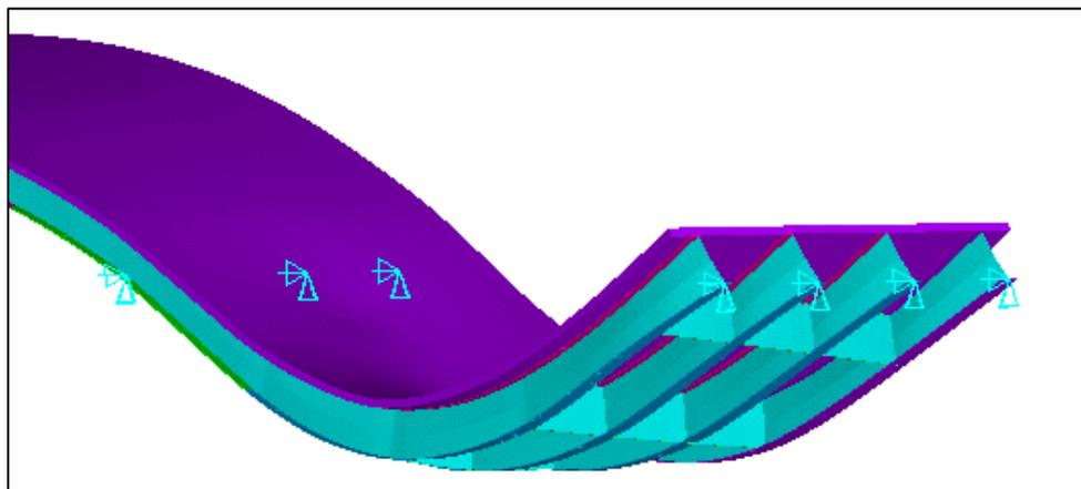
**Figure 8.17. Deflected shape for center truck position**
