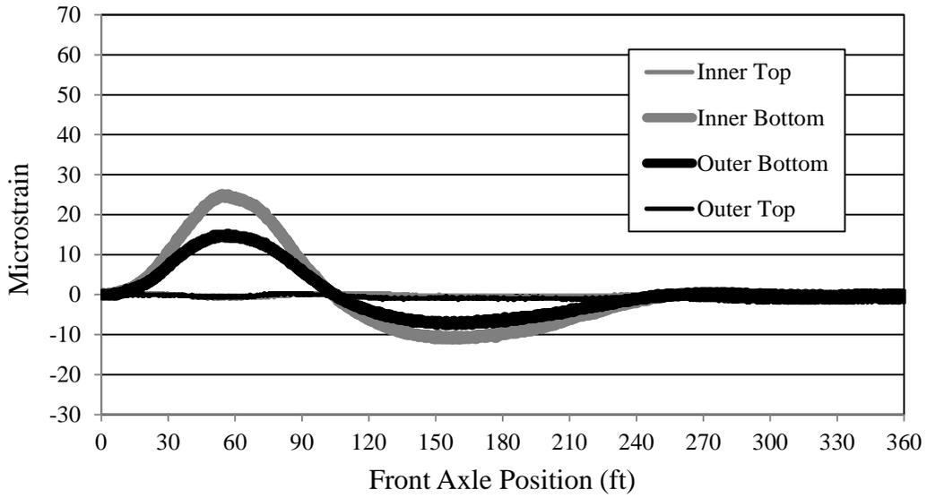
**Figure 7.4. Bridge 309-S1 Girder D strain (LP2)**
