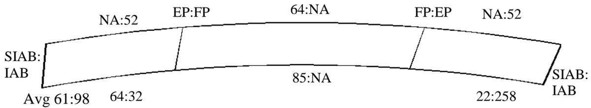
**Figure 6.41. Bridge 209:2208 lateral bending strain bottom flange**
