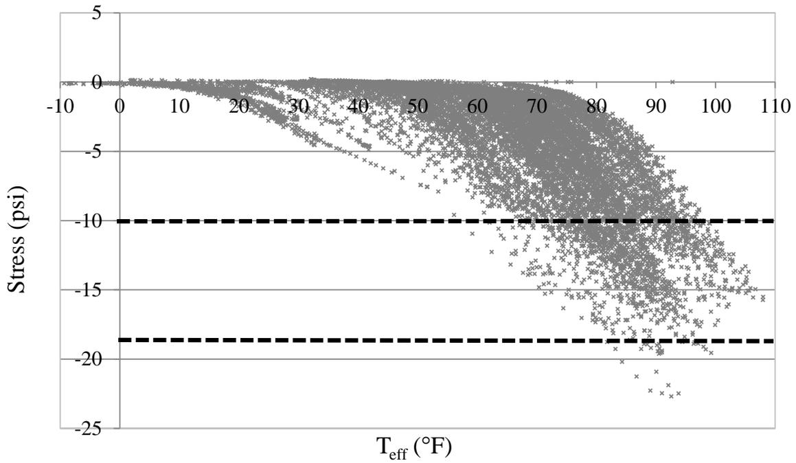
**Figure 6.49. Northeast abutment backwall pressure versus effective temperature**
