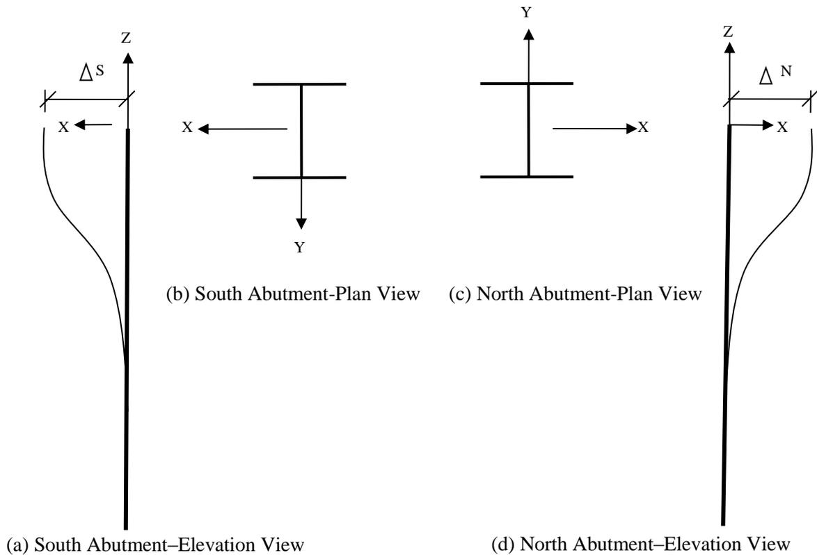
**Figure 5.16. Integral Abutment pile coordinate system for Bridge 309**
