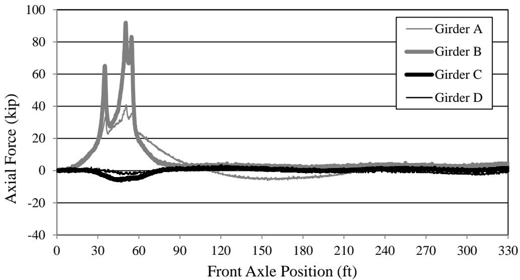
**Figure 7.28. Bridge 309-S2 axial forces in girders (LP3)**
