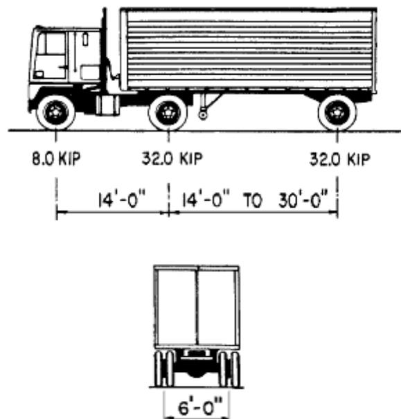
**Figure 8.23. Design truck specifications (from Figure 3.6.1.2.2-1 AASHTO 2010)**
