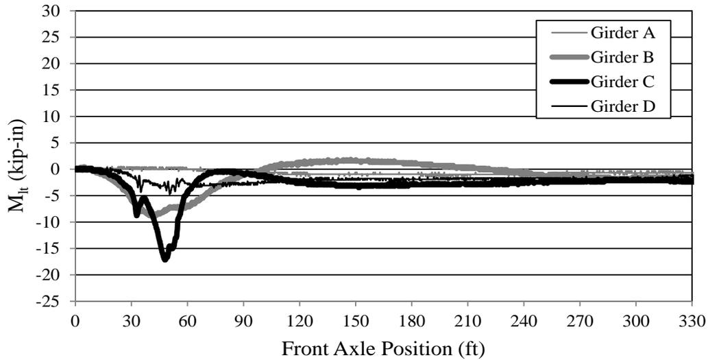
Figure 7.26. Bridge 309-S2 lateral top flange moments (LP3)
