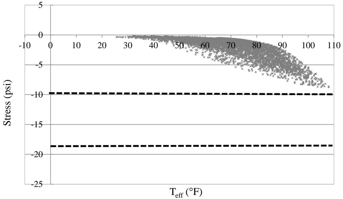
**Figure 6.51. Southeast abutment backwall pressure versus effective temperature**
