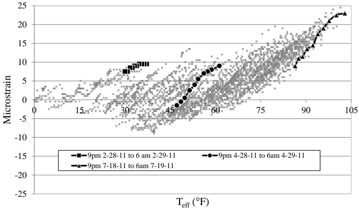
**Figure 6.17. Bottom flange lateral bending versus T<sub>eff</sub>**
