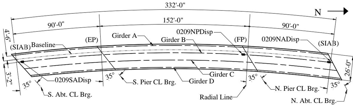
**Figure 5.3. Bridge 209 plan view**
