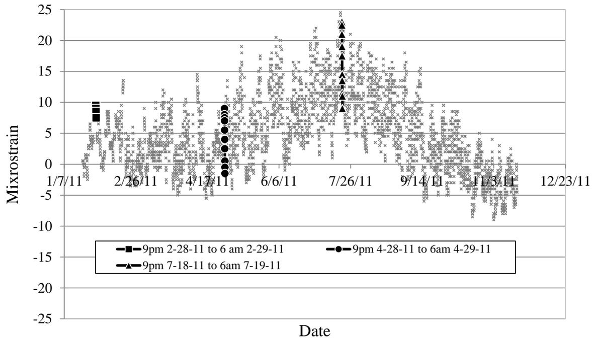
**Figure 6.13. Bottom flange lateral bending versus time**
