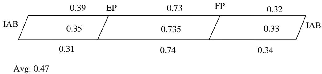
**Figure 6.65. Bridge 109 change in length per span**
