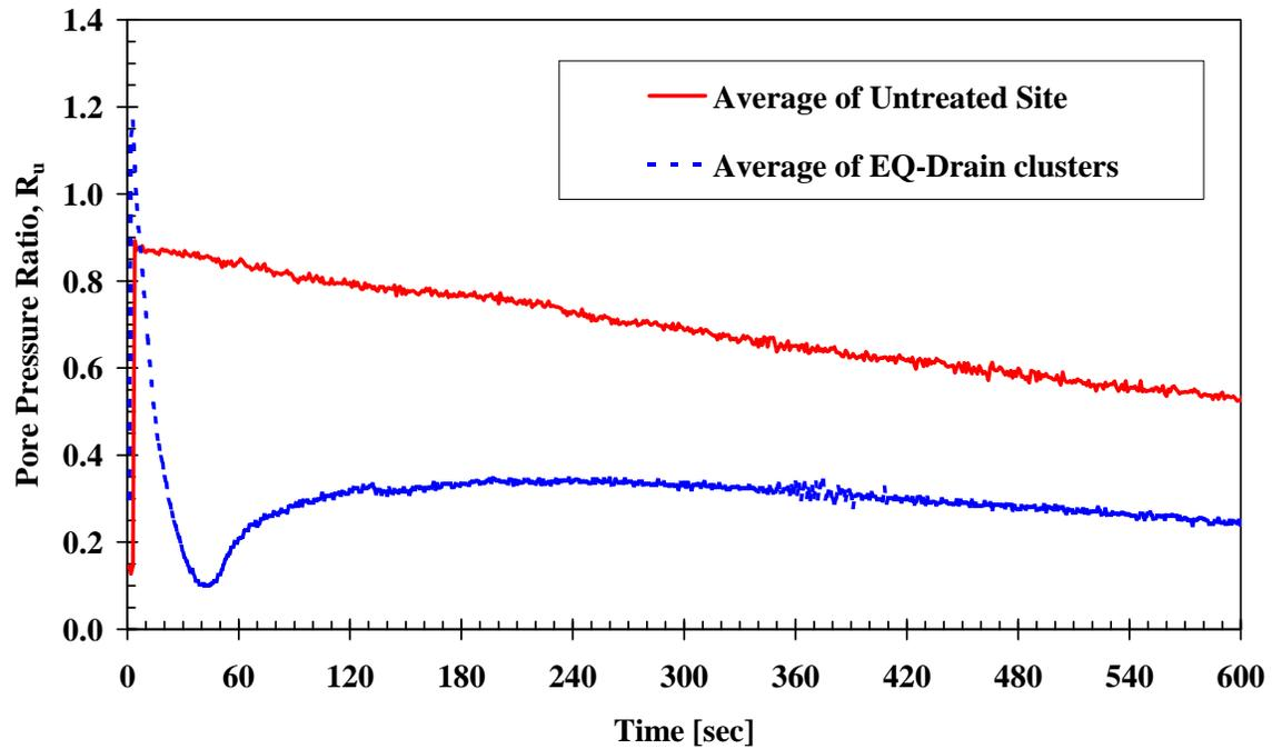
Fig. 3. Comparison of excess pore pressure ratio as a function of time at sites treated with EQ drains relative to an untreated test site (Rollins et al. 2003).
