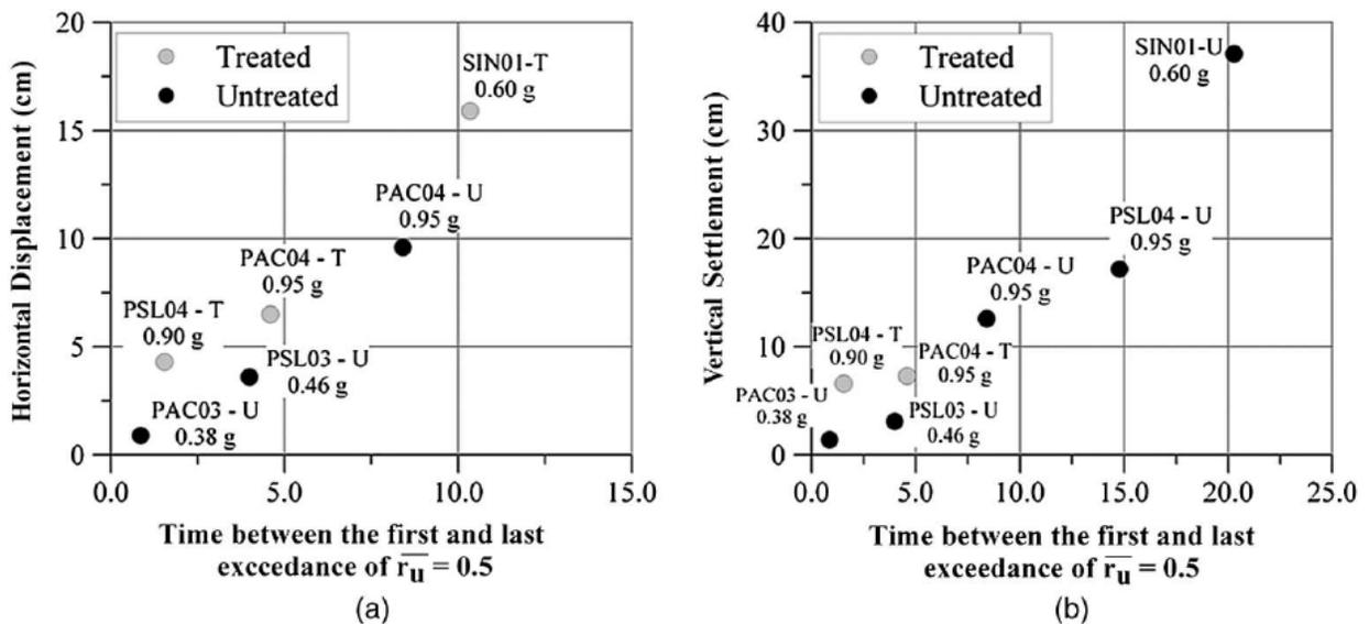
Fig. 13. Horizontal and vertical deformations at midslope in the untreated and treated areas: (a) horizontal displacement, (b) vertical displacements as a function of time between the first and last exceedance of  $r_u=0.5$ . (Howell et al. 2012).
