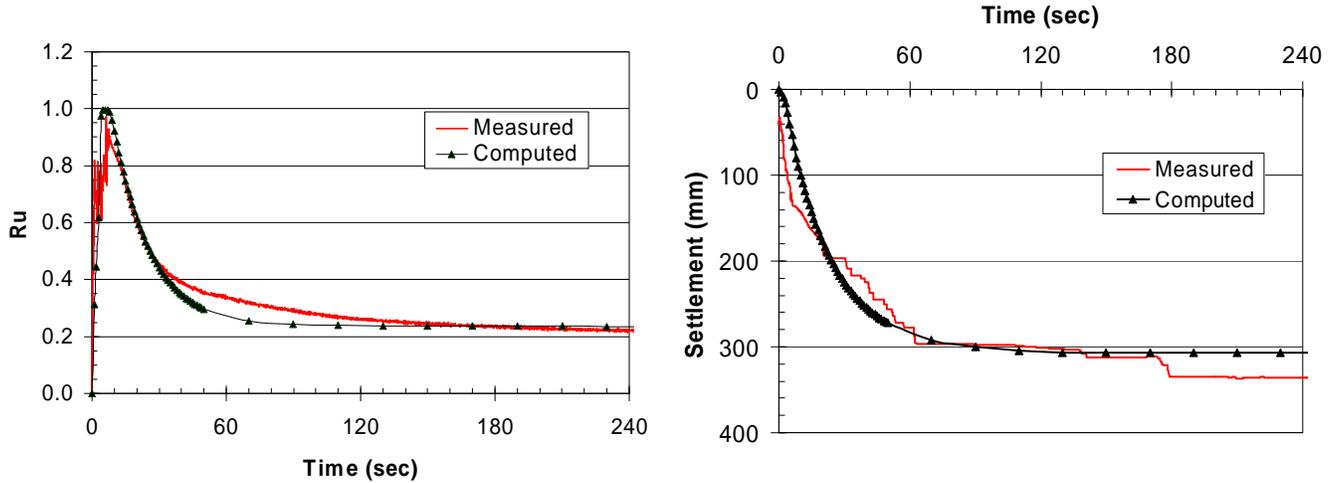
**Fig. 14 Comparison of (a) measured and computed excess pore pressure ratio ( $R_u$ ) versus time at a depth of 11.8 m and (b) measured and computed settlement versus time curves for the Vancouver test site. (Rollins et al, 2004).**
