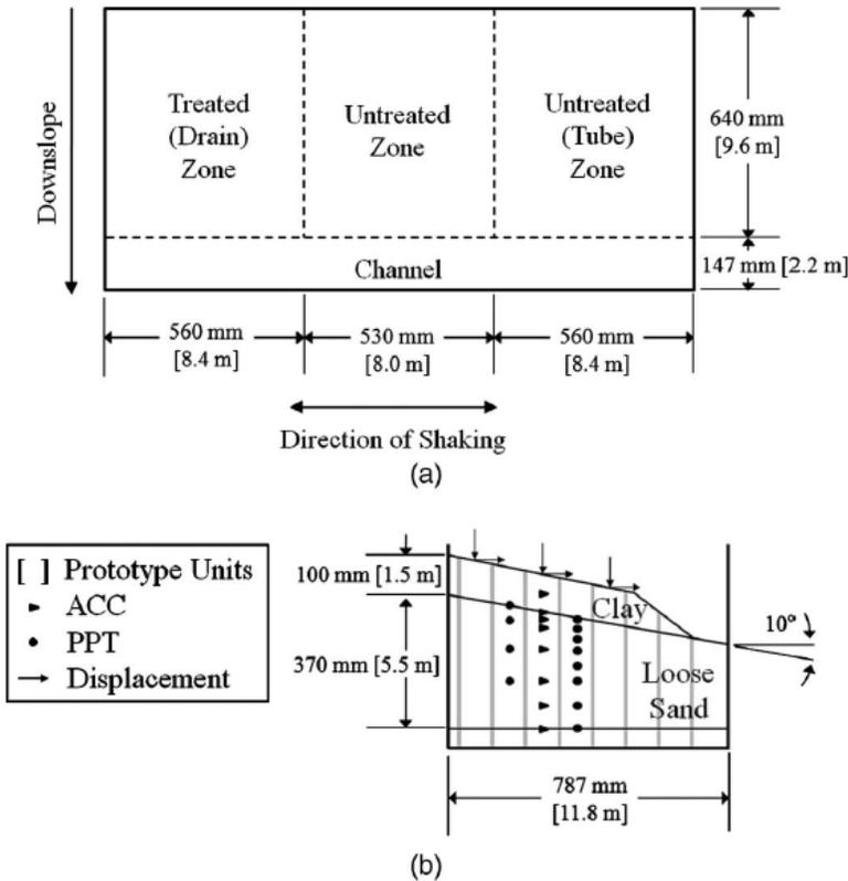
**Fig. 11. Layout for centrifuge test comparing behavior of slopes in liquefiable sand with and without vertical drains to mitigate liquefaction hazard: (a) plan; (b) cross section (Howell et al. 2012).**
