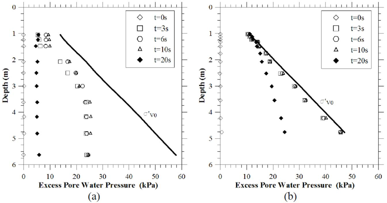
Figure 9. Excess pore water pressure profile for varying times for PGA=0.28g event for (a) treated and (b) untreated sides. (Note: “t=0s” corresponds to the start of shaking.) (Marinucci et al 2008)
