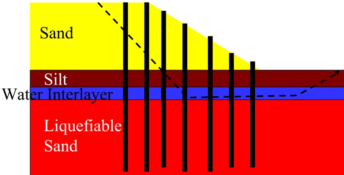
**Fig. 1. Schematic drawing showing the potential for vertical drains to relieve pore pressures and intercept water interlayers which may form below a low permeability silt layer thereby reducing the potential for slope instability and lateral spreading.**
