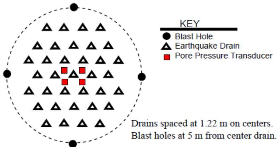
**Fig. 5. Layout of EQ drains, blast holes and pore pressure transducers to monitor effectiveness of drains for liquefaction remediation.**
