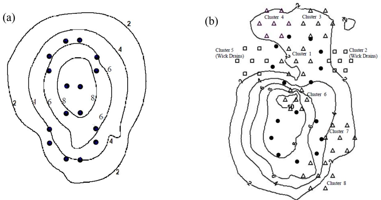
Fig. 4. Contours of measured settlement (in cm) for (a) untreated site and (b) site treated with clusters of EQ drains after detonation of 16 explosive charges around two 4.3 m diameter rings. Rollins et al, (2003).
