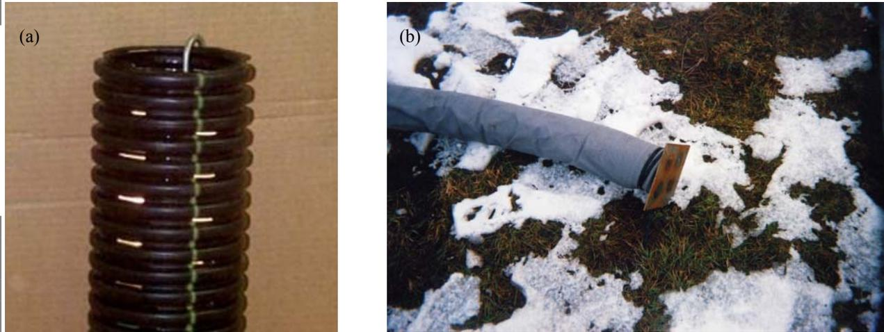
**Fig. 2. (a) EQ Drain without filter fabric showing slots illuminated by light inside pipe and (b) EQ Drain with filter fabric and anchor plate at the end (Rollins et al, 2004).**
