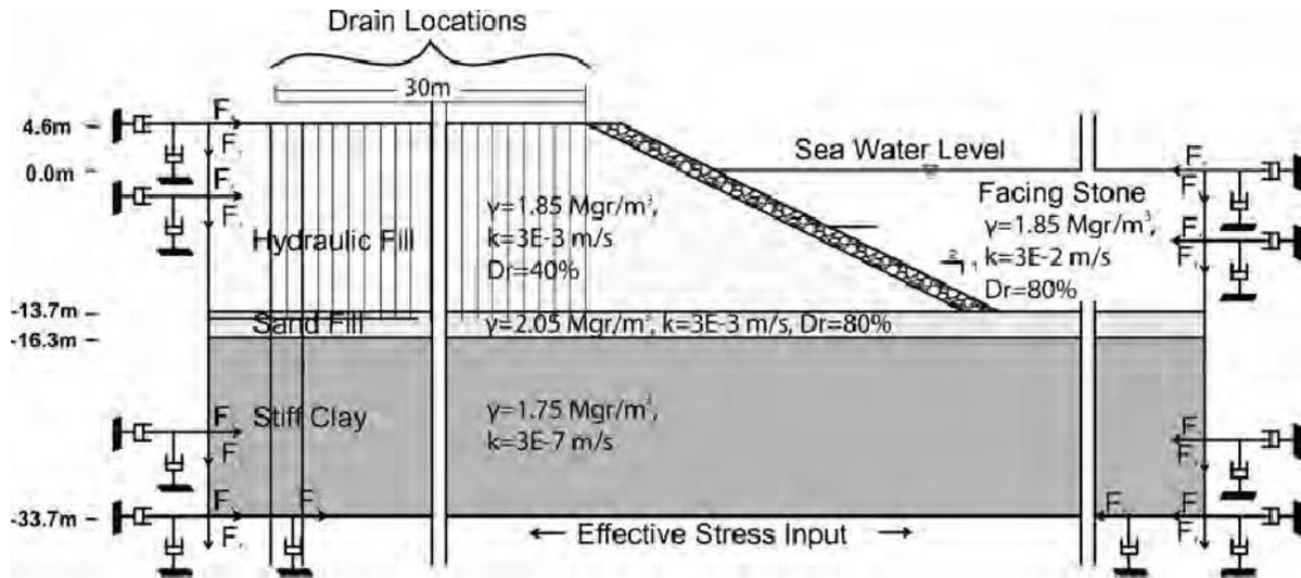
Figure 15. Analyzed section with details of the properties of the finite element numerical model (Vytiniotis et al. 2013).
